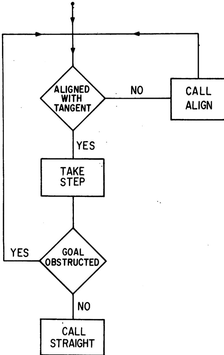
Fig. 6. Flowchart for subalgorithm HUG.
