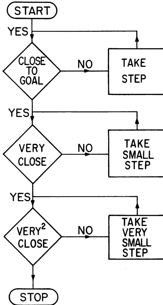
Fig. 7. Flowchart for subalgorithm STRAIGHT.
