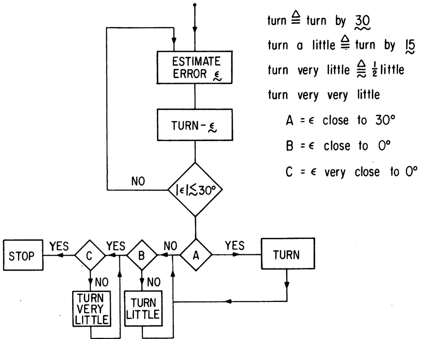
Fig. 5. Flowchart for subalgorithm ALIGN.
