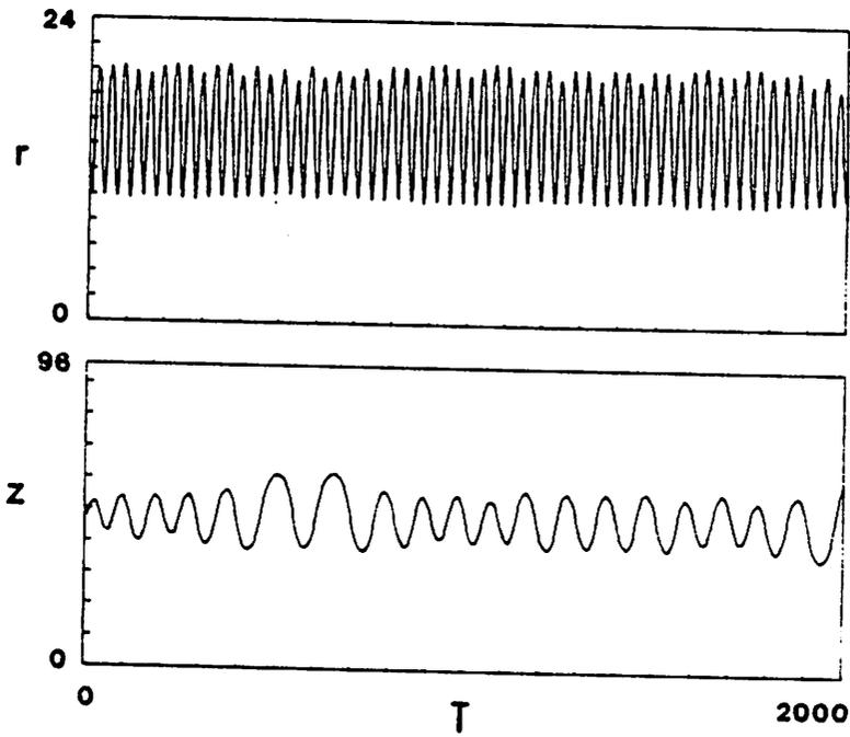
15. Expanded  $r$  and  $z$  histories for the ergodic particle of figs. 9 and 10.
