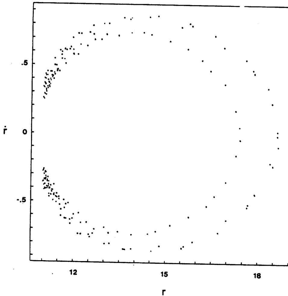
8. Another surface of section plot for the particle of fig. 6., but with diagnostics performed every timestep. Less spread in the pattern is evident.
