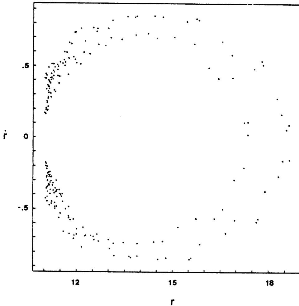
7. A surface of section plot for the particle of fig. 6, as described in the text. Diagnostics were performed every other timestep, and linear interpolation between these points was used. Note that points fall on a crescent but do not fill the area enclosed by the crescent.
