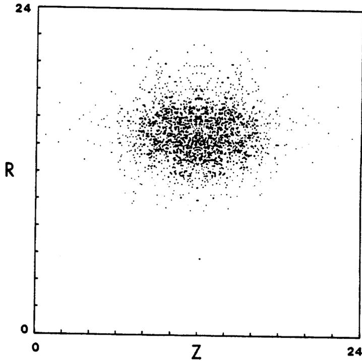
1a. Particle locations in the  $r - z$  plane at timestep 500.
