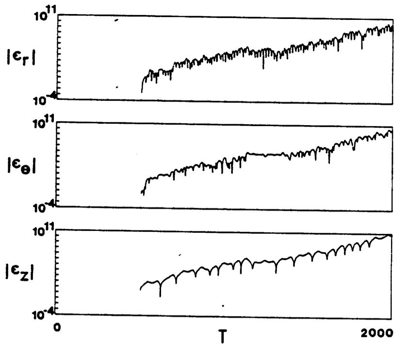
16. Time histories of the magnitudes of the  $r$ ,  $\theta$ , and  $z$  components of  $\underline{\epsilon}$  for the ergodic particle of figs. 9, 10, and 15. Noisy growth is evident.
