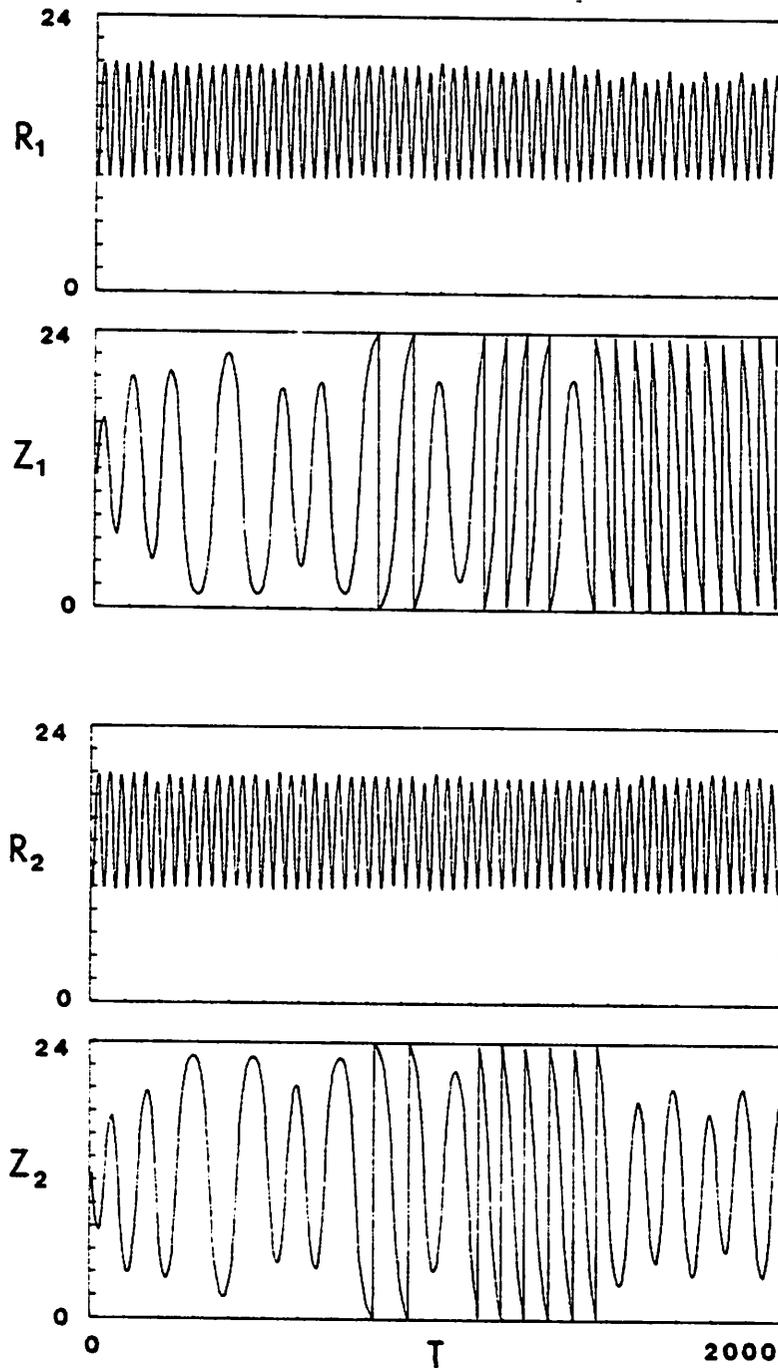
2. The orbits of a pair of particles which were initially a mirror image pair, selected from run JWA with  $\text{EPS} = 10^{-13}$ . The histories of  $r$  and  $z$  as functions of time are shown. Mirror symmetry about  $Z = L/2$  is evident until approximately timestep 1100.
