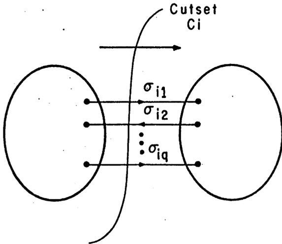
Figure 2 System separation on a cutset
