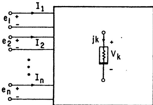
Figure 3 Nonlinear n-port resistive network
