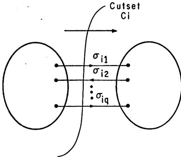
Figure 2 System separation on a cutset
