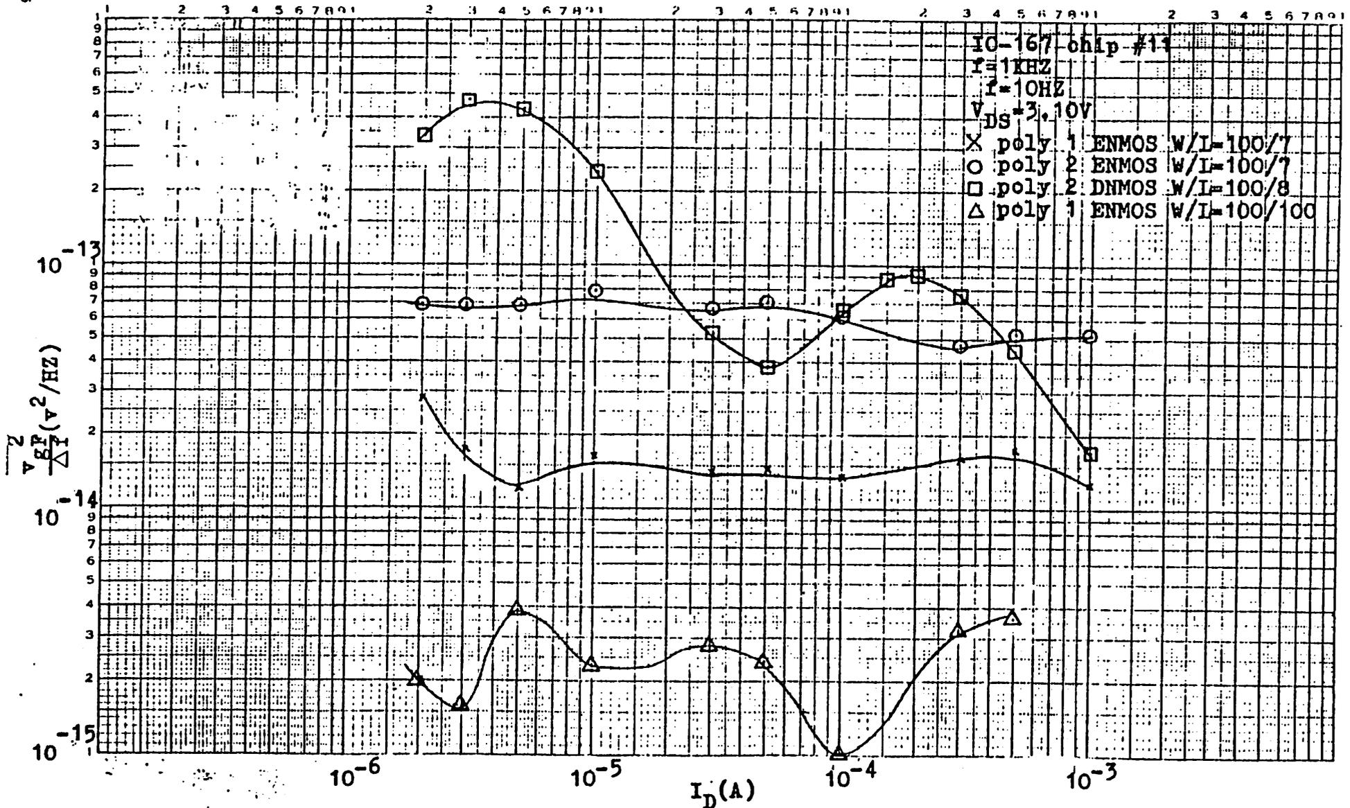
Fig.8a Experimental results on four NMOS's on the same chip showing the variation of the equivalent gate input noise voltage per unit bandwidth with drain current at 1KHZ
