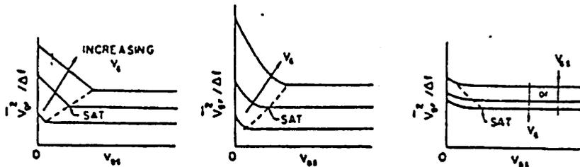
Fig.1 Qualitative representation of the variations of MOS equivalent gate-noise voltage per unit bandwidth, under three different distribution of  $N_{SS}$ , with drain voltage, assuming a constant effective gate-bias voltage [1].
