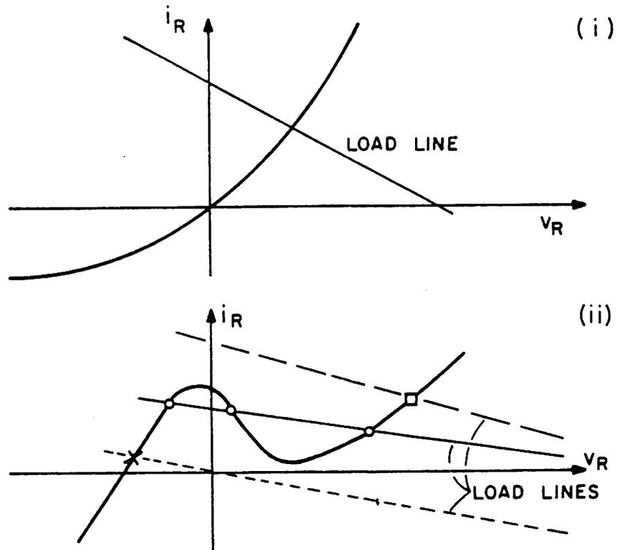
Figure 30. Illustrating multiple solutions arising from nonmonotone resistor characteristics.
