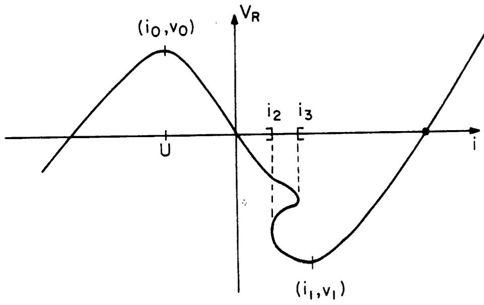
Figure 26. Resistor characteristic for circuit of Figure 1.
