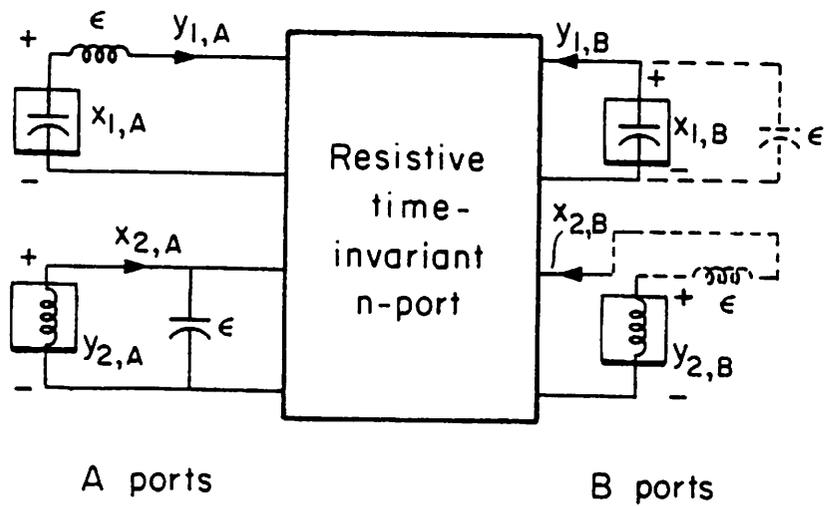
Figure 22. Nonlinear circuit with parasitics introduced.
