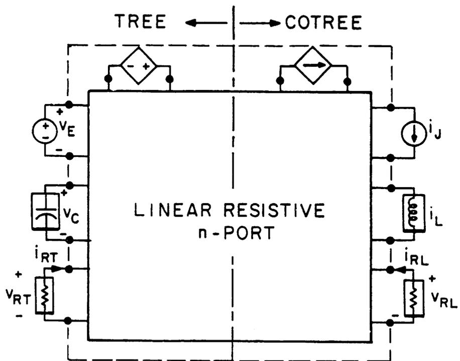
Figure 28. An n-port  $N$  created by extracting all independent sources and nonlinear elements.
