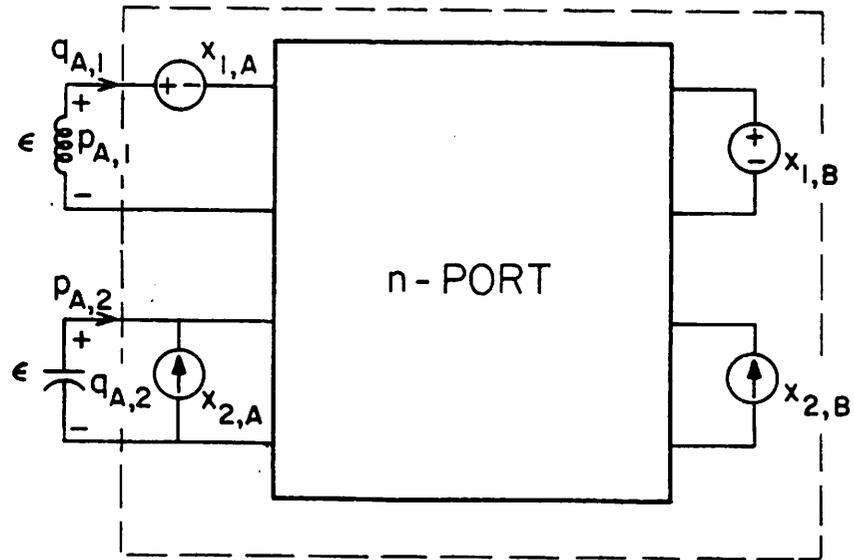
Figure 23. The  $n_A$  port associated with the parasitics with the larger capacitors and inductors frozen.
