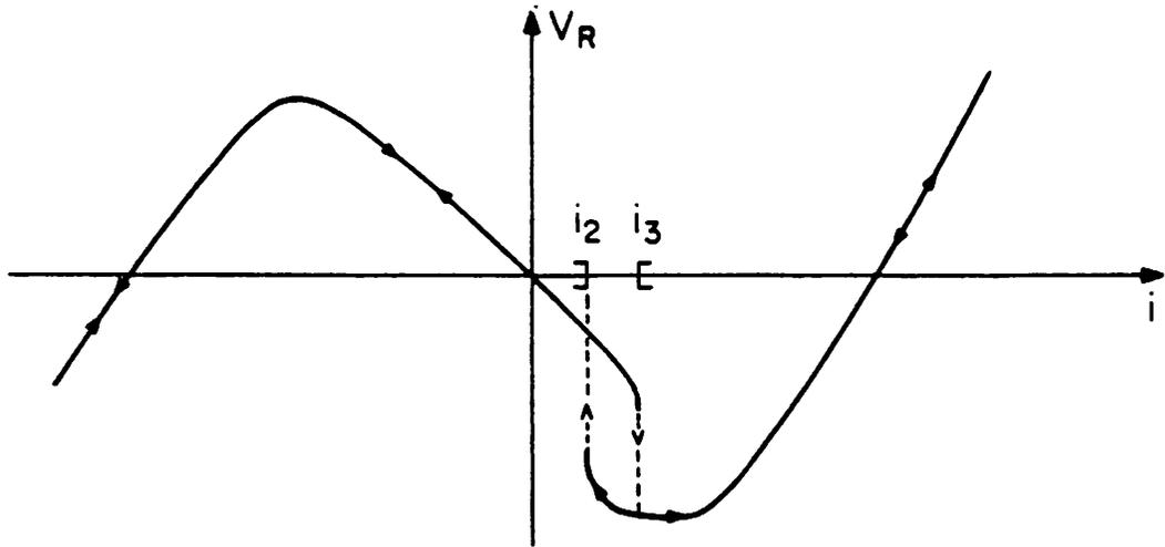
Figure 27. Hysteretic characteristic of resistor shown in Figure 26.
