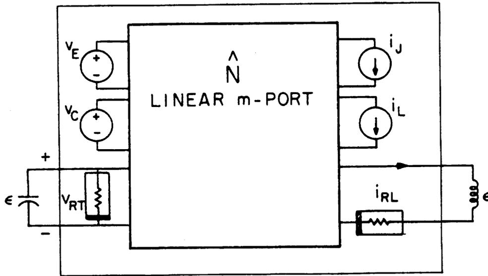
Figure 29. Parasitic augmentation to get circuit equations in normal form.
