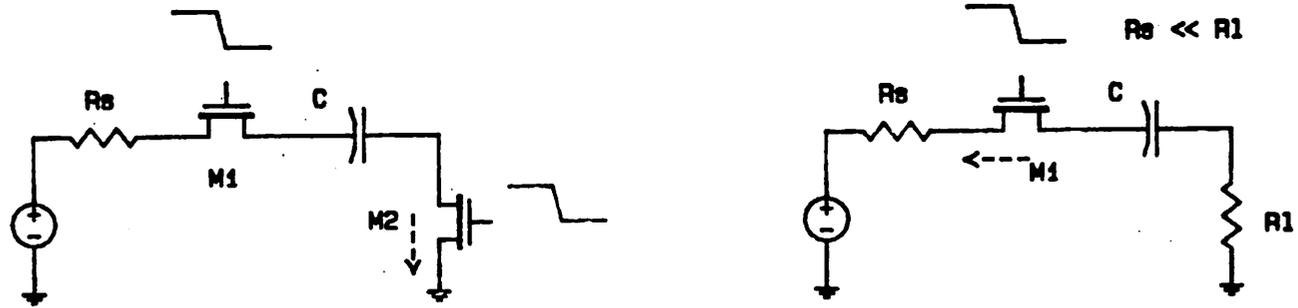
Fig.4.16 Input Switch Channel Charge Injection
