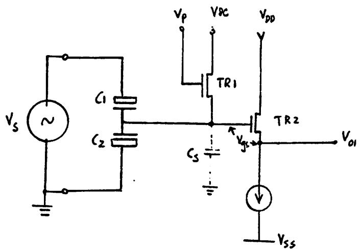
FIG 5.1 On-Chip Capacitance Ratio Measuring Technique
