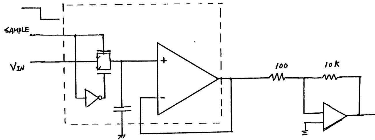
Figure 9-2 Test Setup for Charge Injection Measurement
