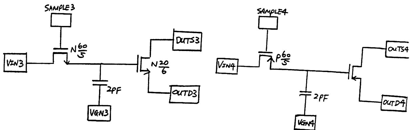
Fig. 10-1 Current mirrors and charge injection without Op-amp
