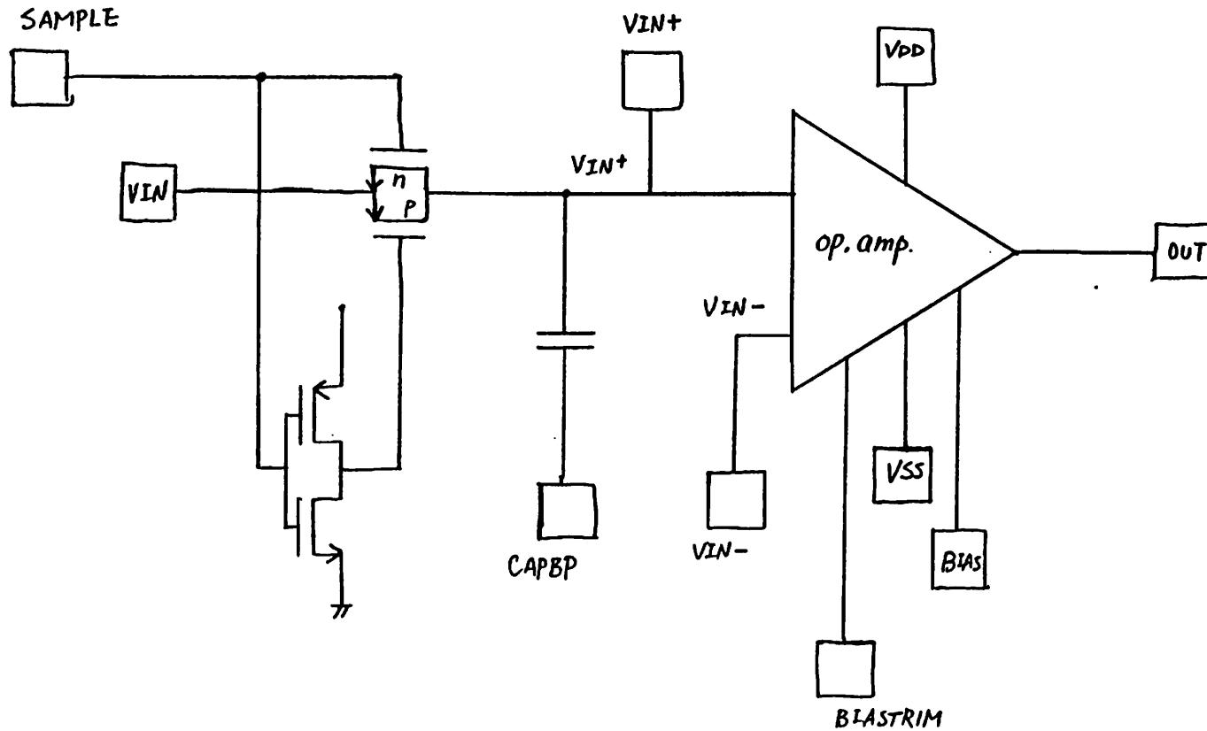
Figure 9-1. Charge Injection Circuit Schematic
