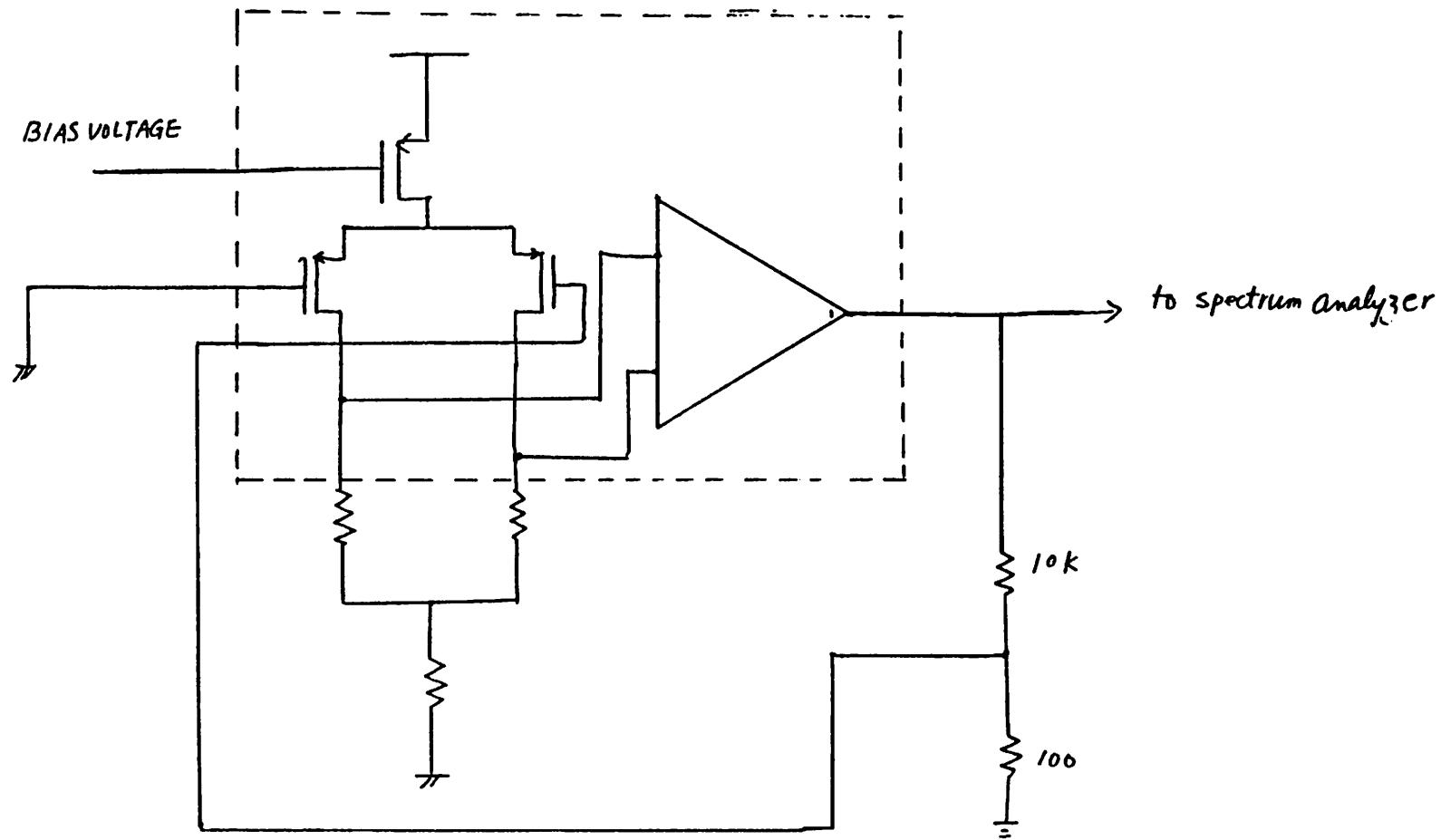
Figure 8-2. Noise Measurement Test Setup
