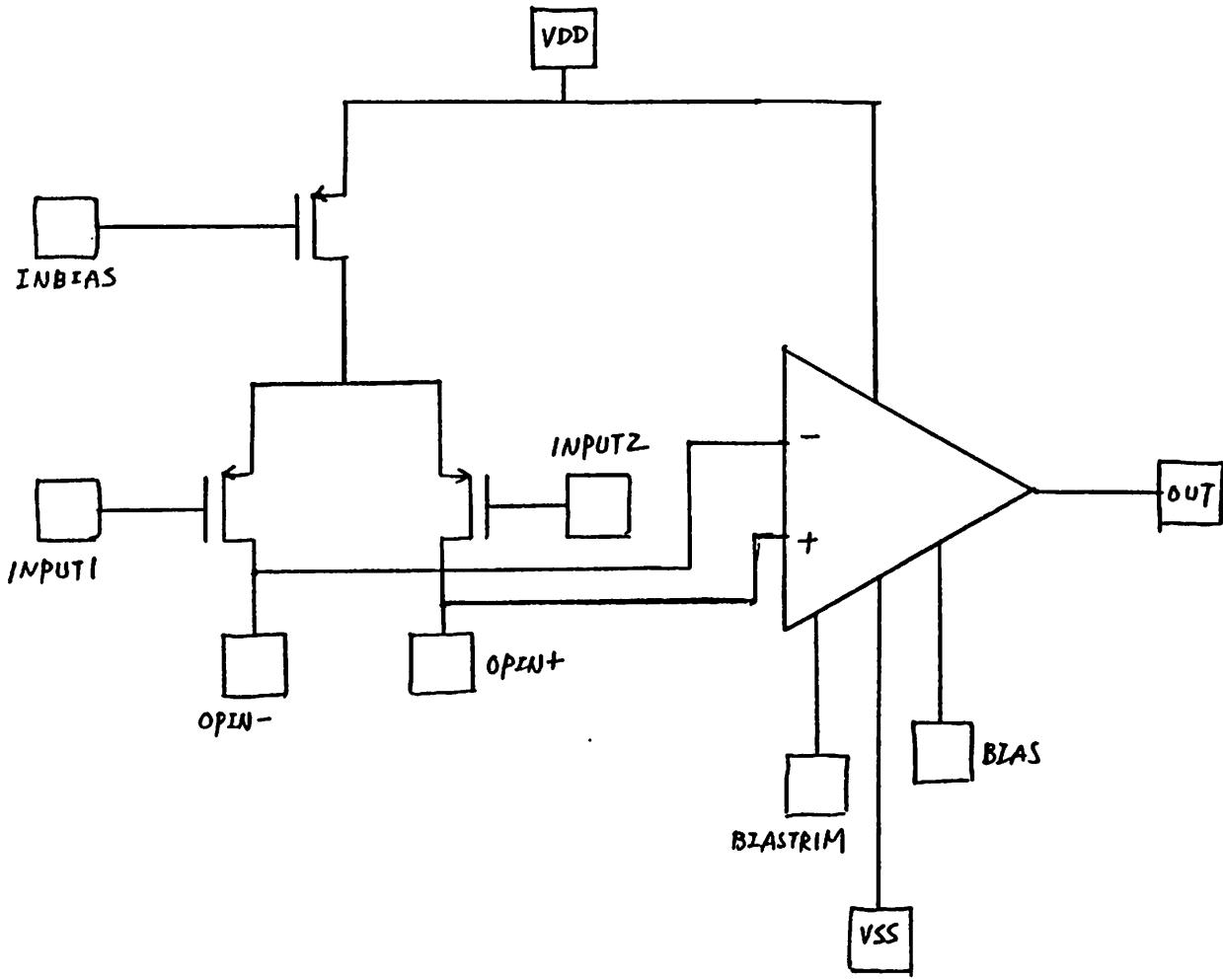
Figure 8-1. Noise Measurement Circuit Schematic
