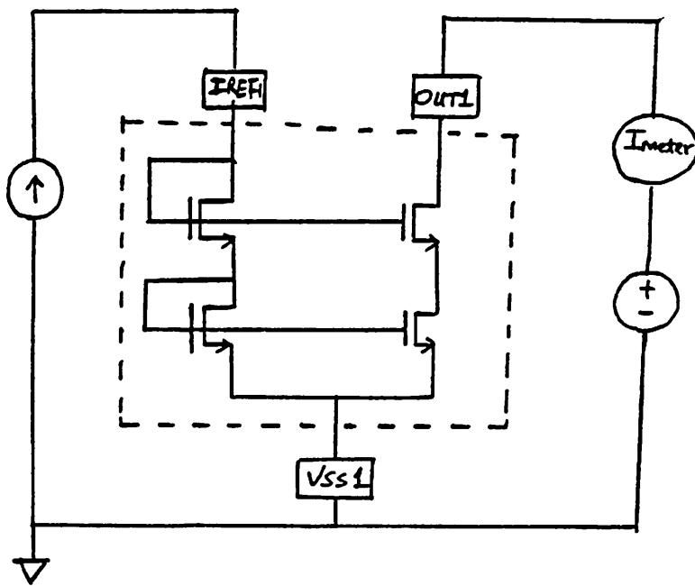
Fig. 10-2 Current Mirror Test setup.
