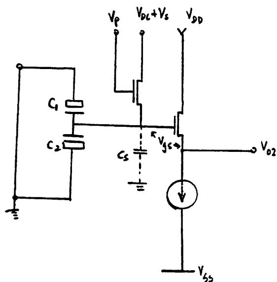
FIG 5.2 2nd Measurement to eliminate  $V_{GS}$
