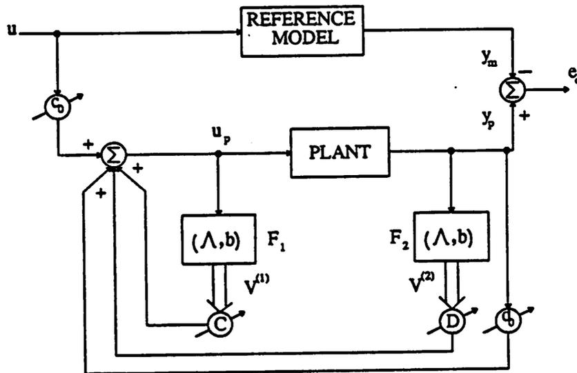
Figure 4.2.1 Model Reference Adaptive Controller
