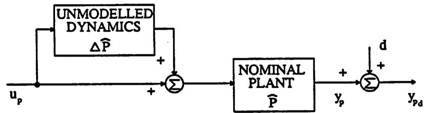
Figure 4.4.1 Unmodelled Dynamics and Output Disturbances
