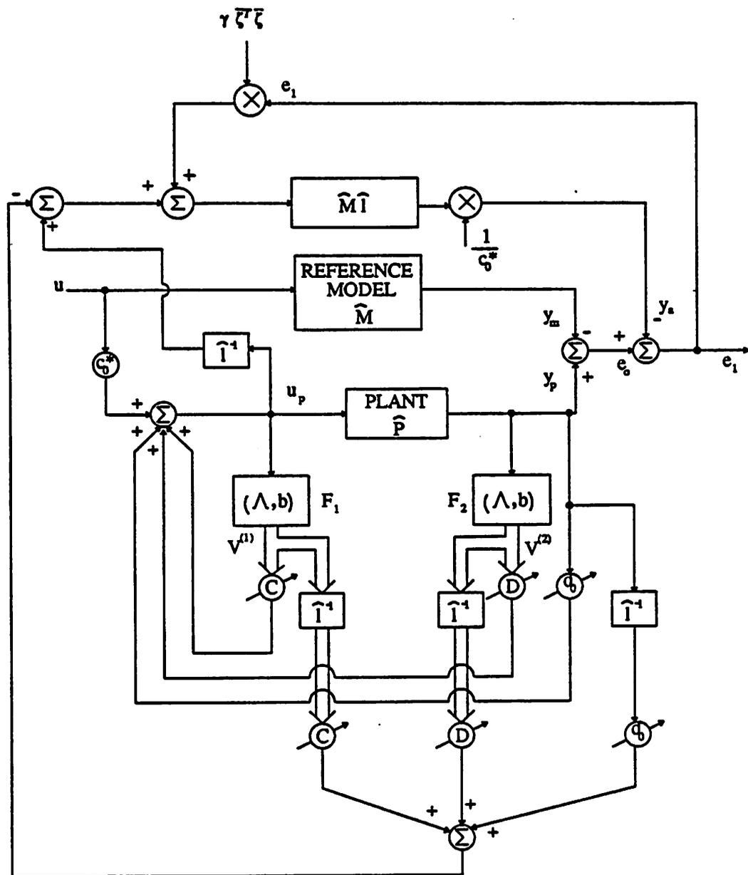
Figure 4.2.3 Modified Model Reference Adaptive Controller
