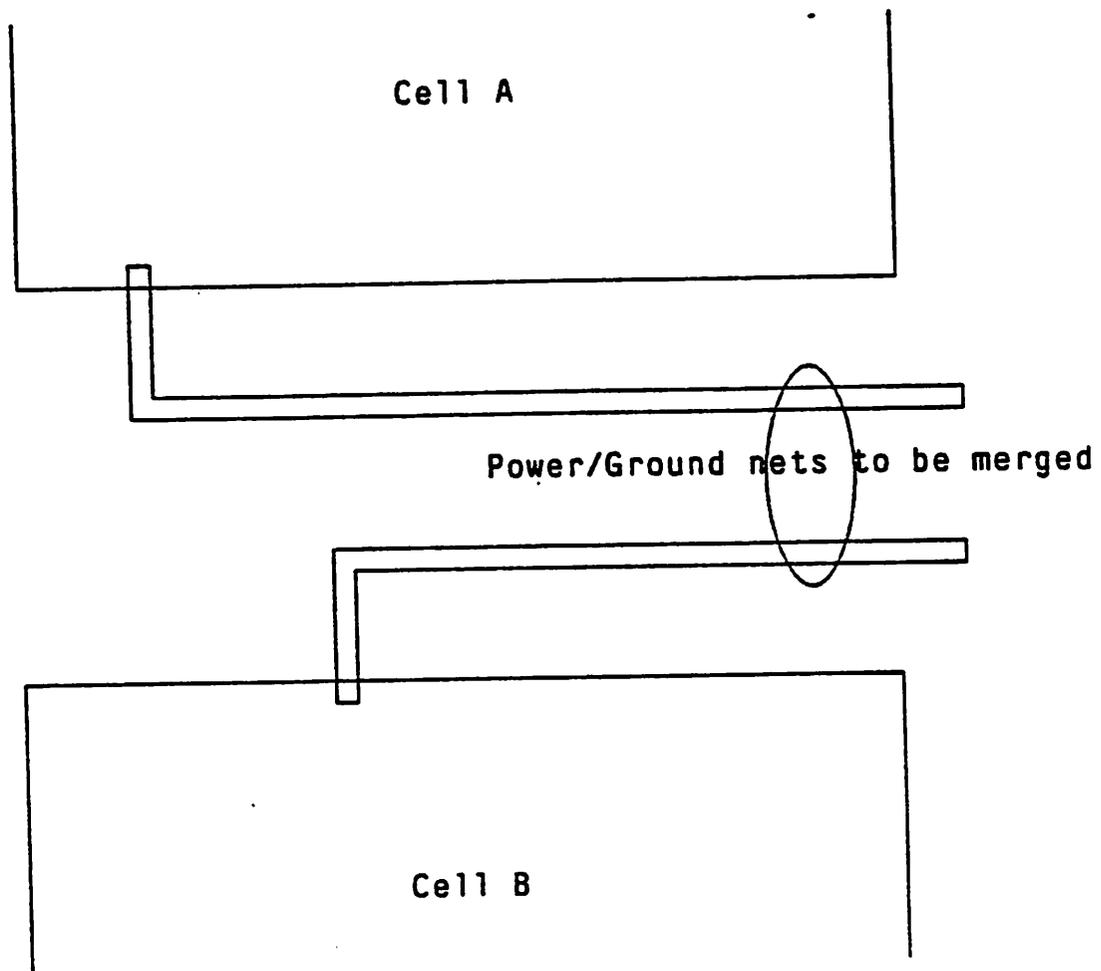
**Figure 3. Merging of Power/Ground nets in the channel.**
