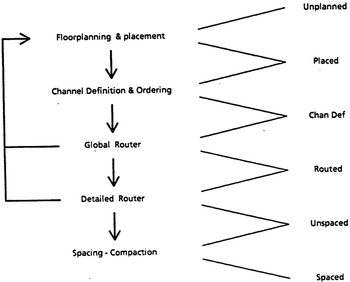
Figure 1. The Layout System and the correspondent OCT views.
