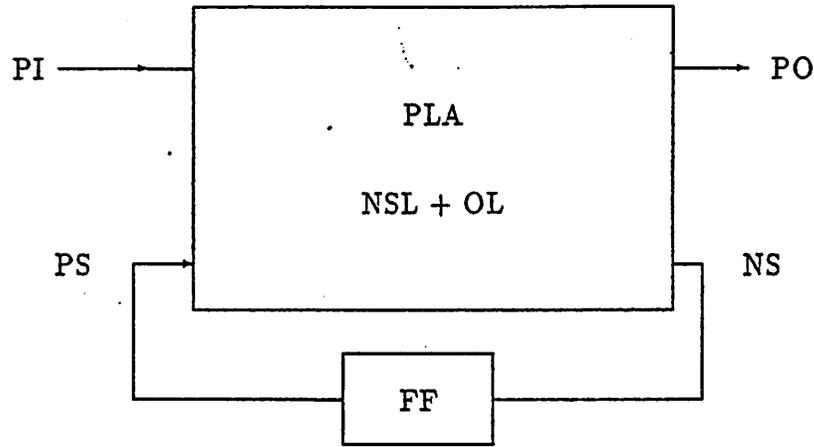
Figure 1: PLA-based Finite State Machine
