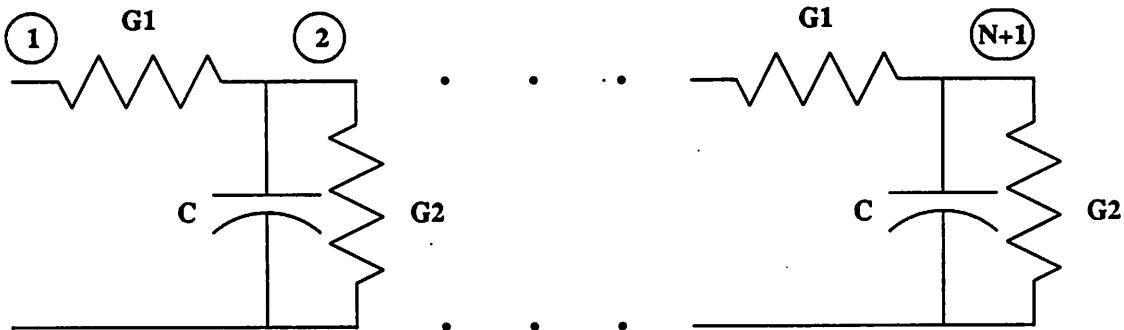
Figure 6.2: RC ladder model for a neuron
