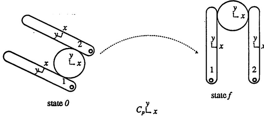
Figure 4: From state 0 to state  $f$  by dexterous manipulation
