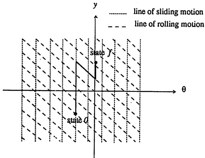
Figure 6: Relative configurations of the object to finger 2 from state 0 to state  $f$ .
