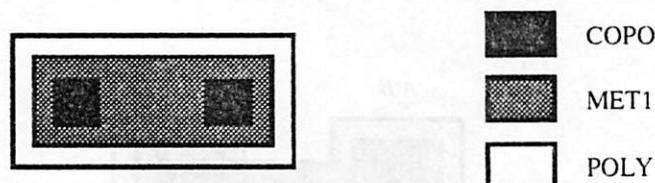
Figure 4.27: Terminal frames of POLY-MET1 contact.
