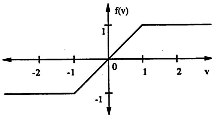
Figure 1: The piecewise-linear sigmoid function is the only non-linearity in each cell of a CNN. This non-linearity maps the state to the interval  $[-1,1]$ .
