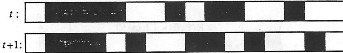
Figure 13: One iteration of the state transition rule which can compute one projection of the Radon Transform of a binary image on a cellular automata. Image pixels with a background pixel to their right at time  $t$  shift to the right in time  $t + 1$ .
