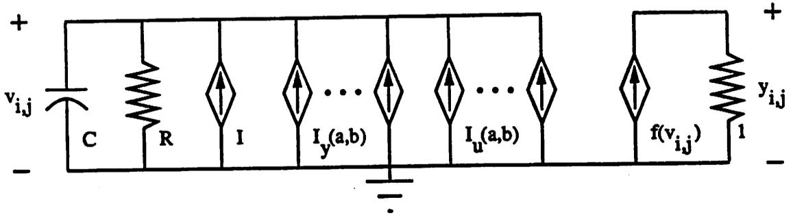
Figure 2: The state equation of each cell of a single layer CNN can be implemented with the above circuit consisting only of a capacitor, resistors, and voltage controlled current sources.  $I_y(a, b) = A(a, b)y_{i+a, j+b}$  and  $I_u(a, b) = B(a, b)u_{i+a, j+b}$ .
