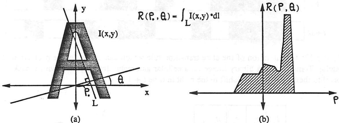
Figure 12: (a) For fixed values of  $\rho_0$  and  $\theta_0$  the Radon Transform  $\mathcal{R}(\rho_0, \theta_0)$  of an image  $I(x, y)$  is the line integral of  $I(x, y)$  along line  $L$ . (b) For fixed  $\theta_0$ , the function  $\mathcal{R}(\rho, \theta_0)$  is the projection of the image onto the line  $\theta = \theta_0$ .
