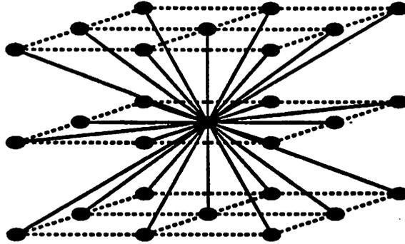
Figure 5: The interconnections of a CNN are restricted to nearest neighbor couplings. This figure illustrates the interconnections for a cell in layer two of a three layer CNN.
