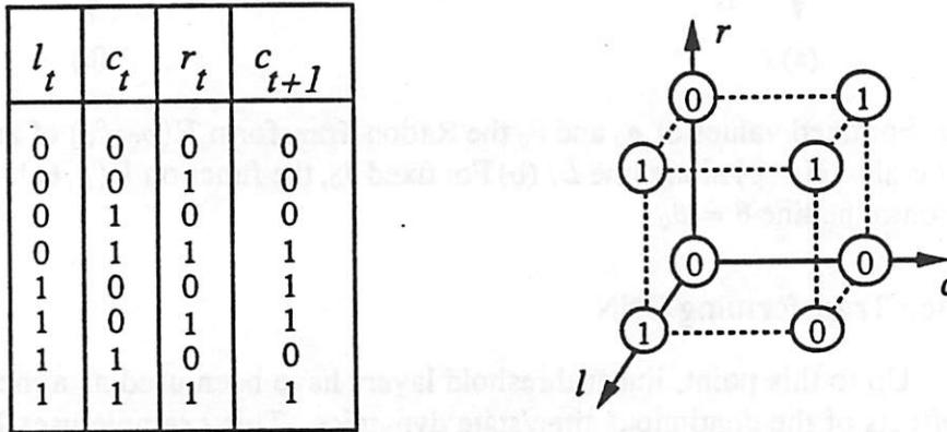
Figure 14: The values which map to zero and one by the boolean function (10) are not separable by a plane in  $(l, c, r)$  variable space
