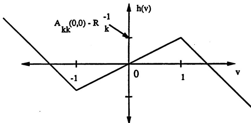
Figure 3: The function  $h(v)$  determines the contribution from the state of a linear threshold single layer CNN to its derivative.
