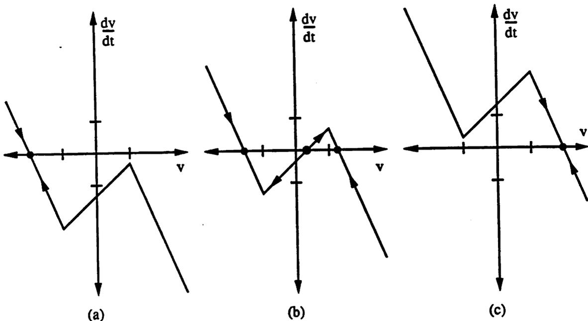
Figure 4: The value of  $g$  determines the dynamic routes for a cell in the linear threshold layer. (a)  $g < -(A(0, 0) - R_1^{-1})$ . (b)  $|g| < (A(0, 0) - R_1^{-1})$ . (c)  $g > (A(0, 0) - R_1^{-1})$ .
