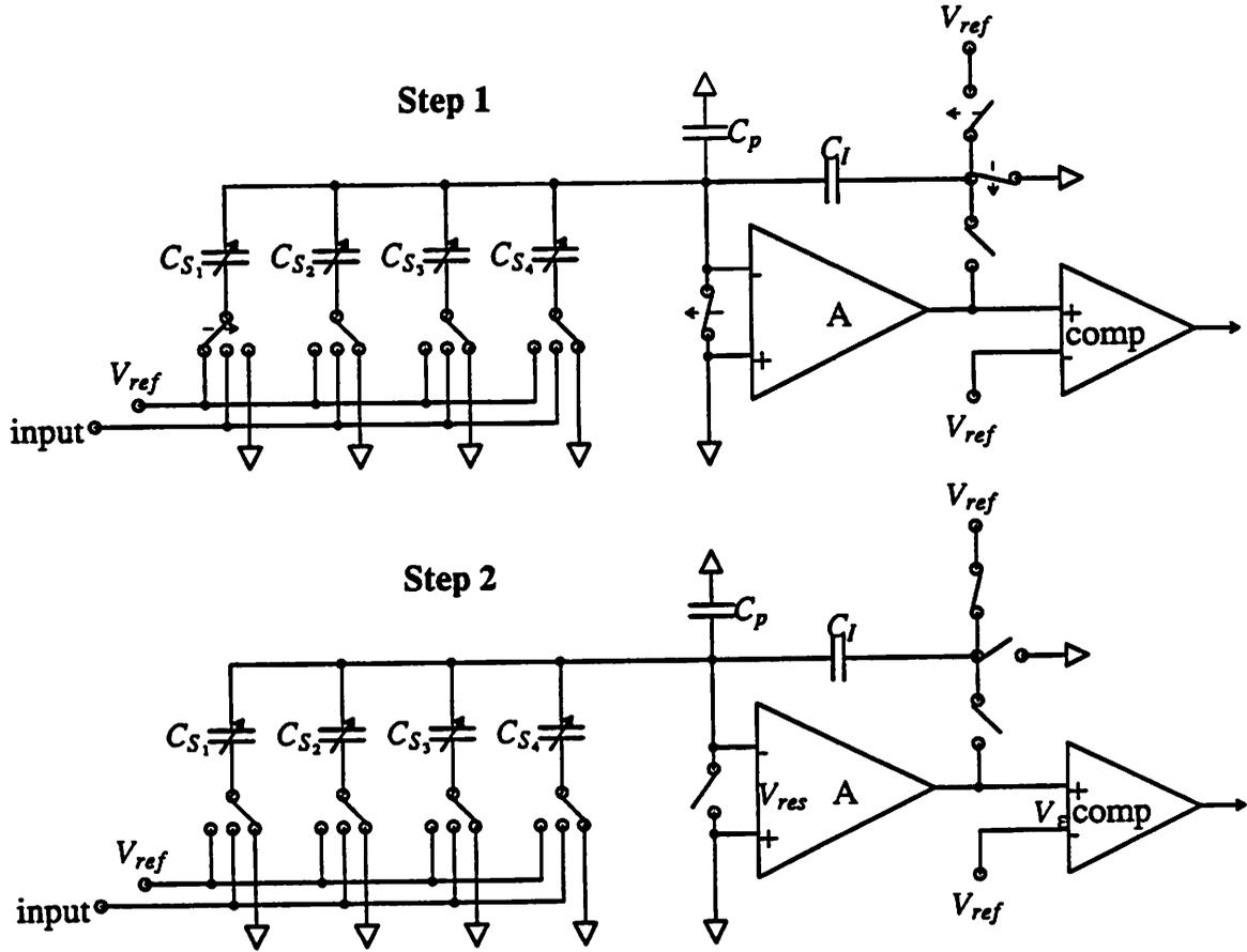
Fig. 4.14 Principle of Self-Calibration Technique
