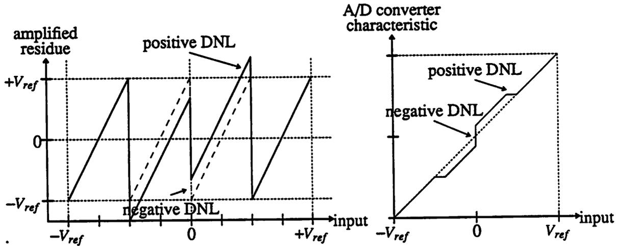
Fig. 4.5 Transition Magnitude Mismatch in a Pipelined Stage
