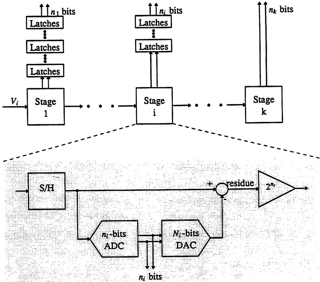
Fig. 3.4 Pipelined A/D Converter
