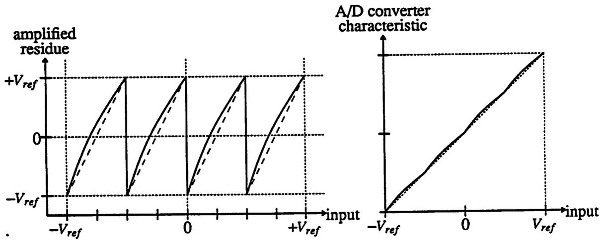
Fig. 4.7 Nonlinearity in a Pipelined Stage
