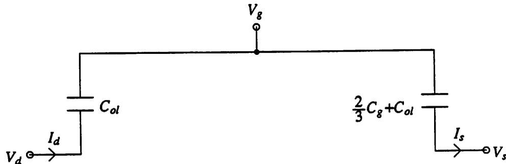
Fig. 2.6 Equivalent Circuit of a MOS Switch in Saturation Region
