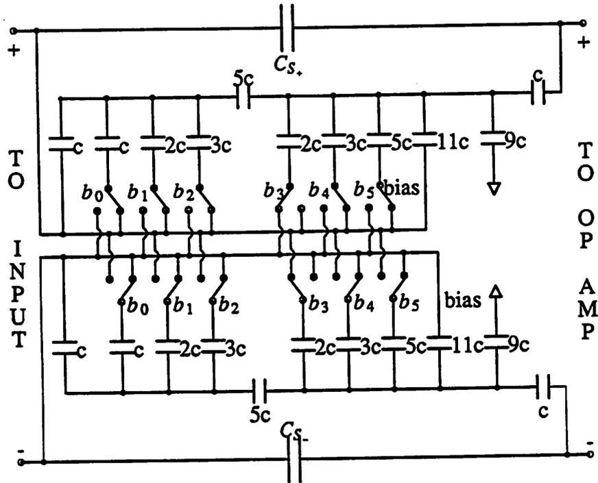
Fig. 5.8 Trim Capacitor for the First Stage
