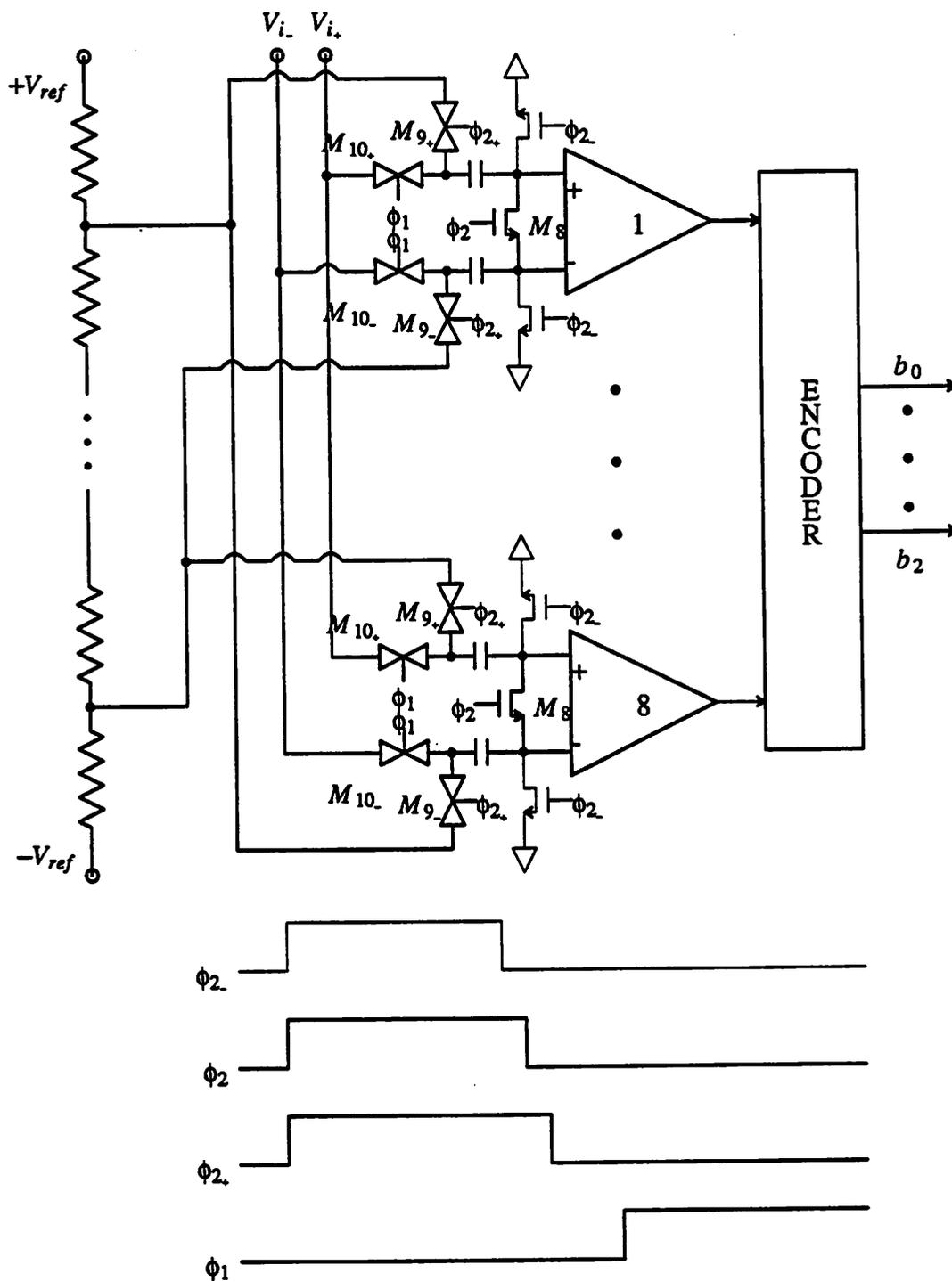
Fig. 5.4 3-bit Differential A/D Subconverter
