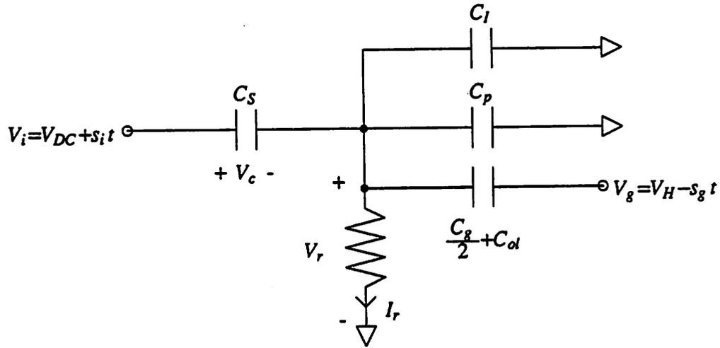
Fig. 2.9 Equivalent Circuit of a Single-Ended Bottom-Plated T/H in Linear Region
