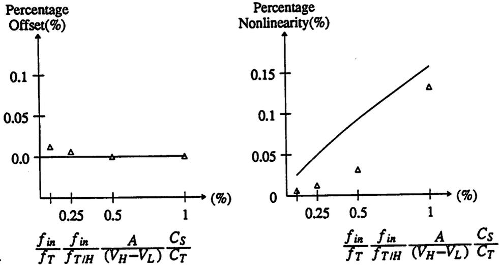
Fig. 2.16 Performance of the Differential T/H Circuit with Single Sampling Switch
