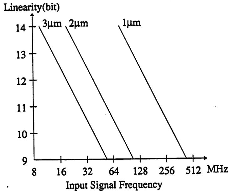
Fig. 7.1 Achievable Linearity vs. Signal Frequency
