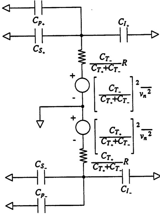
Fig. 5.3  $\frac{kT}{C}$  Noise Calculation
