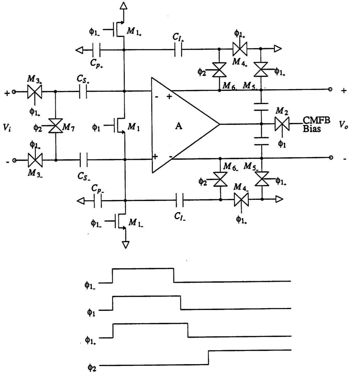
Fig. 5.2 Input S/H Circuit
