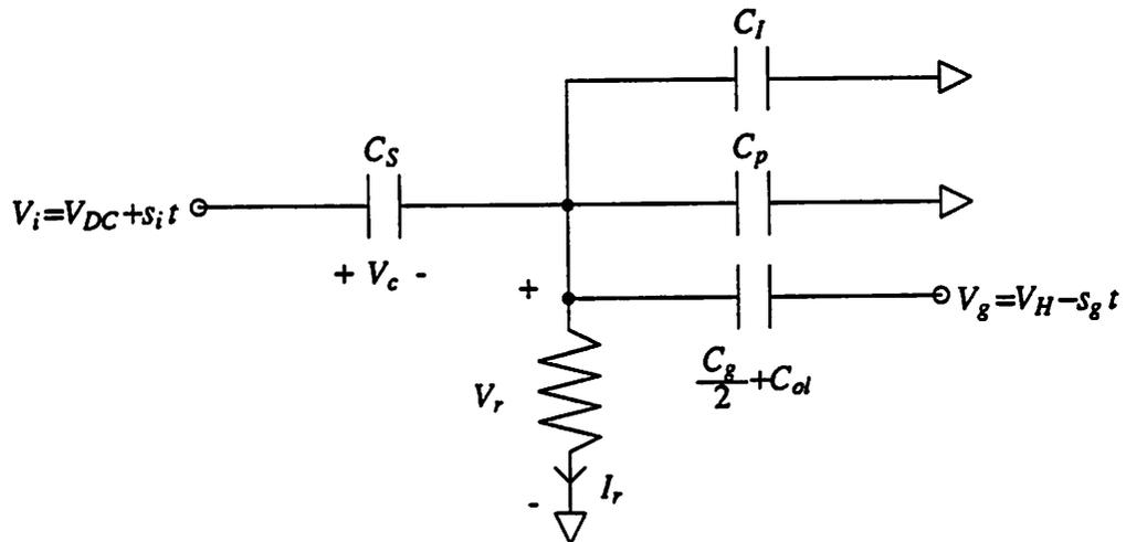
Fig. A.1 Equivalent Circuit of a Single-Ended Bottom-Plated T/H in Linear Region
