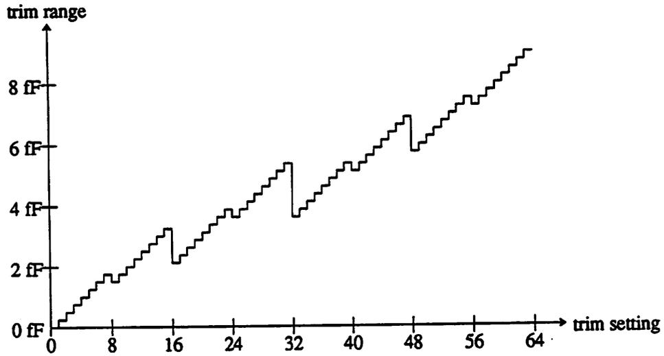
Fig. 5.10 Trim Capacitor for the First Stage
