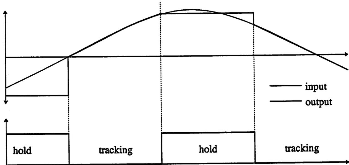
Fig. 2.1 Input and Output Waveform of an Ideal T/H Circuit
