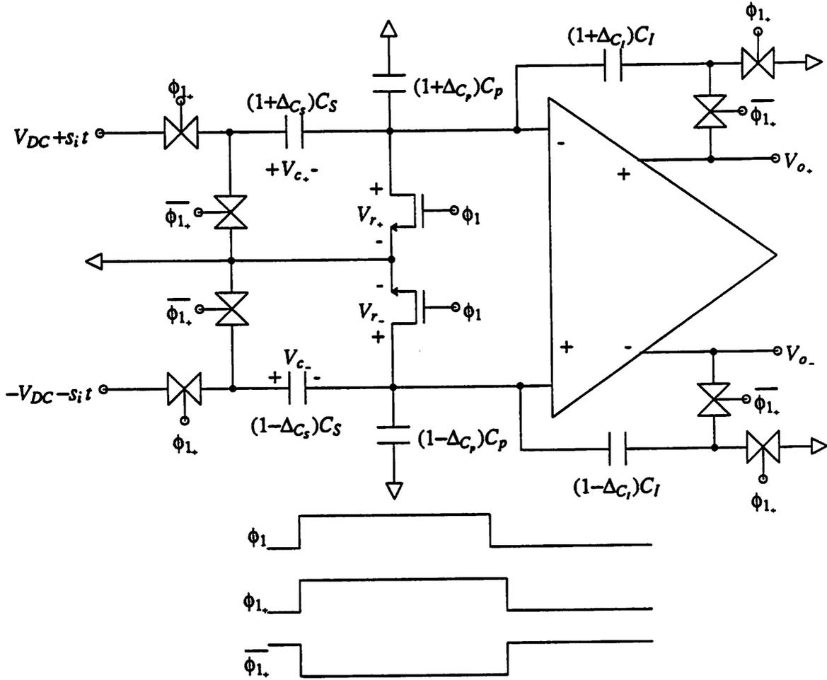
Fig. 2.10 Differential Bottom-Plated T/H Circuit
