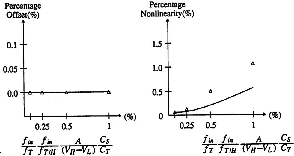
Fig. 2.14 Performance of the Differential T/H Circuit
