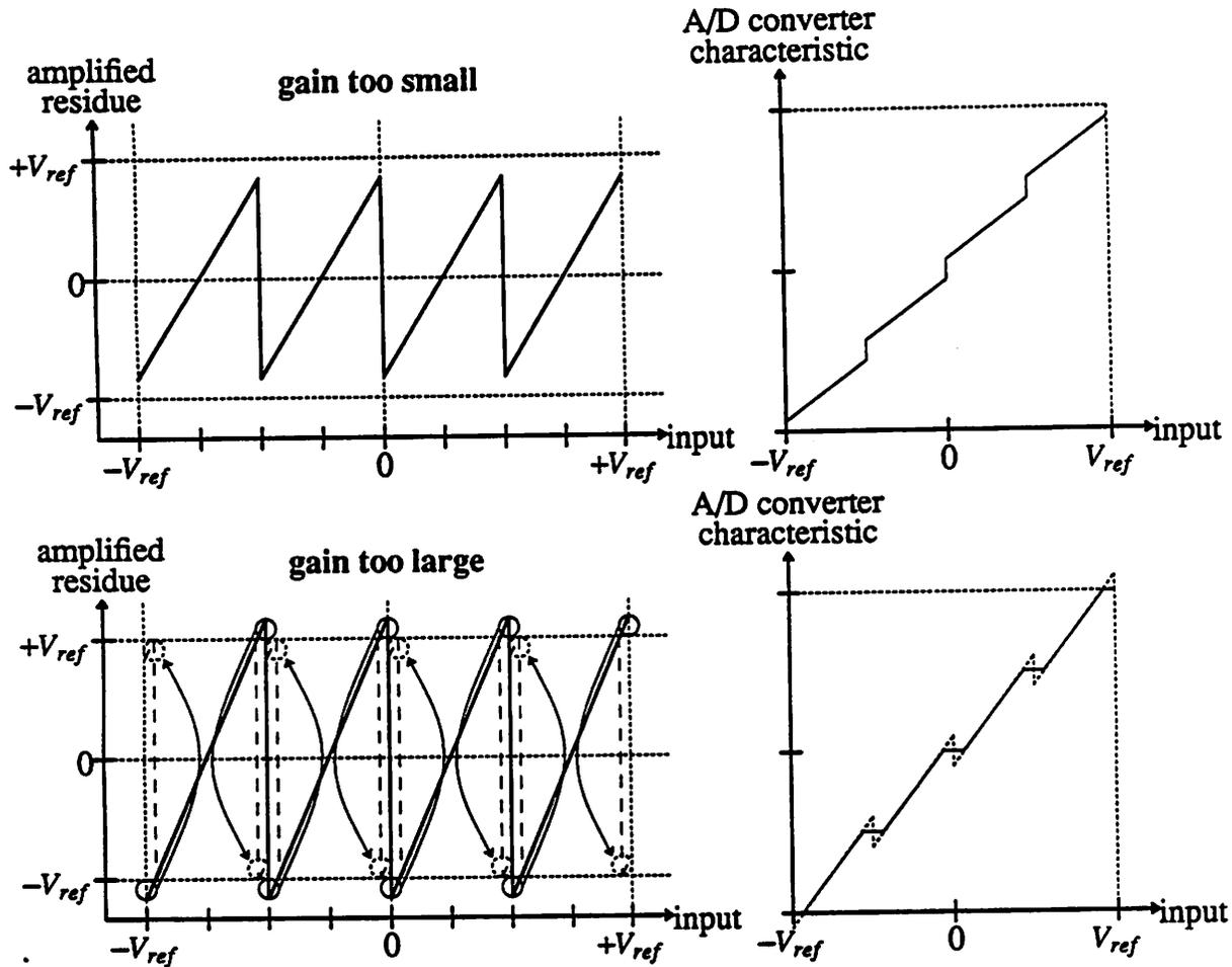
Fig. 4.11 Transition Magnitude Gain Error in a Pipelined Stage with Digital Error Correction
