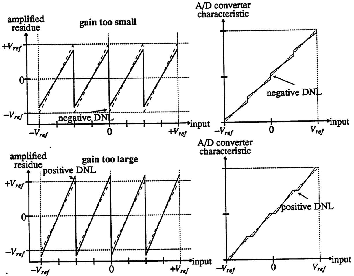
Fig. 4.6 Transition Magnitude Gain Error in a Pipelined Stage
