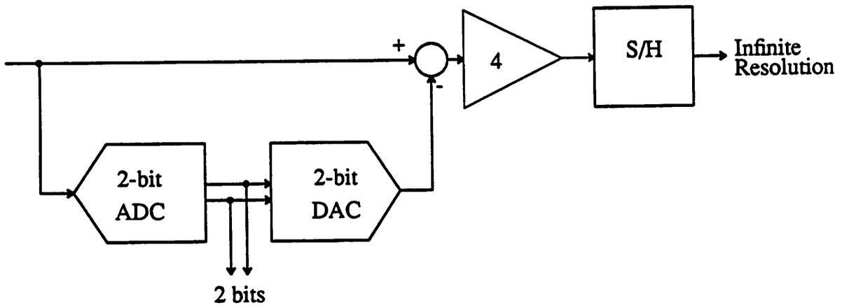
Fig. 4.1 Block Diagram of a 2-bit Pipelined Stage
