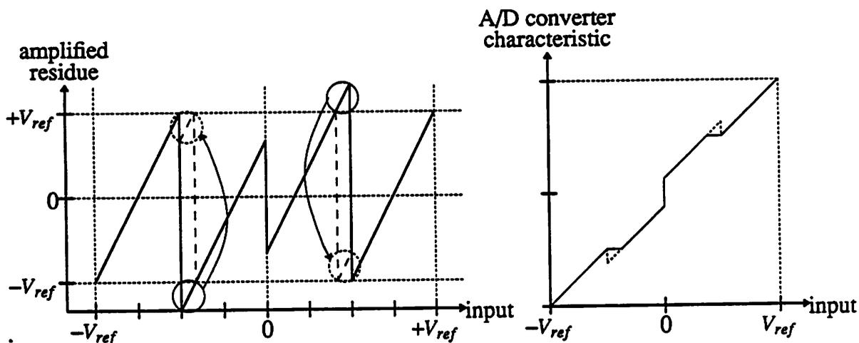
Fig. 4.10 Transition Magnitude Mismatch in a Pipelined Stage with Digital Error Correction encountered in a pipelined A/D converter.
