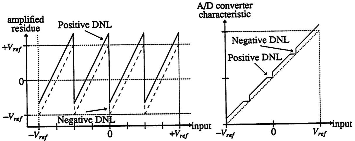
Fig. 4.3 Offset in a Pipelined Stage
