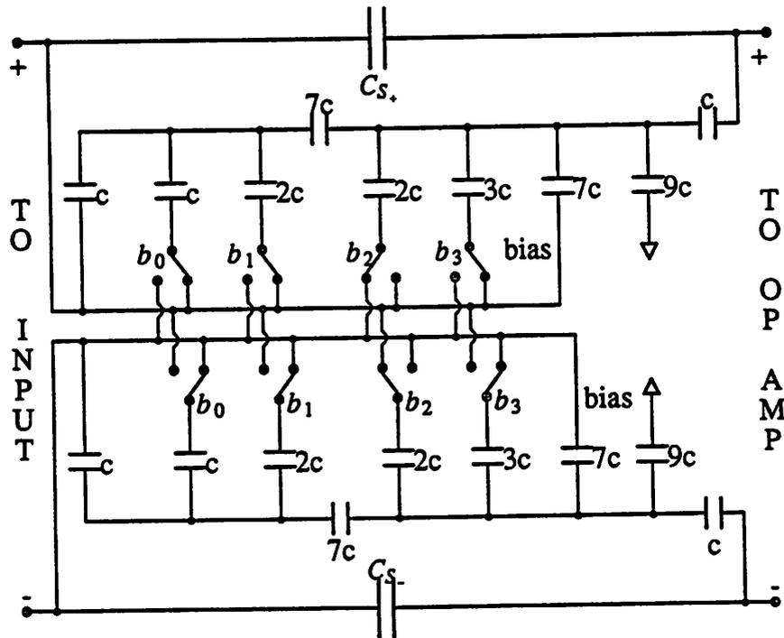
Fig. 5.9 Trim Capacitor for the Second Stage
