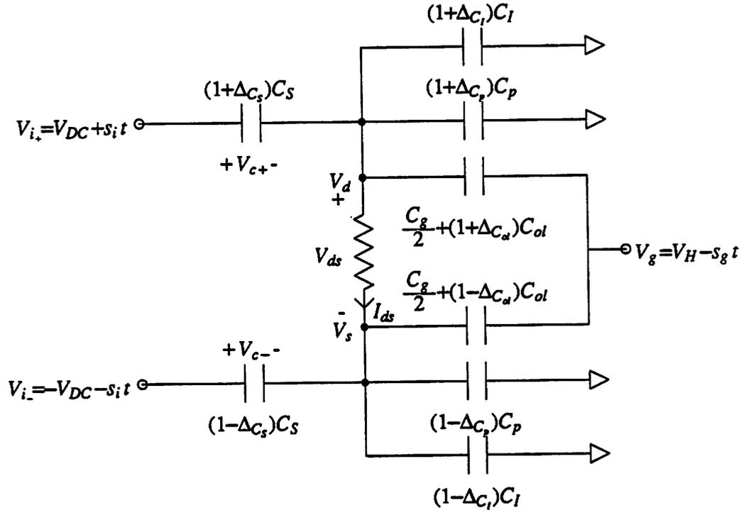
Fig. 2.12 Equivalent Circuit of Differential T/H Circuit with Single Sampling Switch
