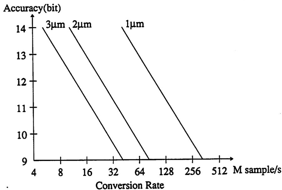
Fig. 7.2 Accuracy vs. Peak Achievable Conversion Rate
