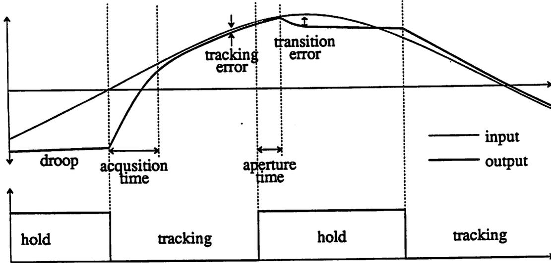
Fig. 2.2 Input and Output Waveform of a Real T/H Circuit
