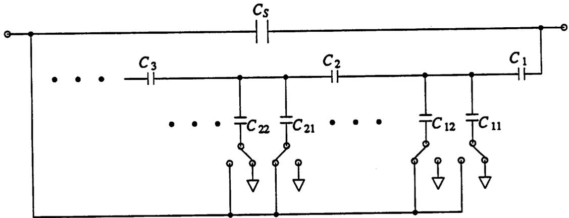
Fig. 4.15 A Generalized Capacitor Array
