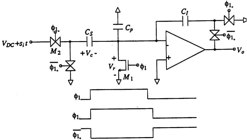
Fig. 2.7 Single-Ended Bottom-Plate T/H Circuit
