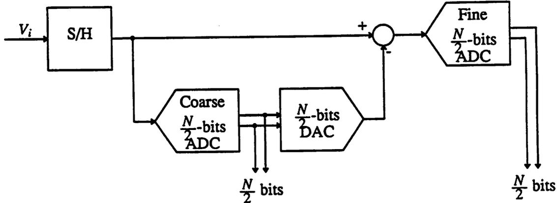
Fig. 3.3 Subranging A/D Converter
