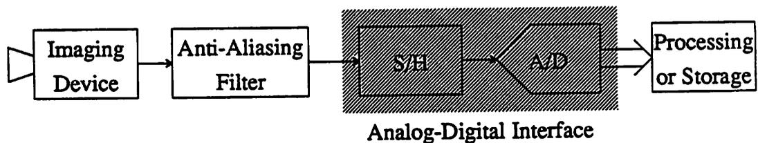
Fig. 1.1 Video Image Processing System
