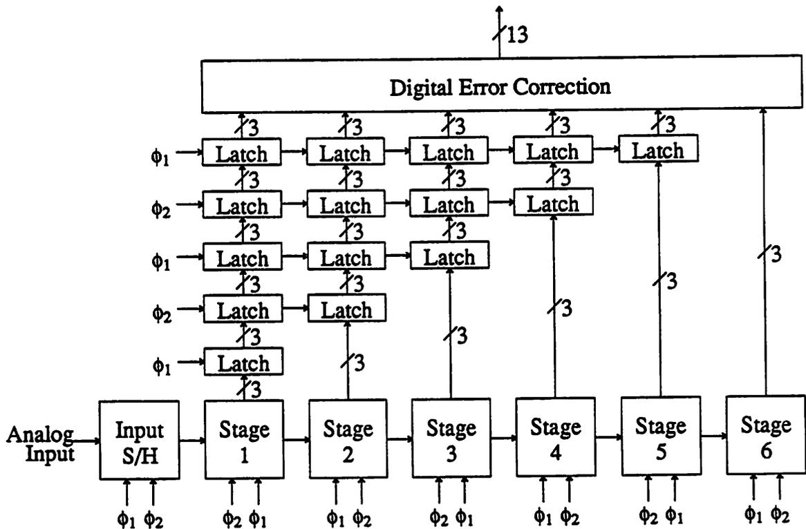
Fig. 5.1 Block Diagram of 13-bit Pipelined A/D Converter
