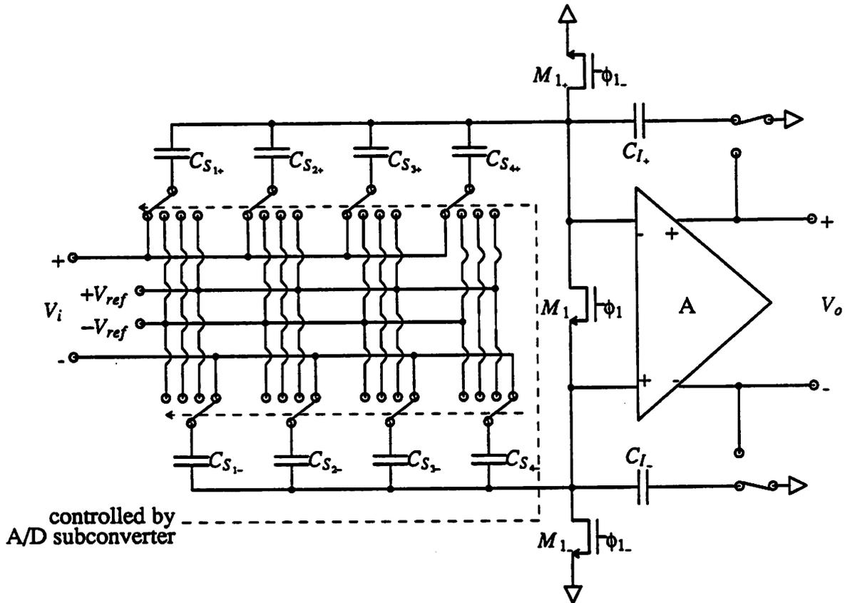
Fig. 5.6 Implementation of a 3-bit Pipelined Stage
