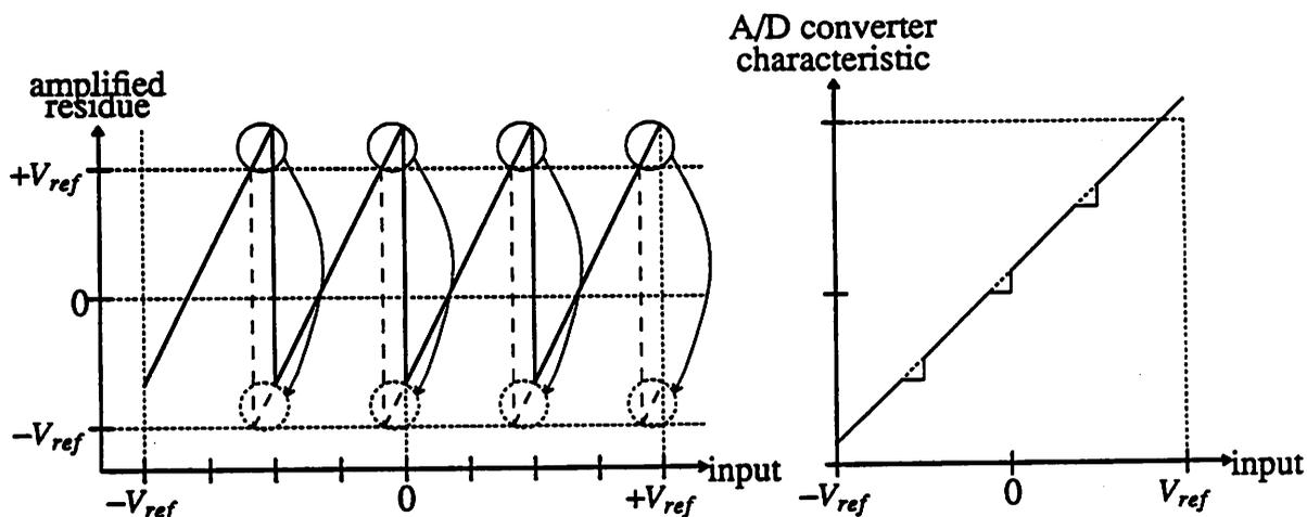
Fig. 4.9 Offset in a Pipelined Stage with Digital Error Correction
