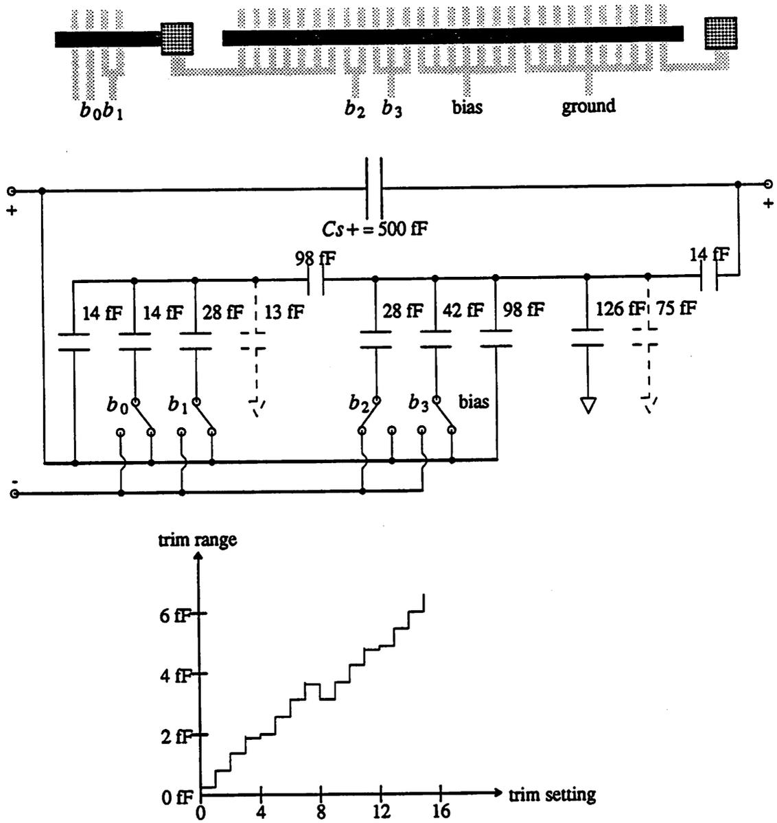
Fig. 5.11 Trim Capacitor for the Second Stage
