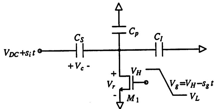
Fig. 2.8 Single-Ended Bottom-Plate T/H Equivalent Circuit
