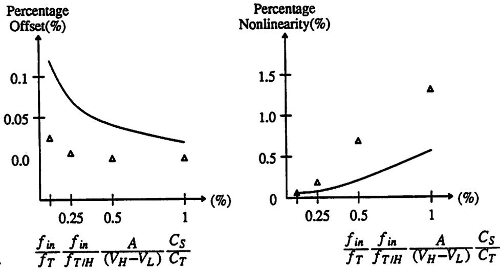
Fig. 2.15 Performance of the Differential T/H Circuit(1% Mismatch)
