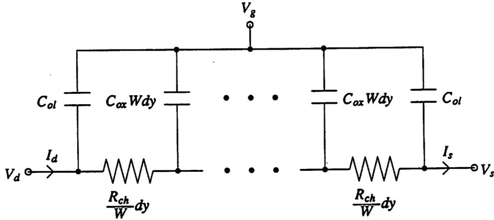
Fig. 2.4 Quasi-Static Switch Model
