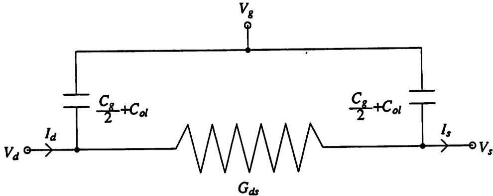
Fig. 2.5 Equivalent Circuit of a MOS Switch in Linear Region
