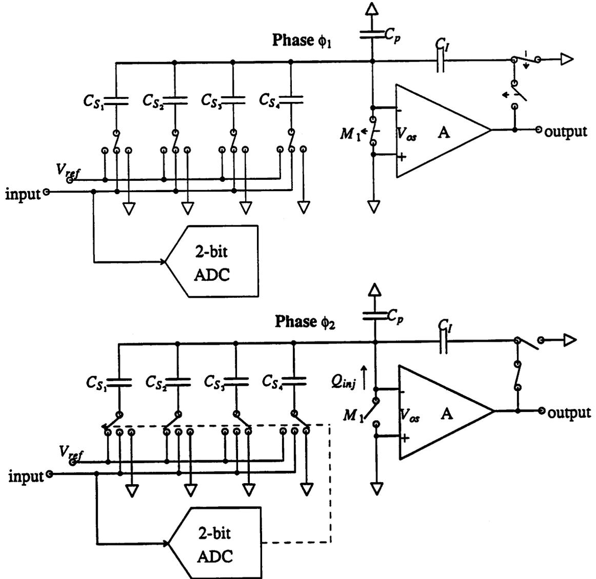
Fig. 4.12 Implementation of a S/C 2-bit Pipelined Stage
