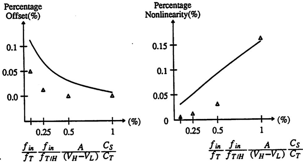
Fig. 2.17 Performance of the Differential T/H with Single Sampling Switch (1% mismatch)
