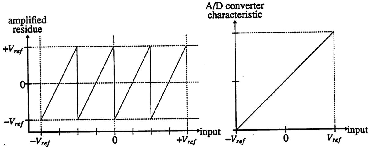
Fig. 4.2 Input-Output Relationship of an Ideal 2-bit Pipelined Stage
