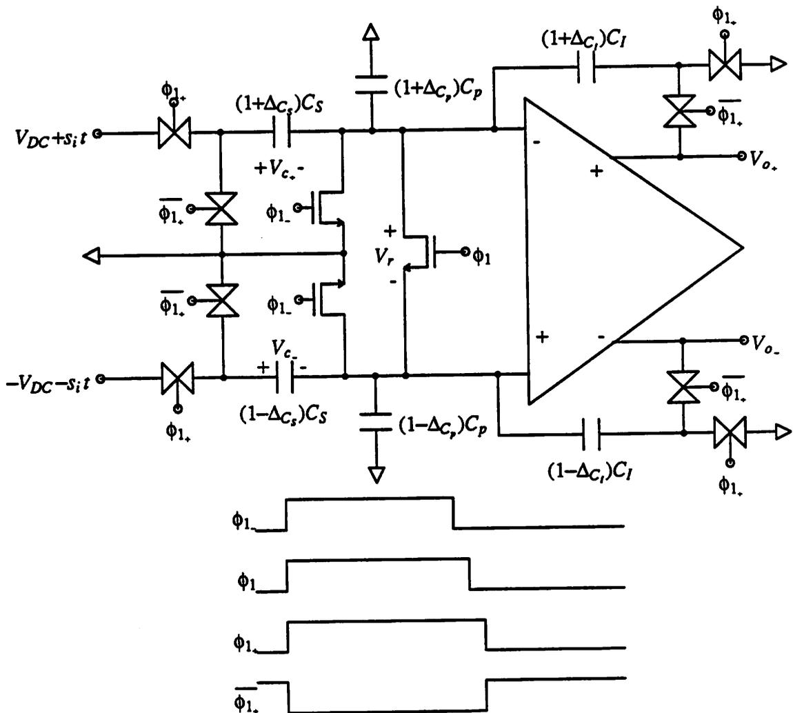
Fig. 2.11 Differential T/H Circuit with Single Sampling Switch
