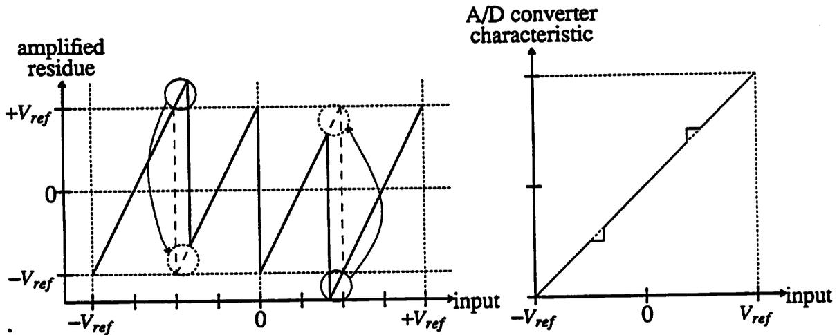
Fig. 4.8 Principle of Digital Error Correction
