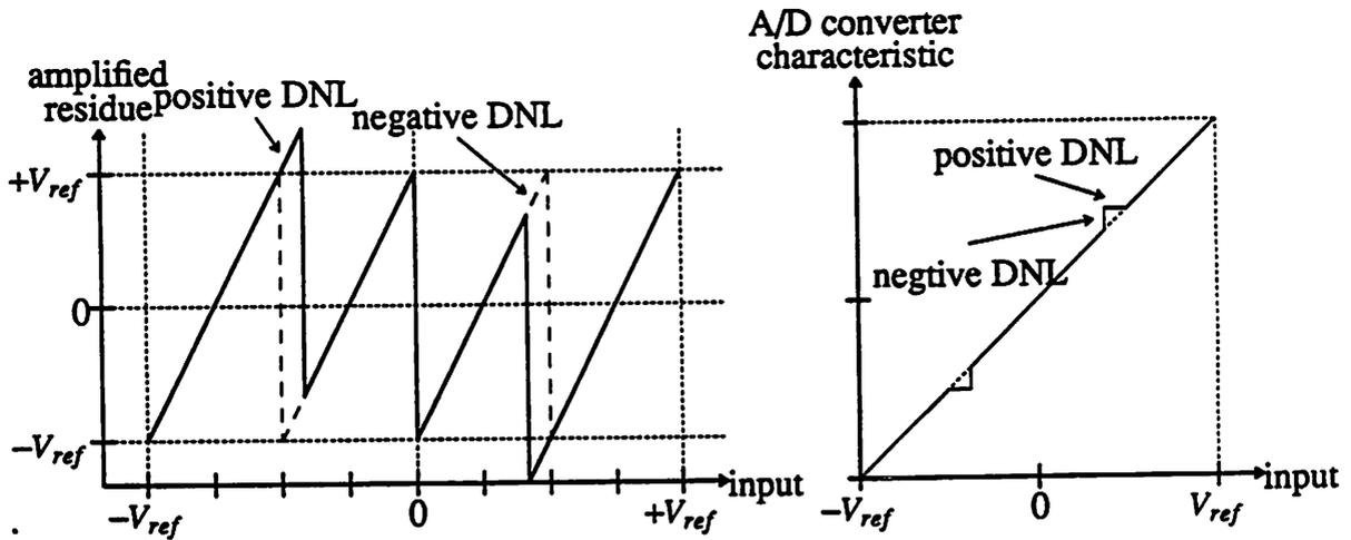
Fig. 4.4 Nonideal Transition Position in a Pipelined Stage
