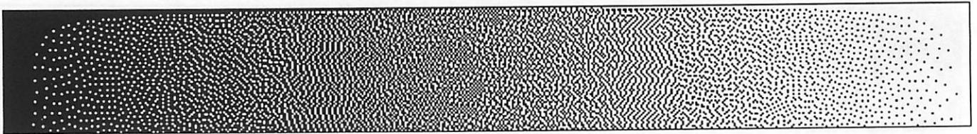
Figure 8: Floyd Error Filters Ramp Output
