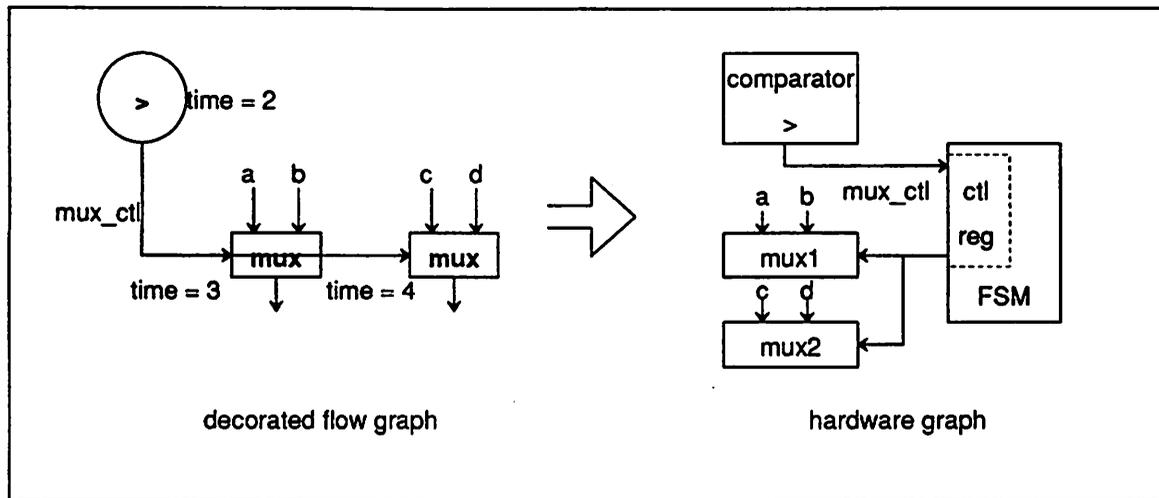
Figure 2.20: Control Register Allocation
