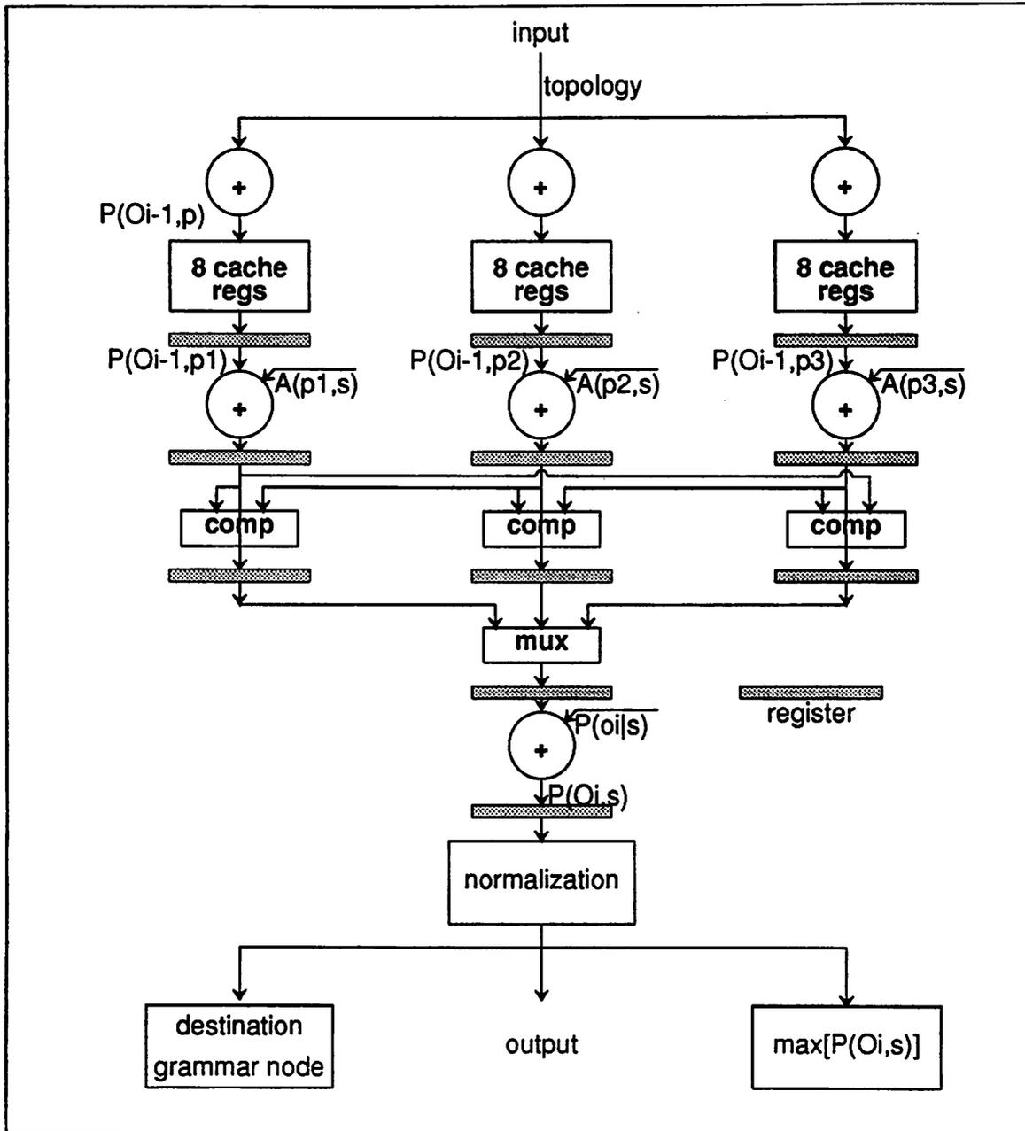
Figure 4.7: Architecture of the Viterbi Processor
