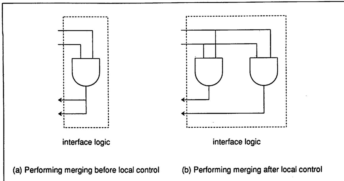
Figure 2.22: Different Interface Logic Structures As Resulting From Two Control Optimization Orders
