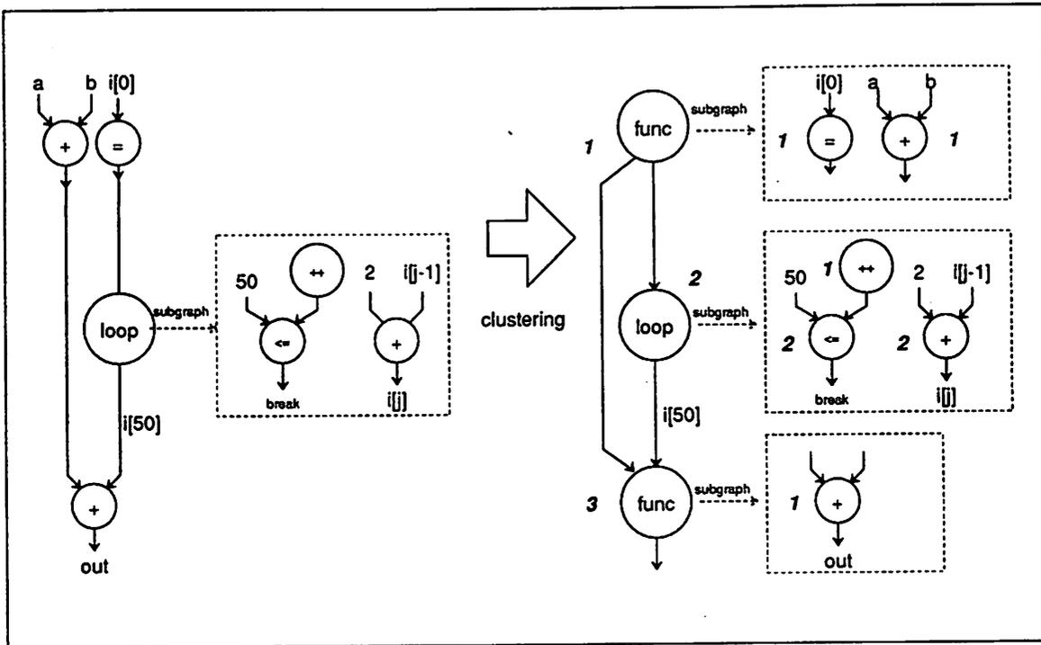
Figure 3.12: Node Clustering in Hierarchical Flow Graphs
