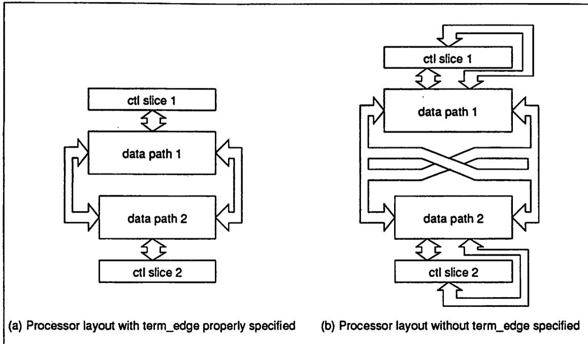
Figure 2.23: Comparison Between Layouts With and Without `TERM_EDGE` Property
