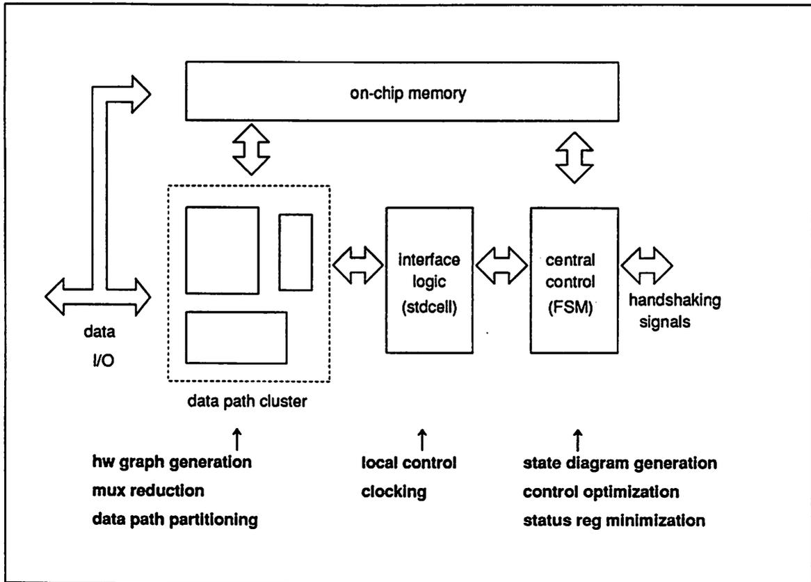
Figure 2.2: Target Architecture of HYPER
