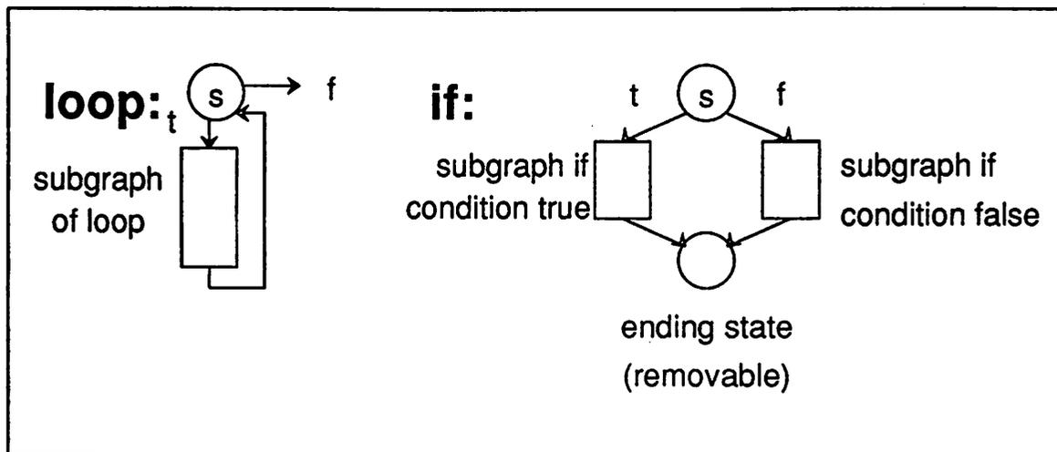
Figure 2.15: Rules for State Transition Diagram Generation
