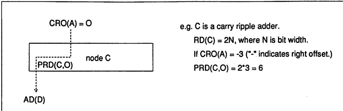
Figure 3.6: Flow Graph to Demonstrate the Ripple Offset
