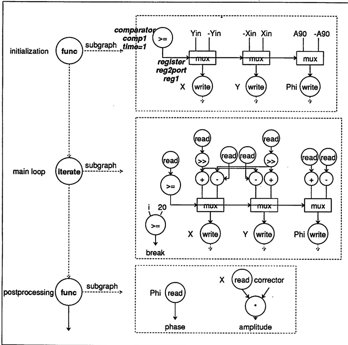
Figure 2.1: Flow Graph of the CORDIC Algorithm
