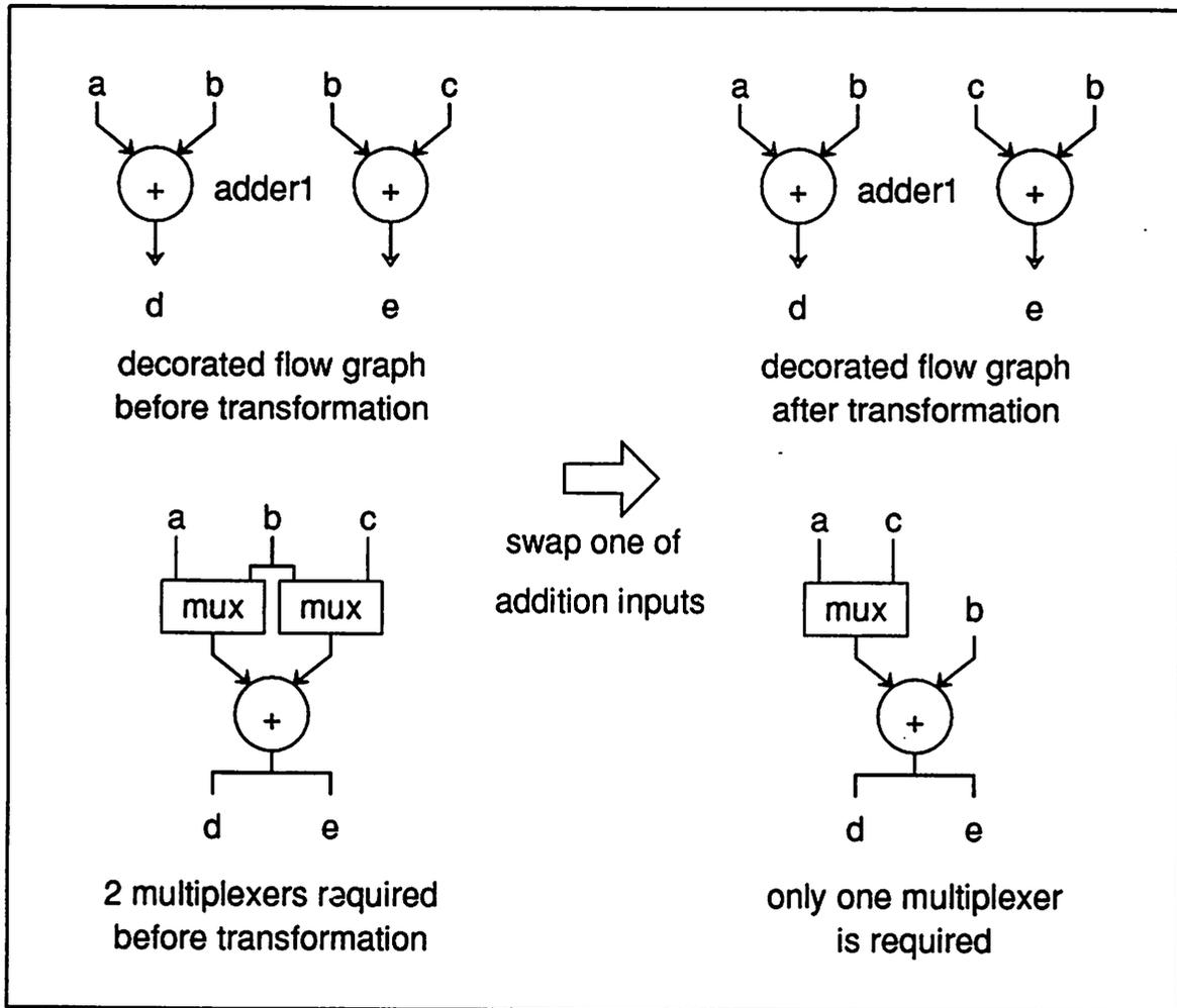
Figure 2.11: Algebraic Commutativity for Multiplexer Reduction
