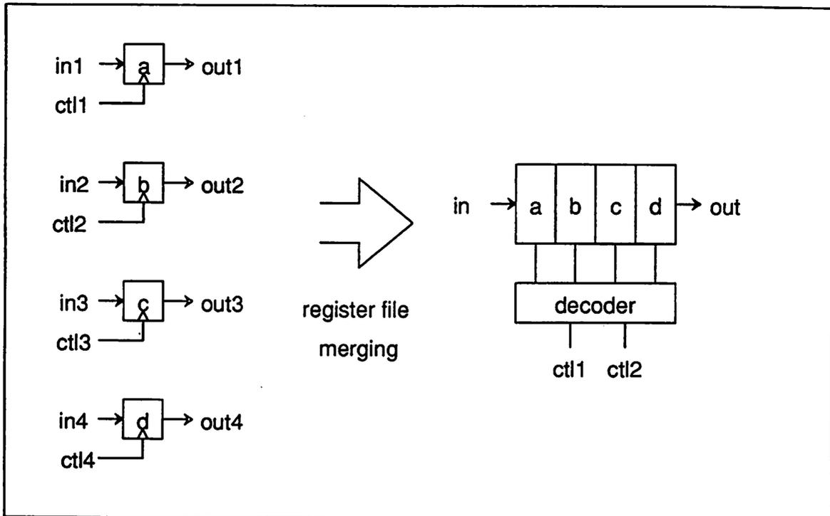
Figure 2.5: Register File Merging
