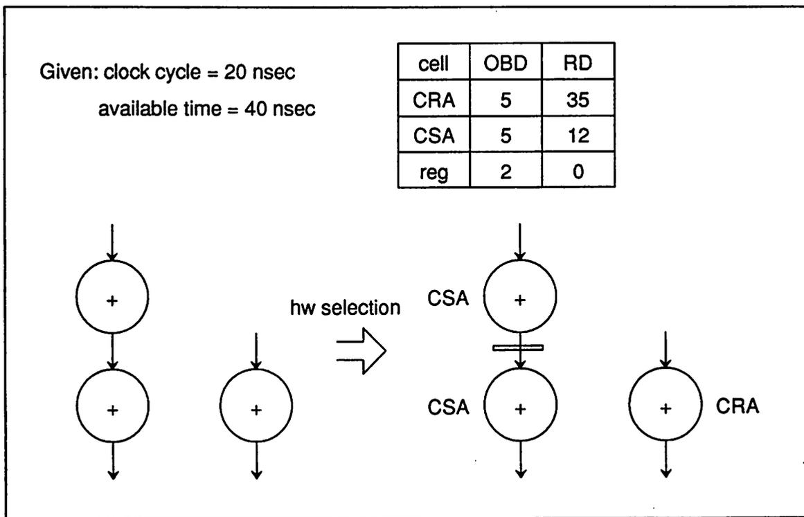
Figure 3.19: Hardware Swapping to Meet Throughput Constraints
