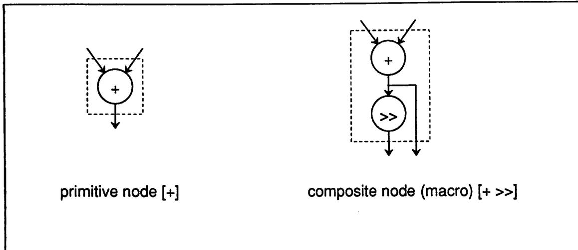
Figure 3.2: Primitive Node and Composite Node
