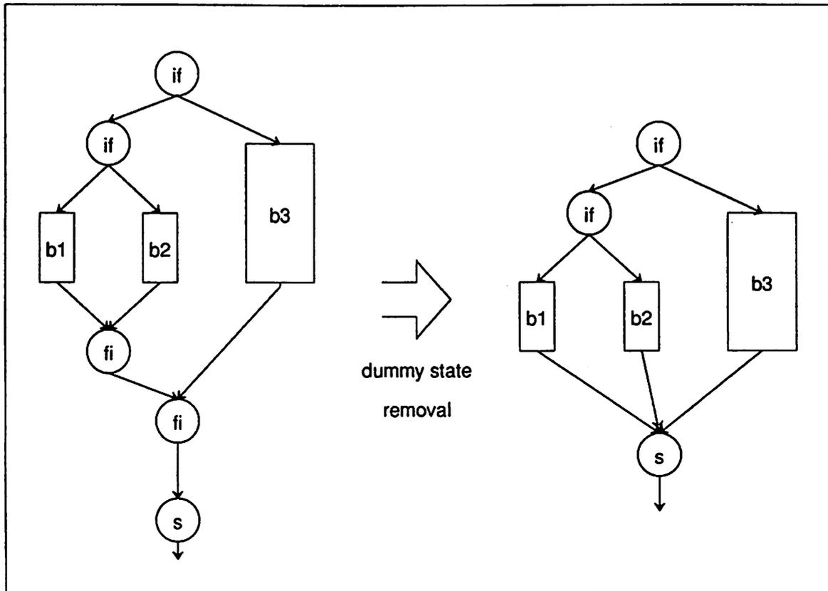
Figure 2.17: Dummy State Removal
