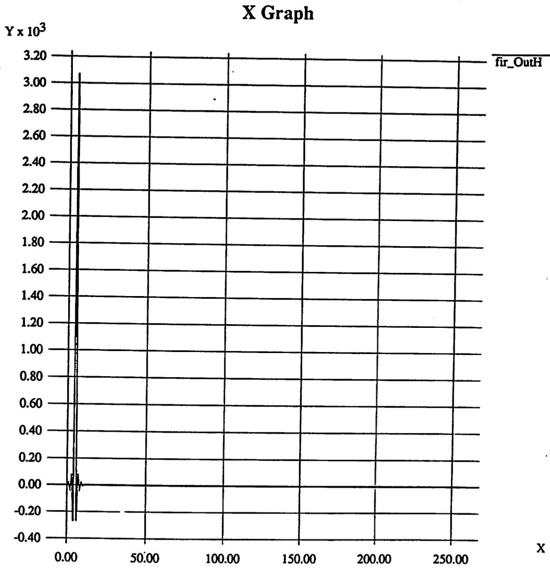
Figure 4.17: Impulse Response of the FIR Filter
