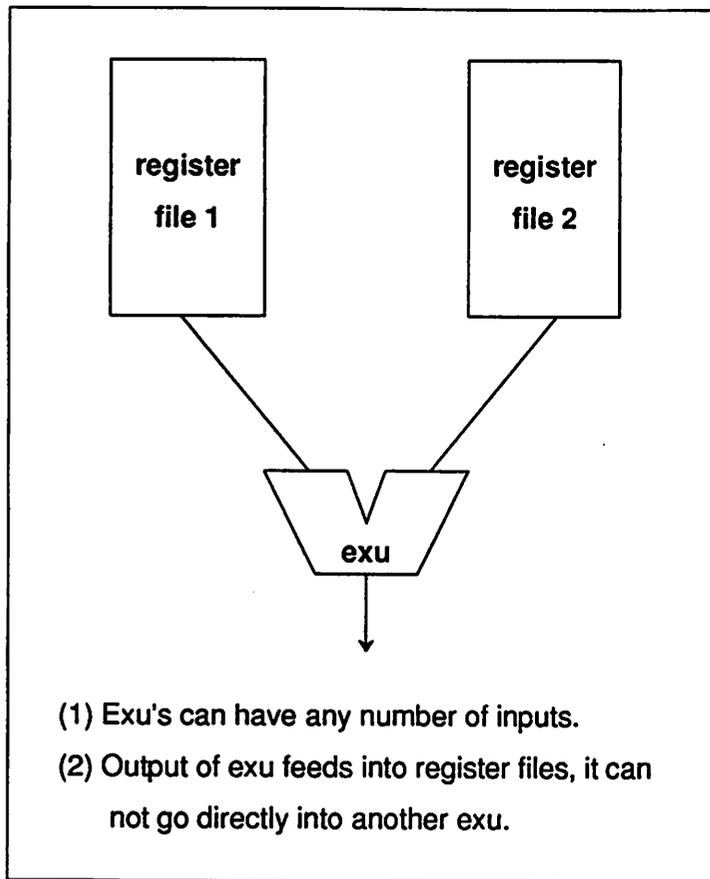
Figure 2.7: Hardware Model of HYPER
