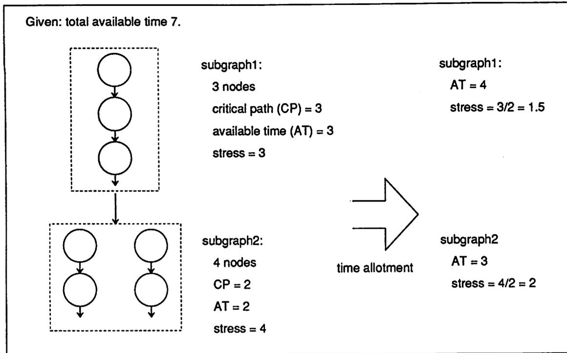
Figure 3.13: Example to Illustrate Time Allotment
