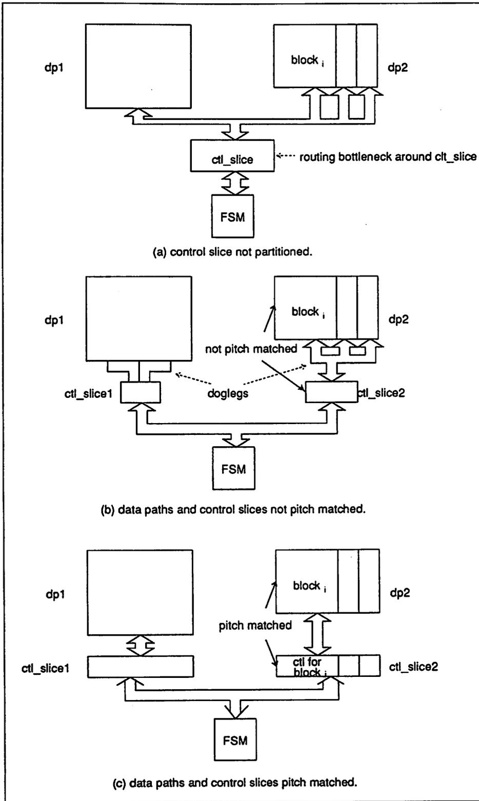
Figure 2.18: Three Types of Control Slice Structures
