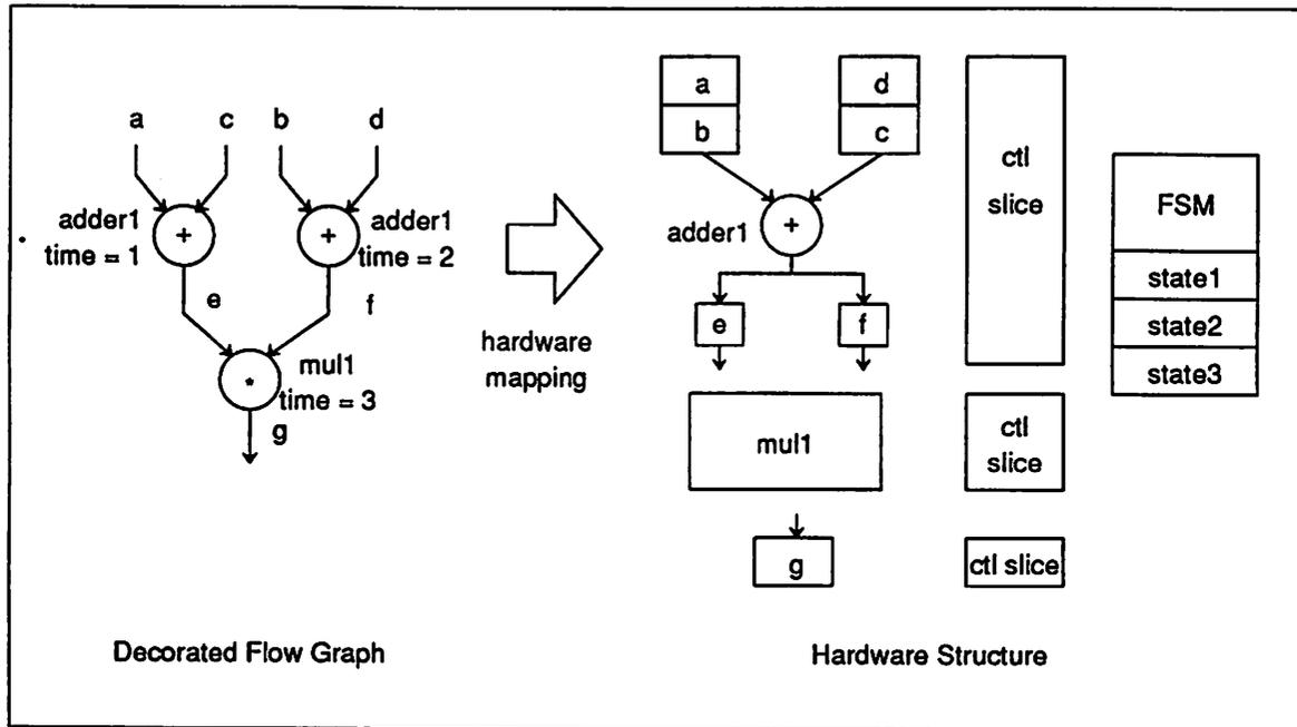
Figure 2.3: Example to Illustrate Hardware Mapping
