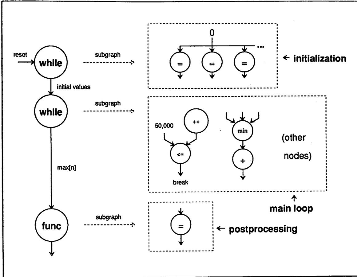
Figure 4.6: Flow Graph of the Viterbi Processor
