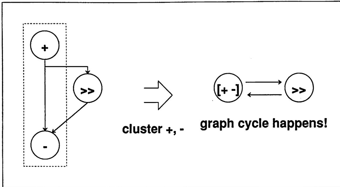
Figure 3.8: Graph Cycles Caused by Clustering
