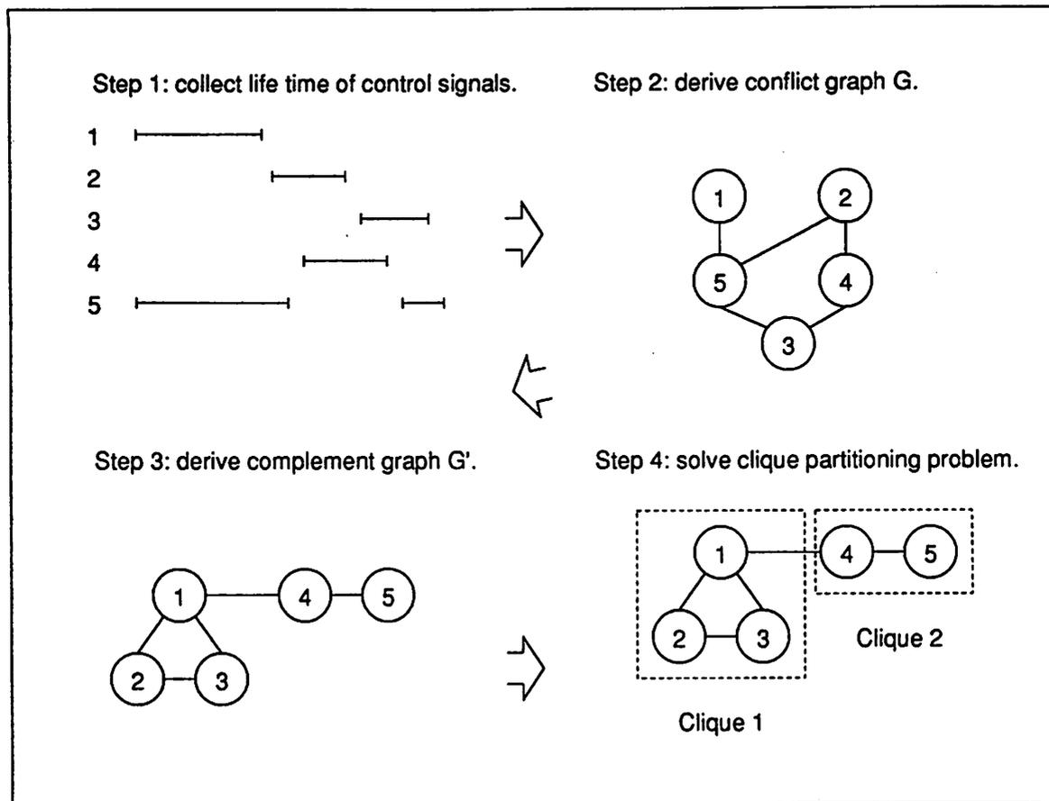
Figure 2.21: Procedure for Allocating Control Register
