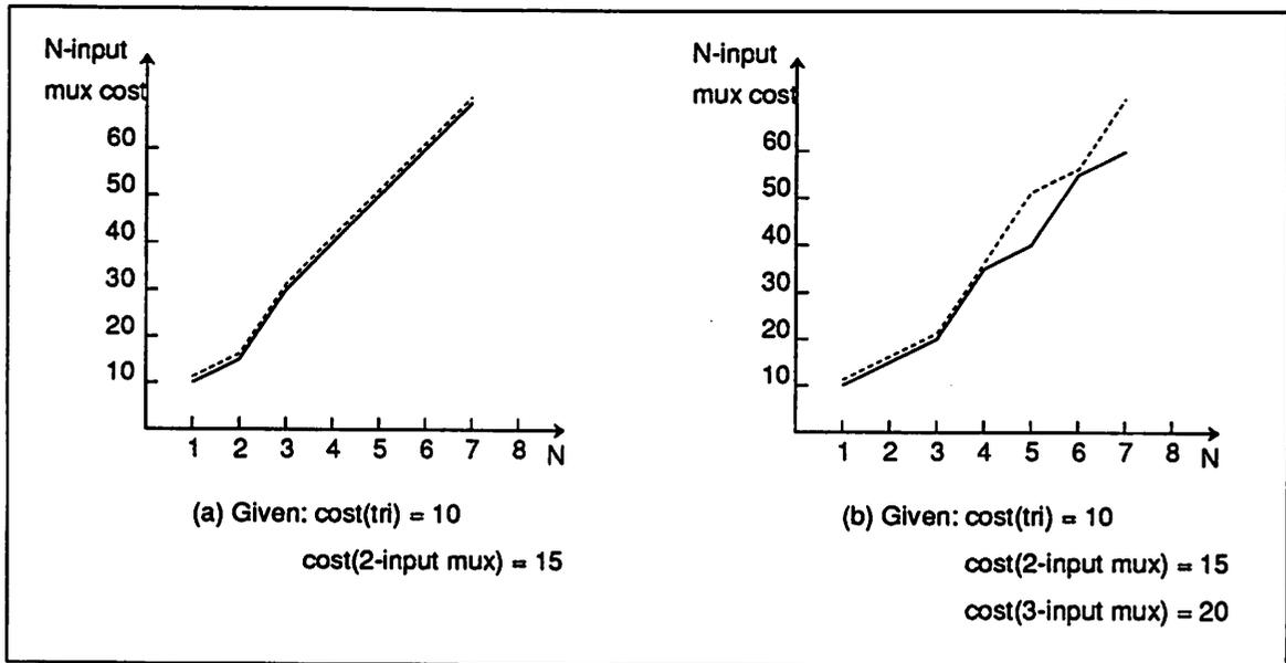
Figure 2.12: Multiplexer Cost Found by Proposed Approach and Exhaustive Search
