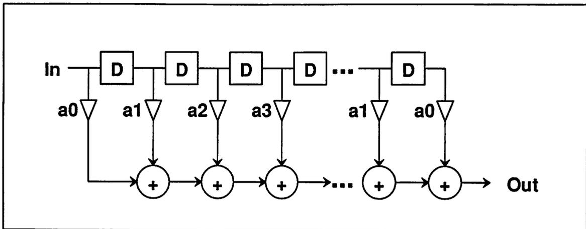
Figure 4.15: Flow Graph of the FIR Filter
