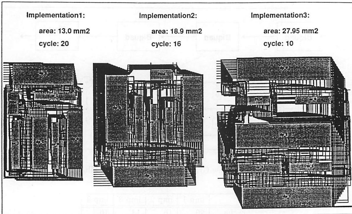
Figure 4.10: 3 IIR Filter Layouts of Different Implementations
