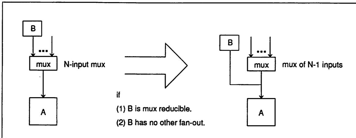
Figure 2.8: Multiplexer Reducible Modules
