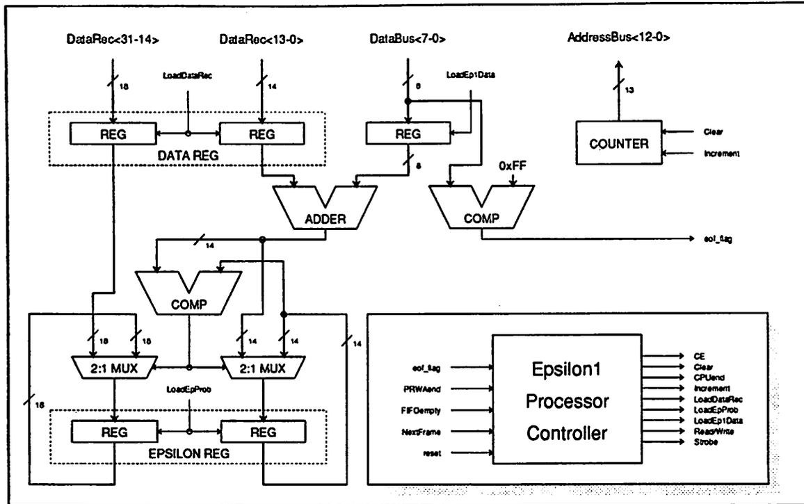
Figure 4.2: Data Path of the Epsilon Processor
