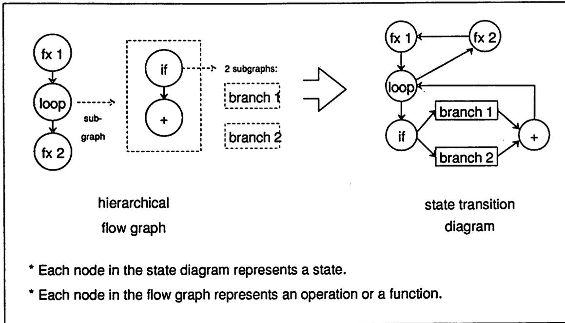
Figure 2.16: An Example of State Transition Diagram Generation
