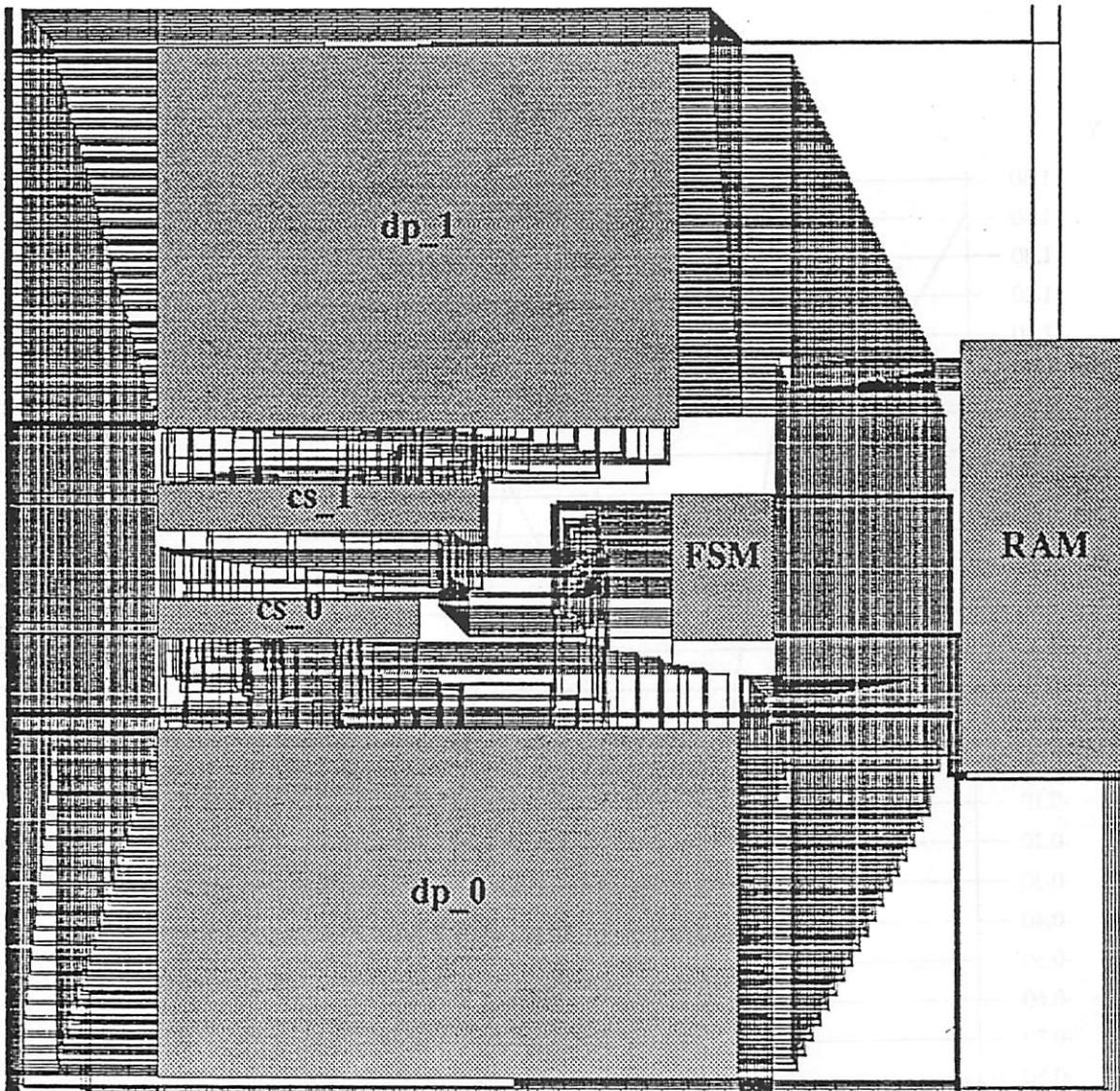
Figure 4.18: Layout of the CORDIC Example
