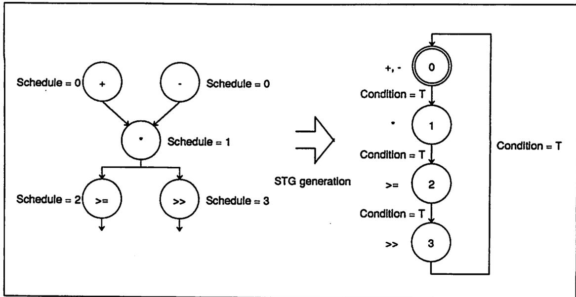
Figure 2.14: State Transition Diagram Generation
