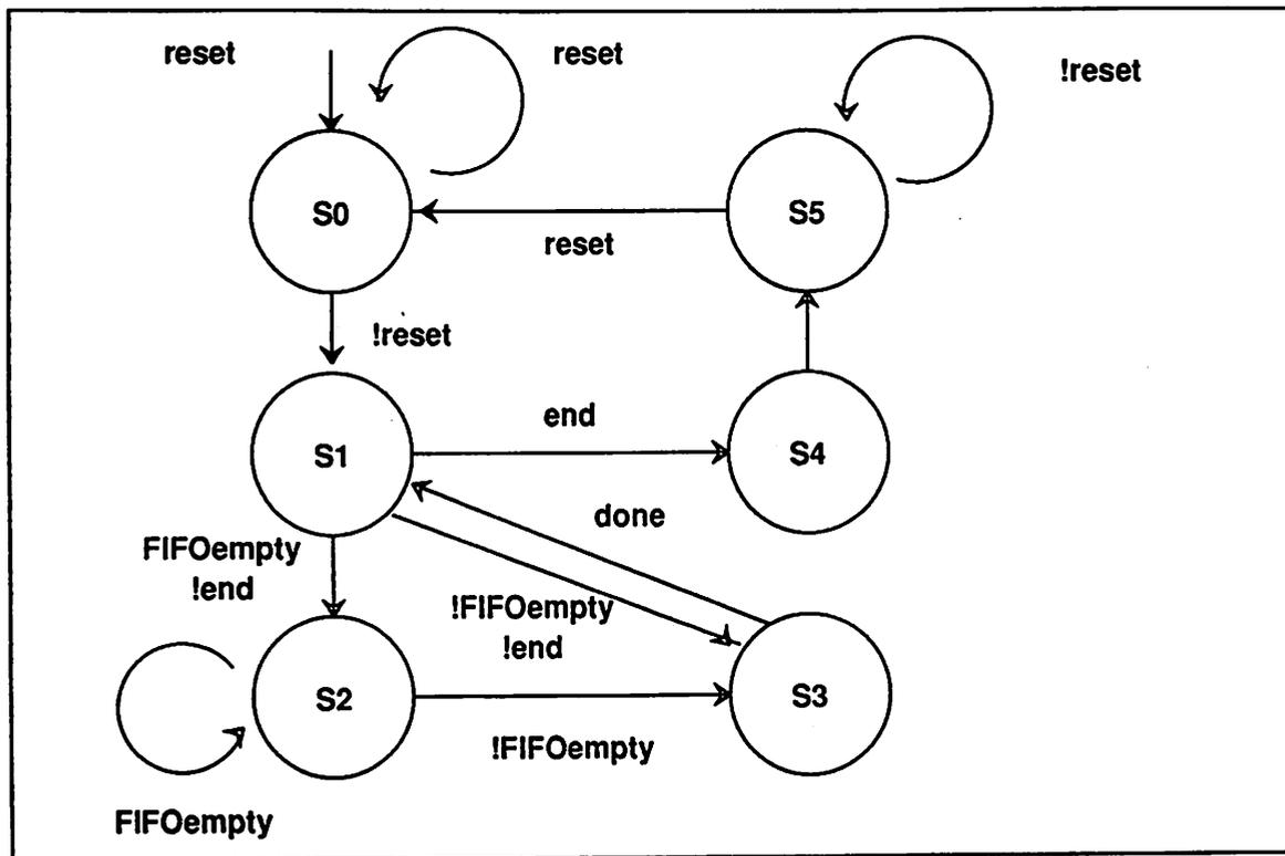
Figure 4.3: State Transition Diagram of the Epsilon Processor
