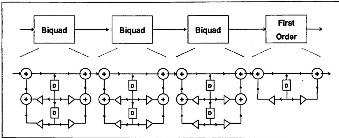
Figure 4.9: Flow Graph of the 7th Order IIR Filter
