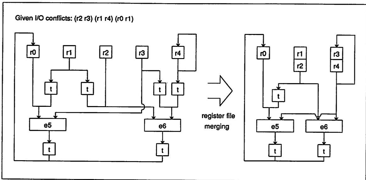
Figure 2.9: Optimal Register File Structure for Toy
