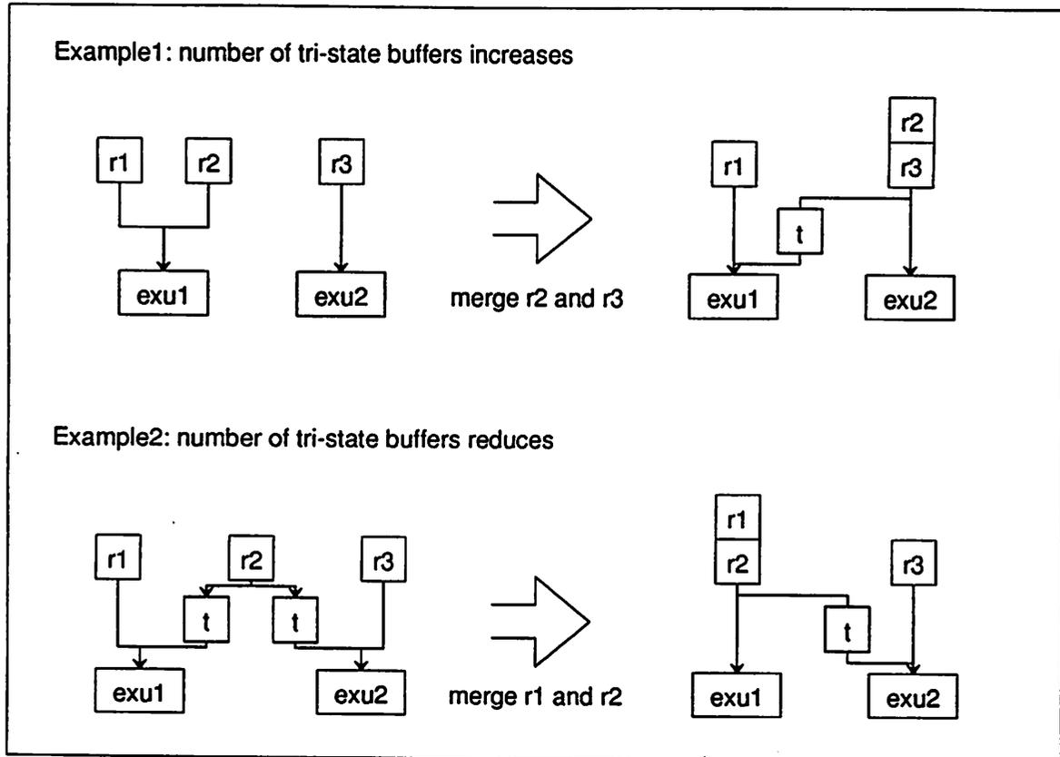
Figure 2.6: Multiplexer Increasing/Decreasing Due to Register File Merging
