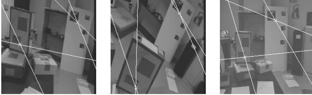
Figure 6: Three images taken by a zooming camera, with epipolar lines
