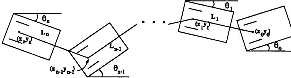
FIGURE 4. The N-trailer system, with a steering wheel at the front of the chain.
