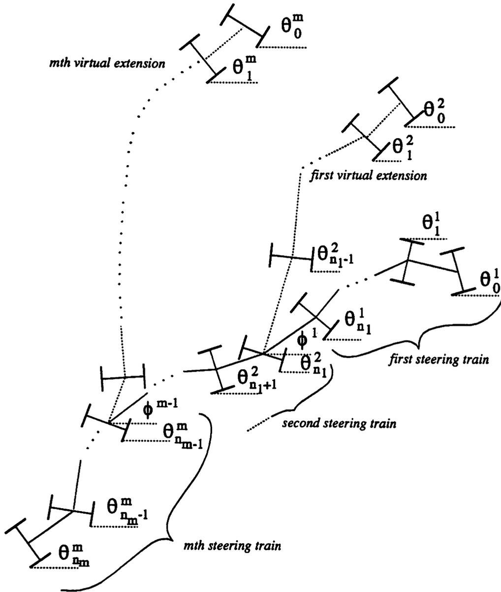
FIGURE 7. The multi-steering system, showing the virtual axes that must be added to convert the system into multi-input chained form.
