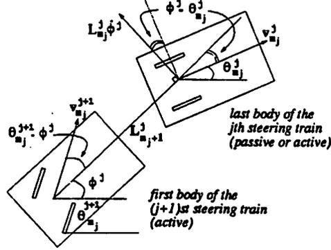
FIGURE 3. Showing the velocity relationships between two bodies when the rear body is an active car.
