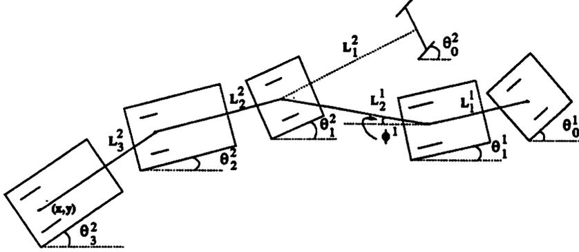
FIGURE 9. The five-axle, two-steering system showing the virtual extension which is added in front of the second steering wheel. Such a system could be envisioned as being used in a nuclear power plant or in a mining area where maneuverability around narrow passageways in danger zones is of utmost importance.
