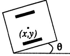
FIGURE 5. The unicycle model. The robot is allowed to drive forwards or backwards and to spin about its center axis.
