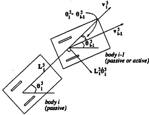
FIGURE 2. Showing the velocity relationships between adjacent bodies when the rear body is a passive trailer.
