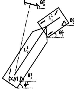
FIGURE 8. A sketch of the fire truck system showing the virtual extension that is added in front of the rear steering wheel. These vehicles are equipped with a long ladder on the trailer and are used by fire departments in large cities in the United States. The extra steering wheel at the rear of the trailer is used for improved maneuverability on narrow city streets.
