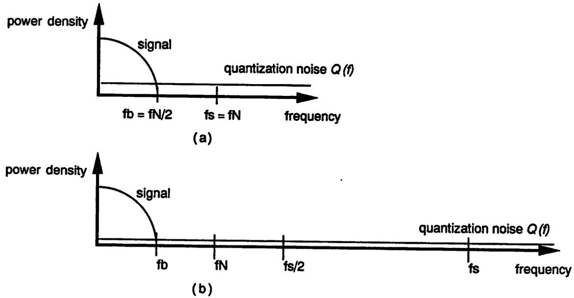
**FIGURE 2.3** Spectral distribution of signal and quantization noise power
