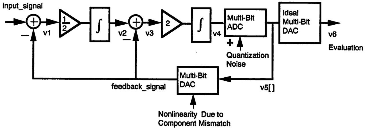
FIGURE 4.4 Block diagram used for the simulation
