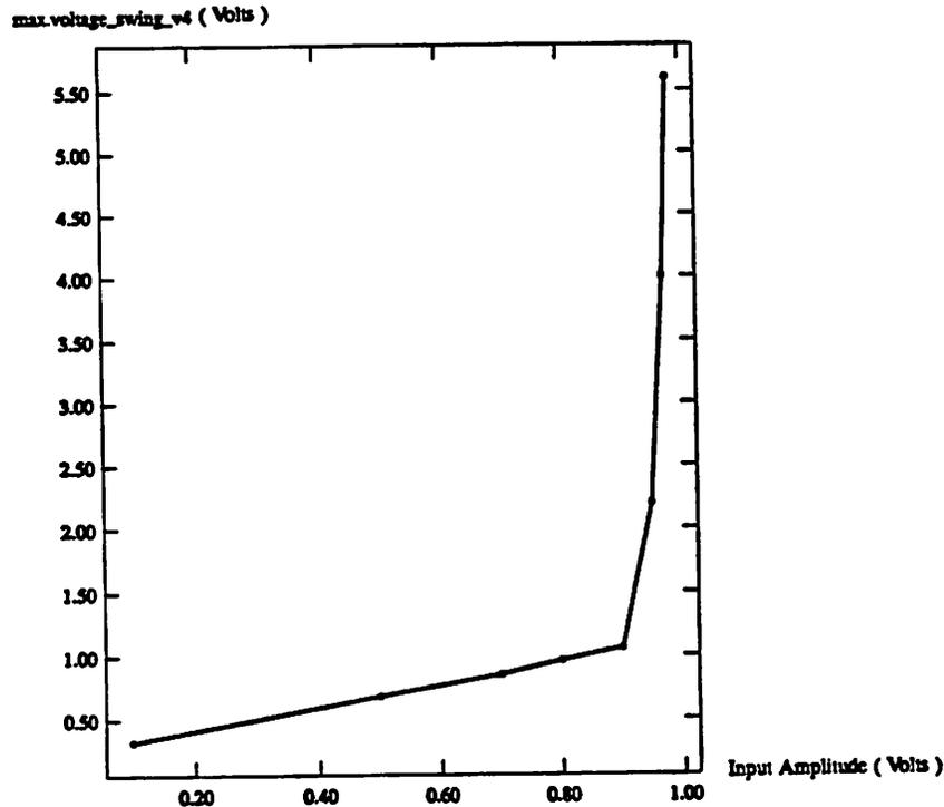
**FIGURE 5.9** Op-amp output swing vs input signal amplitude
