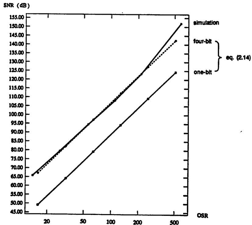
FIGURE 5.4 Signal to Noise Ratio vs Over Sampling Ratio
