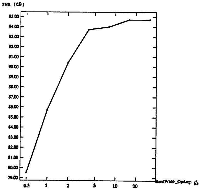
FIGURE 5.6 Signal to Noise Ratio vs op-amp band width
