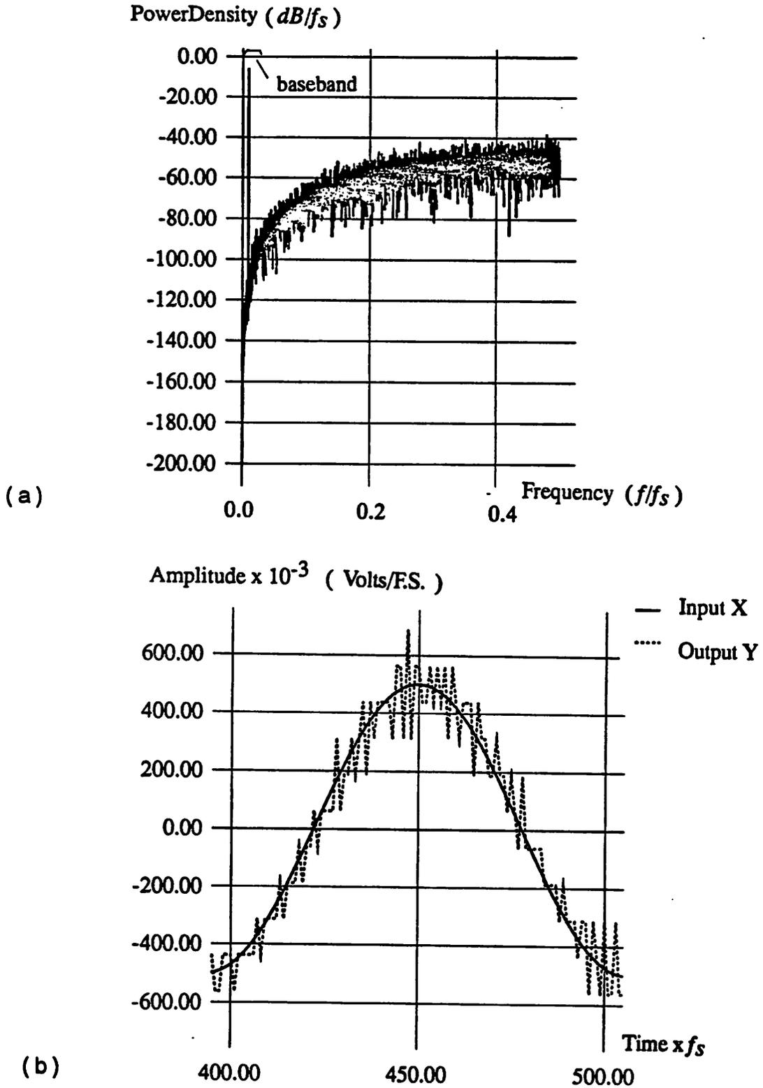
**FIGURE 5.1** Simulation for an input signal equal to -6dB of full scale voltage
