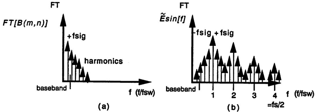
**FIGURE 3.7** Spectrum of the sinusoid input, mismatch and barrel shifting
