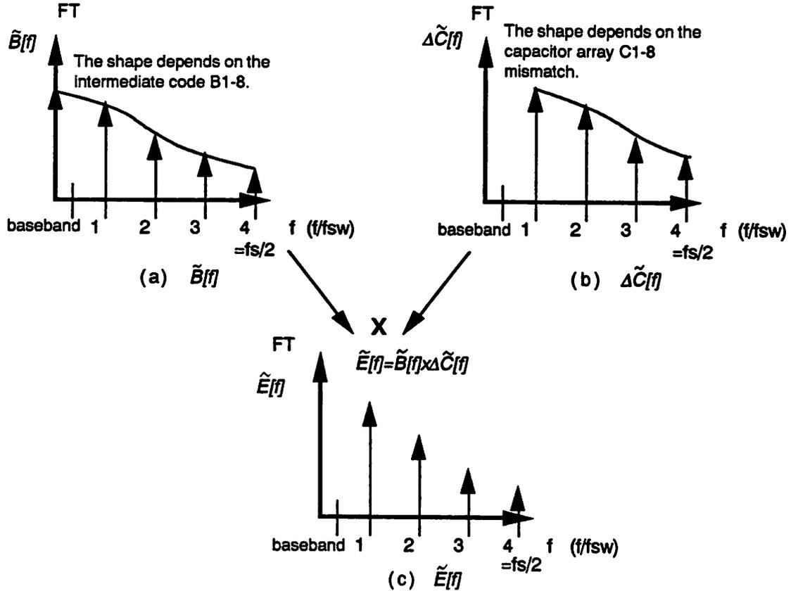
FIGURE 3.6 Spectrum of the output for dc input, mismatch and barrel shifting
