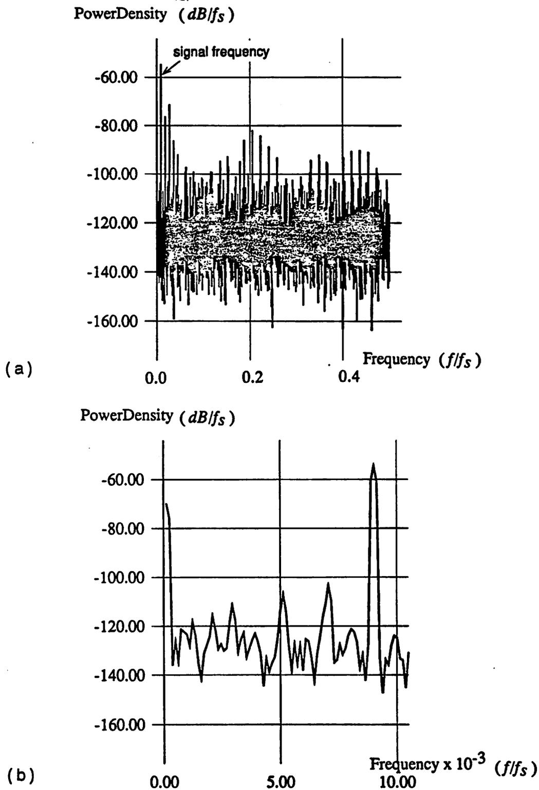
**FIGURE 3.12** Spectral density distribution of the nonlinearity  $\epsilon(z)$  for the open-loop system in Fig. 3.4 CASE 1
