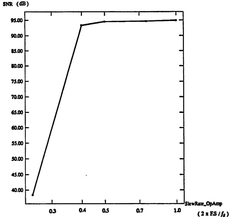
FIGURE 5.7 Signal to Noise Ratio vs op-amp slew rate
