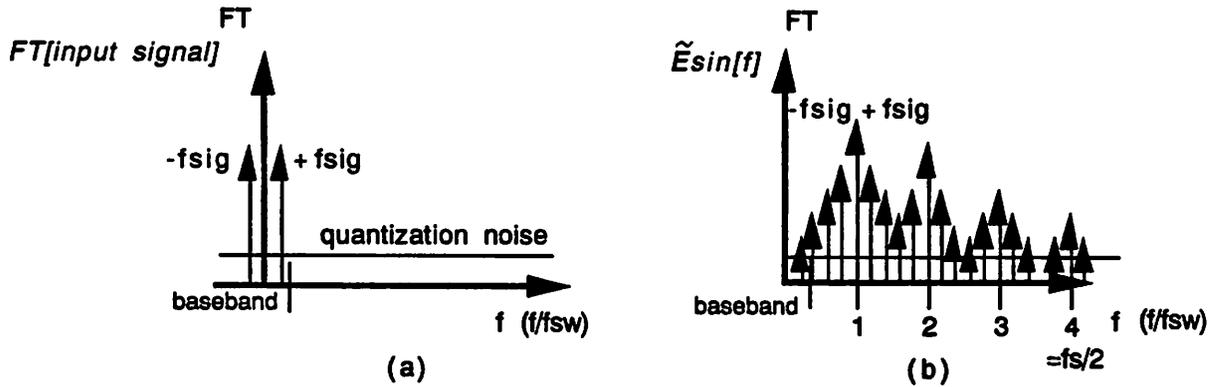
**FIGURE 3.8** Spectrum of the practical input, mismatch and barrel shiting
