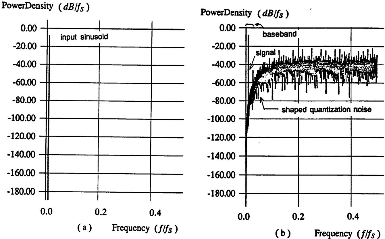
**FIGURE 2.6** Spectral distribution of the output signal  $Y(z)$
