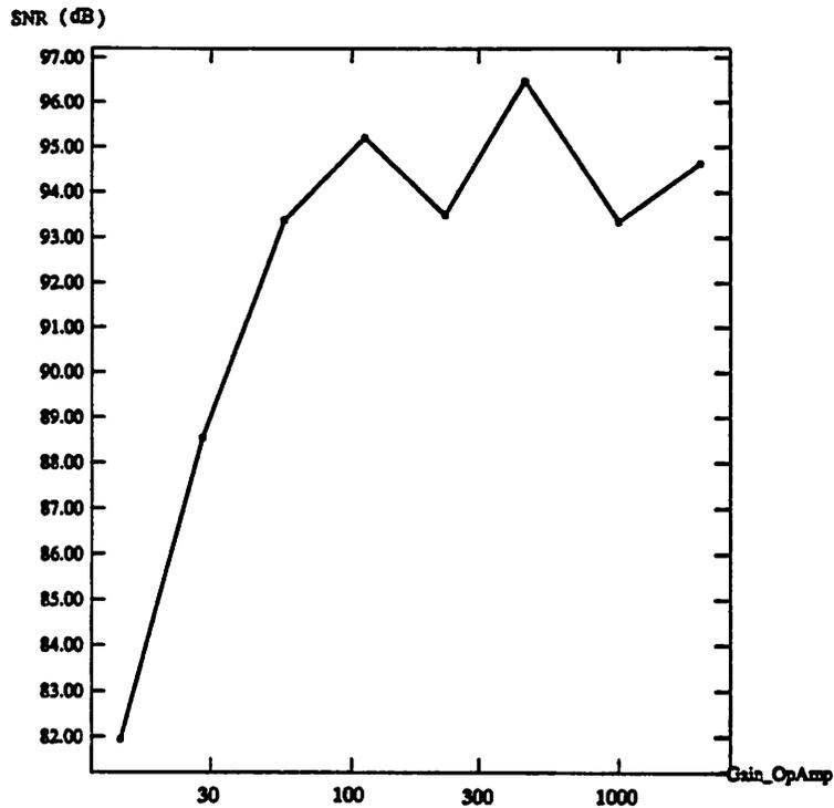
FIGURE 5.5 Signal to Noise Ratio vs op-amp open-loop gain
