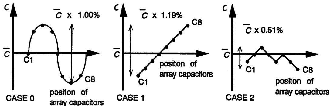
**FIGURE 3.9** Three models of spatial distribution of unit-element values used in the simulation
