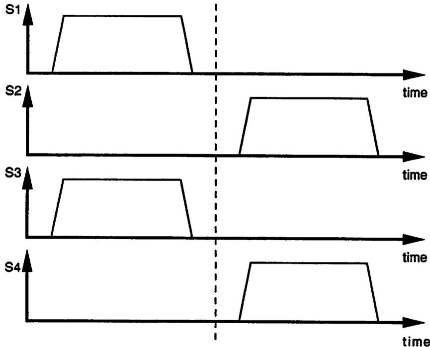
FIGURE 4.2 Non-overlapping two-phase clock
