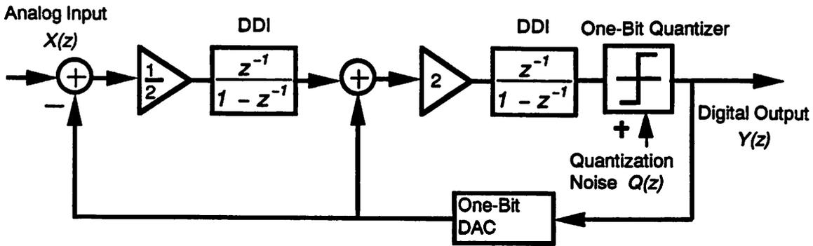
FIGURE 2.8 Block diagram of a second-order  $\Sigma\Delta$  modulator
