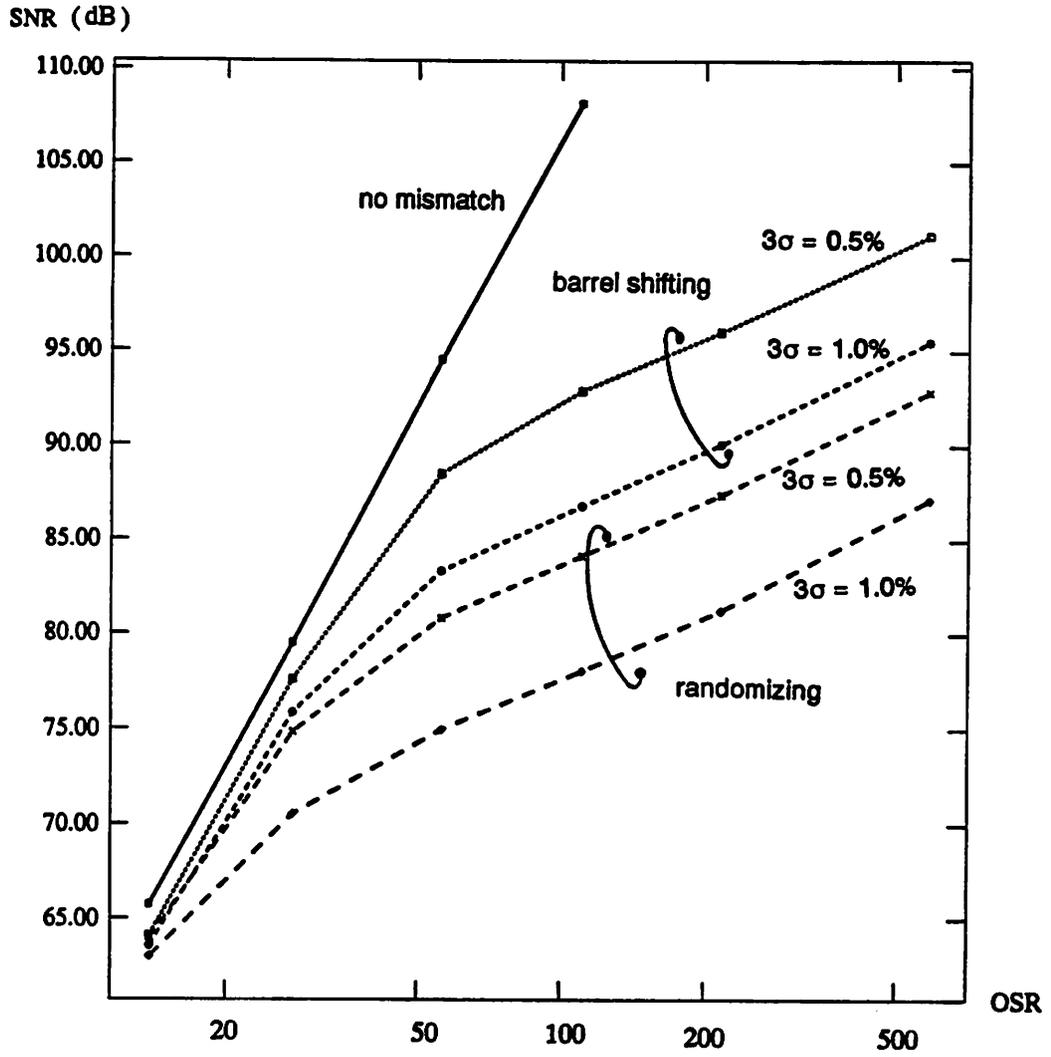
FIGURE 5.15 Signal to Noise Ratio vs Over Sampling Ratio of the four-bit second-order  $\Sigma\Delta$  modulator With randomizing and barrel shifting
