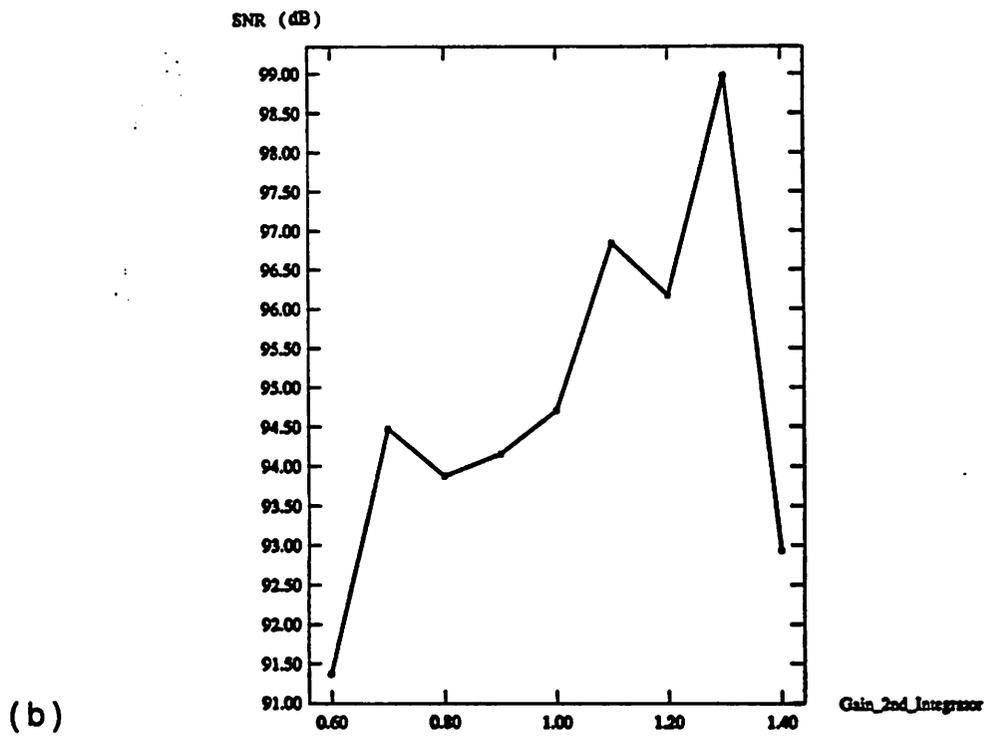
**FIGURE 5.10** Signal to Noise Ratio vs integrator gains
