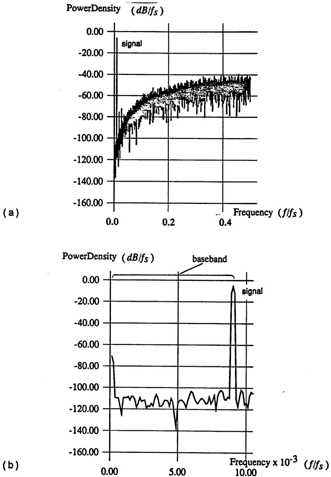
**FIGURE 5.12** Spectral density distribution of the output
