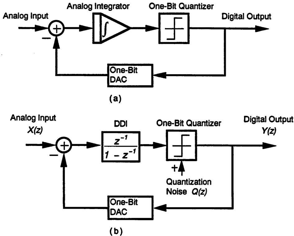
**FIGURE 2.5** Block diagram of a first-order  $\Sigma\Delta$  modulator
