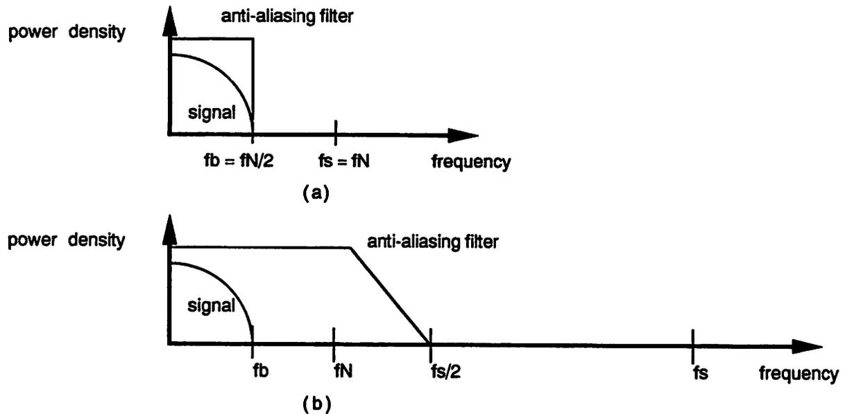
**FIGURE 2.2** Spectral distribution of signal power and filter response
