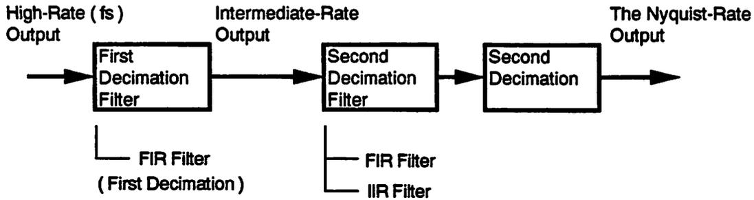
**FIGURE 2.12** Block diagram of the digital decimation filter
