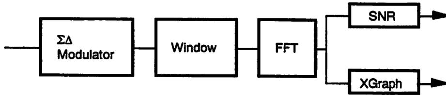
**FIGURE 4.3** Block diagram of the simulation
