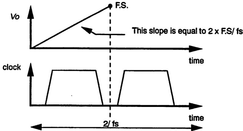
**FIGURE 5.8** Unit of slew rate
