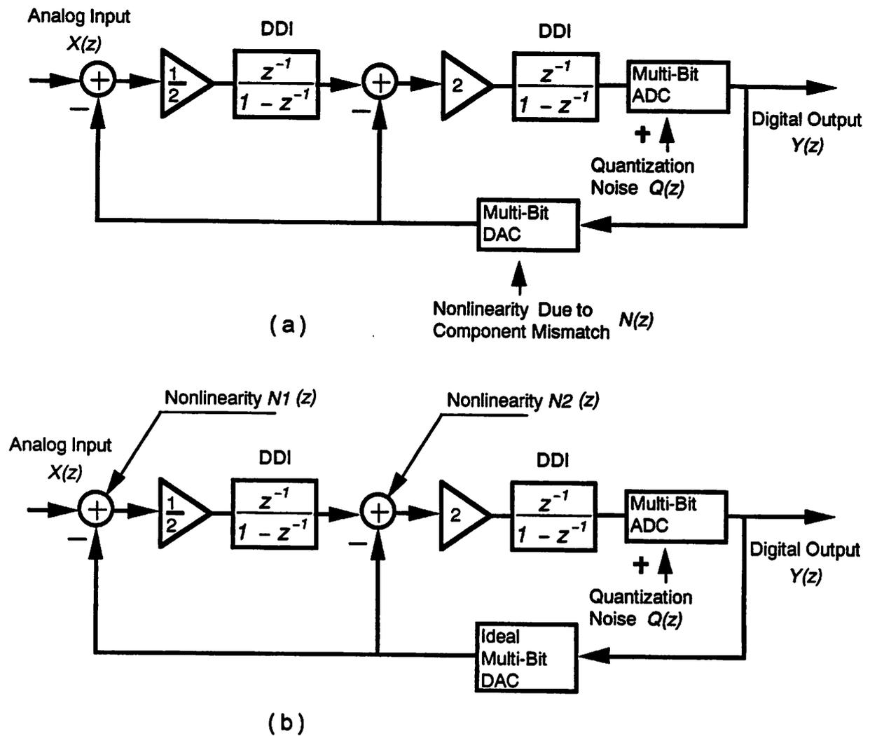
**FIGURE 3.3** Block diagrams of a multi-bit second-order  $\Sigma\Delta$  modulator with nonlinearity
