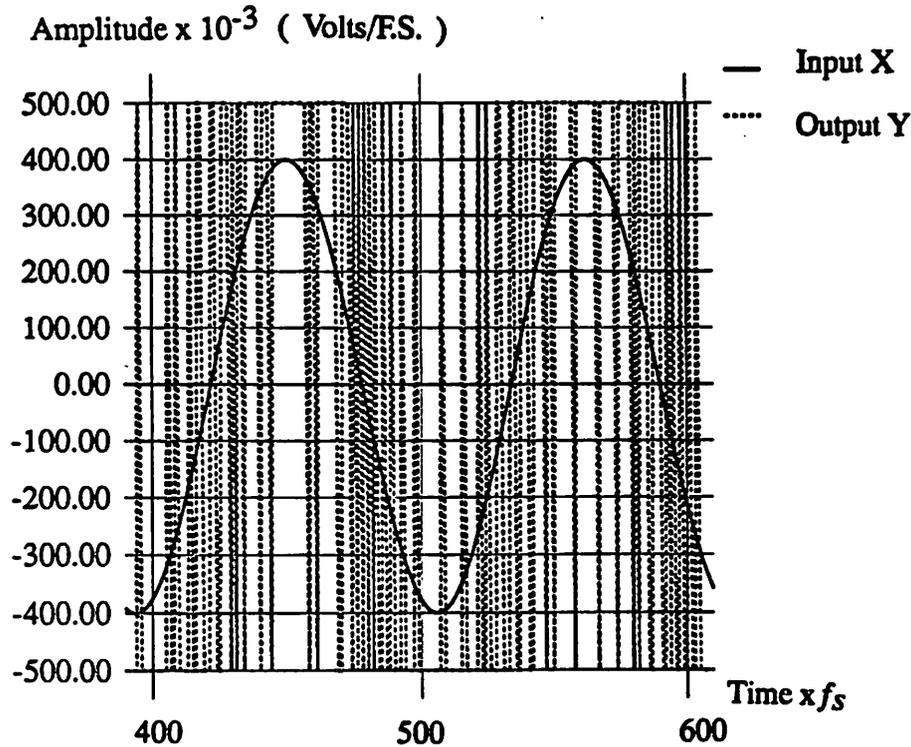
FIGURE 2.7 Time-domain waveforms of signals of a  $\Sigma\Delta$  modulator
