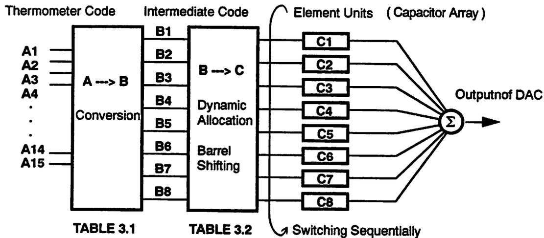
FIGURE 3.2 Block diagram of dynamic allocation of an internal DAC
