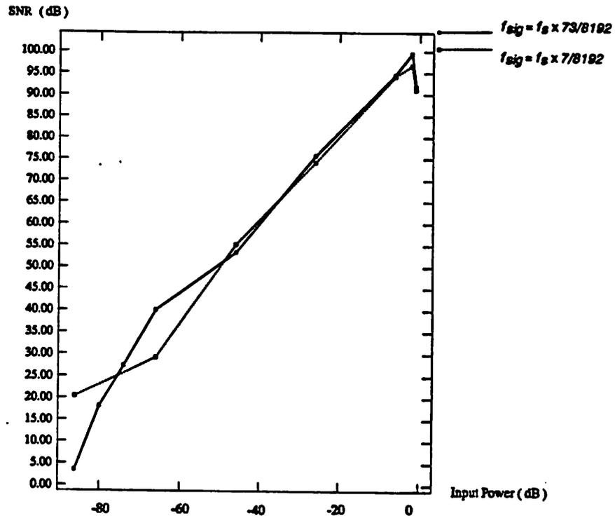
FIGURE 5.3 Signal to Noise Ratio vs input signal amplitude
