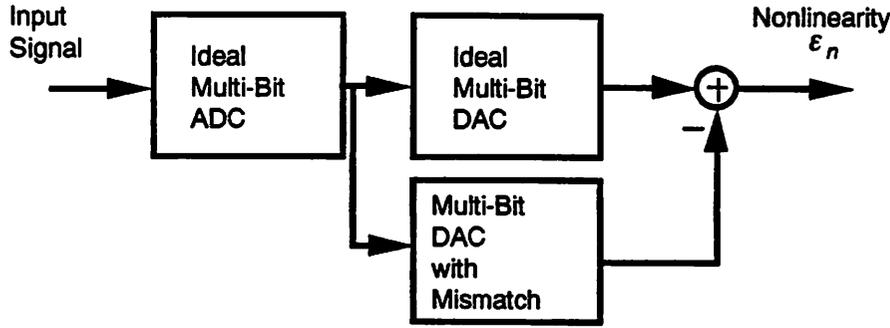
FIGURE 3.4 Cascade of an ADC and a DAC
