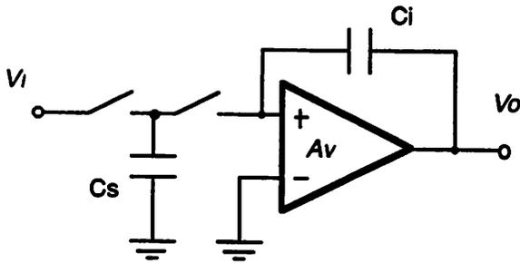
FIGURE 4.5 Diagram of a switched capacitor integrator
