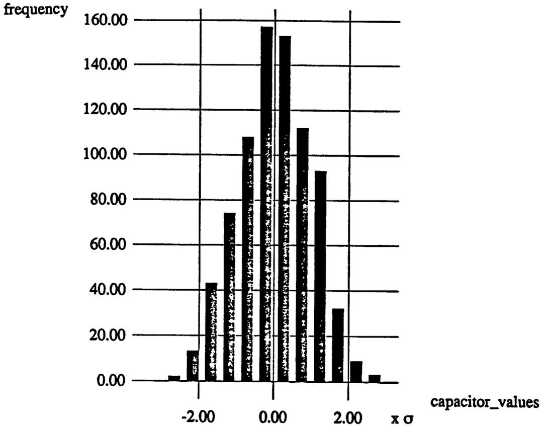
FIGURE 4.7 Distribution of capacitor values used in the simulation
