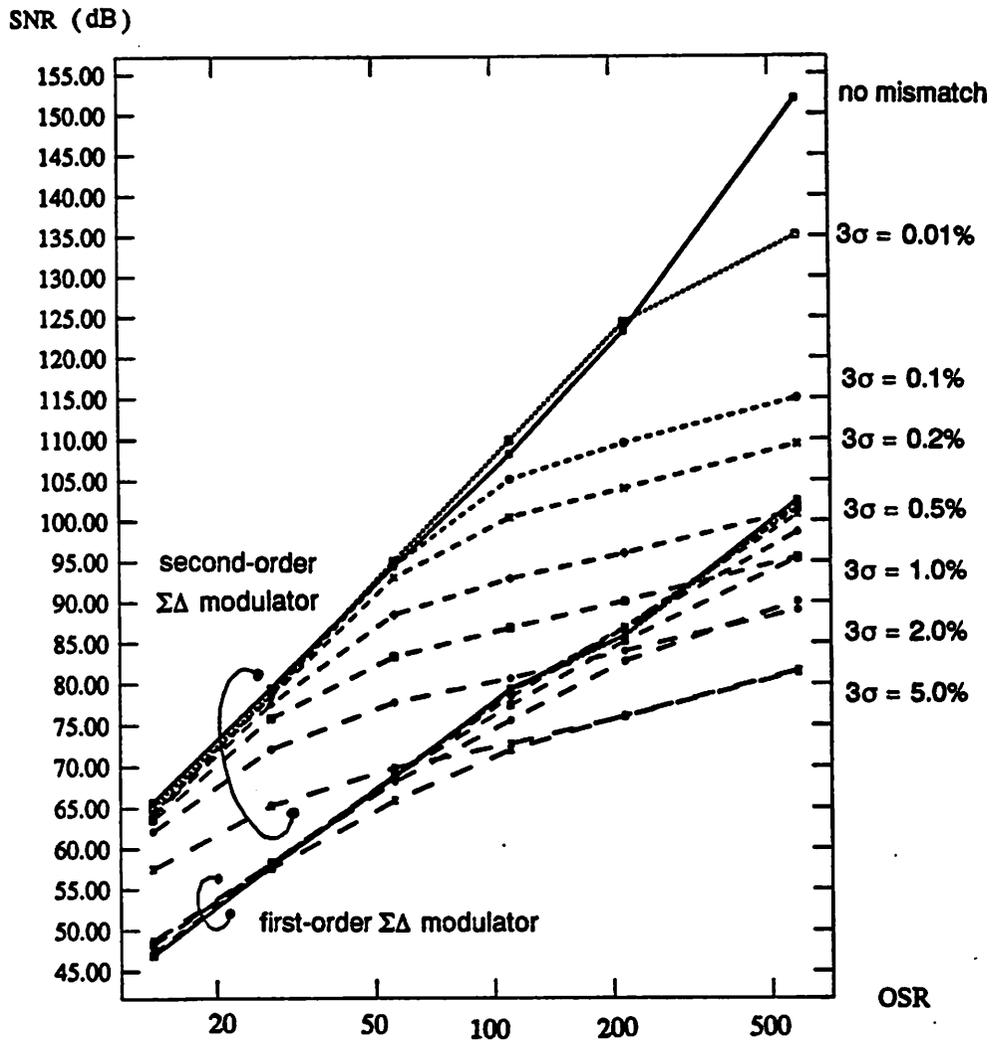
FIGURE 5.17 Signal to Noise Ratio vs Over Sampling Ratio of the four-bit first-order  $\Sigma\Delta$  modulator
