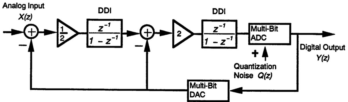
FIGURE 3.1 Block diagram of a multi-bit second-order  $\Sigma\Delta$  modulator
