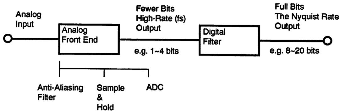
FIGURE 2.4 Basic architecture of oversampled A/D converters
