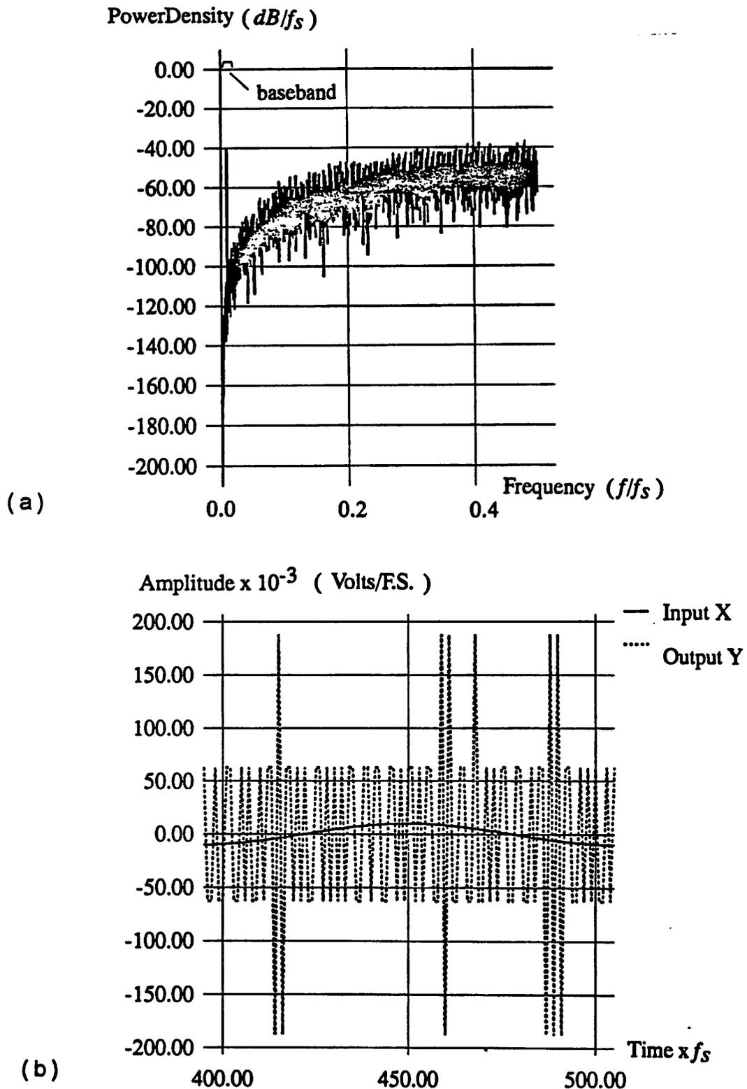
**FIGURE 5.2** Simulation for an input signal equal to -40dB of full scale voltage
