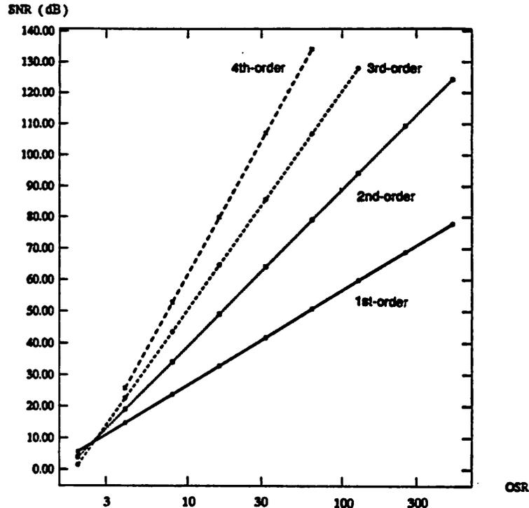
FIGURE 2.9 The signal to noise ratio SNR vs the oversampling ratio OSR
