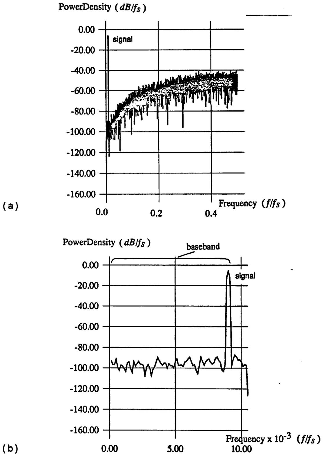
**FIGURE 5.13** Spectral density distribution of the output
