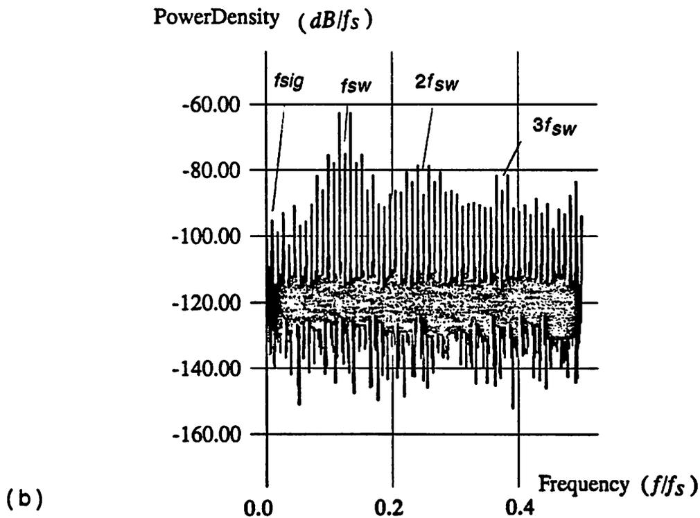
Note : Power density is specified relative to a F.S. sinusoid.
