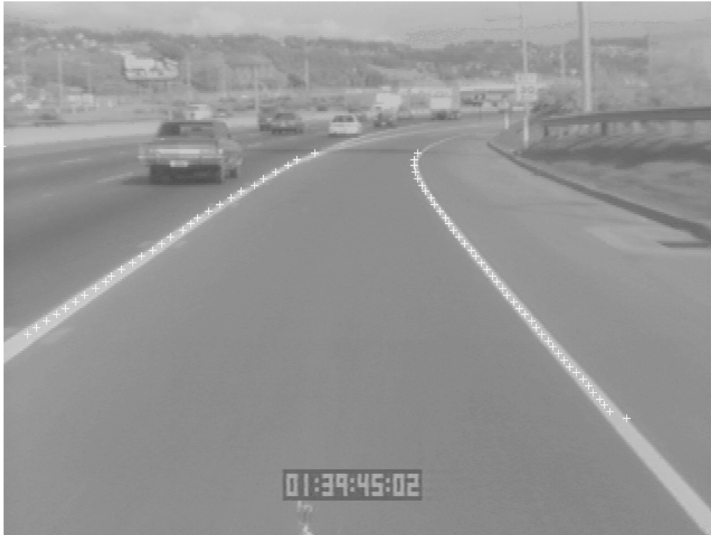
Figure 8: The initialization of the algorithm is done by detection of portions of straight lines of common orientation (top left). Within the search zone predicted using current the current lane markers parameters (top right), a precise model-based localization of lane markers points is performed (bottom).
