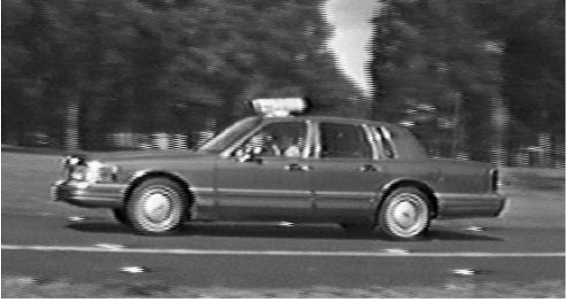
Figure 10: The Lincoln towncar with which we recorded test sequences on highways using the stereo camera rig mounted on top of the roof.
