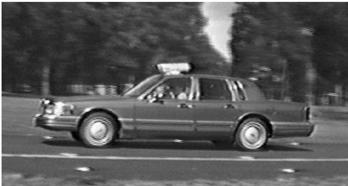
Figure 10: The Lincoln towncar with which we recorded test sequences on highways using the stereo camera rig mounted on top of the roof.
