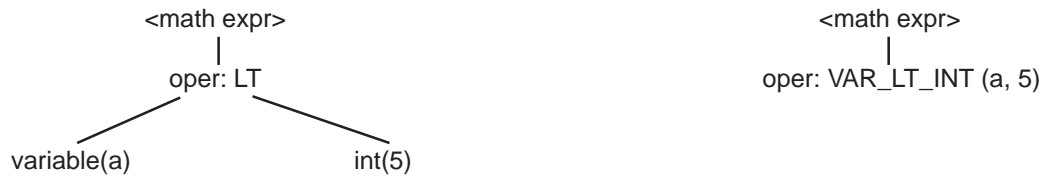
Figure 11: abstract syntax tree for { $a < 5 } , without compression (left) and with compression (right).
