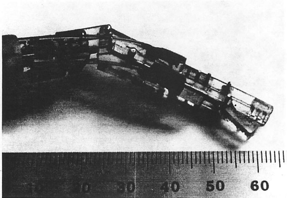
Figure 12: Hydraulic end-effector with two degrees of freedom.
