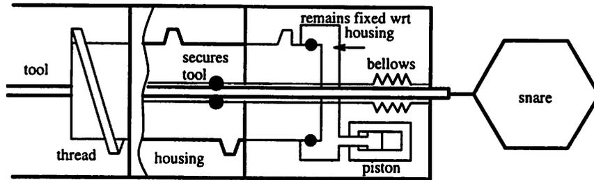
Figure 2: Rotary screw actuator.
