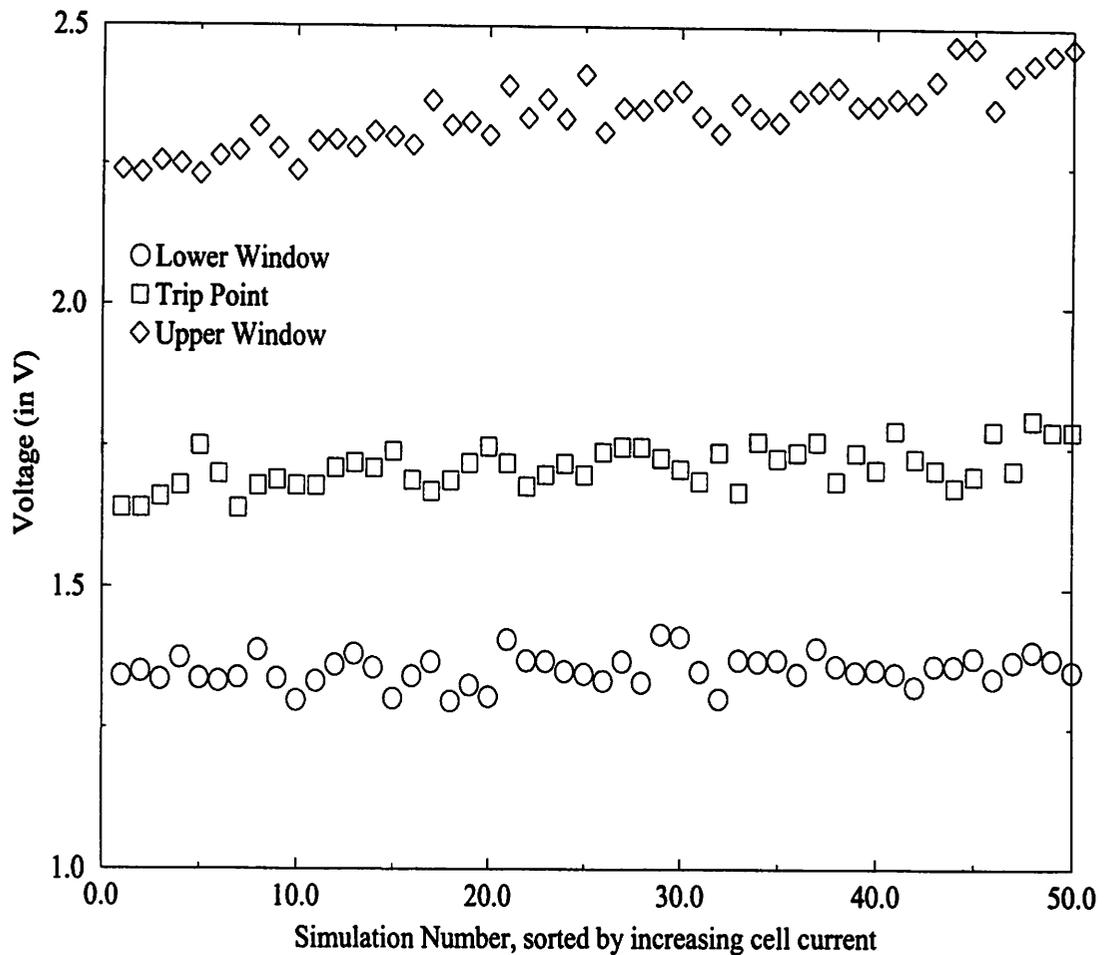
**Figure 6-11** Monte Carlo: Window Levels for Sense Amplifier - New Design
