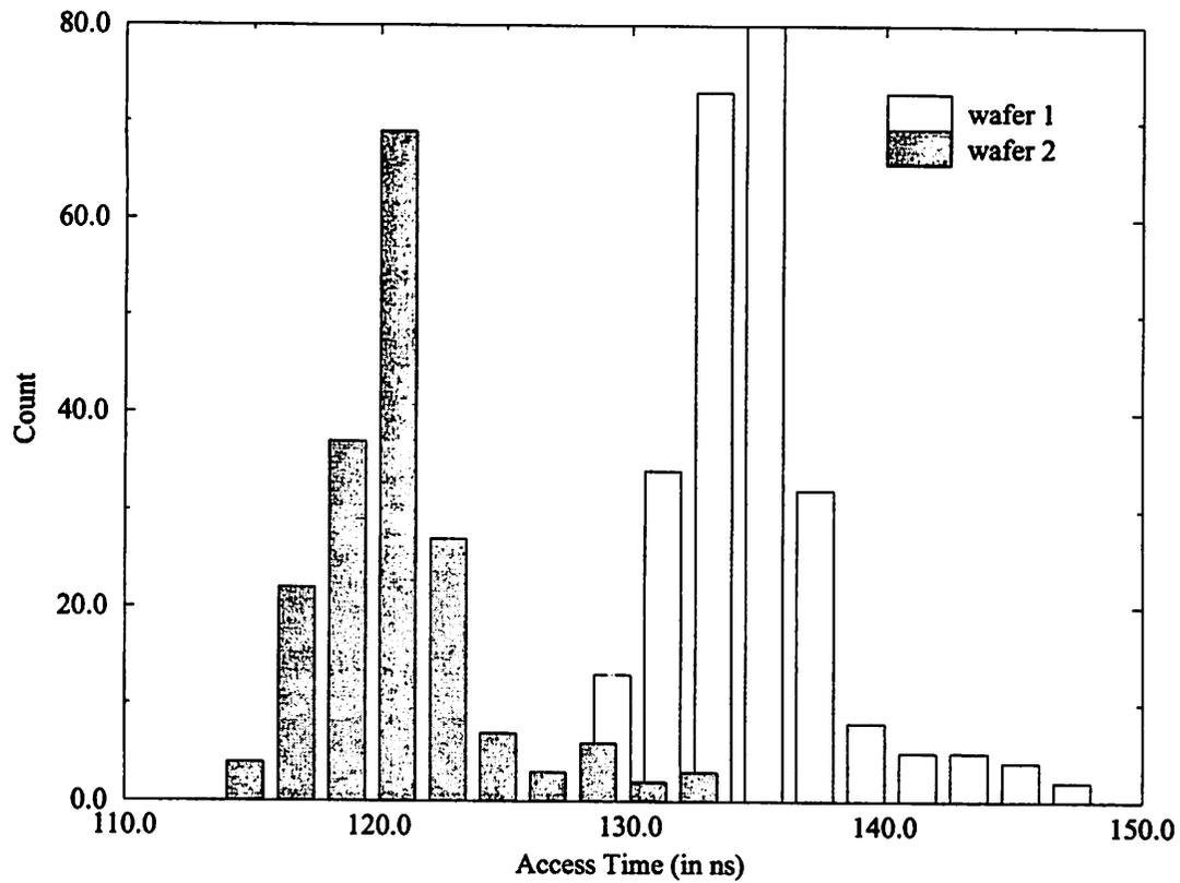
**Figure 4-3** Detailed Histogram of Product Performance for Two Wafers
