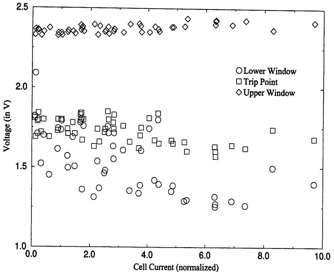
**Figure 6-14** Monte Carlo Simulation Including Mismatch: Window Levels for Sense Amplifier - Original Design
