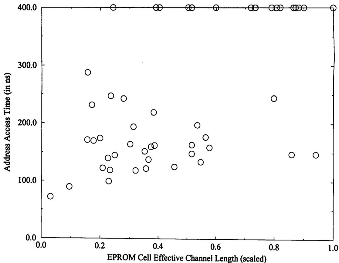
**Figure 6-2** Monte Carlo Result: Address Access Time versus Effective Channel Length for 1 Mbit EPROM
