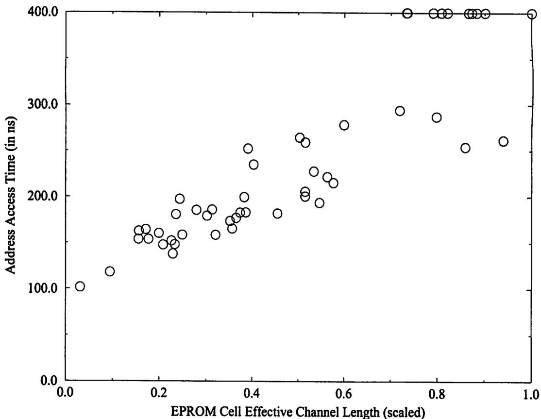
**Figure 6-3** Monte Carlo Result Varying only Channel Length: Address Access Time versus Effective Channel Length for 1 Mbit EPROM
