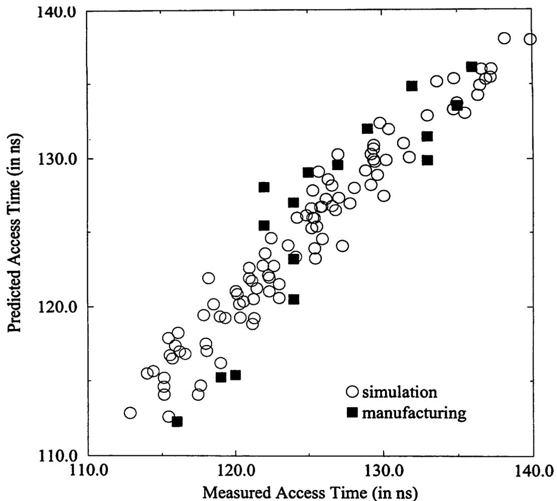
**Figure 6-5** Predicted vs. Measured Access Time, Simulation and Manufacturing Data
