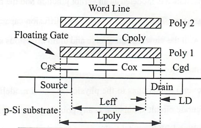
**Figure 5-2** EPROM Cross-Section and Floating Gate Capacitance Model
