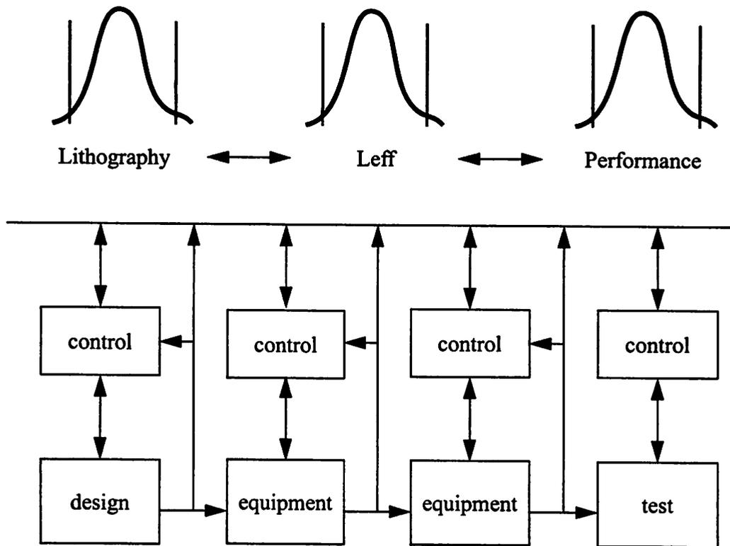
**Figure 4-2** Process Control and Manufacturability
