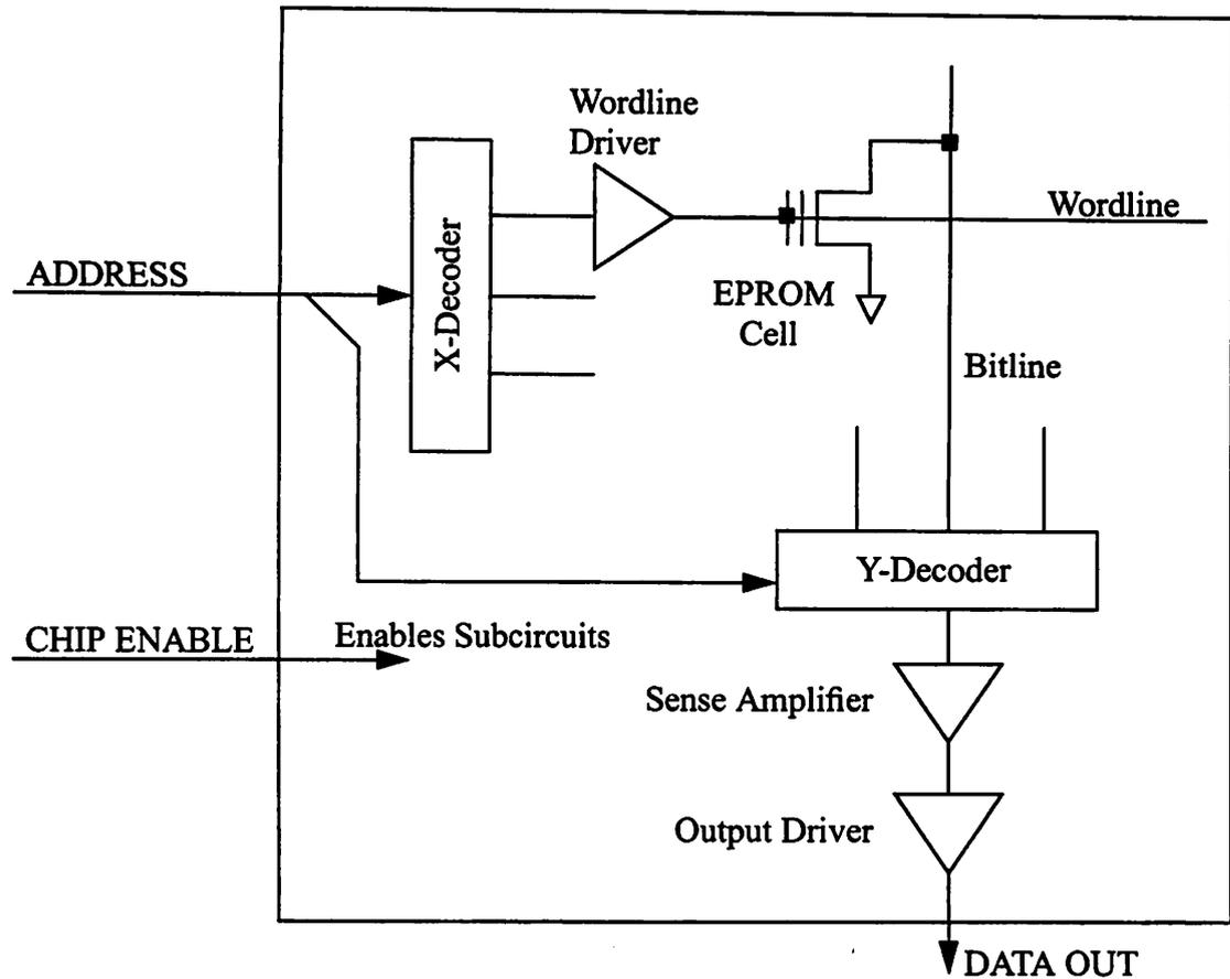
Figure 6-1 Schematic Overview of an EPROM
