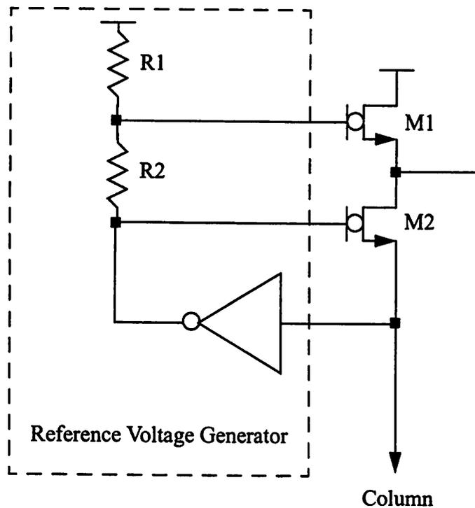
**Figure 6-10** Reference Voltage Generator Equivalent Circuit
