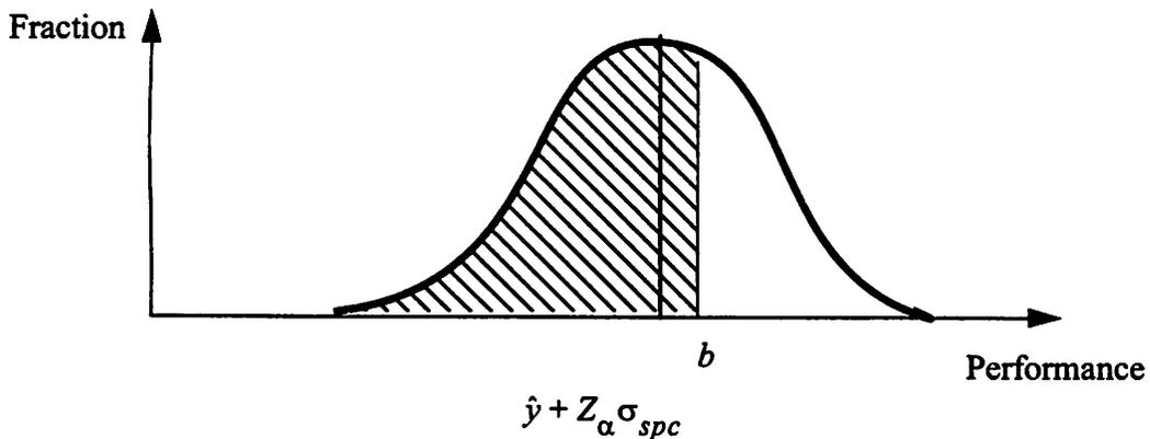
Calculation of the lower control limit for lower bin.
