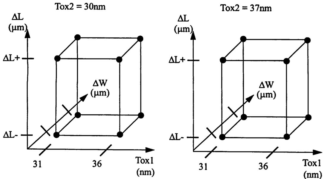
Figure 6-4 Factorial Design for Model Verification
