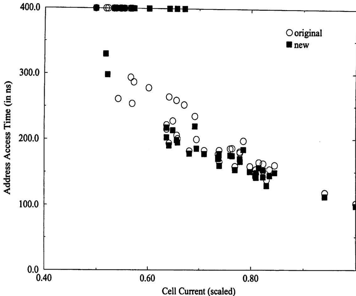
**Figure 6-13** Monte Carlo Varying Only Channel Length: Read Access Time versus Cell Current - Original and New Designs
