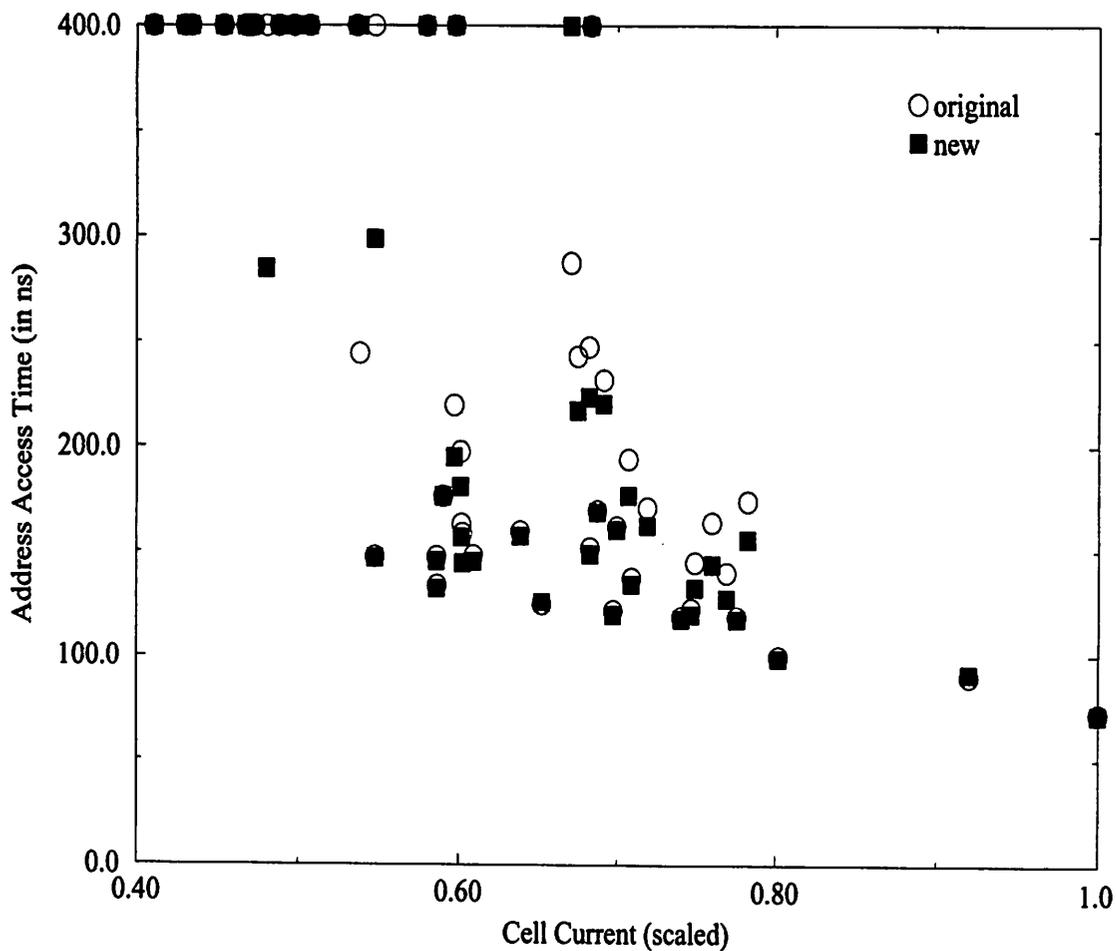
**Figure 6-12** Monte Carlo: Read Access Time versus Cell Current - Original and New Designs
