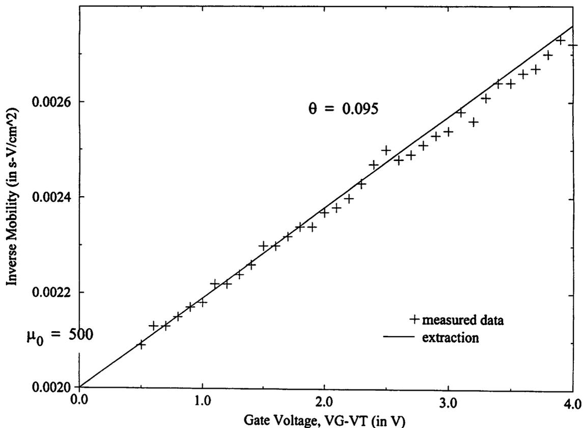
**Figure 5-1** Extraction of Mobility and Mobility Degradation
