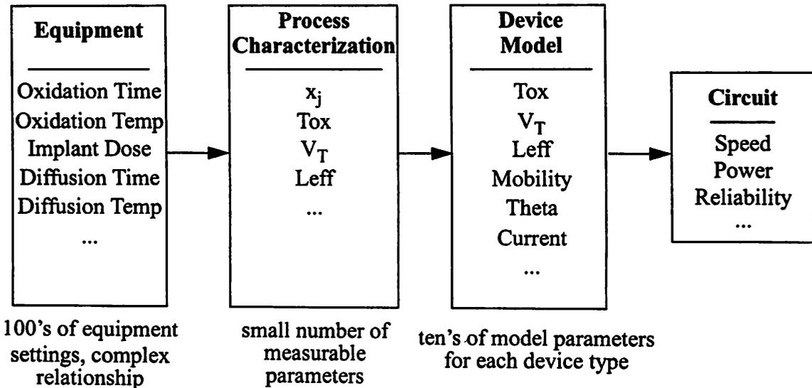
**Figure 3-3** Manufacturability Modeling Regimes (MOS process example)
