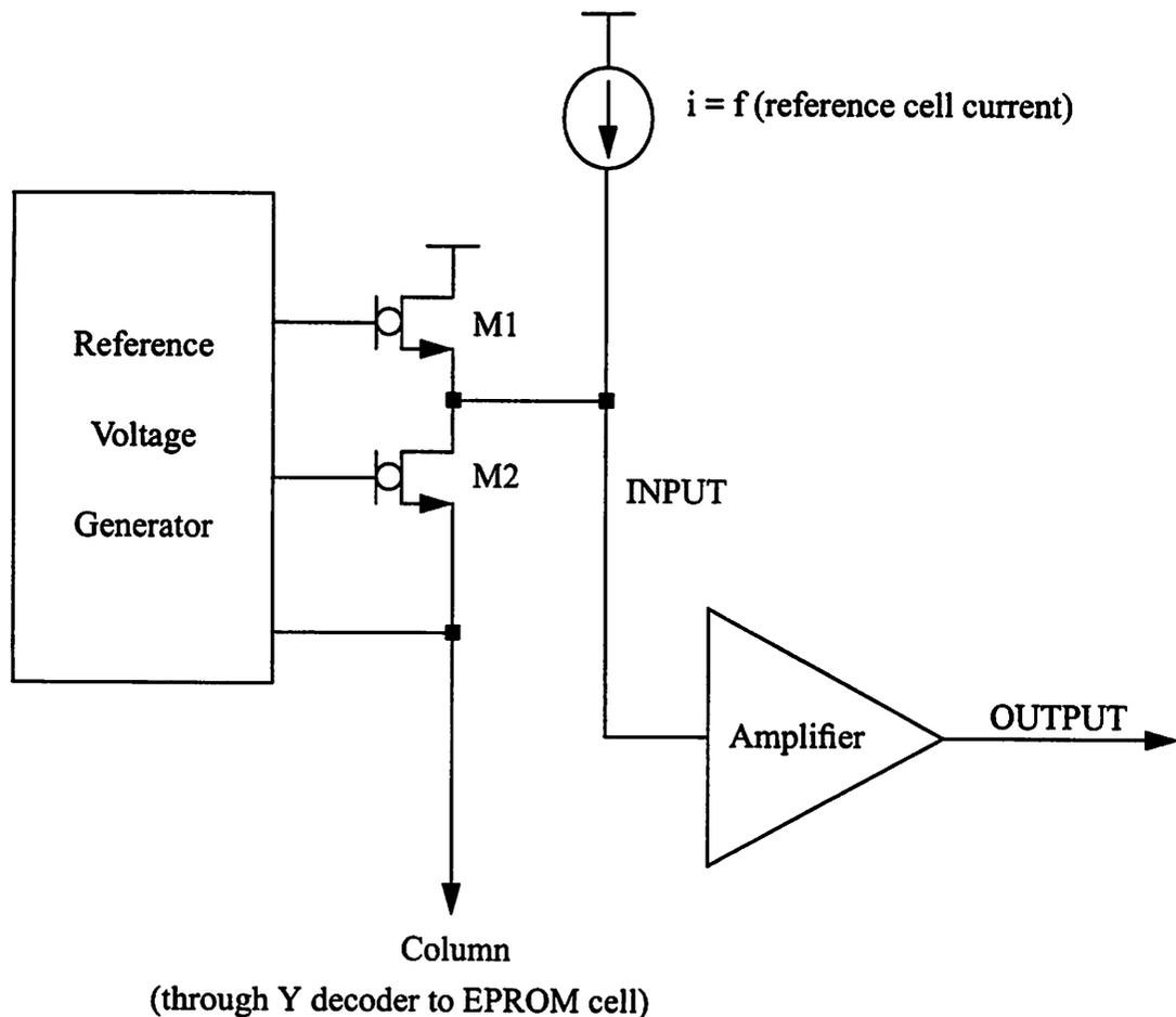
NOTE: The devices with a circle between the gate and body are zero threshold devices.
