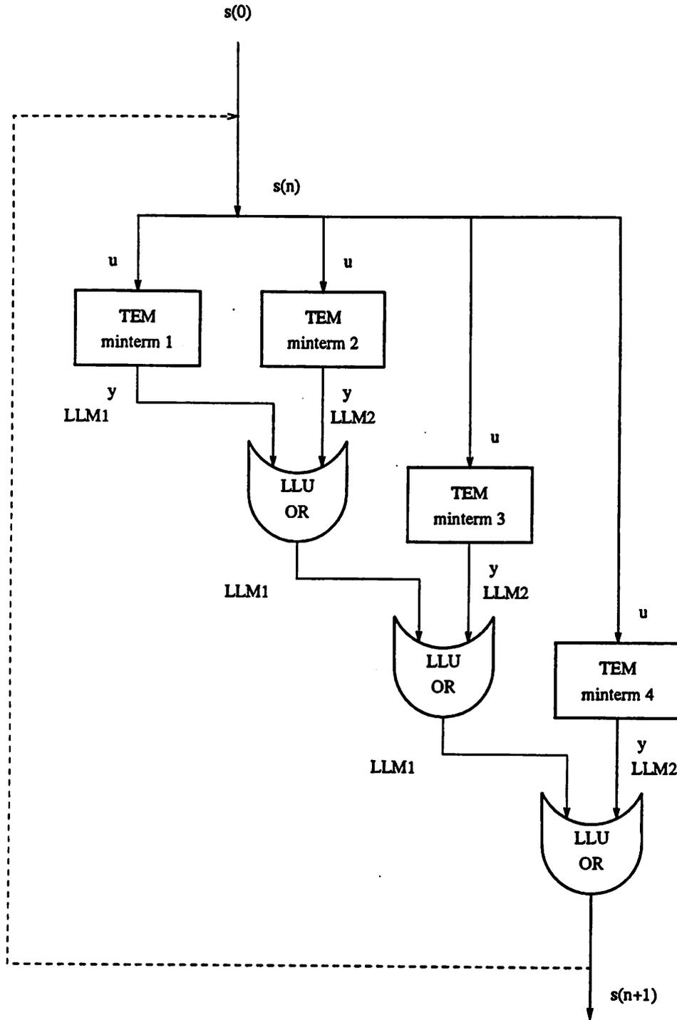
Figure 3: A flow chart of the CNN Universal Machine Algorithm for implementing a cellular automata with a 4-minterm state transition function. The structure can be extended indefinitely. In general the TEM blocks can be any linearly separable boolean operation.
