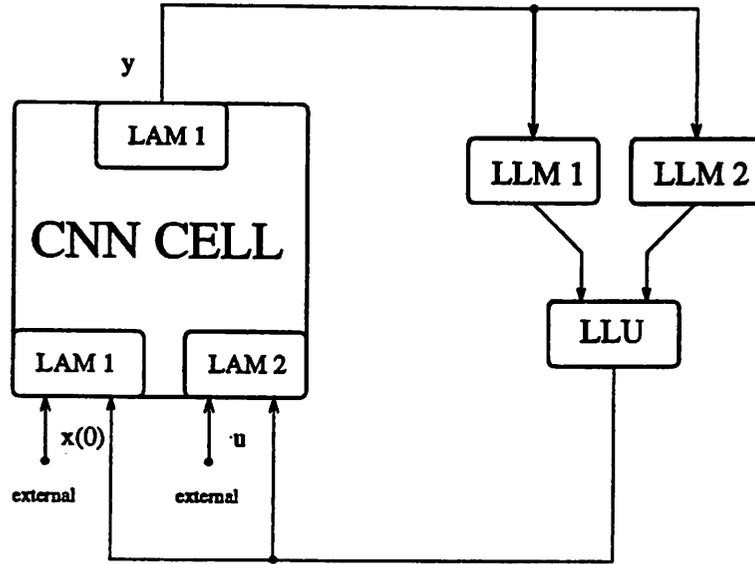
Figure 1: A simplified CNN Universal Machine register transfer diagram, with the obvious implicit multiplexing. The main features are the CNN cell where the analog transient occurs, the Local Analog Memories (LAM) which hold state and input, the Local Logic Memories (LLM) which can each store a binary value for each cell, and the Local Logic Unit (LLU) which can perform arbitrary intra-cell logic functions on the contents of the LLM.
