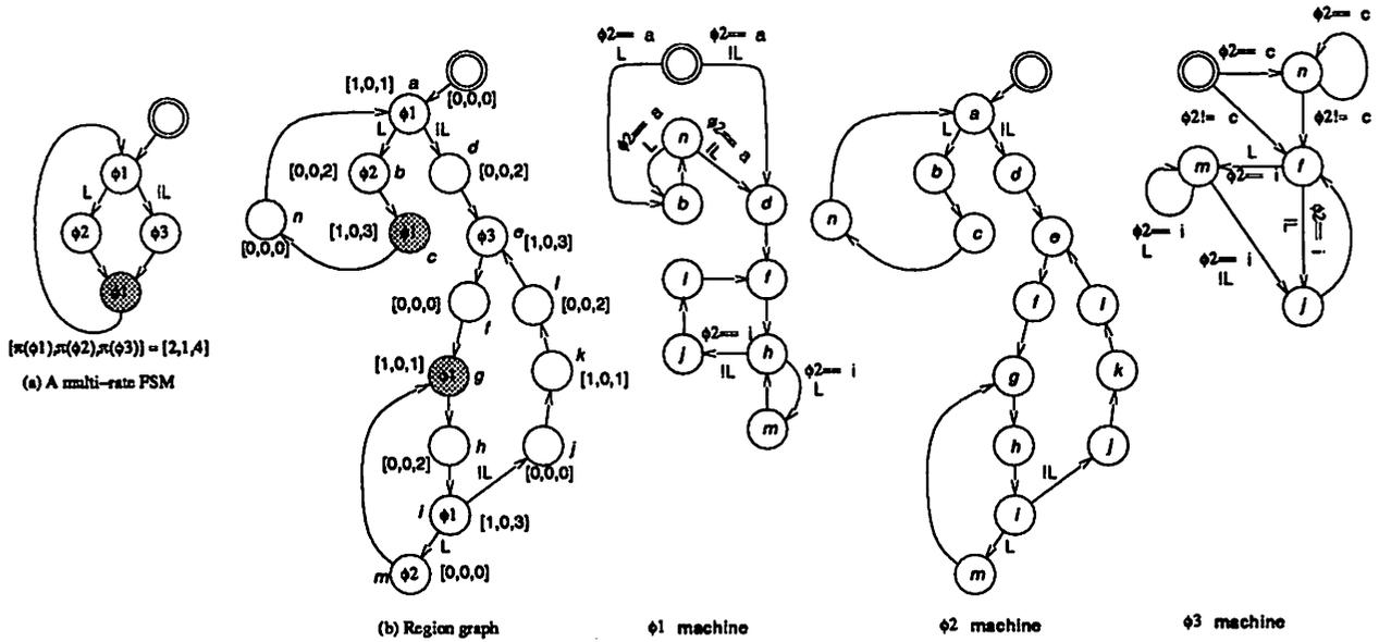
Figure 1: A multi-phase FSM, its region graph, and extracted single-phase FSMs.
