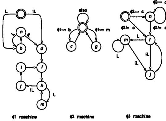
Figure 3: Relabelling  $\phi_1$  and  $\phi_3$  in Figure 1 to optimize the single-phase FSM for  $\phi_2$ .
