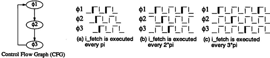
Table 1: A multi-phase system in Verilog/VHDL and the impact of clock configurations on system behavior.
