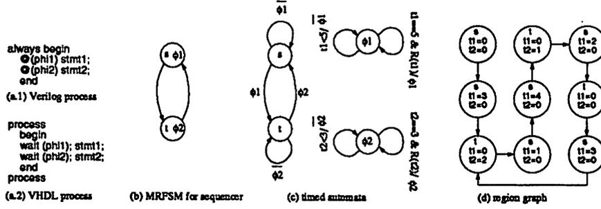
Figure 2: Region expansion and multi-phase FSM of a hardware description language (HDL) process.
