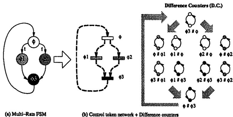
Figure 4: Decomposing a multi-phase FSM into a token network and difference counters.
