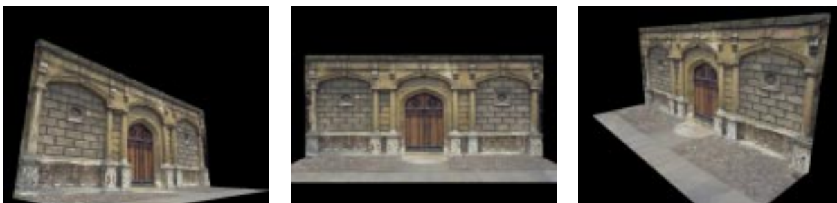
Figure 19: Novel views of the scene generated from four original photographs. These are frames from an animated movie in which the façade rotates continuously. The depth is computed from model-based stereo and the renderings are made using image-based rendering combined with view-dependent texture-mapping.
