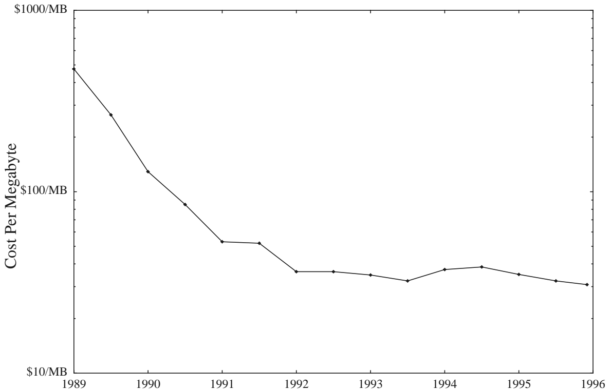
FIGURE 2-2. DRAM price per megabyte. Each point indicates the cost per megabyte of DRAM memory based on advertisements from Byte magazine. All prices reflect memory purchased in 9-bit-wide SIMM form with access times of 80 ns or better. To provide the best price for each data point, points before July of 1991 are the prices for 1MB SIMMs, and points from July of 1991 and later are one quarter of the prices of 4 MB SIMMs. Note the log scale for the y axis.
