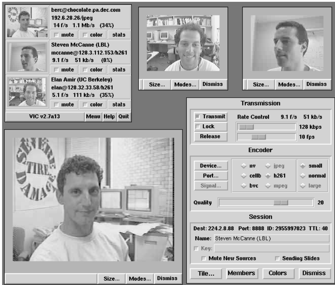
Figure 7.4: Vic's User Interface. The video-only user interface consists of three window types: a thumbnail listing in the upper left corner, a control panel in the lower right corner, and viewing windows.
