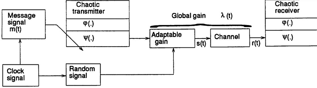
Figure 2: Block diagram of a GS-based secure communication scheme.
