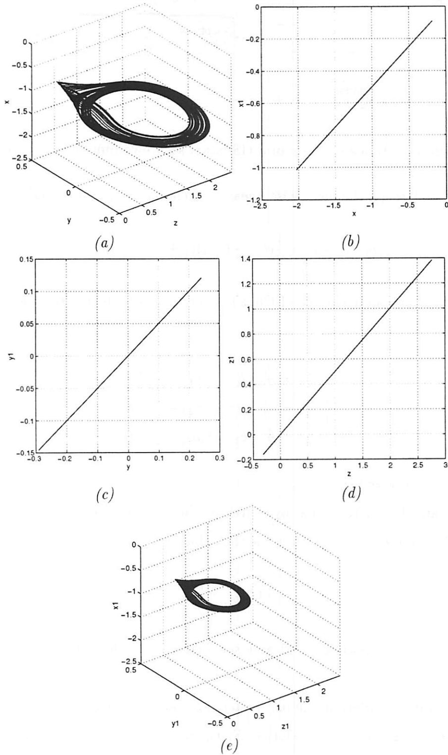
Figure 1: Simulation results with a linear channel with unknown gain. (a) Attractor of the driving system. (b) the  $x - x_1$  GS plot. (c) the  $y - y_1$  GS plot. (d) the  $z - z_1$  GS plot. (e) Corresponding attractor of the driven system.
