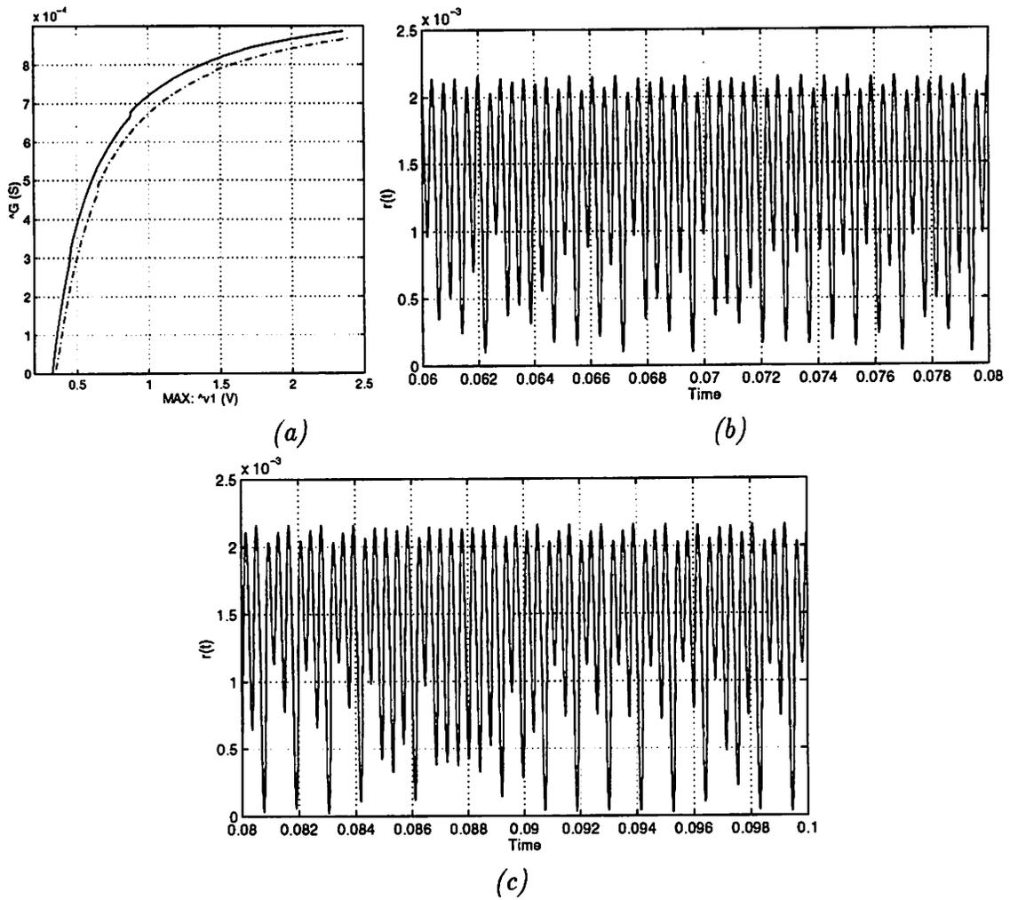
Figure 3: Bit detection maps corresponding to two qualitatively similar waveforms. (a) The difference between the two  $|\hat{v}_1| - \hat{G}$  plots corresponding to the two parameter sets for coding bit-0 and bit-1. (b) Waveform of  $r(t)$  for coding bit-0. (c) Waveform of  $r(t)$  for coding bit-1.
