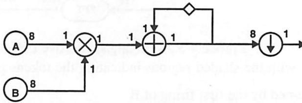
**Figure 4-7** An attempt to use 1D-SDF to repeatedly compute inner products.
