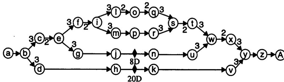
**Figure 3-17** SDF graph for a non-uniform filterbank. The highpass channel retains  $1/3$  of the spectrum and the lowpass channel retains  $2/3$  of the spectrum.
