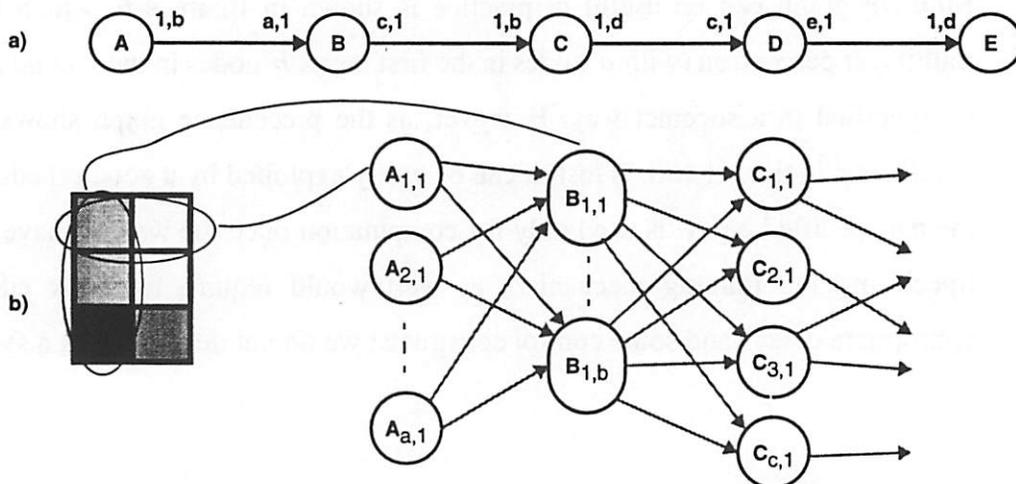
**Figure 4-6** a) Multilayer perceptron expressed as an MDSDF graph.
