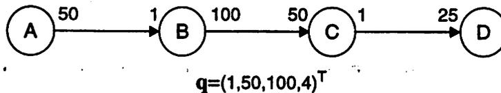
**Figure 3-2** Example to illustrate the inefficiency of using shared buffers. graphs; the general case is more complicated). Consider the graph in Figure 3-2. The shared-buffer cost for the schedule  $S = (A)(50B)(100C)(4D)$  for this graph is given by
