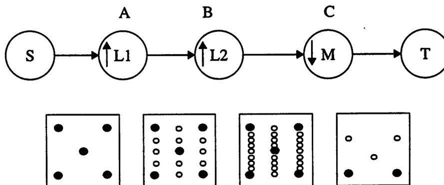
**Figure 5-18** System for doing multistage sampling structure conversion from 4/3 aspect ratio to 16/9 aspect ratio for a 2:1 interlaced TV signal.
