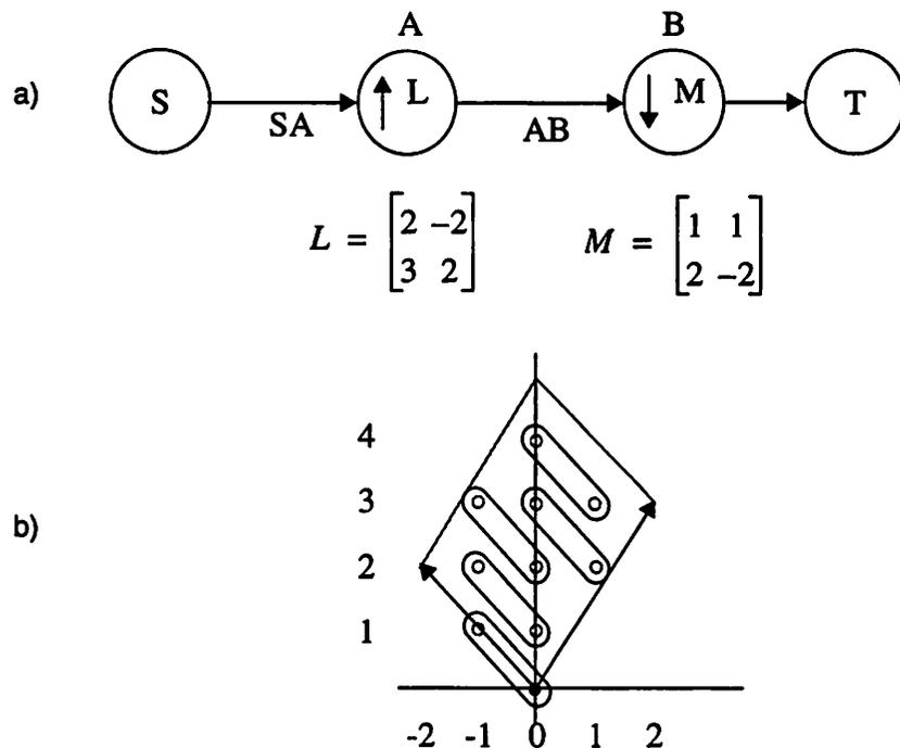
**Figure 5-9** An example to illustrate balance equations and the need for some additional constraints. a) The system. b) Ordering of data into a  $5 \times 2$  rectangle inside  $FPD(L)$ .
