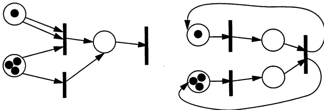
**Figure 1-2** a) A Petri net. Places are the circles, and transitions are the heavy lines. The dots in the places indicate tokens. b) A Petri net equivalent to a dataflow graph.
