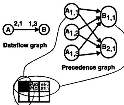
**Figure 4-4** Data exchange in an MD-SDF graph.
