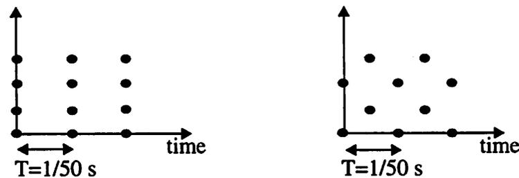
**Figure 5-16** Progressive scanning and 2:1 interlaced scanning in the vertico-temporal plane
