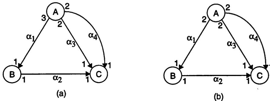
**Figure 2-2** (a) An SDF graph that does not have a periodic schedule.
