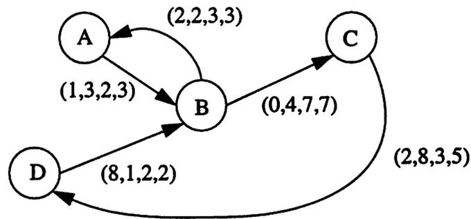
**Figure 1-1** A computation graph. The 4-tuple associated with an edge represents the number of initial tokens, the number of tokens produced onto the arc, the number of tokens consumed from the arc, and the threshold parameter of the arc.
