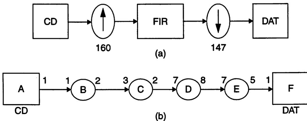
**Figure 3-10** (a). CD to DAT sample rate change system.
