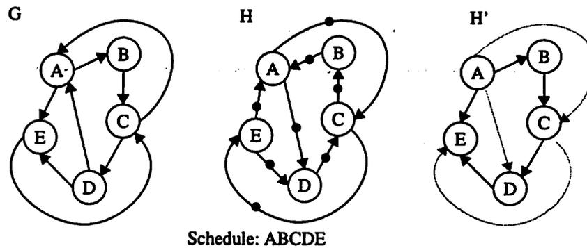
**Figure 2-6** Example to illustrate proof of Theorem 2-3. A filled dot on an edge indicates a delay on that edge. The shaded edges in the  $H'$  graph show the edges that are reversed w.r.t  $G$
