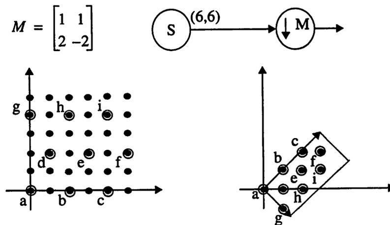
**Figure 5-7** Output samples from the decimator renumbered to illustrate concept of support matrix. The circled samples on the left are labeled as shown.
