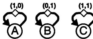
**Figure 4-11** Three macro actors with state represented as a self-loop.
