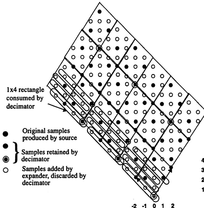
**Figure 5-12** Total amount of data produced by the source in one iteration of the periodic schedule determined by the balance equations in equation 5.11. The samples that are kept by the decimator are the lightly shaded samples.
