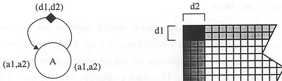
**Figure 4-12** (a) An actor with a self loop. (b) Data space on the edge.
