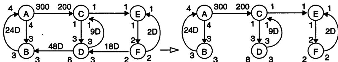
**Figure 3-26** An example to illustrate the inability of the scheduling framework in [Bhat94b] to yield buffer-optimal single appearance schedules when combined with techniques presented in this chapter.
