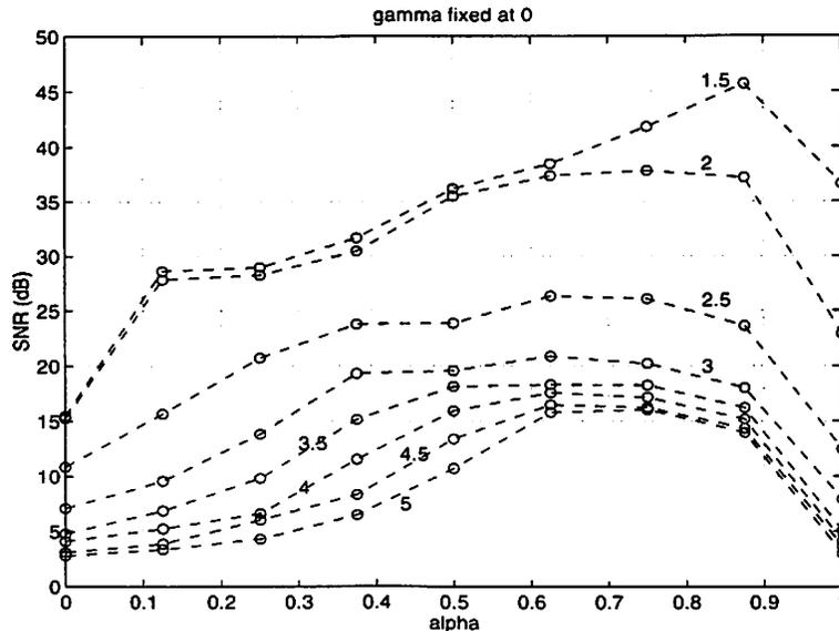
Figure 4.1: Pyramid coder performance as a function of  $\alpha$  for fixed  $\gamma = 0$  (2-layer coding). Automatic  $\sigma$ -scaling uniform quantizers were used in the coder. Values of  $G$  are indicated by the labels on the plot lines.
