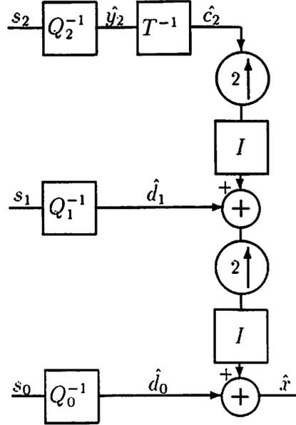
Figure 2.3: Structure of a two-stage pyramid decoder. Subscripts refer to layer numbers. Received signals are  $s_i$ ,  $i = 0, 1, 2$ , and the decoded output signal is  $\hat{x}$ .
