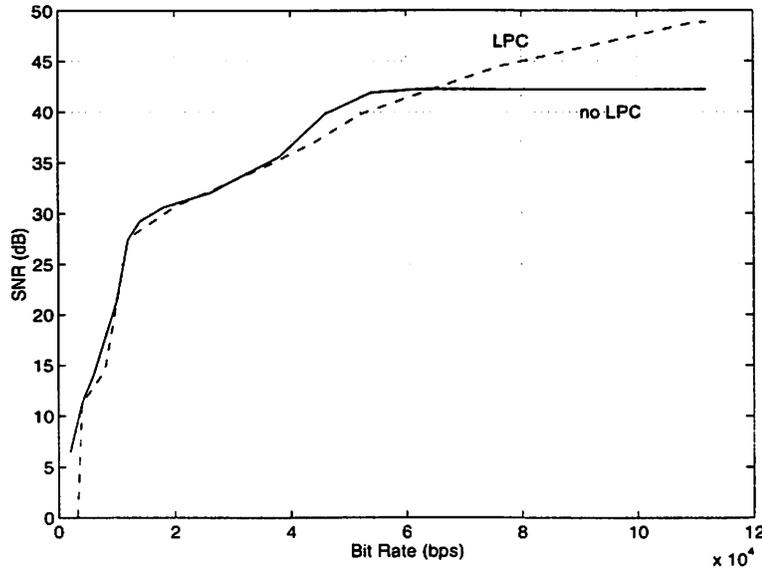
Figure 2.8: Effects of LPC transform coding on pyramid coder performance. Automatic  $\sigma$ -scaling uniform quantizers and a windowed length-19 sinc filter were used to generate the data.
