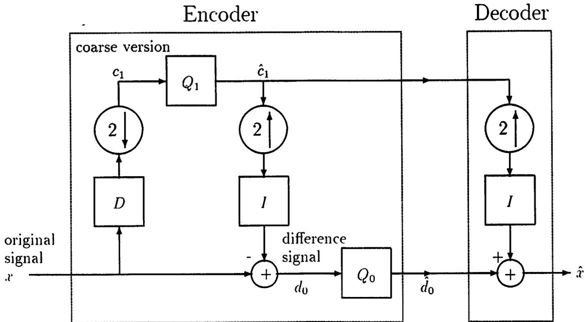
Figure 2.1: Structure of a single-stage pyramid coder. Subscripts refer to layer numbers.
