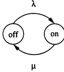
Figure 3.1: Single source on/off model.
