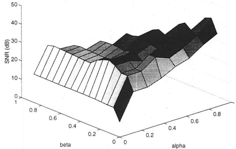
Figure 2.10: Pyramid coder performance under lossless network conditions. Data calculated for  $b = 8$  bits/samples, length-19 windowed sinc filters, automatic  $\sigma$ -scaling uniform quantizers, and no transform coding.
