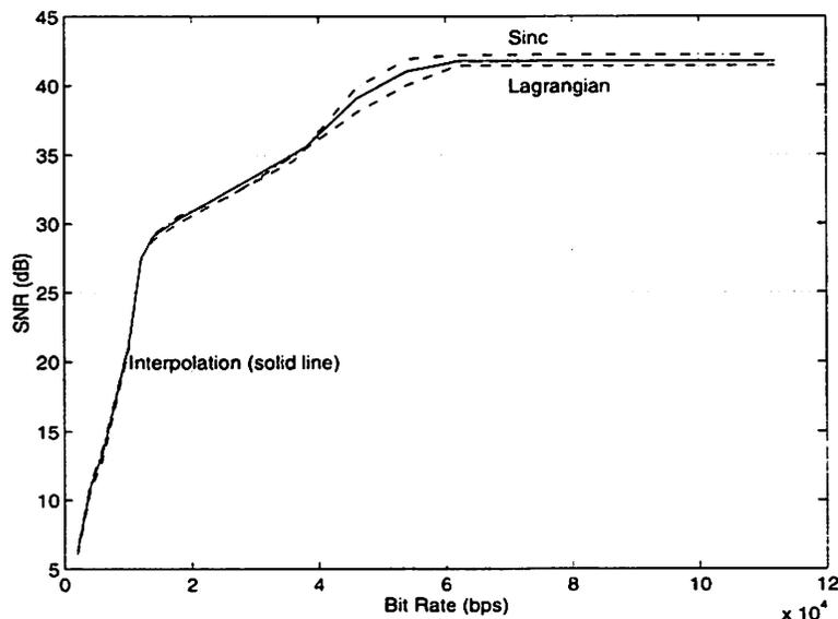
Figure 2.5: Effects of filter choice on pyramid coder performance. Performance of length-19 windowed sinc, Lagrangian, and bandlimited interpolation filters is shown.
