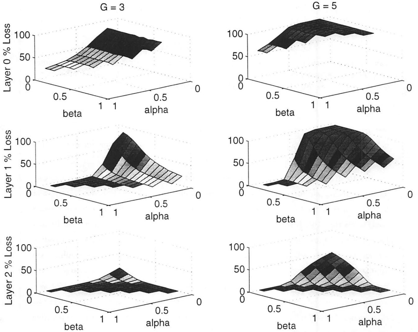
Figure 3.4: Average percent packet loss rates for two values of  $G$  when a priority drop-tail queue is used. Loss rates are shown for Layers 0, 1, and 2 as a function of  $\alpha$  and  $\beta$ , for  $G = 3$  (left column) and  $G = 5$  (right column).
