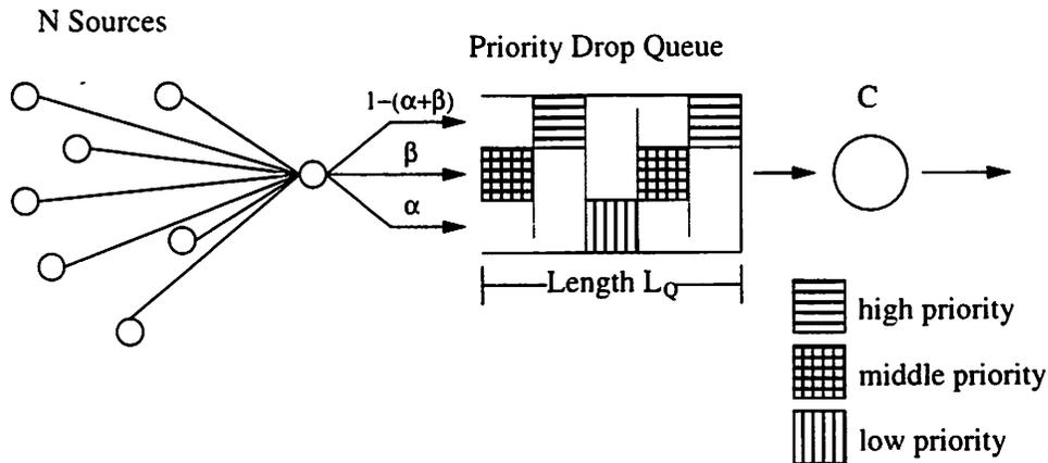
Figure 3.3: Network model illustrating a priority-drop queue and sources producing three layers of data.
