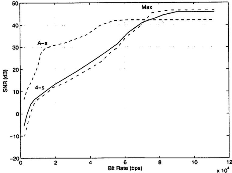
Figure 2.4: Effects of quantizer choice on pyramid coder performance. Labels refer to choice of overload regions for uniform quantizers.
