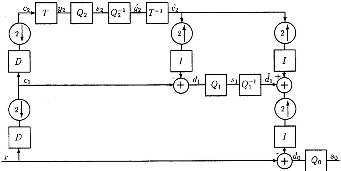
Figure 2.2: Structure of a two-stage pyramid encoder. Subscripts refer to layer numbers. The input signal is  $x$ , and transmitted encoded signals are  $s_i$ ,  $i = 0, 1, 2$ .
