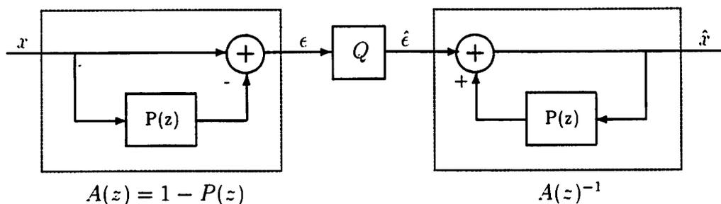
Figure 2.7: The coefficients of  $P(z)$  are computed using LPC analysis of the input data.
