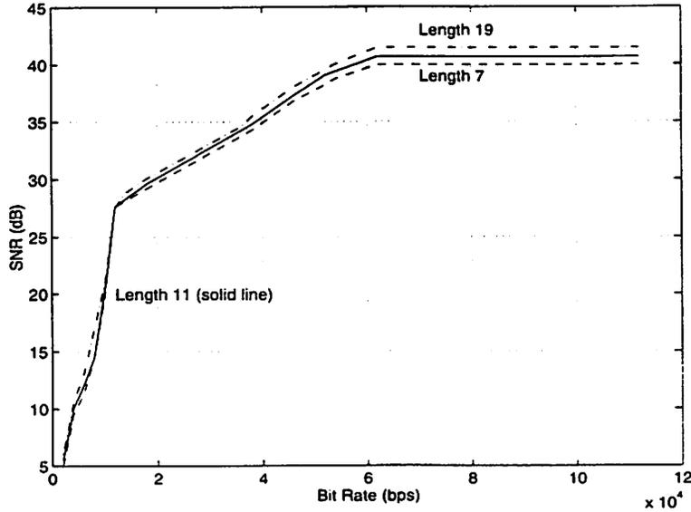
Figure 2.6: Effects of filter length choice on pyramid coder performance. Performance of length-7, 11, and 19 Lagrangian interpolation filters is shown.
