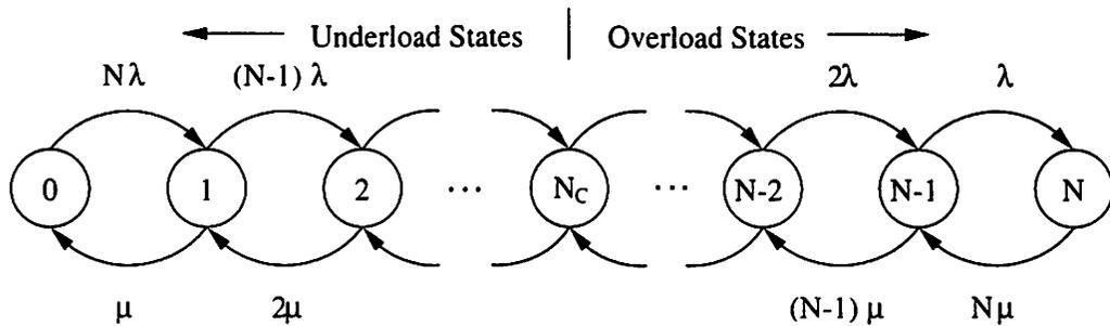
Figure 3.2: Markov chain for  $N$ -source model. States are the number of active sources,  $n(t)$ .
