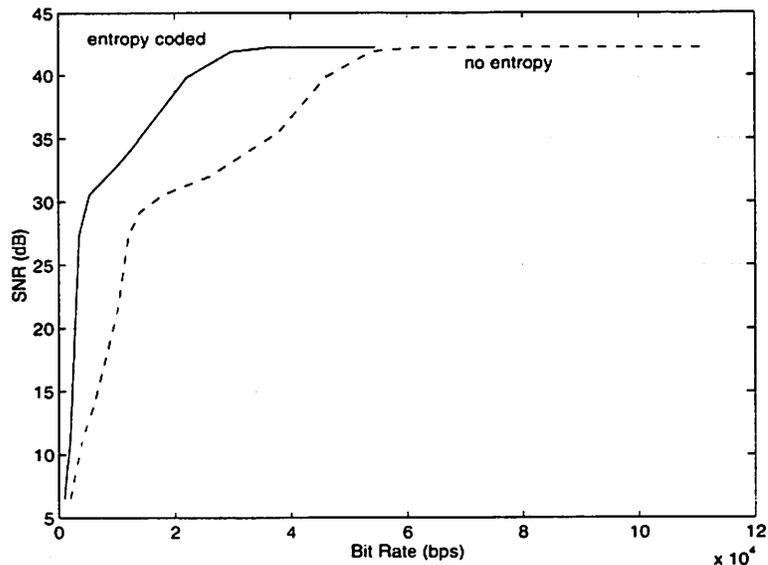
Figure 2.9: Effects of entropy coding on pyramid coder performance. Automatic  $\sigma$ -scaling uniform quantizers and a windowed length-19 sinc filter were used to generate the data.
