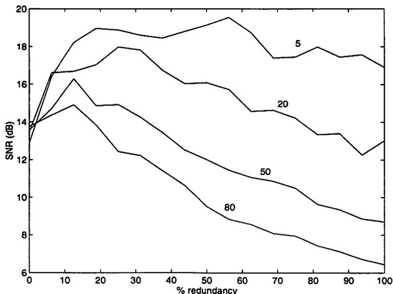
Figure 4.2: Effects of data redundancy as the amount of redundancy used and percentage of total traffic using redundancy varies. The x-axis measures how much redundancy is being added to the base data. The number on each plot line indicates what percentage of users are adding this level of redundancy to their data.
