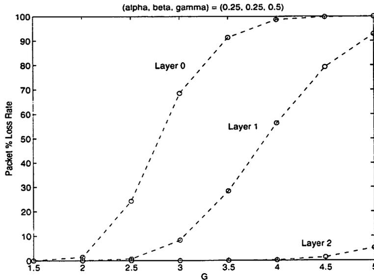
Figure 3.5: Packet percent loss rates across layers as a function of  $G$ . Bit-rate allocations  $(\alpha, \beta, \gamma)$  were fixed at  $(0.25, 0.25, 0.5)$ .
