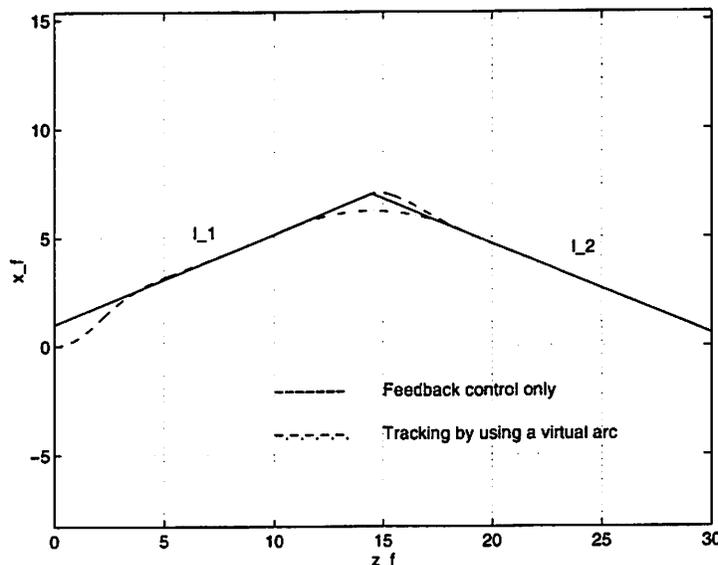
Figure 10: Comparison between two schemes for tracking a piecewise straight-line curve: 1. Using only the feedback tracking control law; 2. Using a pre-designed approximating virtual curve (an arc in this case) around the intersection point.
