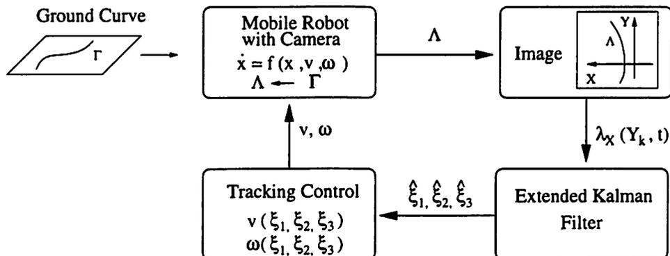
Figure 13: The closed-loop vision-guided navigation system for a ground-based mobile robot.
