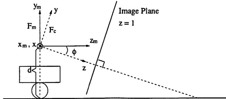
Figure 2: The side-view of the unicycle mobile robot with a camera facing downward with a tilt angle  $\phi > 0$ .
