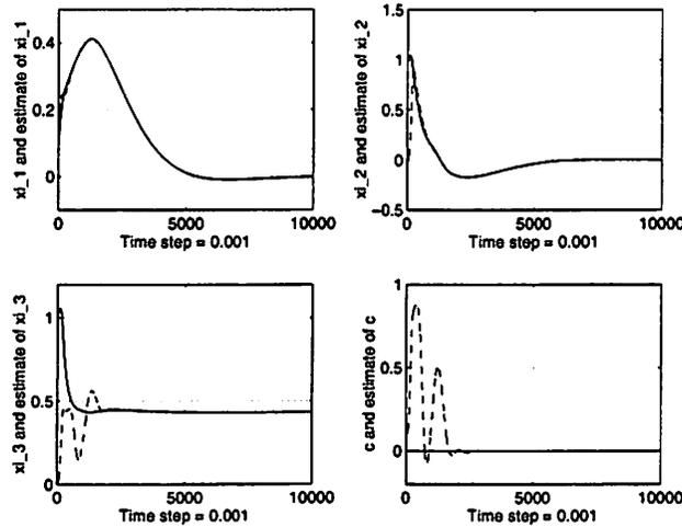
Figure 12: The simulation results of using the Extended Kalman Filter to estimate the image quantities  $\xi^3$  and  $\eta (= c = k'(s))$  with the number of output measurements  $N = 1$ : Solid curves are for true states; dashed curves are for estimates.
