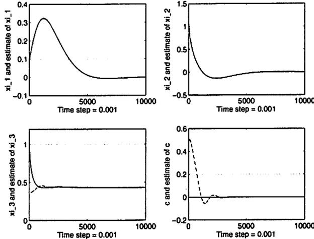
Figure 11: The simulation results of using the Extended Kalman Filter to estimate the image quantities  $\xi^3$  and  $\eta (= c = k'(s))$  with the number of output measurements  $N = 5$ : Solid curves are for true states; dashed curves are for estimates.
