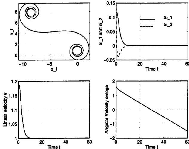
Figure 9: Simulation results for tracking a linear curvature curve ( $c = k'(s) = -0.05$ ). Subplot 1: the trajectory of the mobile robot in the reference coordinate frame; subplot 2: the image curve parameters  $\xi_1$  and  $\xi_2$ ; subplot 3 and 4: the control inputs  $v$  and  $\omega$ .
