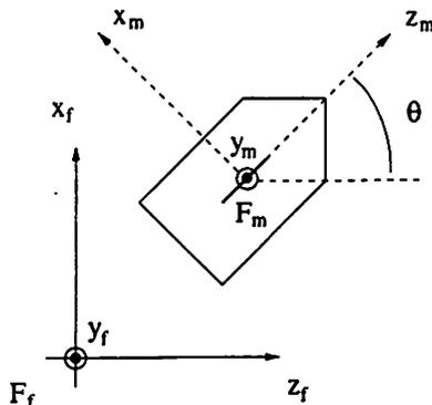
Figure 1: Model of the unicycle mobile robot.
