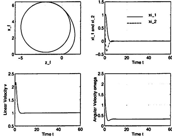
Figure 8: Simulation results for tracking a circle. Subplot 1: the trajectory of the mobile robot in the reference coordinate frame; subplot 2: the image curve parameters  $\xi_1$  and  $\xi_2$ ; subplot 3 and 4: the control inputs  $v$  and  $\omega$ .
