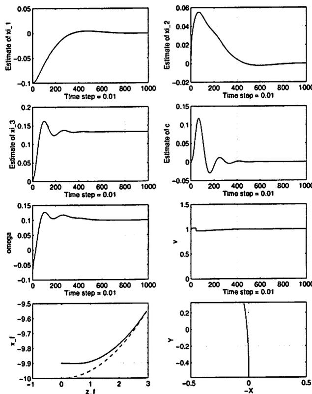
Figure 14: Simulation results for the closed-loop vision-guided navigation system for the case when the ground curve is a circle: In subplot 7, the solid curve is the actual mobile robot trajectory (in the space frame  $F_f$ ) and the dashed one is the nominal circle; subplot 8 is the image of the circle viewed from the camera at the last simulation step, when the mobile robot is perfectly aligned with the circle.
