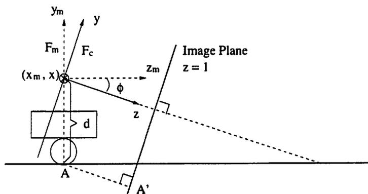
Figure 5: The orthographic projection image of the point  $A$  where the wheel touches the ground.
