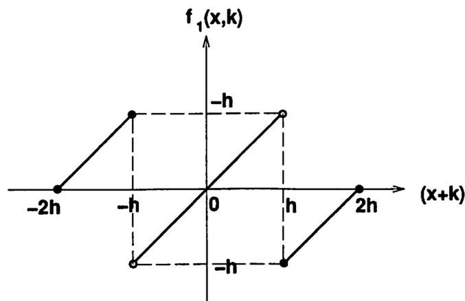
Figure 3 Nonlinear function used in continuous shift cipher.
