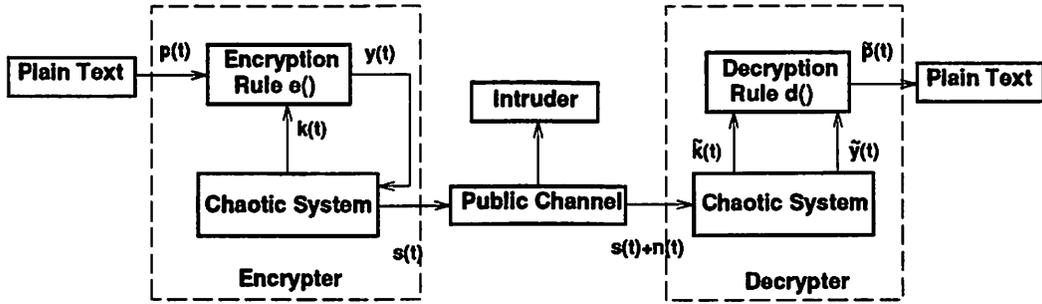
Figure 1: Block diagram of the chaotic cryptosystem.
