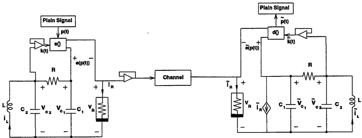
Figure 2 Block diagram of the Chua's circuits based cryptosystem.
