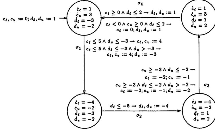
Figure 6: The initialized singular automaton  $B_A^c$
