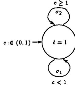
Figure 10: The initialized rectangular automaton  $\bar{A}$  for which  $\text{Lang}^c(\bar{A})$  not limit-closed
