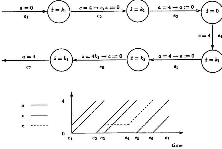
Figure 20: Doubling  $c$  using the two-slope variable  $z$  with the slopes 0 and  $k_1$
