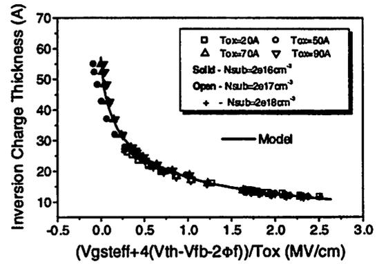
Figure 4. For all  $Tox$  and  $Nsub$ , modeled inversion charge thickness agrees with numerical quantum simulations.
