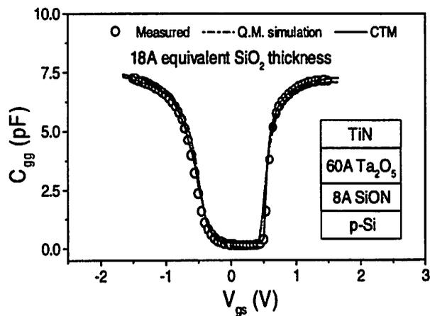
Figure 11. Universality of CTM is demonstrated by modeling the  $C_{gg}$  of NMOSFET with SiON/Ta<sub>2</sub>O<sub>5</sub>/TiN gate stack.
