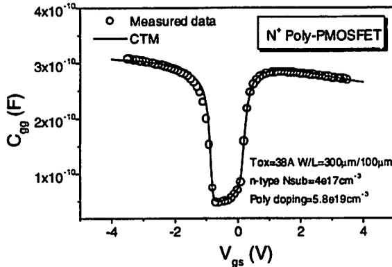
Figure 8. Measured and CTM modeled  $C_{gg}$  of  $N^+$ -poly (buried-channel) PMOSFET. Gate depletion occurring in the accumulation region is correctly modeled.
