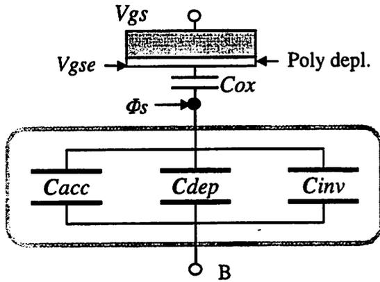
Figure 2. Charge-thickness capacitance concept in this model.  $Vgse$  accounts for poly-depletion.
