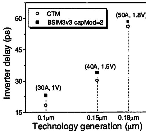
Figure 12. Simulated unloaded CMOS inverter delay is shorter with CTM than BSIM3v3 capMod=2.  $W_n/W_p=10\mu\text{m}/15\mu\text{m}$ .
