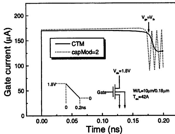
Figure 13. Comparison of gate currents in turn-on and turn-off transients between CTM and BSIM3v3.1 capmod=2 for an NMOSFET with  $W/L=10\mu\text{m}/0.18\mu\text{m}$  and  $T_{ox}=42\text{\AA}$ . The absence of the gate current oscillation in CTM helps convergence.
