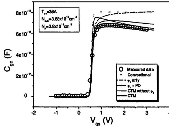
Figure 10. Measured and modeled gate-to-channel capacitance  $C_{gc}$  of an NMOSFET with different physical effects considered in simulation.  $T_{ox} = 36\text{A}$ ,  $W/L = 100\mu\text{m}/100\mu\text{m}$ ,  $N_p = 3.8 \times 10^{19} \text{cm}^{-3}$  and  $N_{sub} = 3.68 \times 10^{17} \text{cm}^{-3}$ . PD stands for Polysilicon Depletion.
