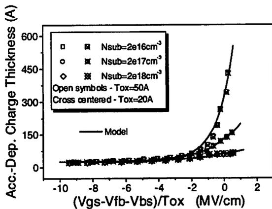
Figure 3. For all  $Tox$  and  $Nsub$ , modeled charge thickness agrees with numerical quantum simulations throughout accumulation and depletion regions.
