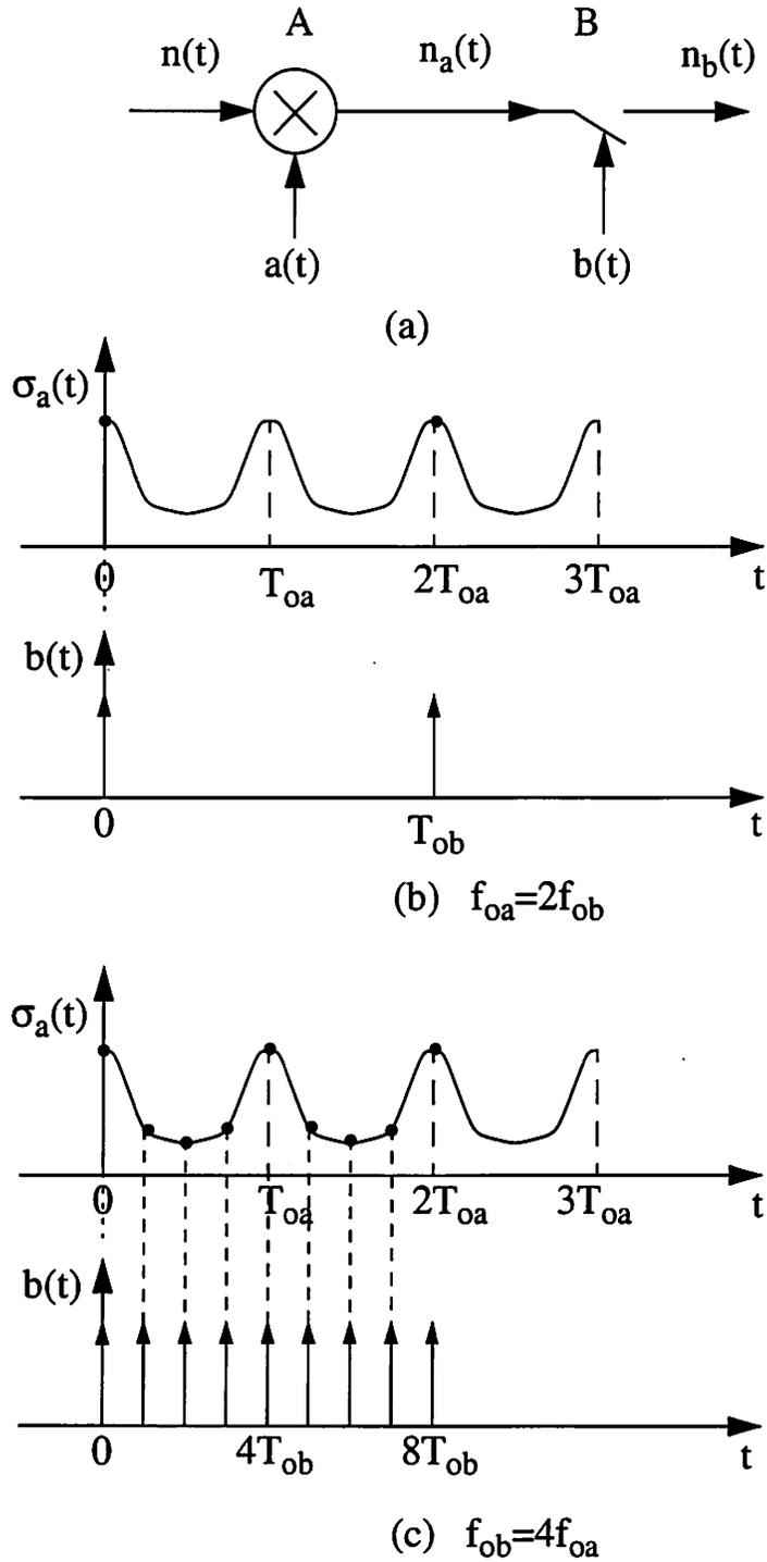
Fig. 2. Sampling cyclostationary noise.
