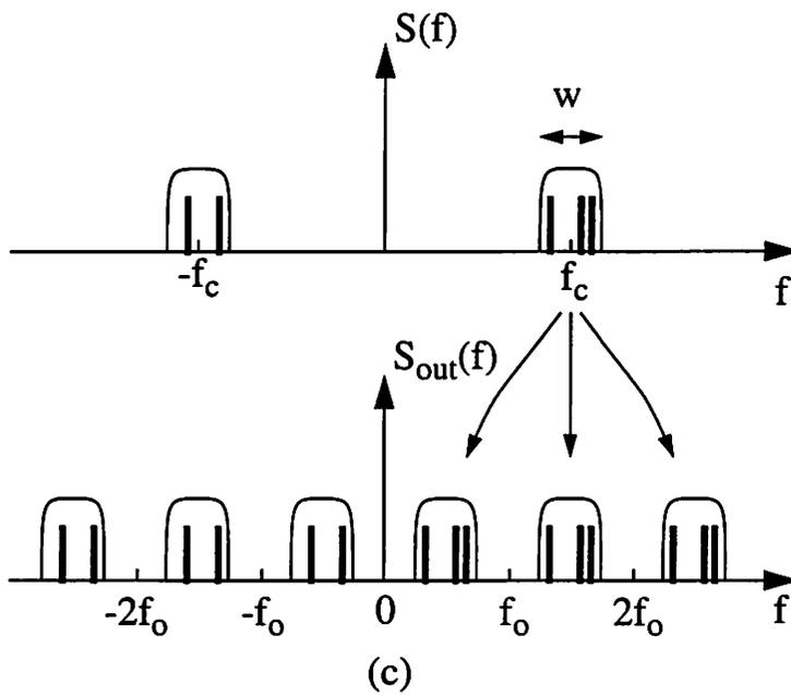
Fig. 4. Mixing band-limited cyclostationary noise
