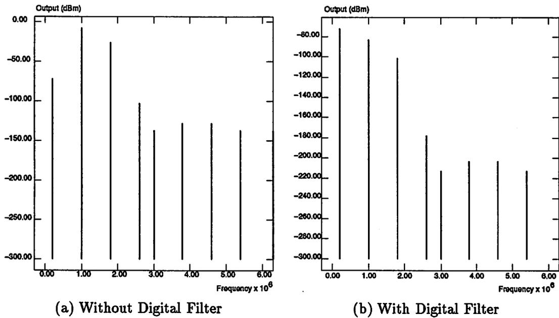
Figure 4.19: Simulator Output for Wideband IF Receiver - 2 tones
