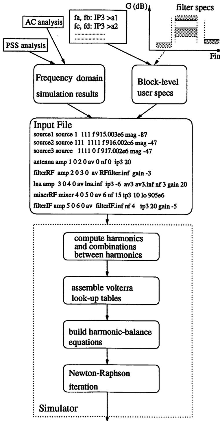
Figure 4.12: Behavioral Simulator Flow Diagram
