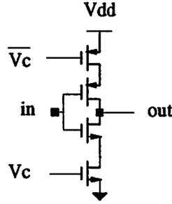
Figure 3.15: Current-Starved Ring Oscillator VCO Cell
