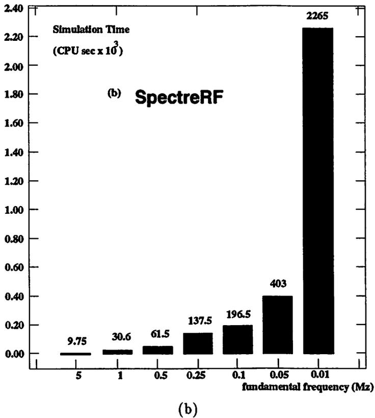
Figure 4.15: (a) VHSIM Simulation Speed (b) SPECTRERF Simulation Speed
