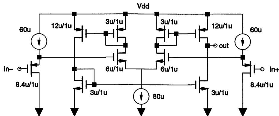
Figure 3.19: Level Restoring Circuit
