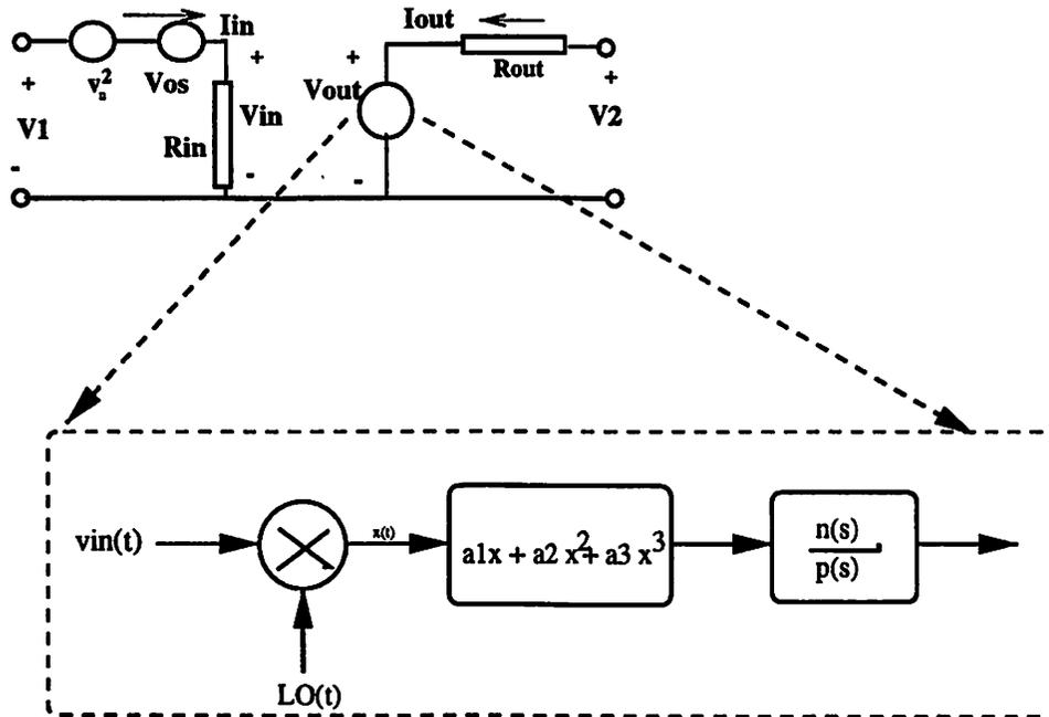
Figure 4.2: Mixer Behavioral Model in SPECTREHDL
