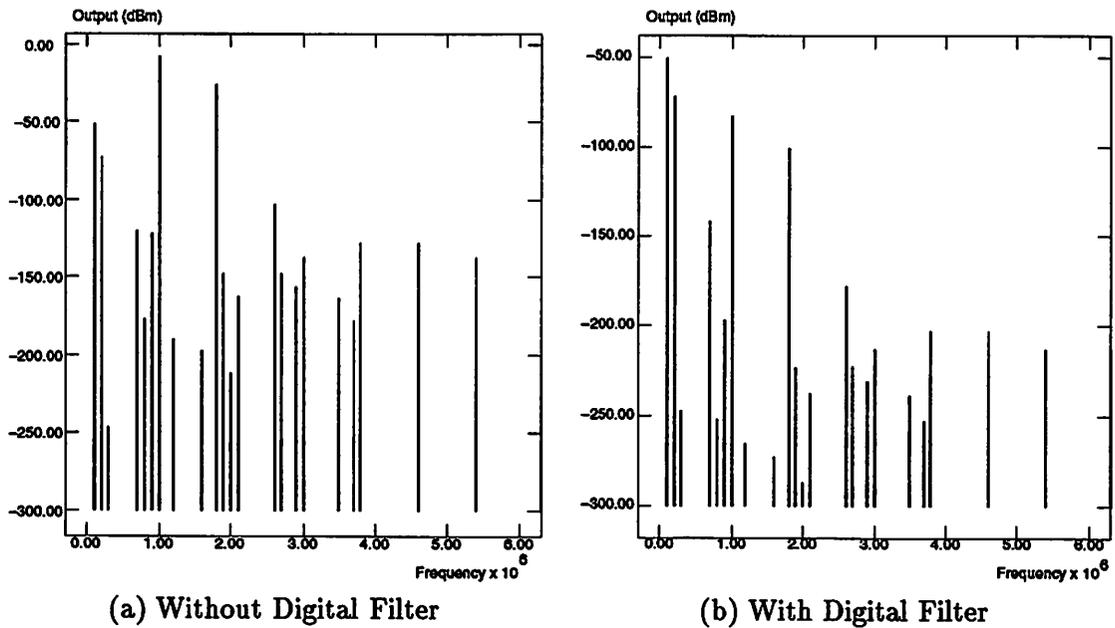
Figure 4.20: Simulator Output for Wideband IF Receiver - 3 tones
