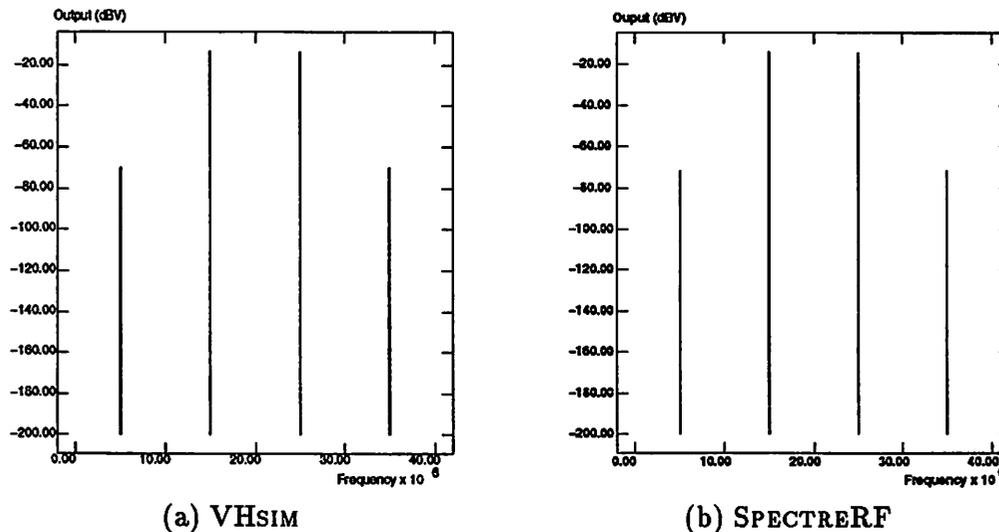
Figure 4.21: Cascade of Mixers  $IM_3$  Simulation
