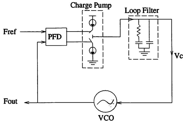
Figure 3.6: Charge Pump PLL
