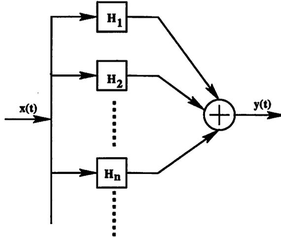
Figure 4.3: System Represented by Volterra Kernels
