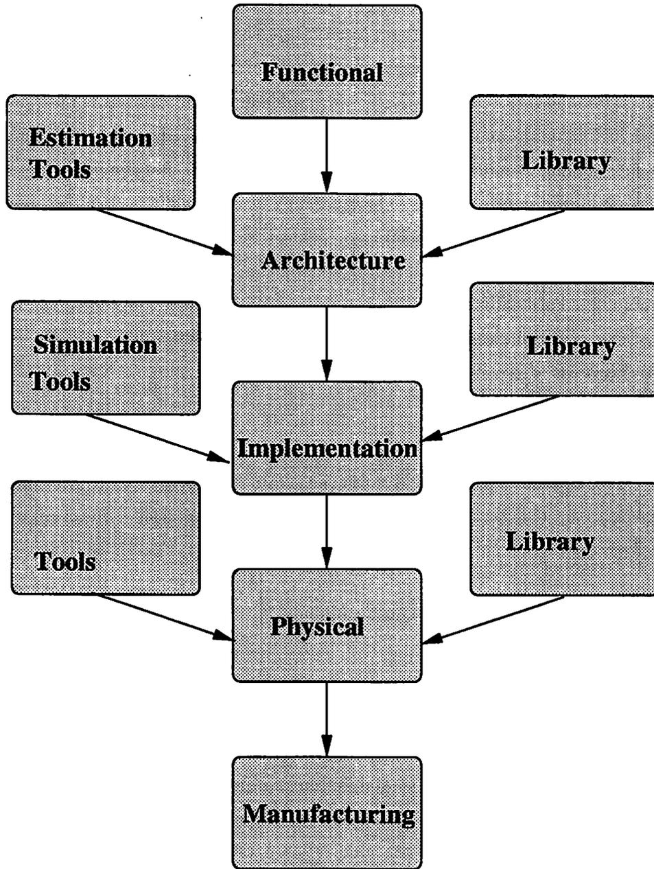
Figure 5.2: Typical Design Flow
