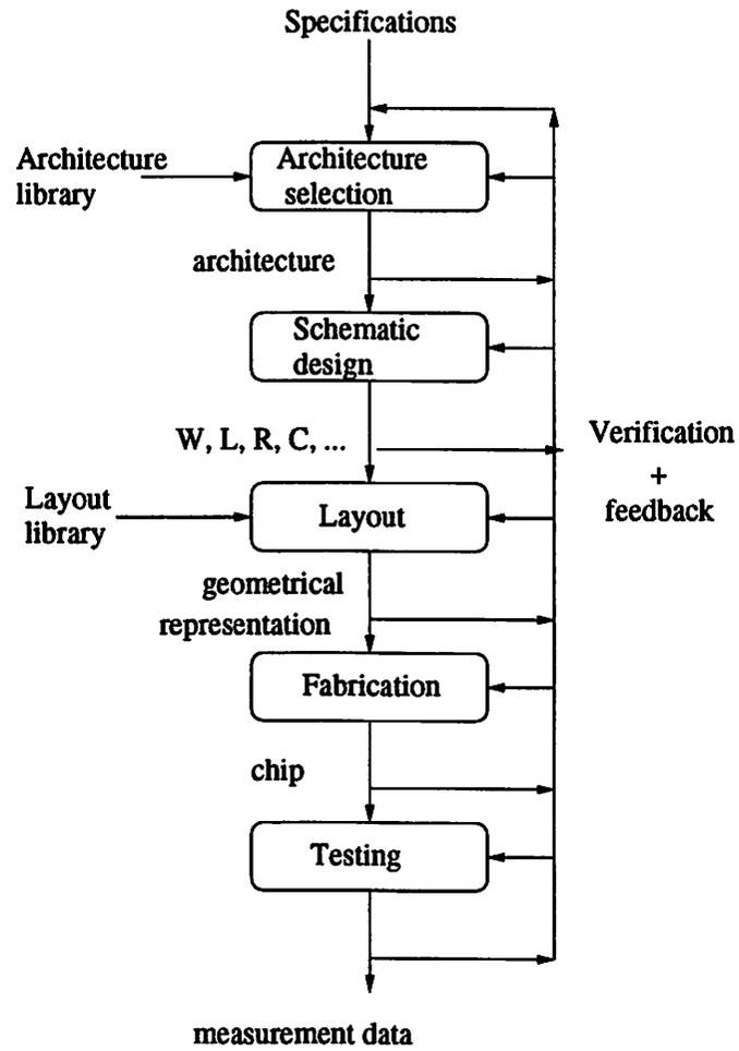
Figure 2.1: Typical IC Design Flow
