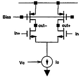
Figure 3.16: Differential Delay Cell
