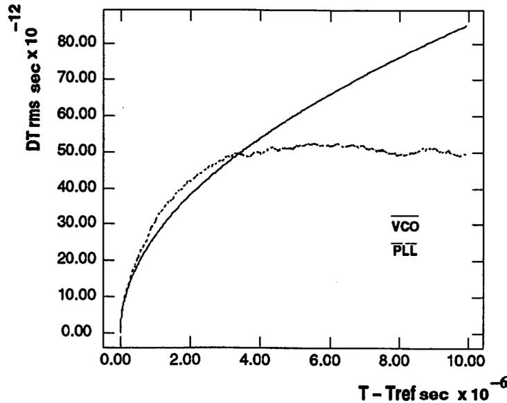
Figure 3.32: PLL Jitter Verification (a)  $\Delta T_{rms}$
