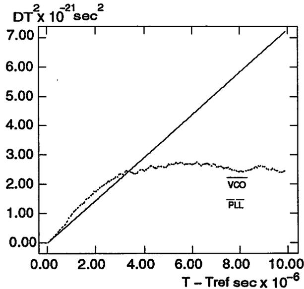
Figure 3.33: PLL Jitter Verification (b)  $\Delta T^2$
