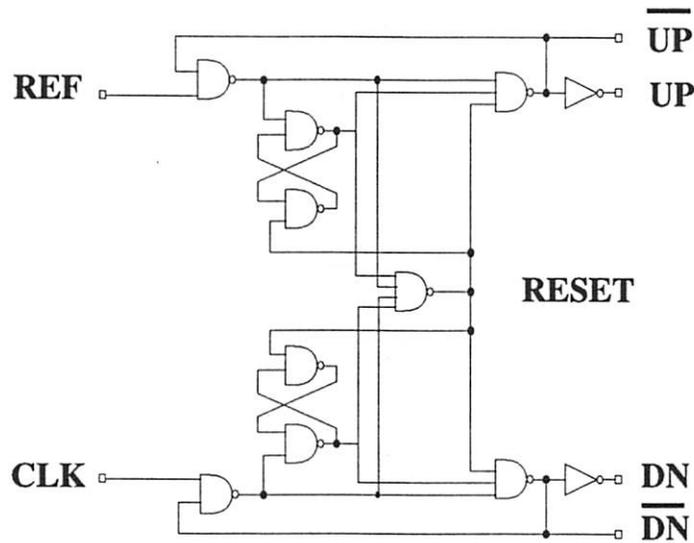
Figure 3.20: Phase-Frequency Detector
