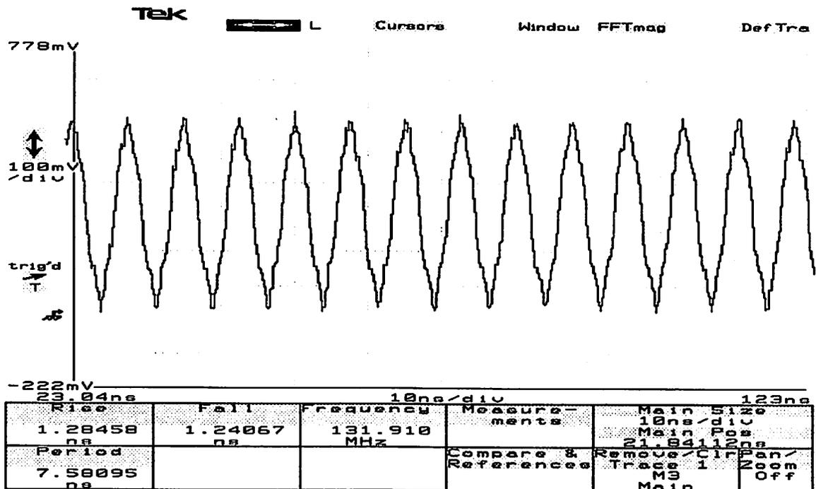
Figure 3.39: Frequency Synthesizer Output
