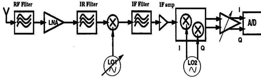
Figure 5.7: Super-Heterodyne Architecture
