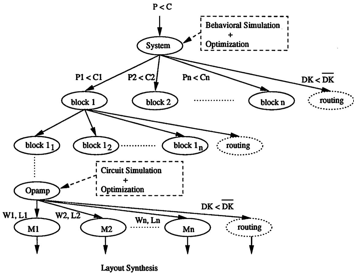
Figure 2.2: Top-Down Design Methodology Flow
