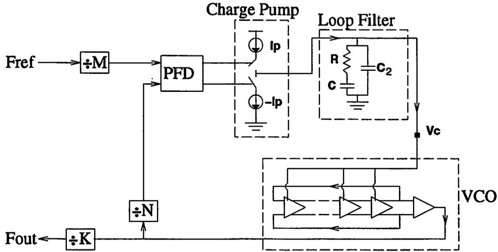
Figure 3.4: PLL Programmable Frequency Synthesizer
