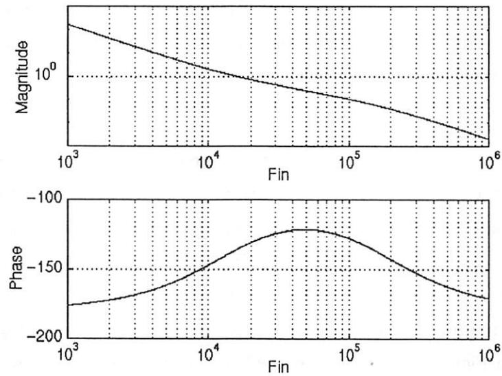
Figure 3.14: PLL Open Loop Characteristic
