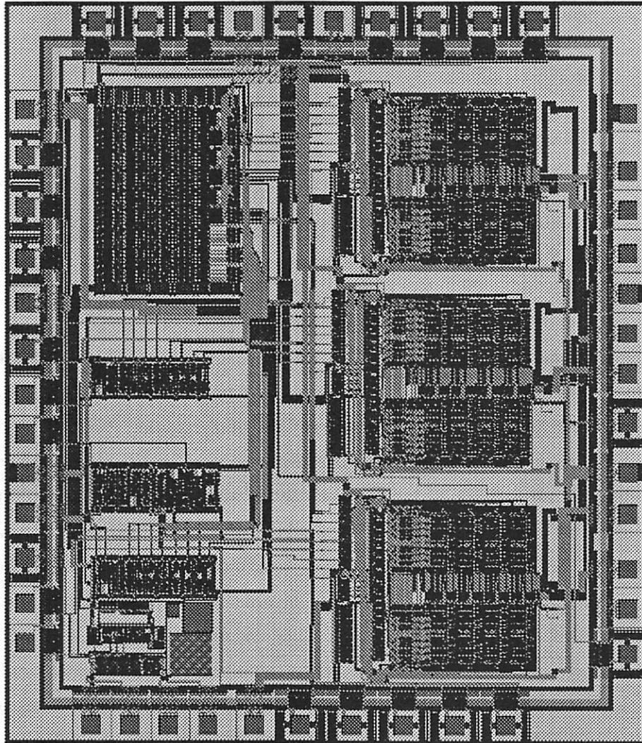
Figure 3.30: Video Driver System Layout
