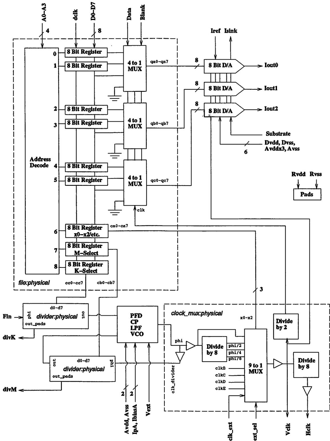
Figure 3.2: Display Driver System Detailed Functional Diagram
