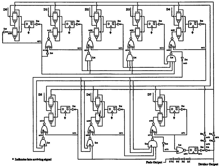
Figure 3.24: Programmable Divider
