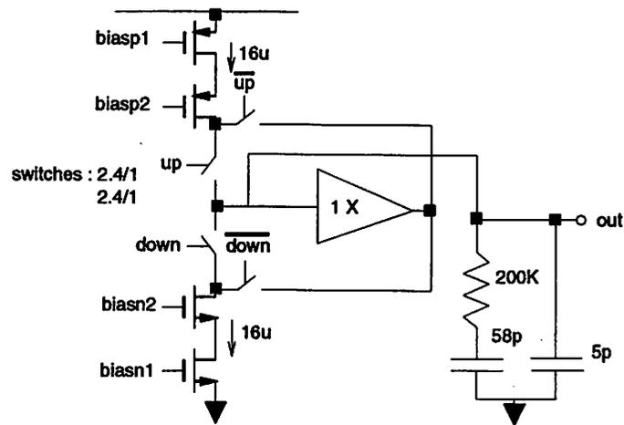
Figure 3.22: Charge-Pump Circuit
