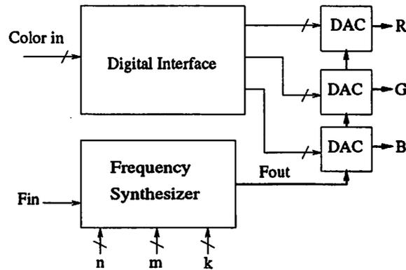
Figure 3.1: Display Driver System Diagram
