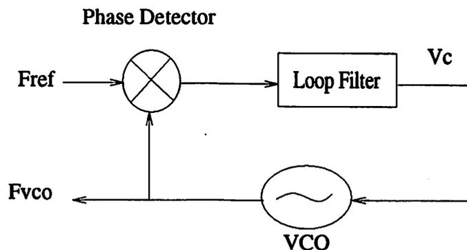
Figure 3.5: PLL Simplified Diagram
