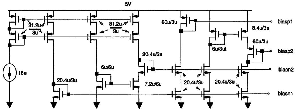
Figure 3.23: Charge-Pump Bias Circuit
