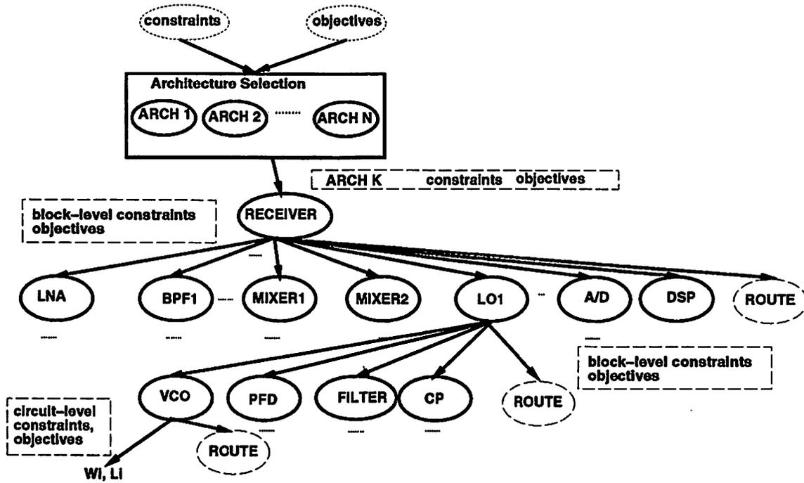
Figure 4.1: RF Receiver Hierarchical Design Decomposition
