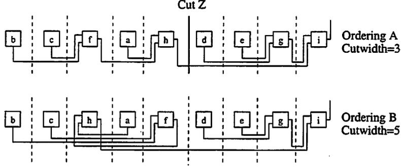
Figure 8: Example cut-widths for the circuit of Figure 6(a)
