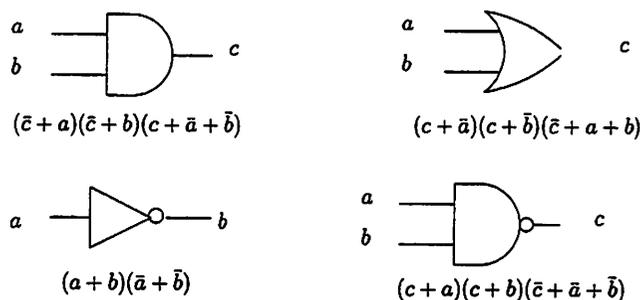
Figure 2: SAT formulas for simple gates
