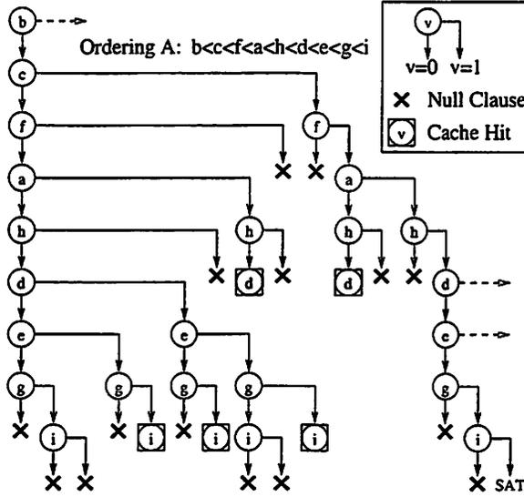
Figure 7: Caching-based backtracking for Formula 4.1
