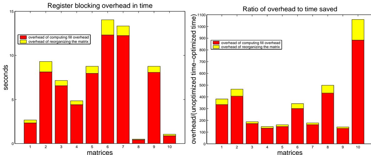
Figure 3.17: **Pre-computation overhead of register-blocked multiplication on 10 sparse matrices taken on a 167 MHz UltraSPARC:** The left figure shows the time used to perform each of the two steps, determining the block size and reorganizing the matrix. The right figure shows the same values divided by the savings of blocked vs. unblocked code; this tells us the number of times a matrix-vector multiplication would have to be performed to amortize the overhead.
