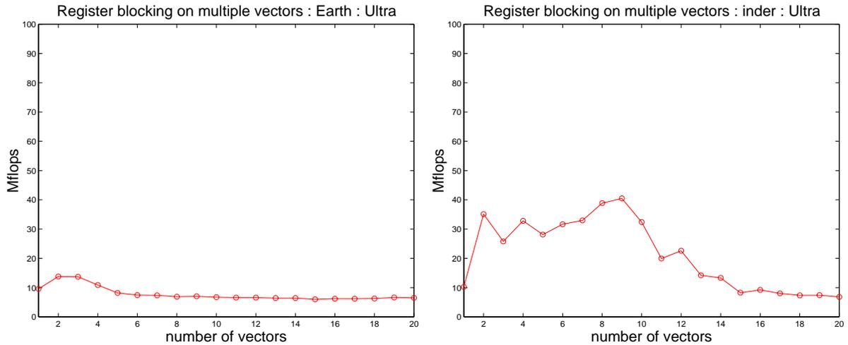
Figure 5.18: Performance of the multiple-vector optimization on an Earth Science (left) and text retrieval (right) matrix on a UltraSPARC I.
