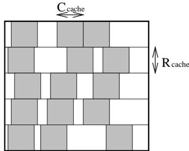
Figure 4.1: **Cache-blocks in a sparse matrix:** The gray areas are sparse matrix blocks that contain nonzero elements in the  $r_{cache} \times c_{cache}$  rectangle. The white areas contain no nonzero elements, and are not stored.
