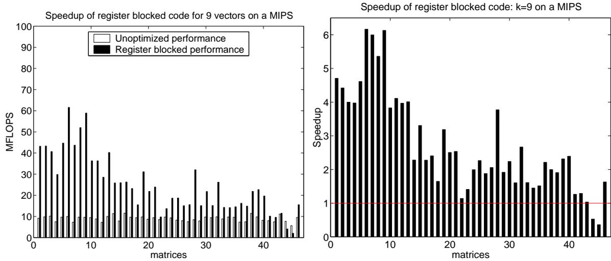
Figure 5.9: **Performance of register-blocked, multiple vector code on a MIPS R10000:** The left-hand plot shows the performance in Mflops of the unoptimized code and the multiple vector version using 9 vectors. The right-hand plot shows the speedup of multiple vectors relative to unoptimized code.
