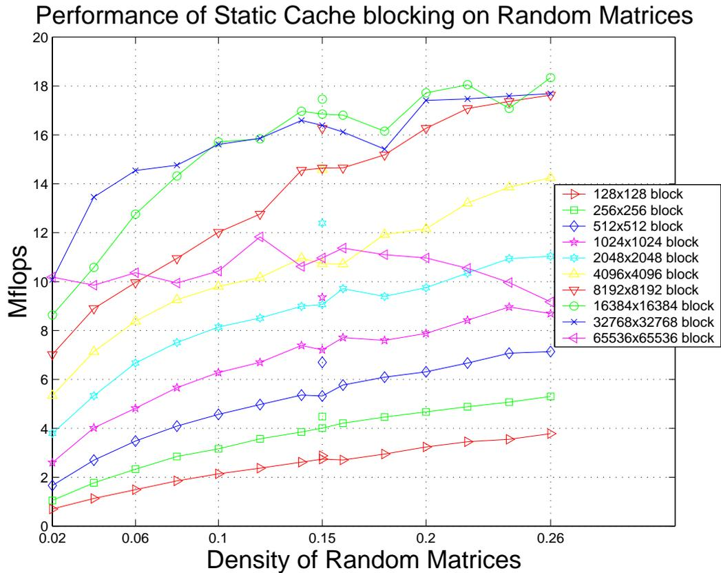
Figure 4.12: **Performance of cache-blocked multiplication on random matrices:** It is measured for  $64K \times 64K$  random matrices with varying densities 0.02–0.26% on an UltraSPARC I. Each line represents different cache block sizes, and the separate points at 0.15% show the performance of the LSI matrix, measured in Mflops.
