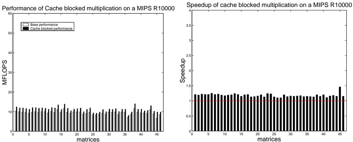
Figure 4.9: Performance of cache blocked multiplication on a MIPS R10000.
