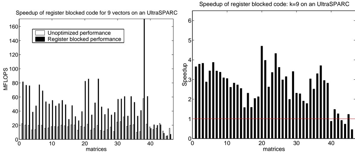
Figure 5.8: **Performance of register-blocked, multiple vector code on an UltraSPARC I:** The left-hand plot shows the performance in Mflops of the unoptimized code and the multiple vector version using 9 vectors. The right-hand plot shows the speedup of multiple vectors relative to unoptimized code.
