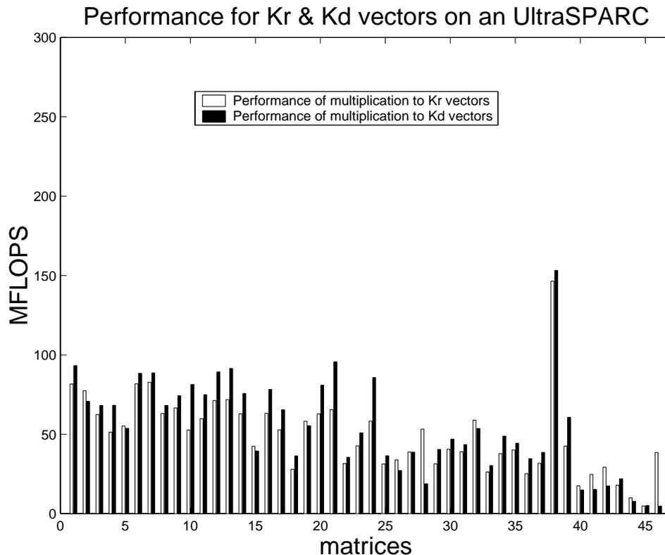
Figure 5.11: **Comparing the dense ( $k_d$ ) and random sparse ( $k_r$ ) matrices to choose the number of vectors on an UltraSPARC 1:** The left bar represents the performance when it is multiplied to the peak value for a dense matrix ( $k_d$ ) and the right bar represents the performance when it is multiplied to the peak value for a random matrix ( $k_r$ ).
