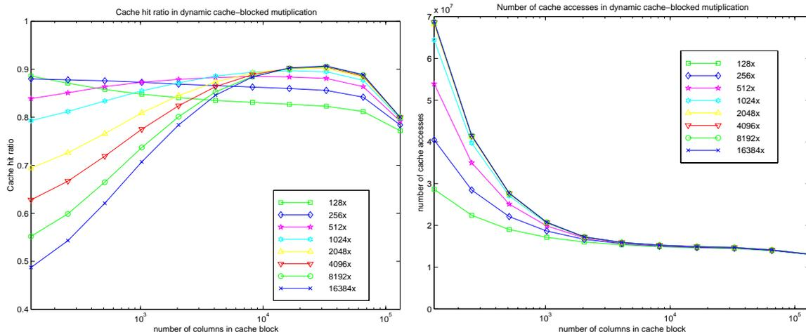
Figure 4.7: **Cache behavior of dynamic cache-blocking on the LSI matrix:** The left figure shows the L2 cache hit ratio and the right figure shows the total number of cache accesses.
