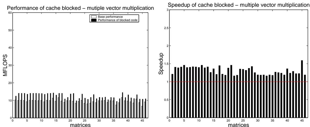
Figure 5.15: **Performance of cache-blocked, multiple-vector multiplication on a MIPS R10000:** The left-hand plot shows the absolute performance of the unoptimized and cache-blocked multiple vector code, and the right-hand plot shows the corresponding speedup.
