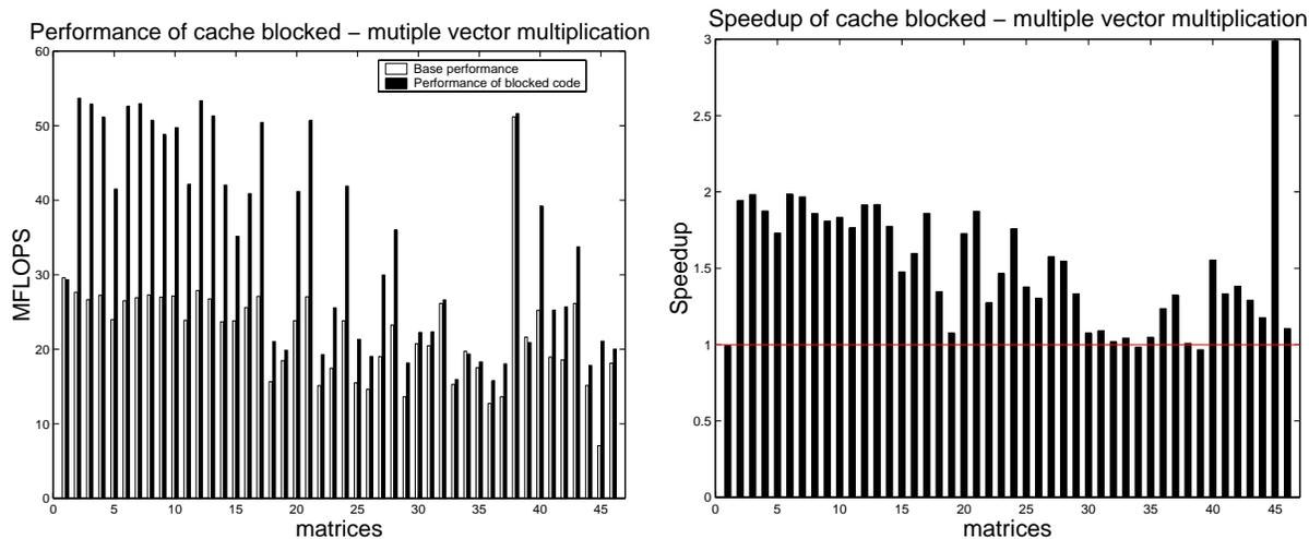
Figure 5.14: **Performance of cache-blocked, multiple-vector multiplication on an Ultra SPARC I:** The left-hand plot shows the absolute performance of the unoptimized and cache-blocked multiple vector code, and the right-hand plot shows the corresponding speedup.
