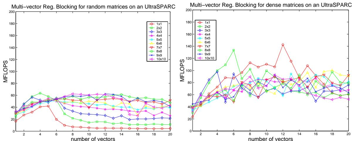
Figure 5.5: **Register-blocked, multiple vector performance on an UltraSPARC I, varying the number of vectors:** The graph on the left uses a random  $10K \times 10K$  matrix with  $200K$  nonzeros, and the graph on the right uses a  $1K \times 1K$  dense matrix in sparse format. Each line indicates a different register blocking. The x-axis shows the number of vectors and the y-axis shows the performance in Mflops.
