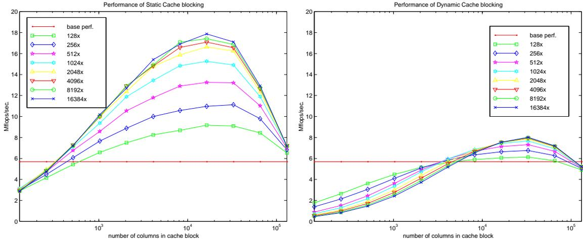
Figure 4.5: **Performance of static and dynamic cache-blocking on the LSI matrix:** This is measured on 167MHz Ultra SPARC I. Each line is for different number of rows in a cache block,  $r_{cache}$  and the horizontal axis is the number of columns in a cache block,  $c_{cache}$ . The horizontal axis is a log scale.
