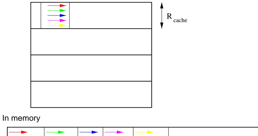
Figure 4.4: **Memory accesses in dynamic cache blocking:** The pointers into the rows in one cache block keep track of the cache block boundaries. Rows in the same cache block are not contiguous in memory.
