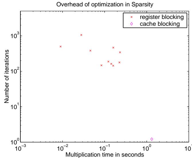
Figure 8.3: **Summary of overhead in Sparsity:** The horizontal axis shows the un-optimized multiplication time in log scale and the vertical axis shows the overhead time divided by the difference between unoptimized multiplication time and optimized multiplication time in log scale. The amount is equivalent to the number of iterations that the optimization pays off. A graph is shown for the subset of benchmark matrices.
