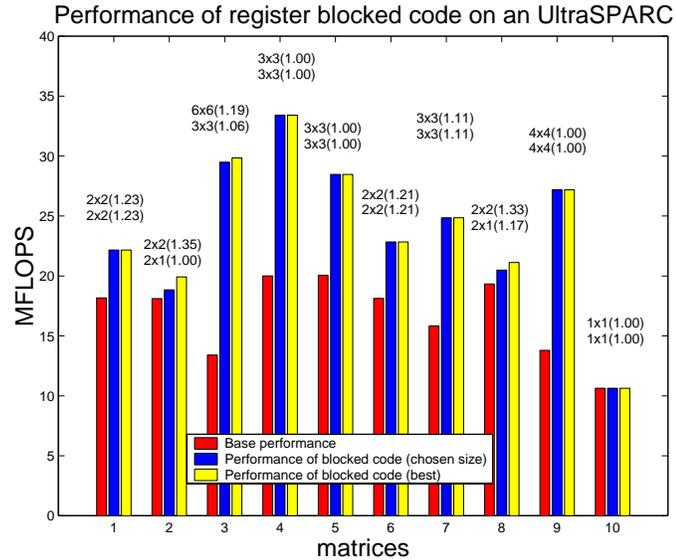
Figure 3.7: **Validation of performance model:** Comparison of the performance of the block size chosen by the performance model (in the middle bar) with the block size chosen by an exhaustive search (in the right bar). on an UltraSPARC I. The left bars indicate unoptimized performance. The upper row of numbers above the bars are the block sizes chosen by the model and the lower row of numbers above the bars are the block sizes chosen by exhaustive search.
