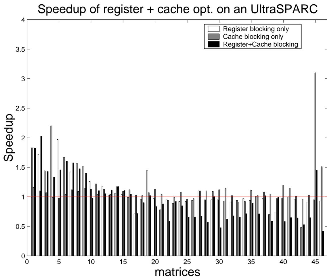
Figure 4.15: Speedup of register and cache blocked multiplication on an UltraSPARC I
