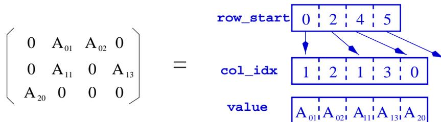
Figure 2.2: Compressed Sparse Row (CSR) representation of a sparse matrix.
