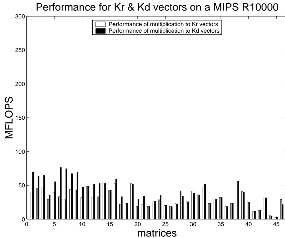
Figure 5.12: **Comparing the dense ( $k_d$ ) and random sparse ( $k_r$ ) matrices to choose the number of vectors on a MIPS R10000:** The left bar represents the performance when it is multiplied to the peak value for a dense matrix ( $k_d$ ) and the right bar represents the performance when it is multiplied to the peak value for a random matrix ( $k_r$ ).
