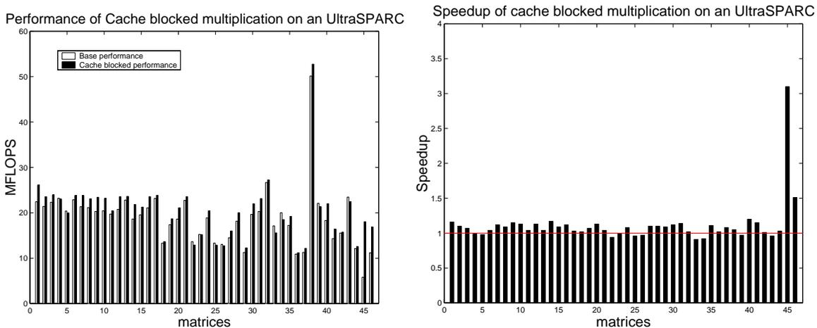
Figure 4.8: Performance of cache blocked multiplication on an Ultra SPARC I.
