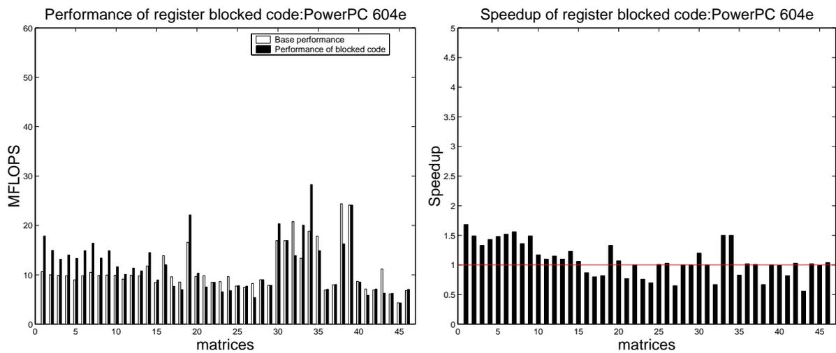
Figure 3.12: Performance of register-blocked multiplication on a PowerPC 604e
