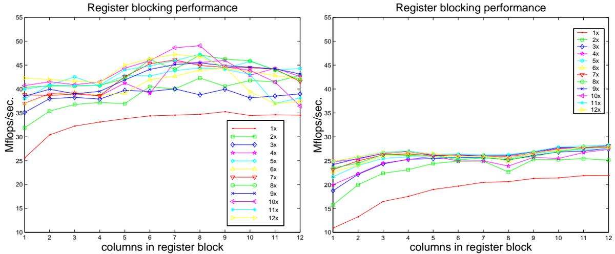
Figure 3.5: **Performance profile of register-blocked code on an UltraSPARC I (left) and a MIPS R10000 (right):** These numbers are taken for a  $1000 \times 1000$  dense matrix represented in sparse format. Each line is for a fixed number of rows ( $r$ ), varying the number of columns ( $c$ ) from 1 to 12.
