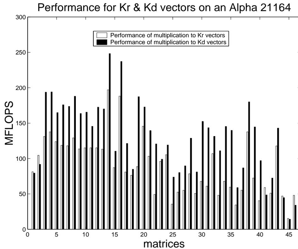
Figure 5.13: **Comparing the dense ( $k_d$ ) and random sparse ( $k_r$ ) matrices to choose the number of vectors on an Alpha 21164:** The left bar represents the performance when it is multiplied to the peak value for a dense matrix ( $k_d$ ) and the right bar represents the performance when it is multiplied to the peak value for a random matrix ( $k_r$ ).
