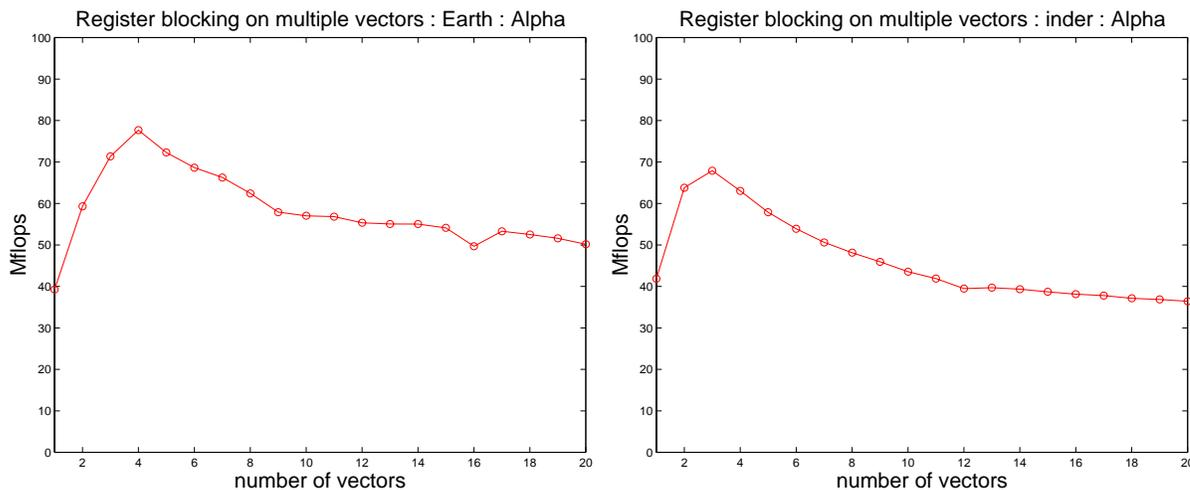
Figure 5.20: **Performance of the multiple-vector optimization on an Earth Science (left) and text retrieval (right) matrix on an Alpha 21164.**
