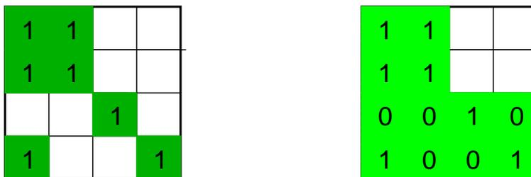
Figure 3.4: **Fill overhead of register blocking:** The BSR format in the right figure stores five extra zero values to make the  $2 \times 2$  block dense.
