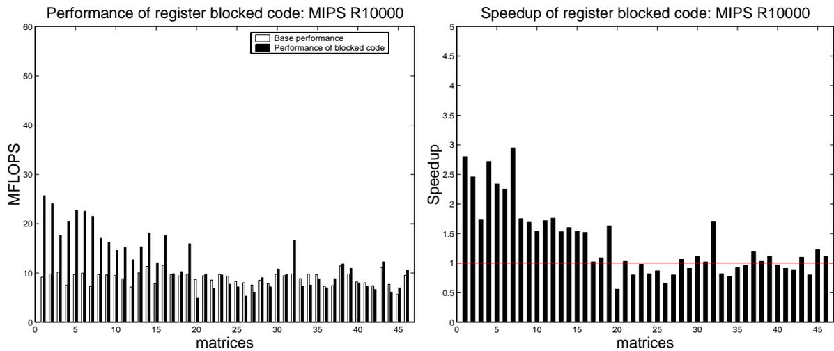
Figure 3.10: Performance of register-blocked multiplication on a MIPS 10000
