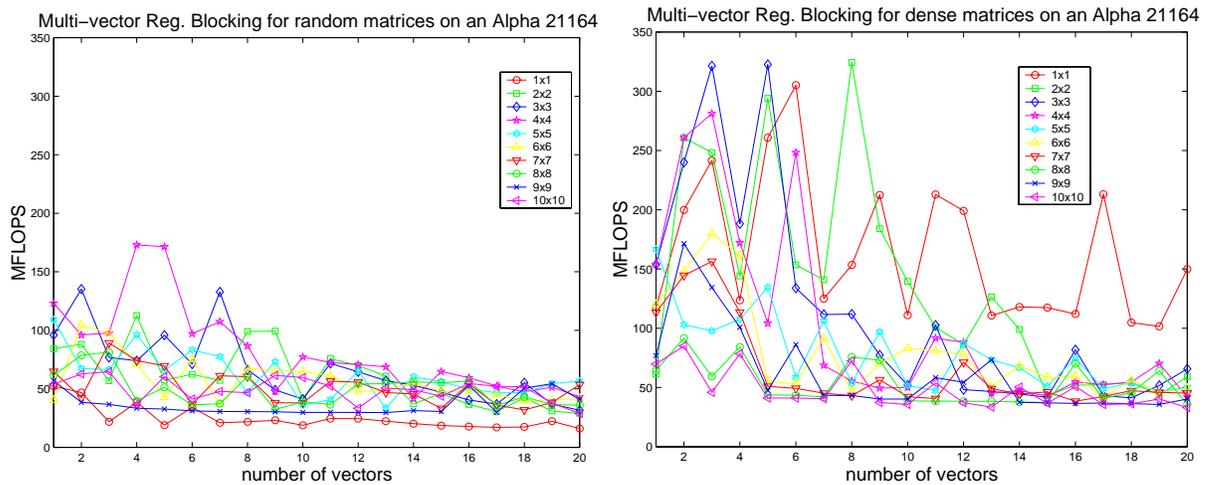
Figure 5.7: **Register-blocked, multiple vector performance on an Alpha 21164, varying the number of vectors:** The graph on the left uses a random  $10K \times 10K$  matrix with  $200K$  nonzeros, and the graph on the right uses a  $1K \times 1K$  dense matrix in sparse format. Each line indicates a different register block size. The x-axis shows the number of vectors and the y-axis shows the performance in Mflops.
