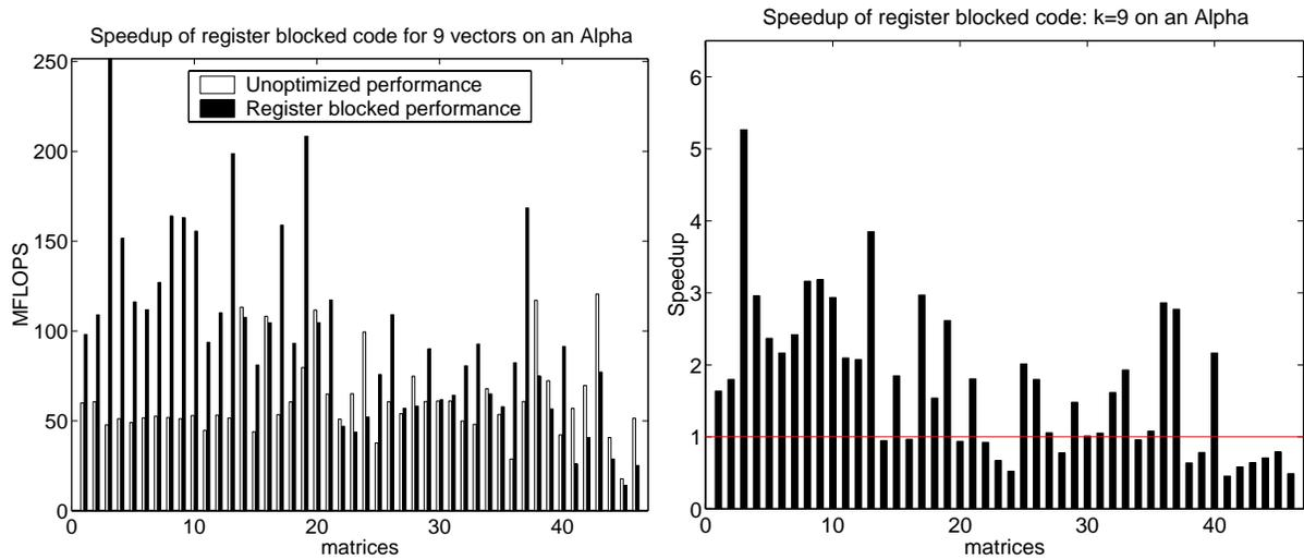
Figure 5.10: **Performance of register-blocked, multiple vector code on an Alpha 21164:** The left-hand plot shows the performance in Mflops of the unoptimized code and the multiple vector version using 9 vectors. The right-hand plot shows the speedup of multiple vectors relative to unoptimized code.
