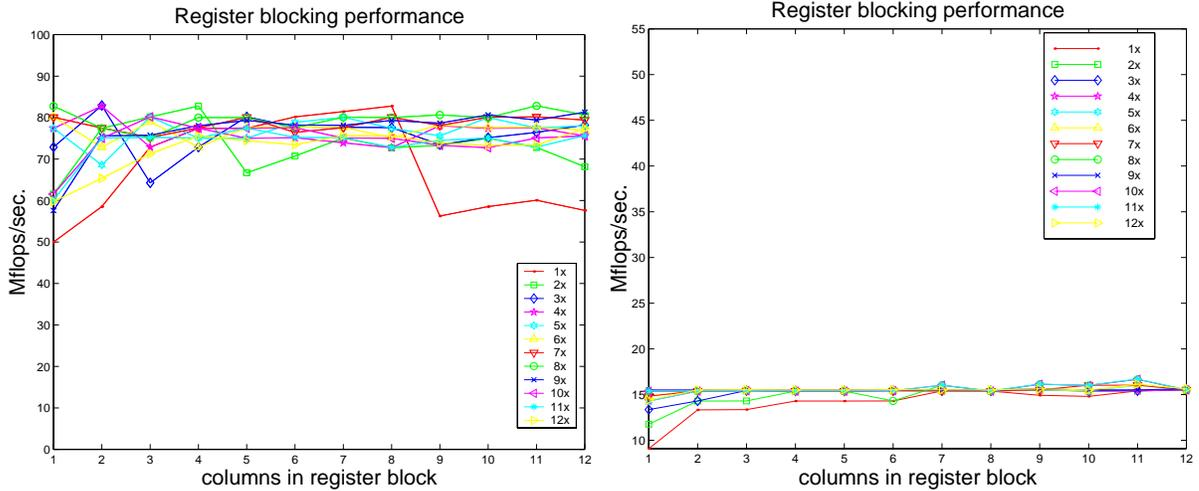
Figure 3.6: **Performance profile of register-blocked code on an Alpha 21164 (left) and a PowerPC 604e (right)** These numbers are taken for a  $1000 \times 1000$  dense matrix represented in sparse format. Each line is for a fixed number of rows ( $r$ ), varying the number of columns ( $c$ ) from 1 to 12.
