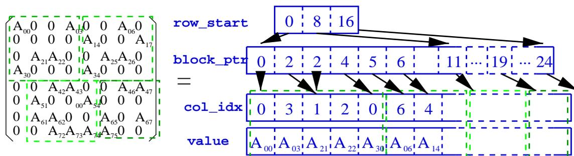
Figure 4.2: **Storage format of a cache-blocked sparse matrix:** In cache blocking, each block is stored in sparse format, similarly to CSR, using data structures *block\_ptr*, *col\_idx* and *value*. This example matrix has 4,  $4 \times 4$  blocks. The *row\_start* array points to the beginning of each row of blocks, while the *block\_ptr* array keeps pointers to the beginnings of individual rows inside those blocks.
