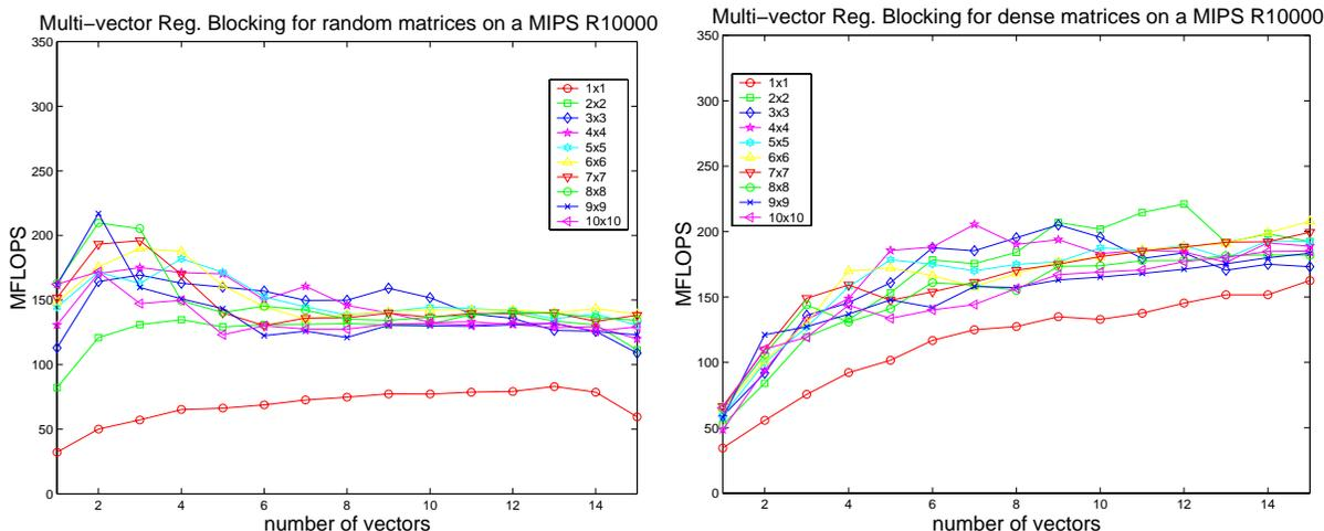
Figure 5.6: **Register-blocked, multiple vector performance on a MIPS R10000, varying the number of vectors:** The graph on the left uses a random  $10K \times 10K$  matrix with  $200K$  nonzeros, and the graph on the right uses a  $1K \times 1K$  dense matrix in sparse format. Each line indicates a different register blocking. The x-axis shows the number of vectors and the y-axis shows the performance in Mflops.
