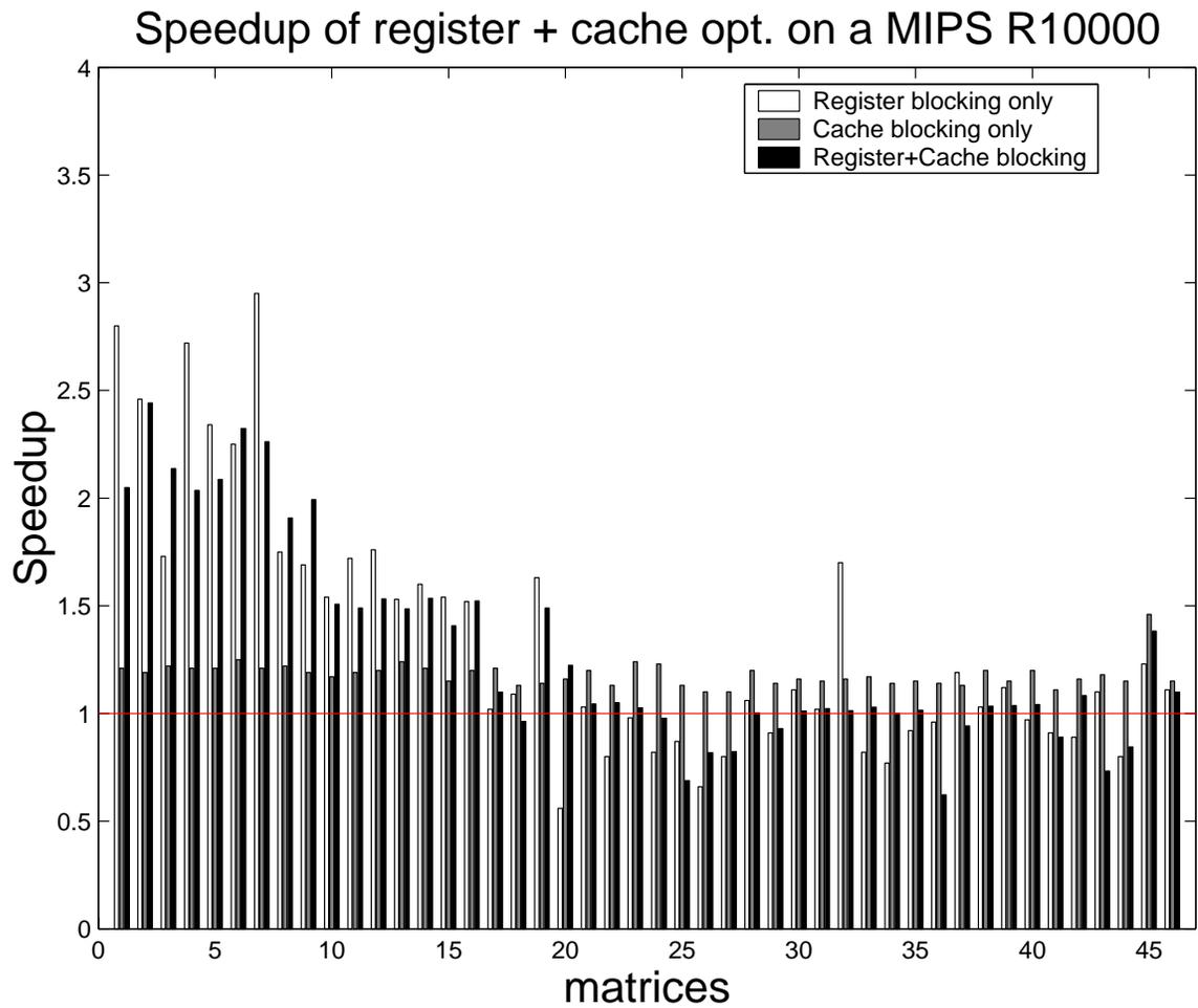
Figure 4.16: Speedup of register and cache blocked multiplication on a MIPS R10000
