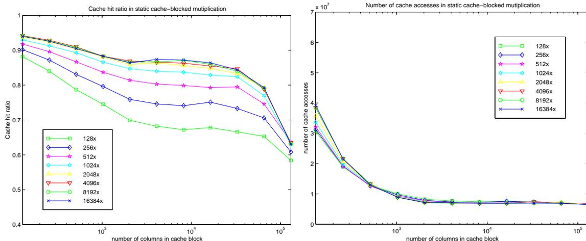
Figure 4.6: **Cache behavior of static cache-blocking on the LSI matrix:** The left figure shows the L2 cache hit ratio and the right figure shows the total number of cache accesses.
