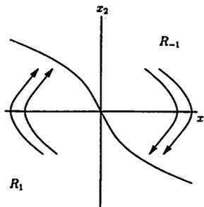
Fig. 7. The switching curve for the double integrator system.
