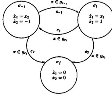
Fig. 1. Hybrid automaton for time optimal control of a double integrator system
