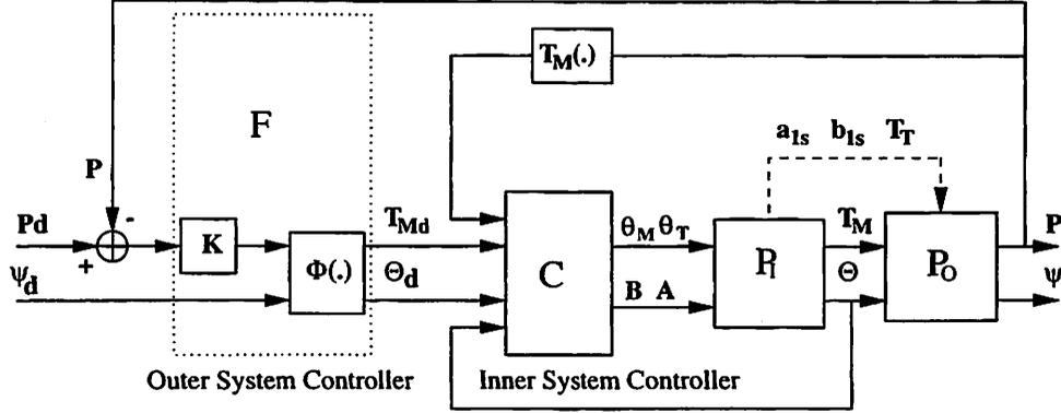
Figure 3.6: Block diagram of control scheme.
