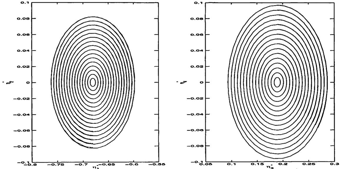
Figure 3.4: Phase portrait of zero dynamics in position and heading control mode
