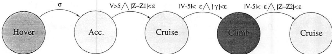
Figure 4.1: Control mode switching for high-altitude take-off of a helicopter. The switching sequence and conditions are based on flight instruction for pilots
