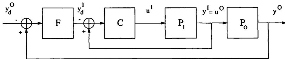
Figure 3.5: Partitioned inner and outer systems.
