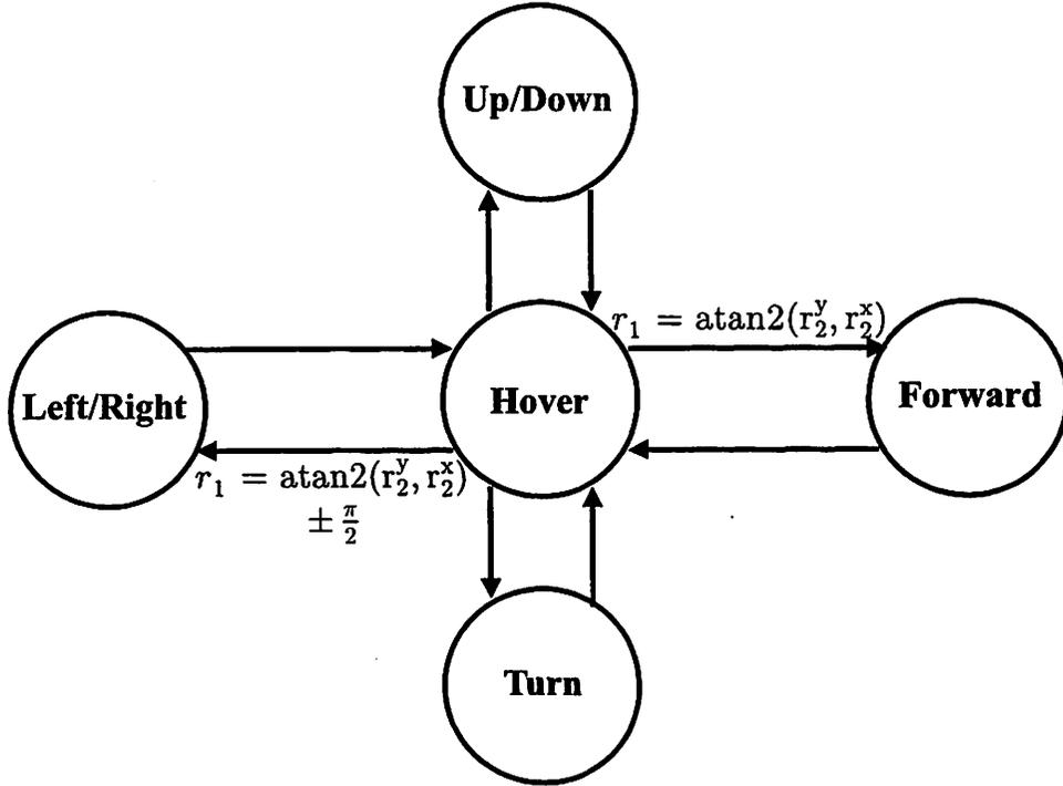
Figure 5.6: Control mode graph of helicopter maneuvers.
