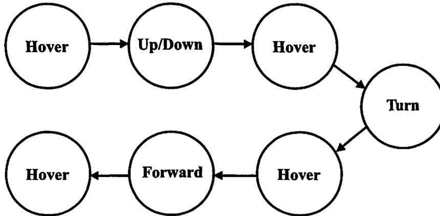
Figure 5.7: FSM representation of Trajectory Planner.
