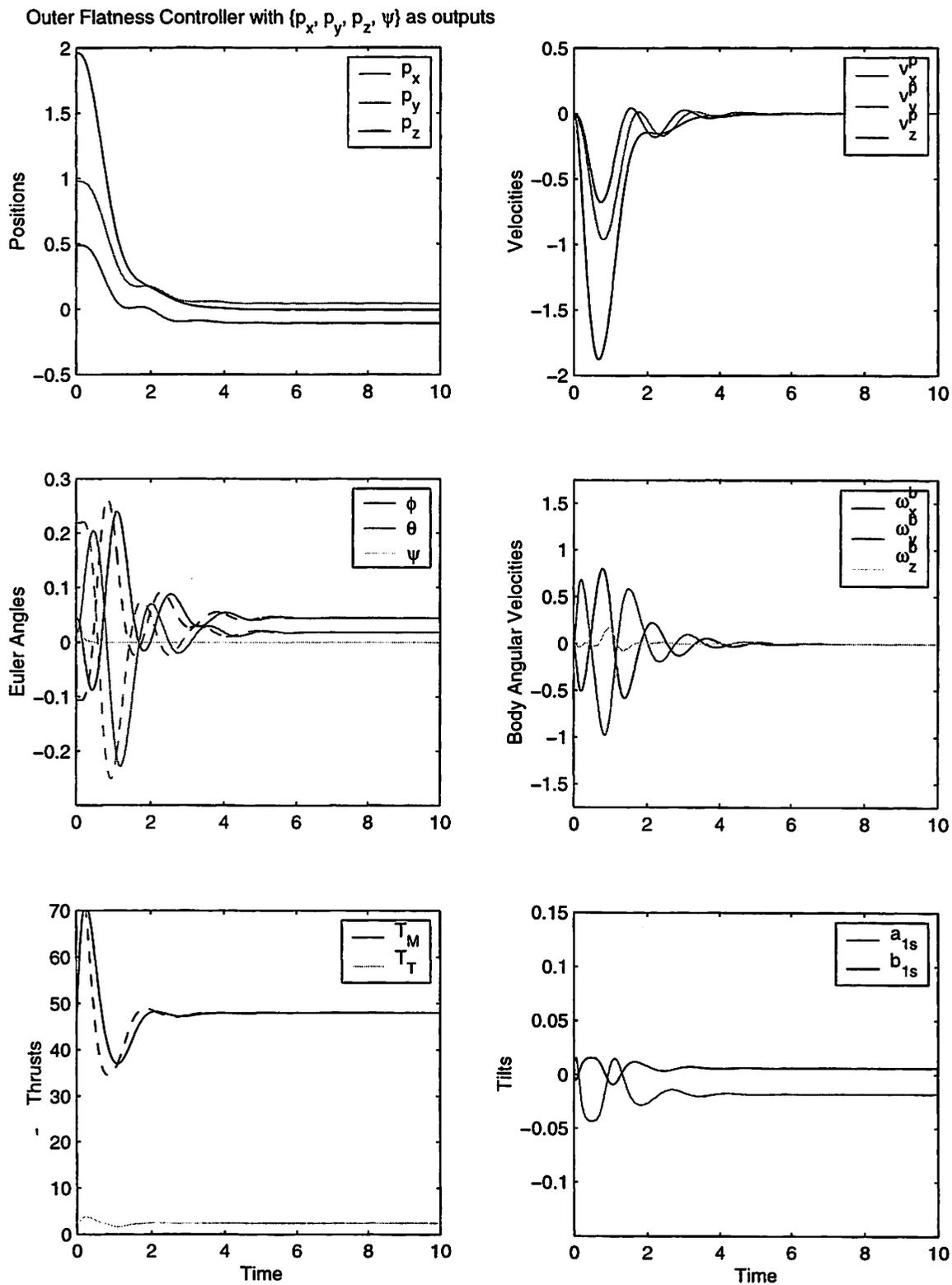
Figure 3.9: Nonlinear control design based on outer flatness with outputs  $\{p_x, p_y, p_z, \psi\}$ . Notice that the dashed lines represent the desired trajectories of  $\phi, \theta, T_M$ .
