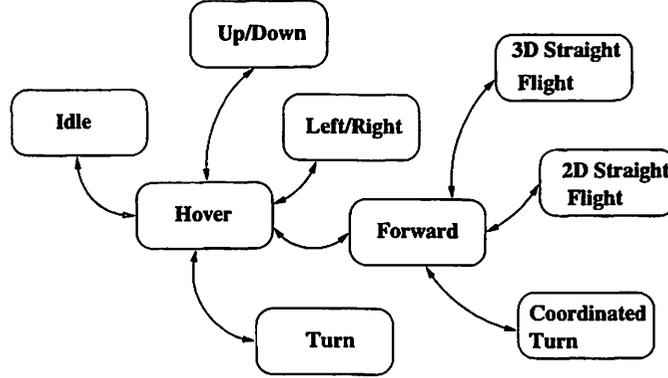
Figure 5.5: Transitions diagram of helicopter maneuvers
