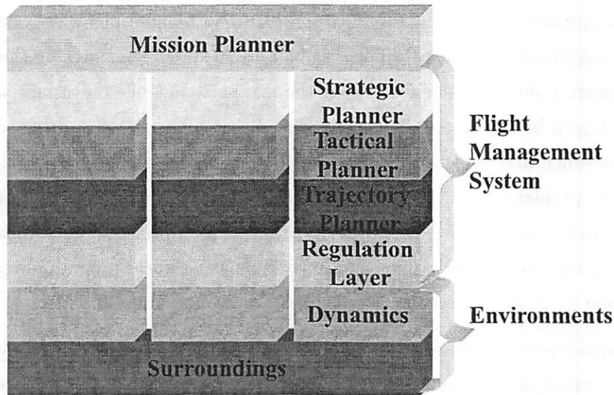
Figure 2.2: Each agent is equipped with a Flight Management System(FMS) which is reactive to mission planner and environments
