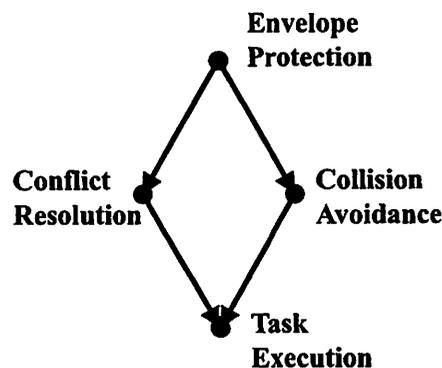
Figure 2.3: In the directed graph, each node represents a mode of operation and each arrow connects a higher priority to a lower one.
