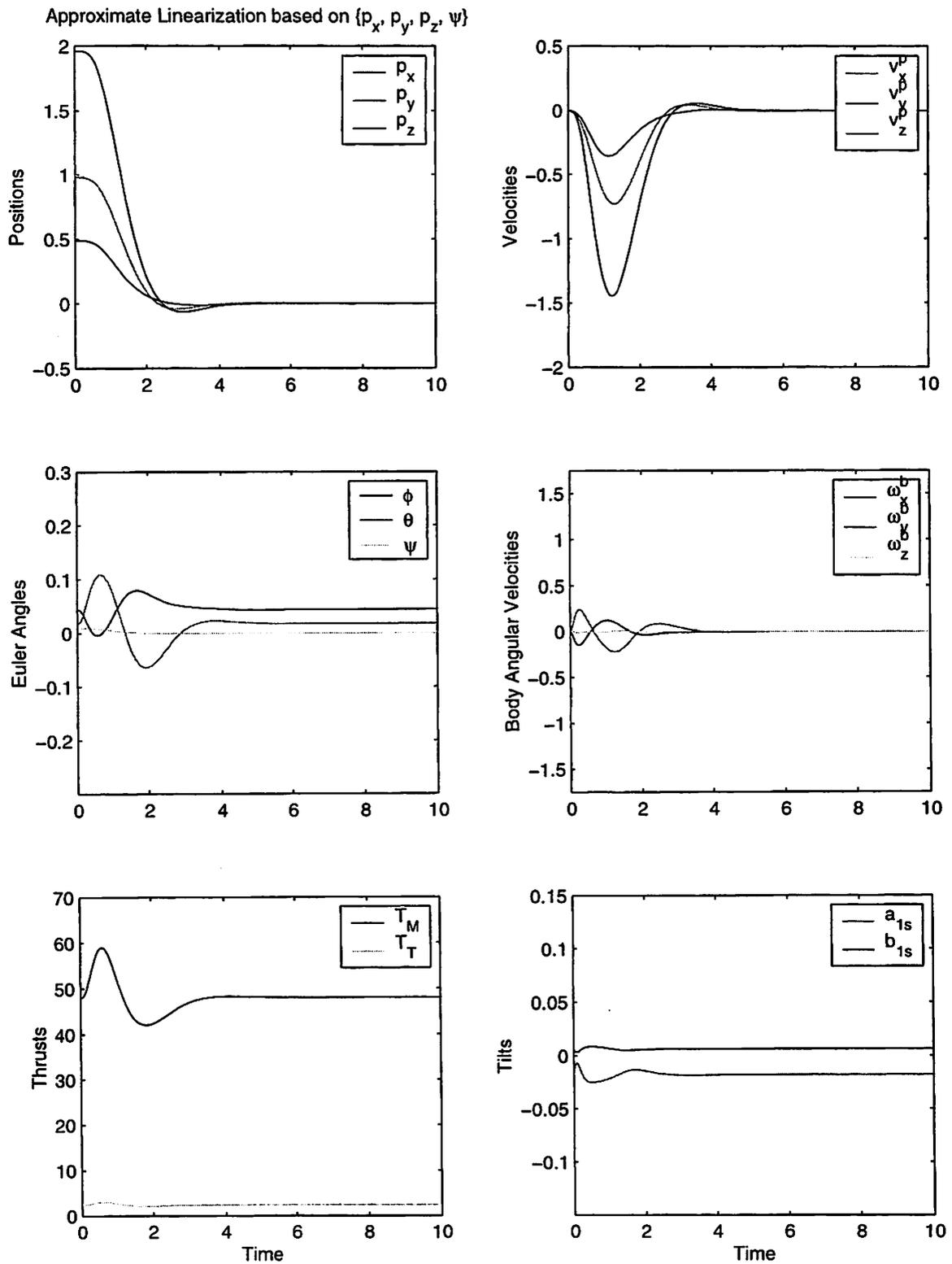
Figure 3.8: Approximate input-output linearization applied on outputs  $\{p_x, p_y, p_z, \psi\}$
