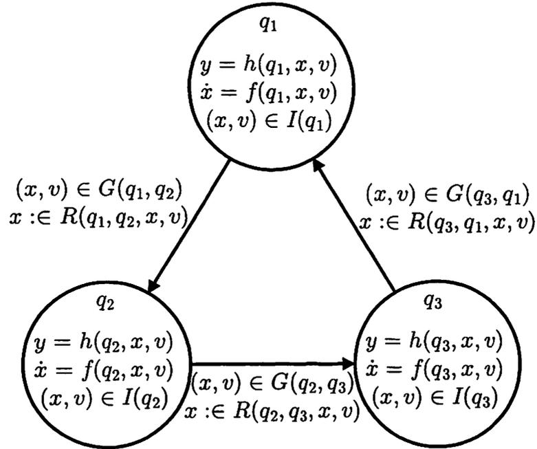
Figure 2.1: Definition of Hybrid Automaton
