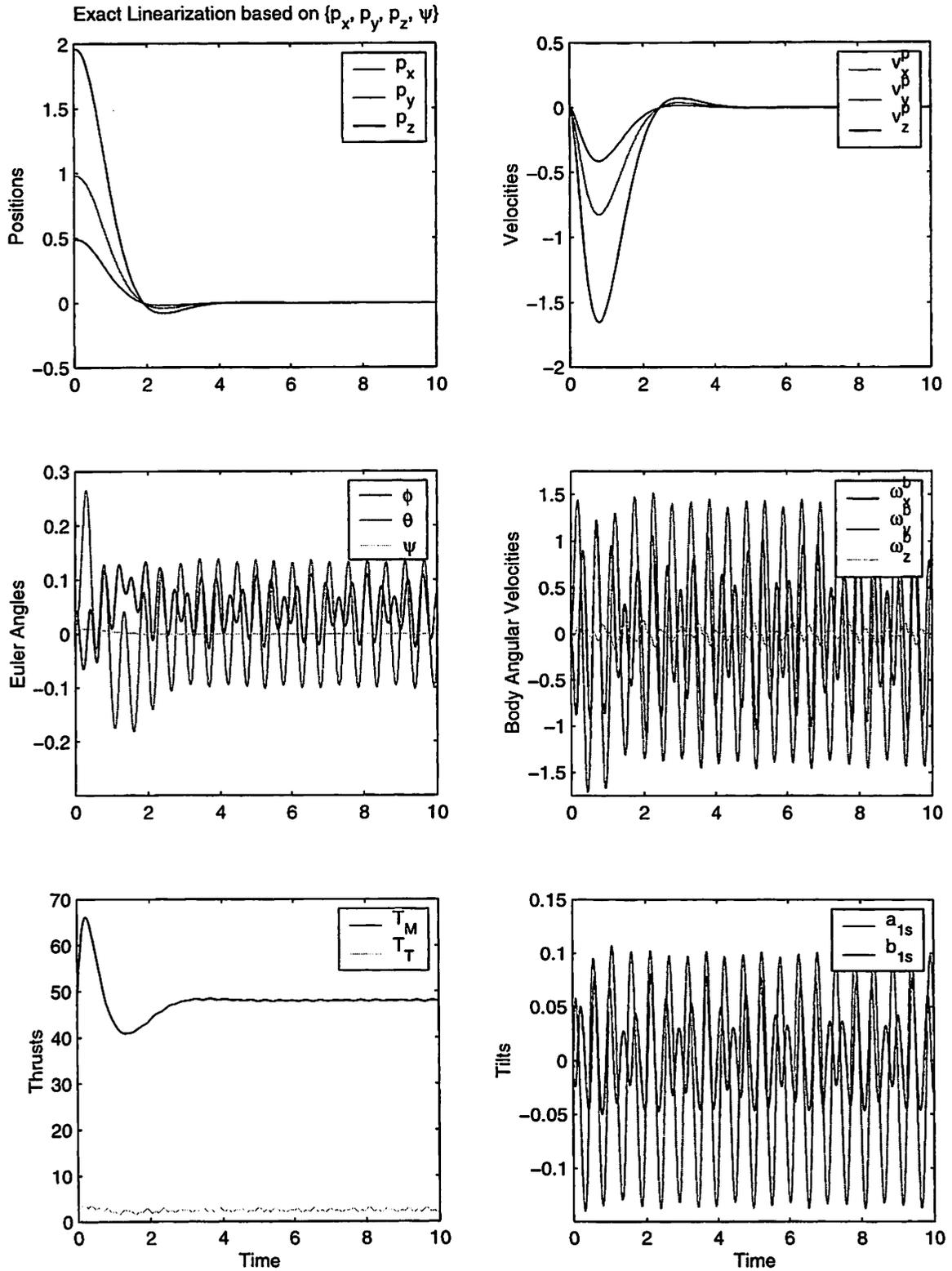
Figure 3.7: Exact input-output linearization applied on outputs  $\{p_x, p_y, p_z, \psi\}$
