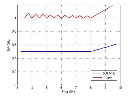
Figure 5: Bandwidth as a function of carrier frequency for a fixed divider architecture
