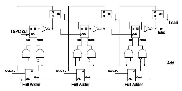
Figure 9: Programmable Divider
