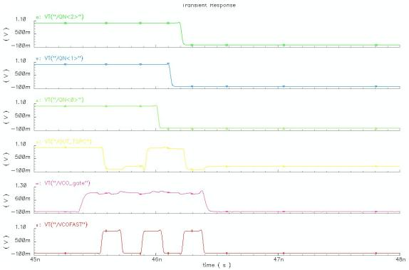
Figure 12: Divider waveforms for div 2 at 3 GHz (error occur)
