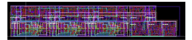
Figure 14: Programmable Divider Layout
