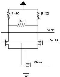
Figure 7: Power Amplifier /Antenna Driver
