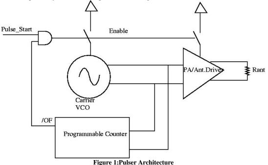
Relying on the accuracy of the VCO obviates the need for bandwidth calibration, and hence of an off the chip frequency reference.
