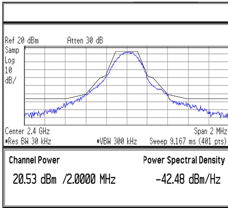
Figure 6.23: Output spectrum with GSM/EDGE signal. Measured PSD at offset frequencies are: at  $\pm 200$ -kHz, -30.75-dBc, -30.3-dBc (spec: -30-dBc); at  $\pm 400$ -kHz, -55.3-dBc, -55-dBc (spec: -54-dBc); at  $\pm 600$ -kHz, -64.4-dBc, -63.9-dBc (spec: -60-dBc)
