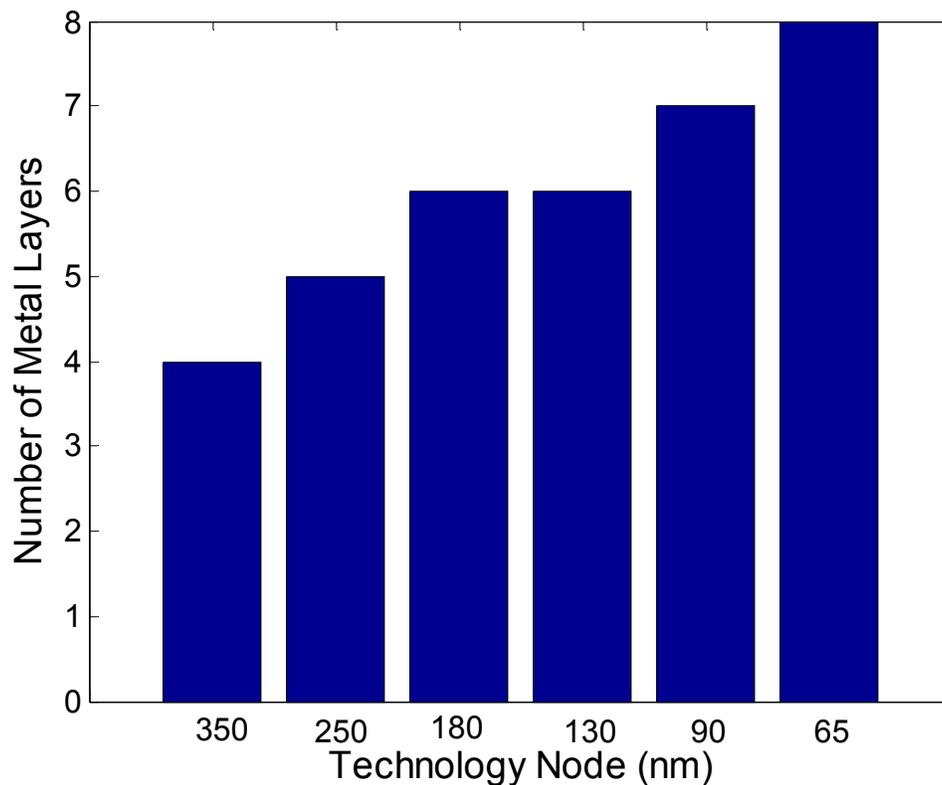
Figure 3.18: Number of Metallization layers vs. technology node
