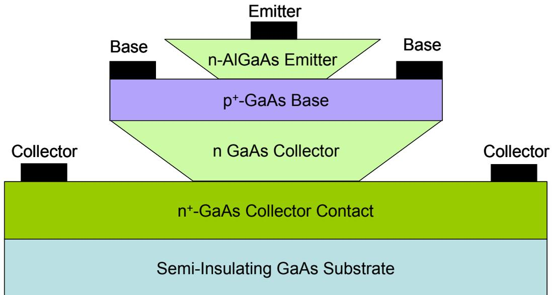
Figure 3.1: An npn GaAs HBT cross-section
