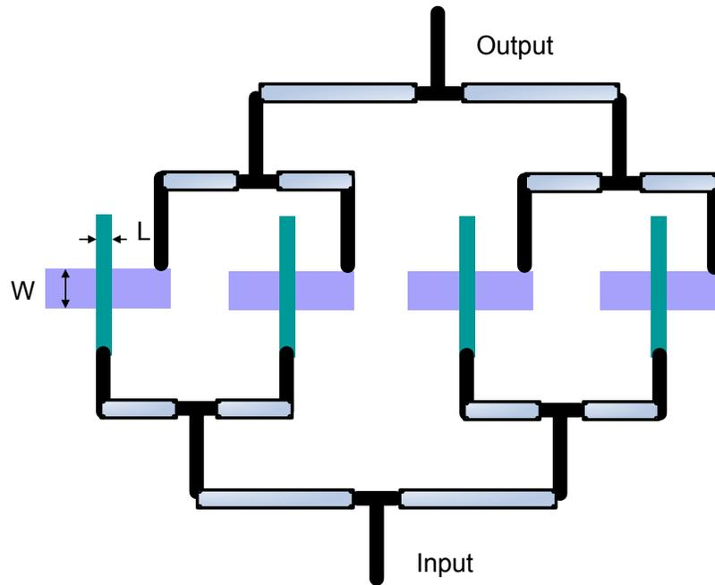
Figure 6.9: A power transistor laid out in "tree" layout.
