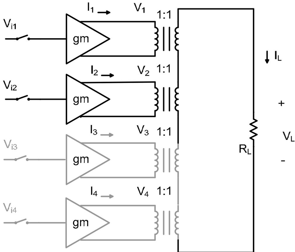
Figure 4.15: A four-way power combining amplifier is reconfigured to a two-way power combining amplifier with digital control for enhanced average efficiency.
