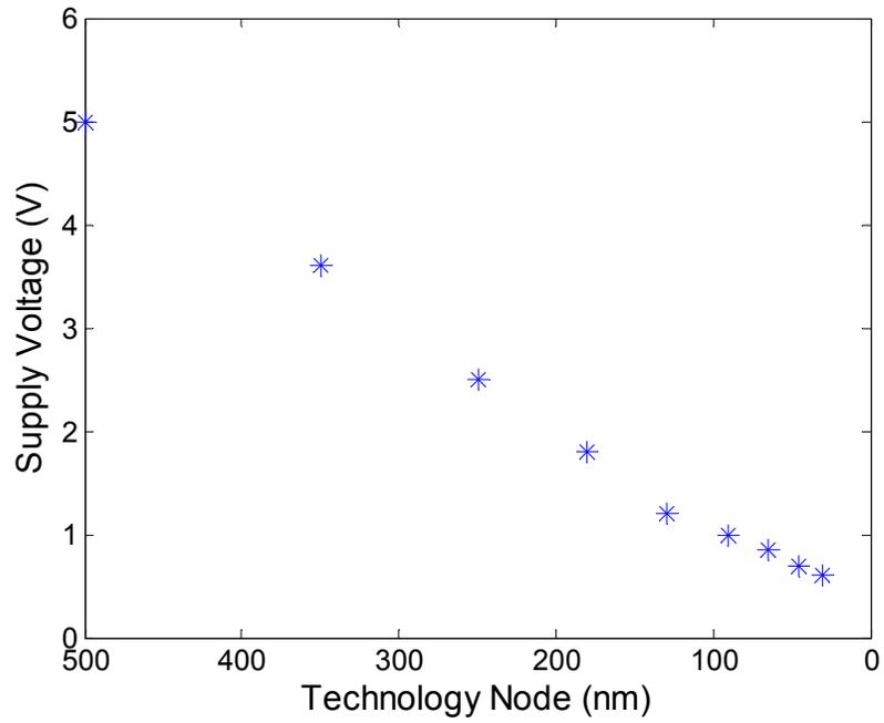
Figure 3.15: Recommended supply voltage as CMOS scaling continues (data collected from ITRS website)
