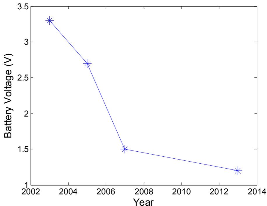
Figure 3.14: Battery voltage projection published by iNEMI
