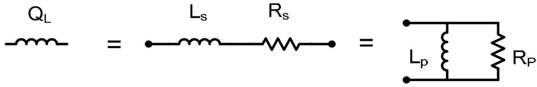
Figure 5.2: Equivalent models of an inductor with quality factor  $Q_L$
