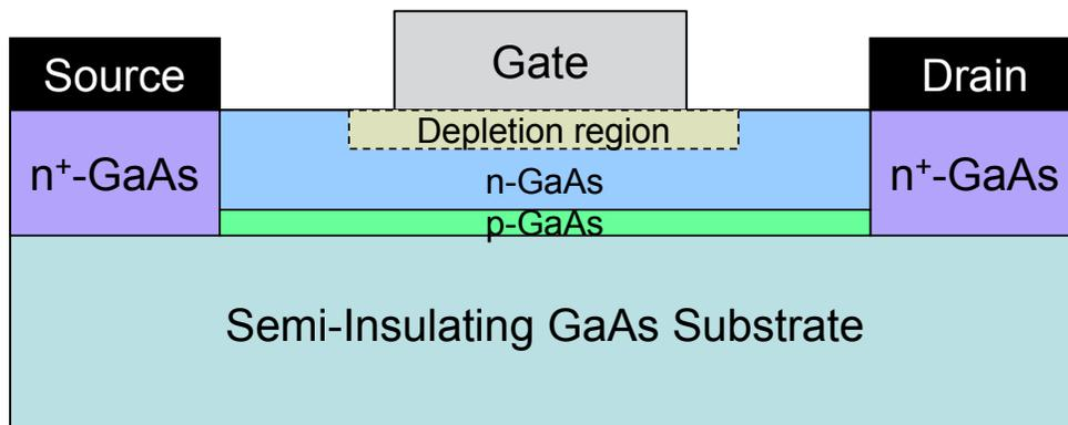
Figure 3.2: A GaAs MESFET cross-section
