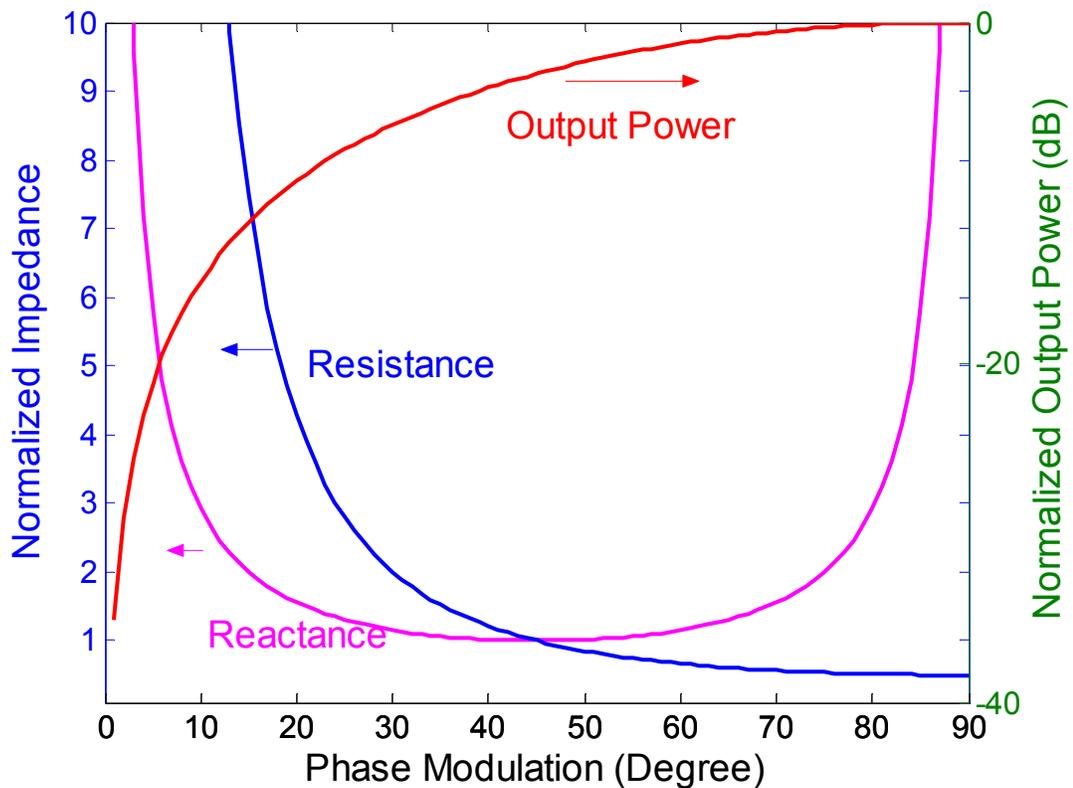
Figure 4.23: Resistance, reactance of the parallel equivalent circuit model, and total output power with phase modulation. (Note:  $R_L$  and  $V$  are normalized with the value of 1).
