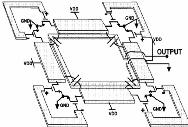
Figure 4.5: An 8-way power combined PA with DAT in [4.6]
