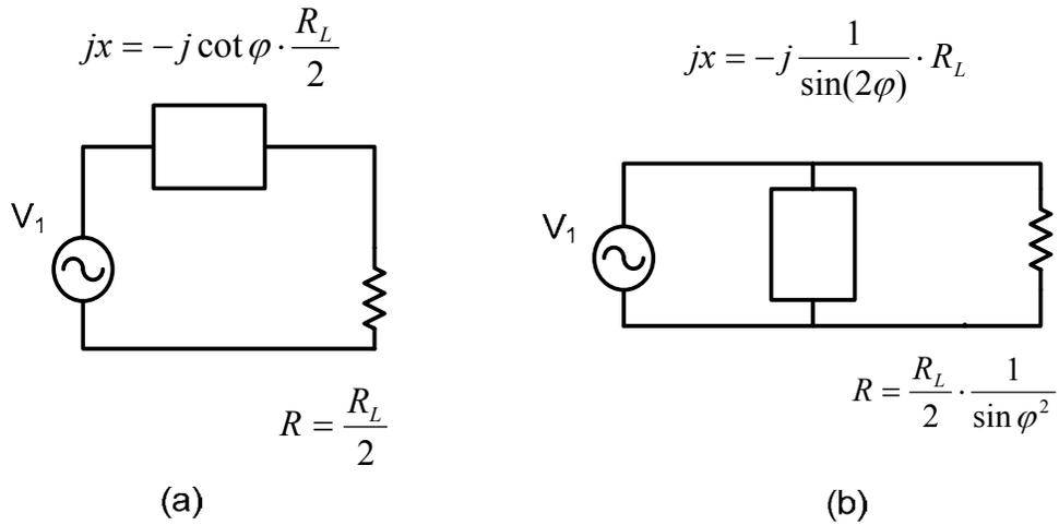
Figure 4.21: (a) RF load seen by the RF generator  $V_1$ ; (b) A parallel equivalent model
