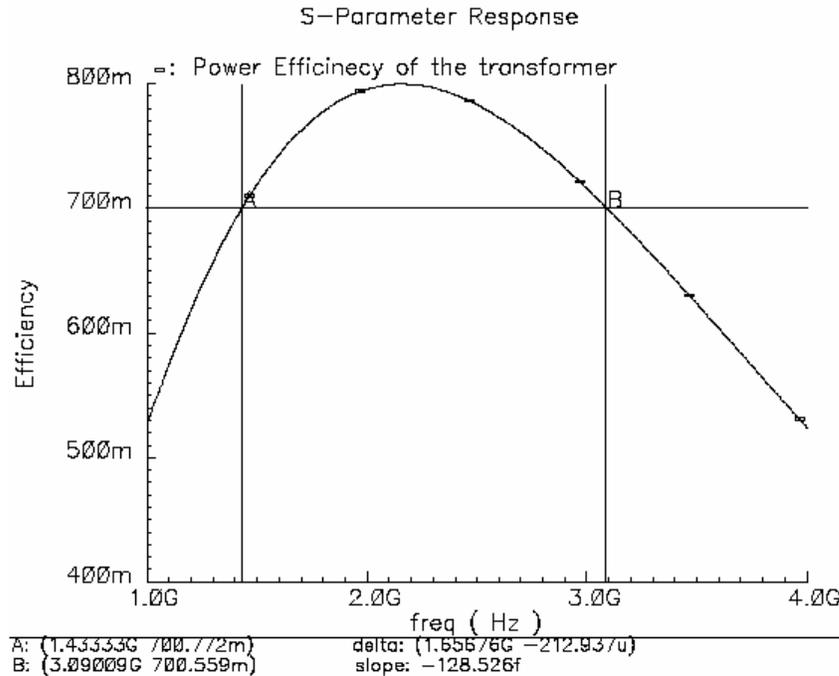
Figure 5.22: Power efficiency vs. frequency for a transformer designed at 2-GHz
