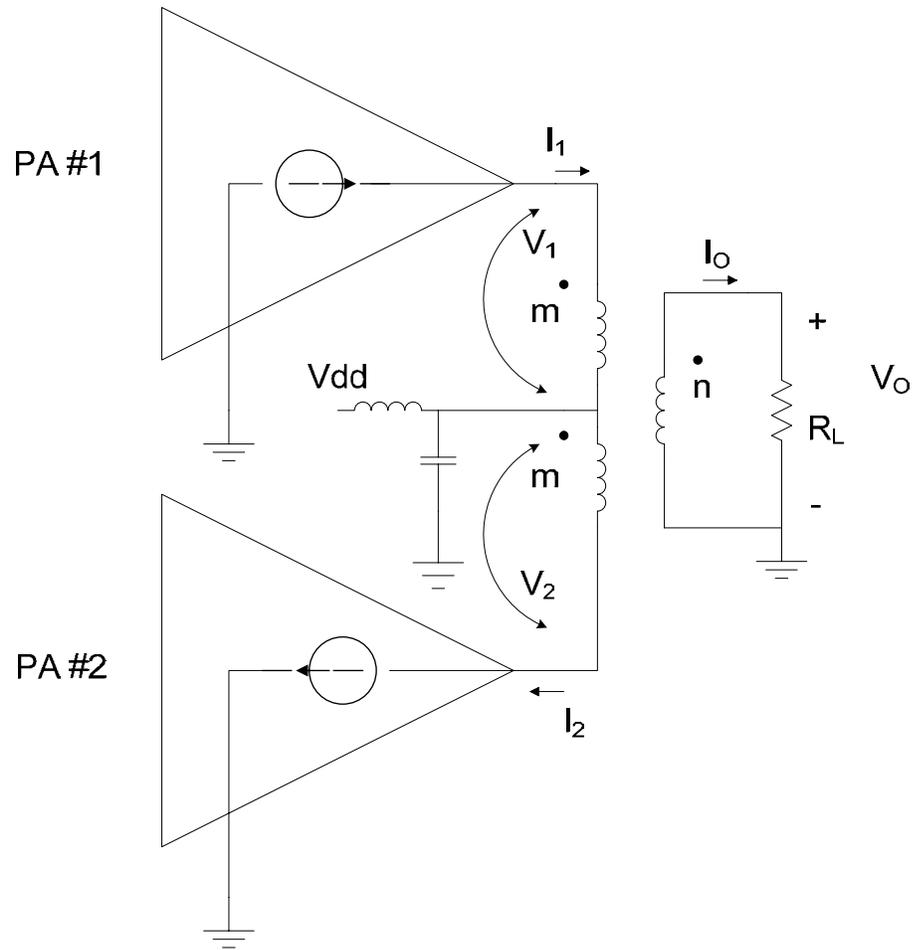
Figure 4.4: A two-way power combined amplifier with transformers
