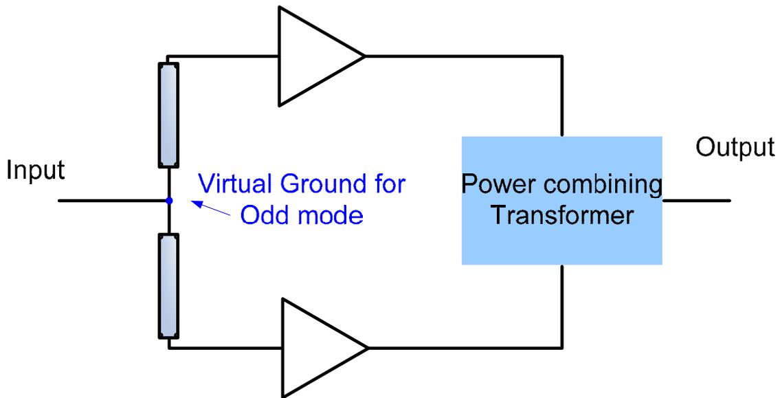
Figure 6.7: A two-way power combined amplifier. Notice the virtual ground of odd mode oscillation.
