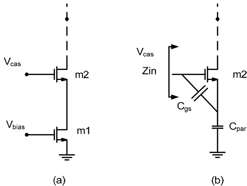
Figure 6.4: (a) A simplified cascode configuration, where m1 is the transconductor device and m2 is the cascode device; (b) An equivalent model for stability analysis.
