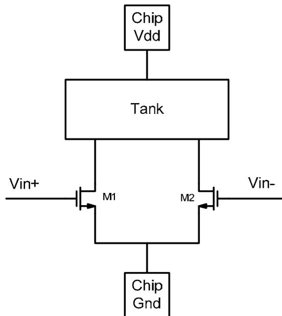
Figure 6.1: A pseudo-differential pair in power amplifier designs
