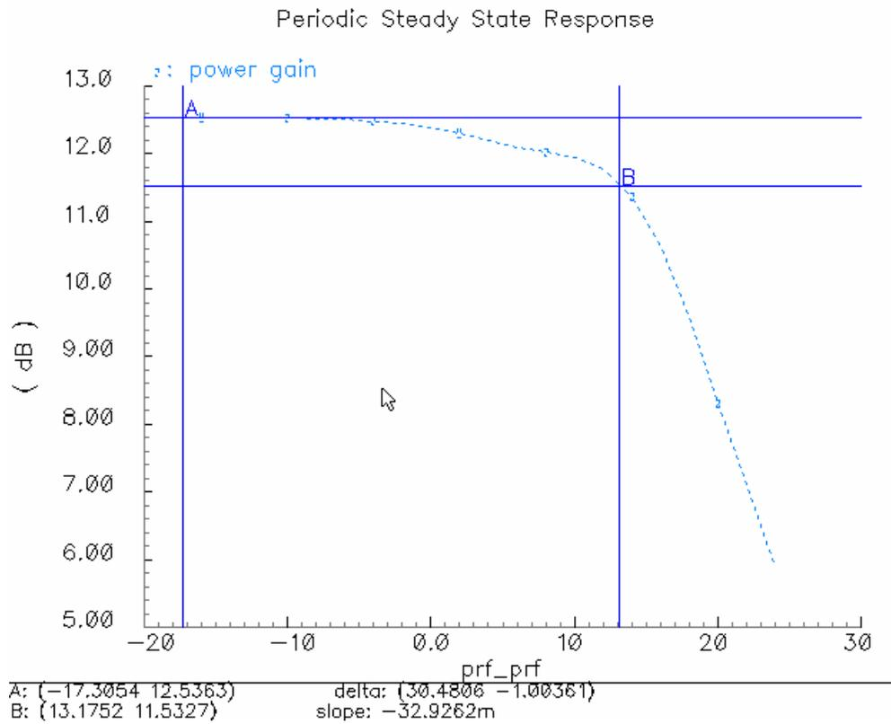
Figure 6.16: The power gain of the prototype when all unit amplifiers are on.
