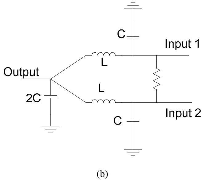
Figure 4.9: (a) A two-way Wilkinson power combiner; (b) Lumped equivalent
