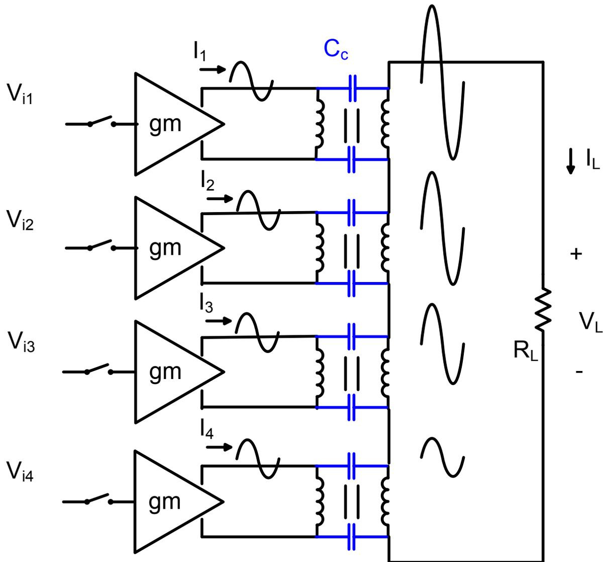
Figure 5.16: Capacitive coupling of the power combining transformer will cause some amplifiers break down earlier than others.
