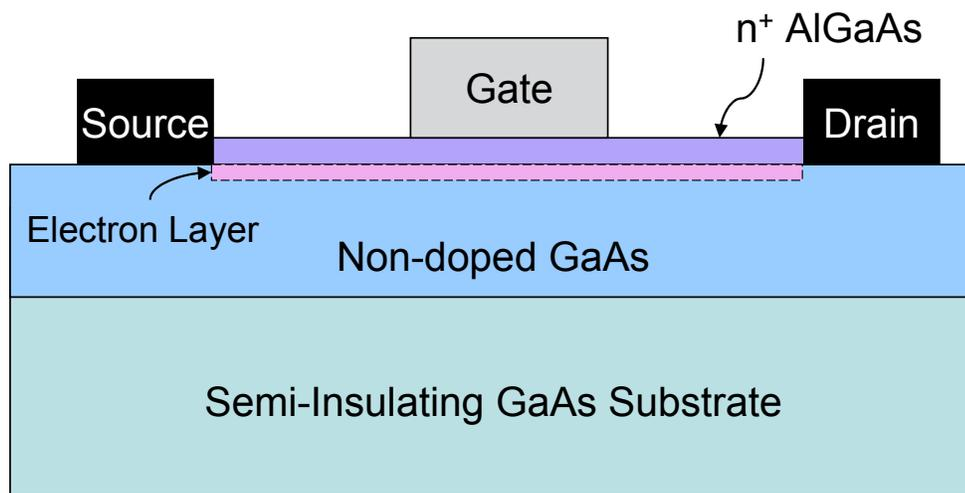
Figure 3.3: A GaAs/AlGaAs HEMT cross-section
