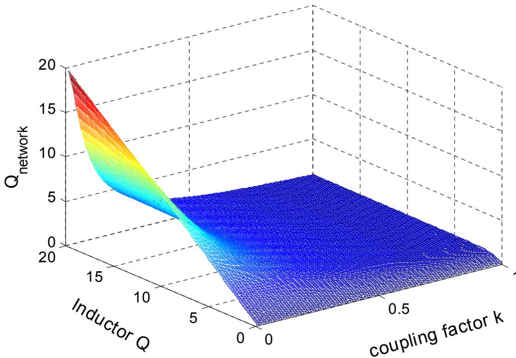
Figure 5.9:  $Q_{network}$  of a 1:n transformer vs. coupling factor and  $Q_{ind}$ , assuming  $Q_1 = Q_2$
