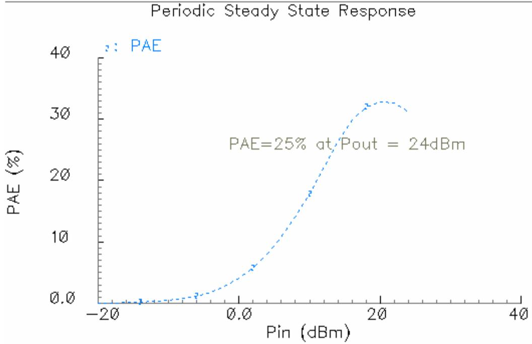
Figure 6.17: One tone simulation results when all unit amplifiers are on.
