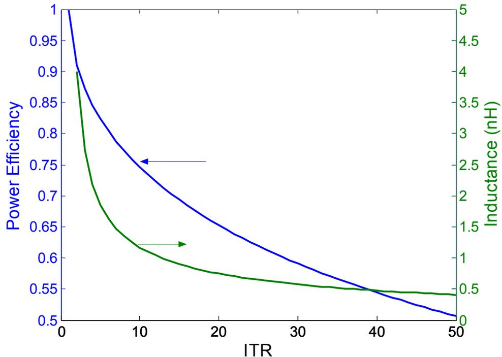
Figure 5.4: Power efficiency and required inductance of a single stage “L-match” network at 2-GHz with inductor  $Q_L = 10$ .
