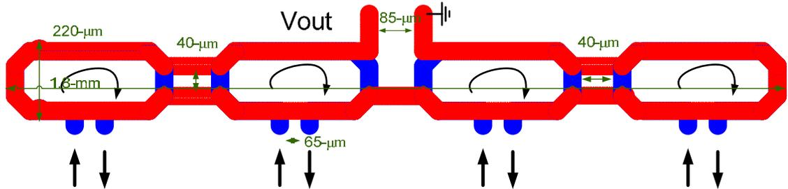
Figure 6.13: The power combining transformer in the prototype
