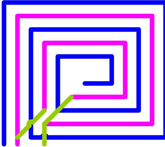
Figure 5.12: An on-chip high turn ratio transformer with shunted primary
