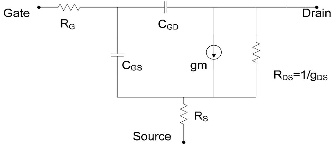
Figure 3.12: A simplified small-signal model for MOSFET
