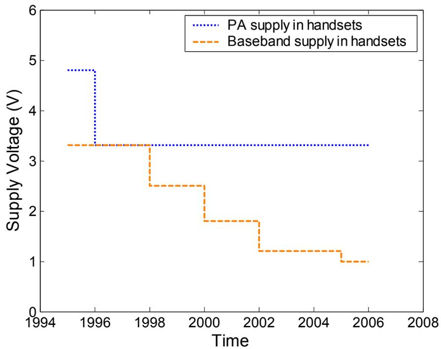
Figure 3.16: The disparity between supply voltages for PAs and that for digital circuits
