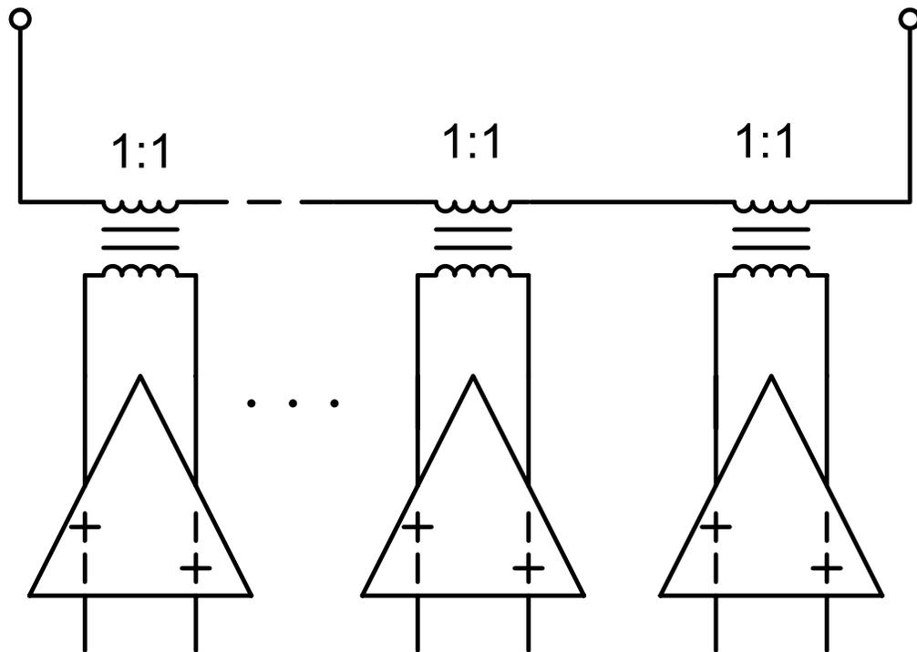
Figure 4.10: Transformer based power combining employing unity transformers<sup>28</sup>
