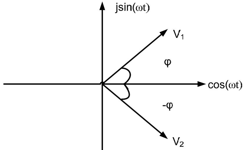
Figure 4.20: Phasor form of two voltages at the output of the two nonlinear power amplifiers for power combining.
