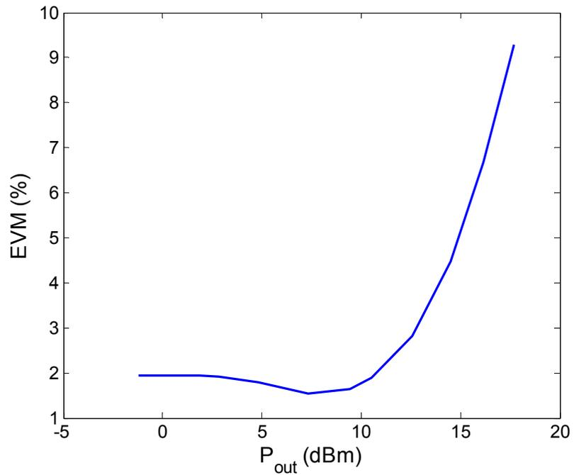
Figure 6.25: Measured EVM vs. output power
