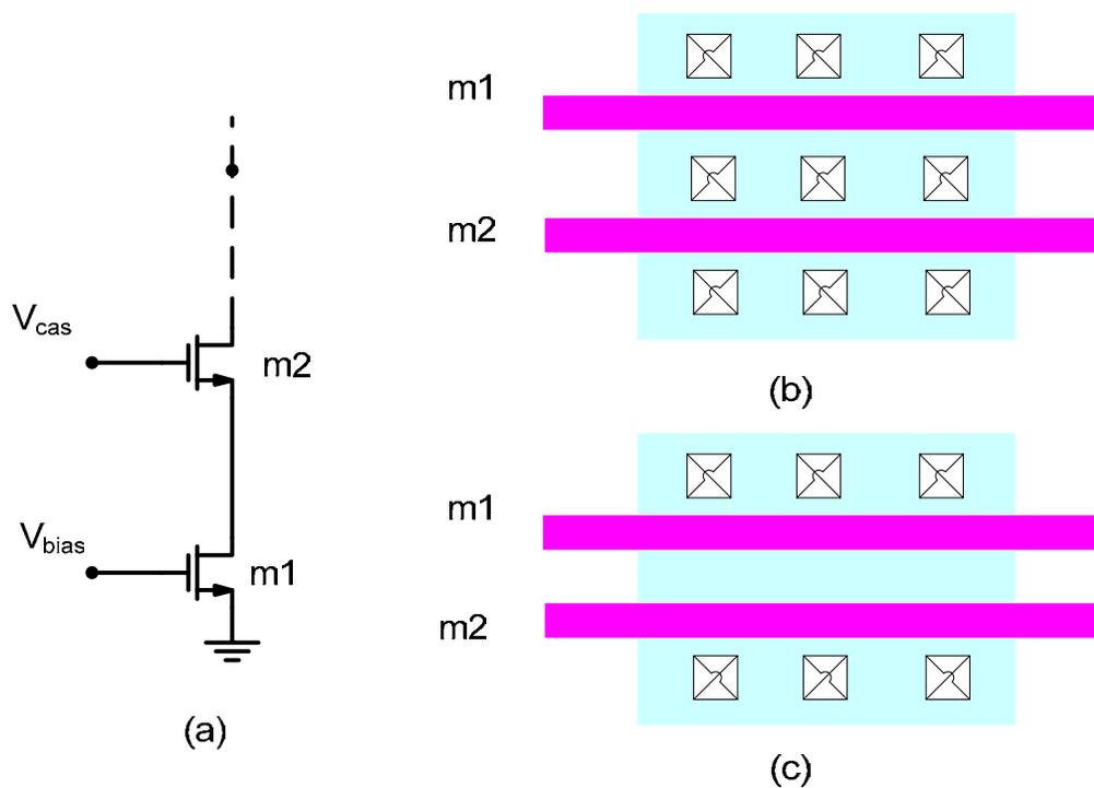
Figure 6.11: (a) The schematic of a cascode circuit; (b) The conventional layout of a cascode circuit, in which cascode devices have the same width; (c) The improved layout of a cascode circuit, with reduced parasitic capacitance at the shared junction.
