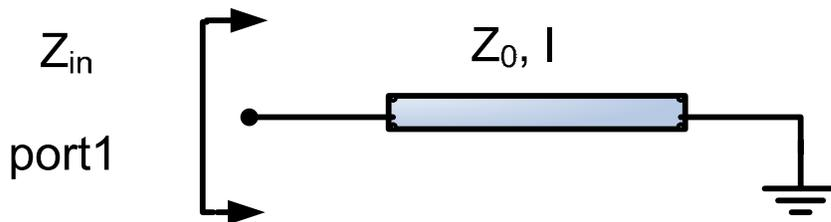
Figure 5.13: A transmission line with one port short-circuited to ground
