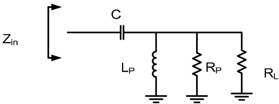
Figure 5.3: A single stage “L-match” resonant matching network with the inductor loss
