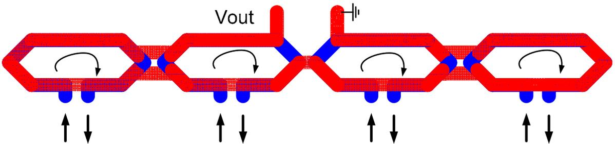
Figure 5.19: A power combining transformer with reduced magnetic coupling between adjacent windings.
