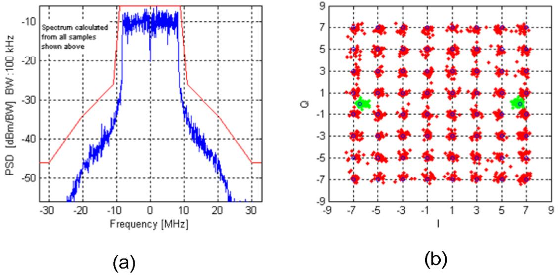
Figure 6.24: Measured at  $P_{\text{out}} = 14.5\text{-dBm}$  with 4.48% EVM. (a) Output spectrum; (b) Rectangular constellation diagram
