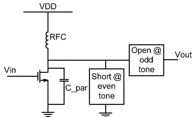
Figure 2.4: A class-F power amplifier with tuned harmonics for waveform shaping
