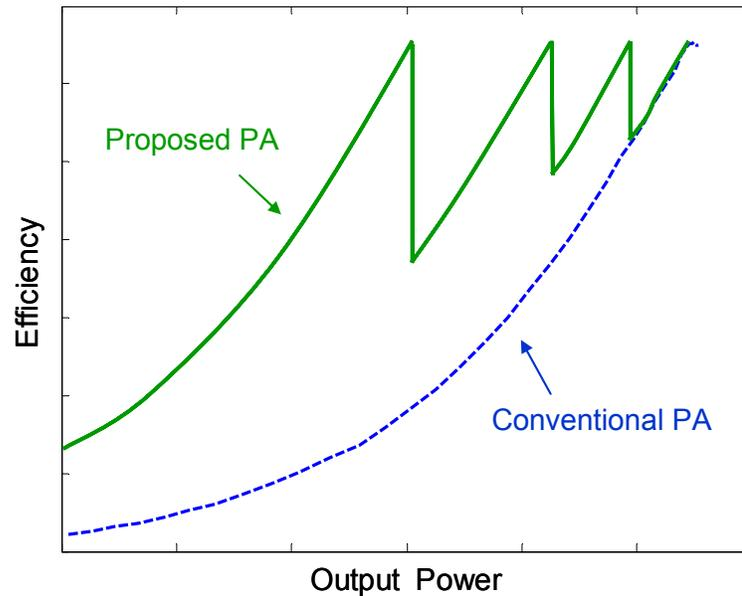
Figure 4.16: A comparison of efficiency between the PA based on proposed power combining transformer and the conventional PA
