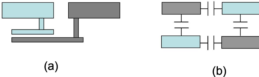
Figure 3.11: The cross section of (a) A MIM capacitor; (b) A finger capacitor
