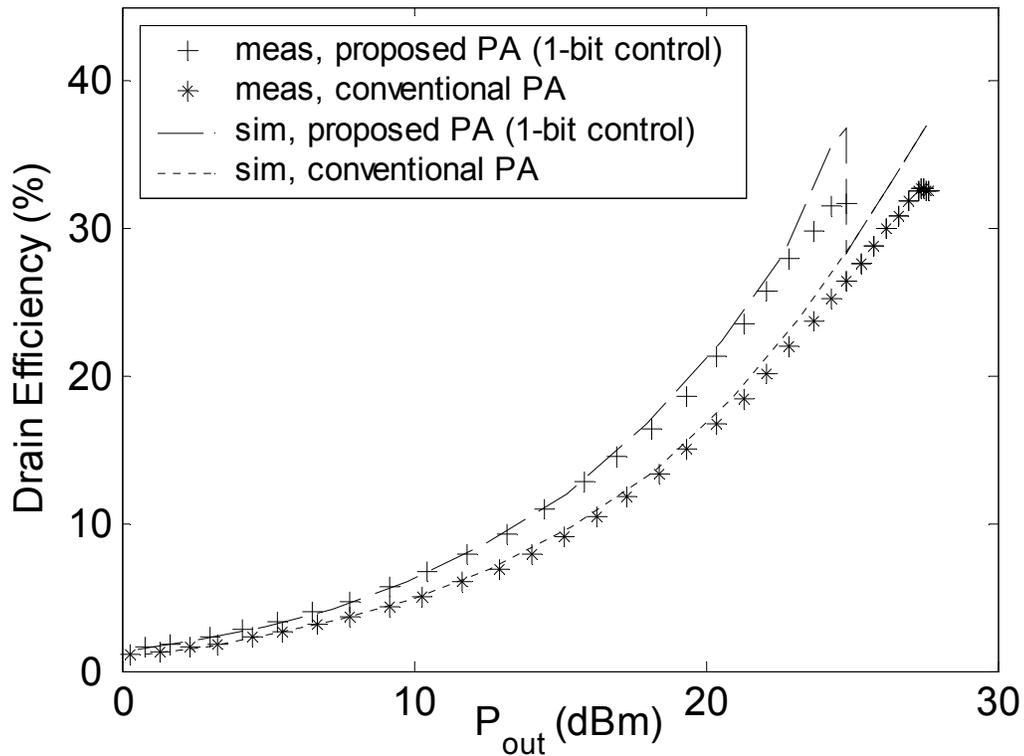
Figure 6.21: Simulated and measured drain efficiency of the proposed PA, in comparison with those for the conventional PA.
