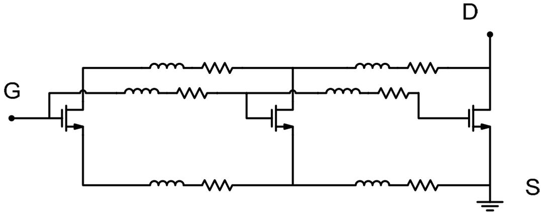
Figure 6.2: A transistor model for power transistors including inductive and resistive parasitic elements
