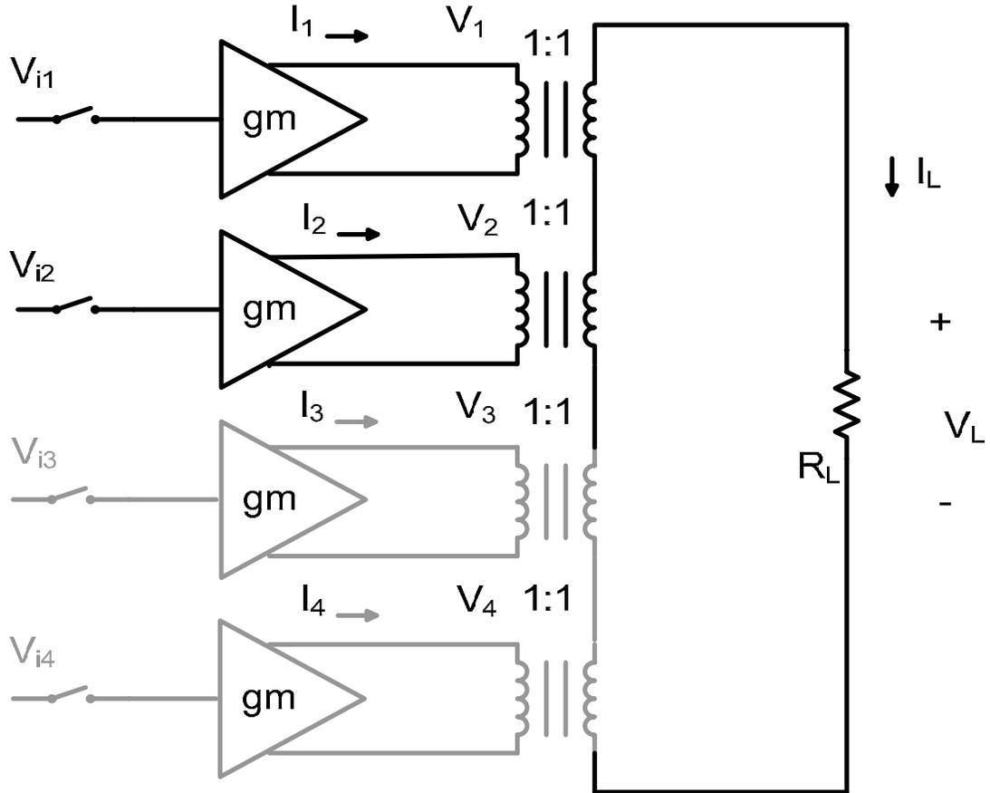
Figure 6.5: An equivalent model of a power combining amplifier. Two amplifiers are turned off, while the other two remain on.
