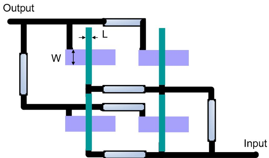
Figure 6.10: A delay-equalized compact layout of a power transistor.
