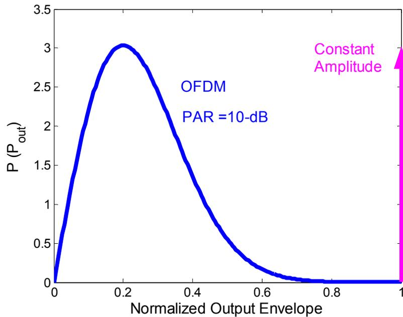
Figure 2.5: PDF of multi-carrier OFDM signals with Rayleigh distribution ( $\sigma=0.2$ ) at its maximum output. The corresponding PAR is approximately 10-dB. In contrast, the constant amplitude signal is always at peak power.
