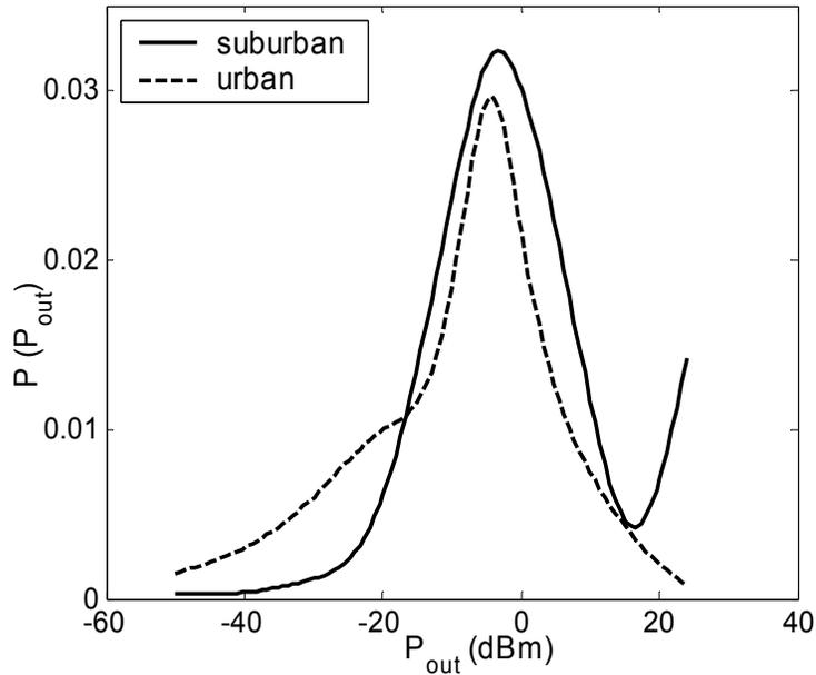
Figure 2.6: Output Power PDF of a single carrier mobile transmitter
