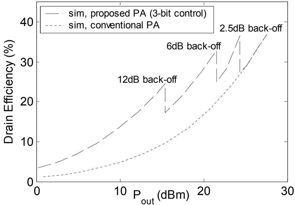
Figure 6.22: Simulated drain efficiency of the proposed PA with power back-off, in comparison with that for the conventional PA
