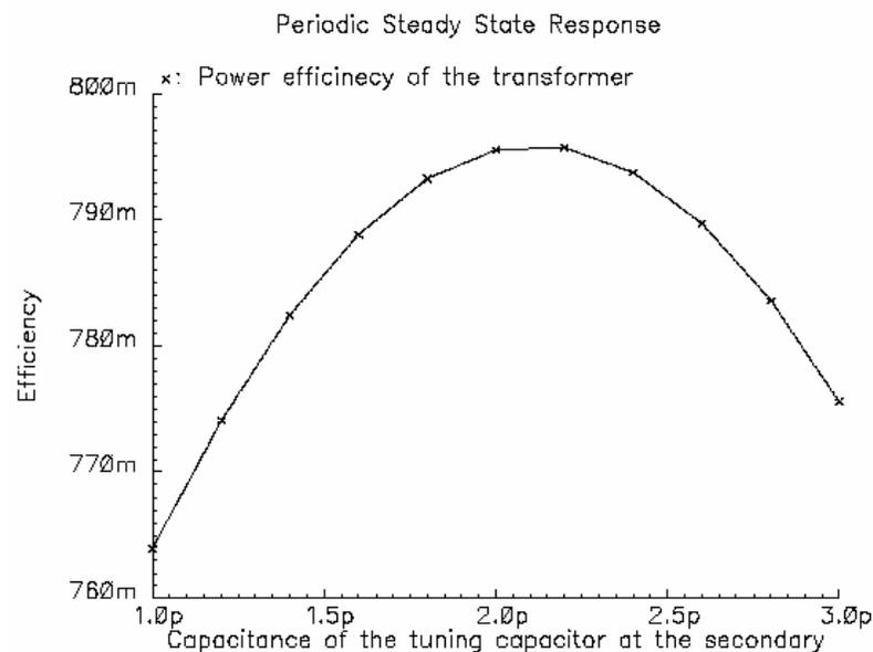
Figure 5.21: Power efficiency vs. the secondary tuning capacitance at 2-GHz
