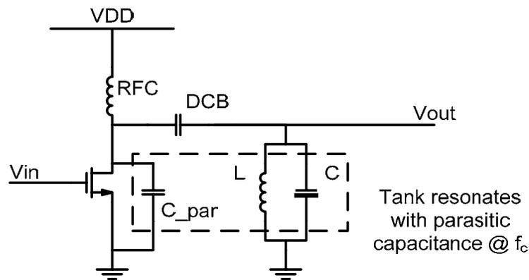
Figure 2.1: A generic topology for class-A, AB, B, and C power amplifiers
