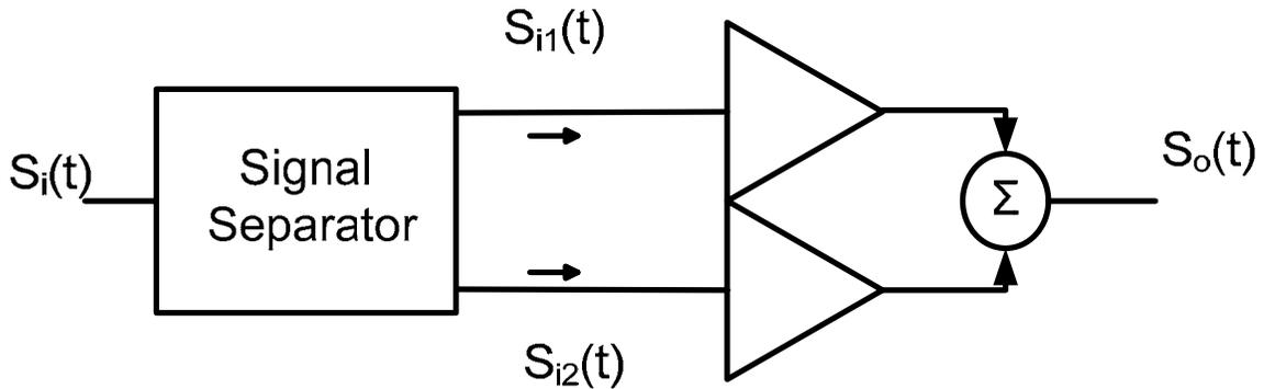
Figure 4.17: Simplified block diagram of an outphasing amplifier
