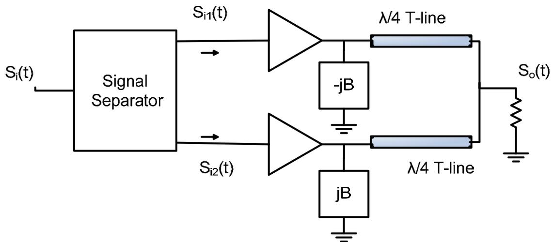
Figure 4.18: A Chireix's outphasing amplifier
