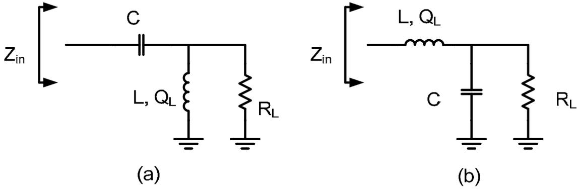
Figure 5.1: (a) A single stage “L-match” with a series capacitor and a parallel inductor; (b) A single stage “L-match” with a parallel capacitor and a series inductor
