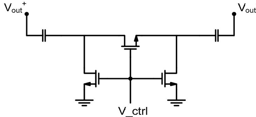
Figure 6.6: A switched capacitor array. This configuration takes advantage of differential operation to minimize switch losses without the need for large size switches.
