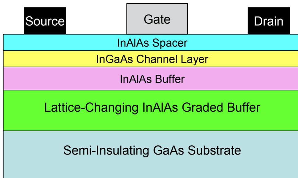
Figure 3.5 An InGaAs MHEMT cross-section
