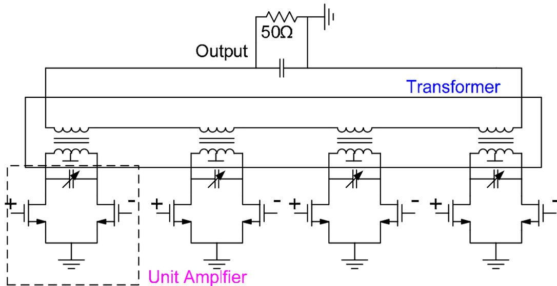
Figure 6.12: The simplified schematic of the prototype.
