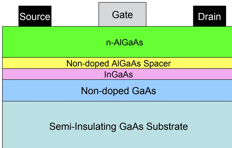
Figure 3.4: An InGaAs PHEMT cross-section
