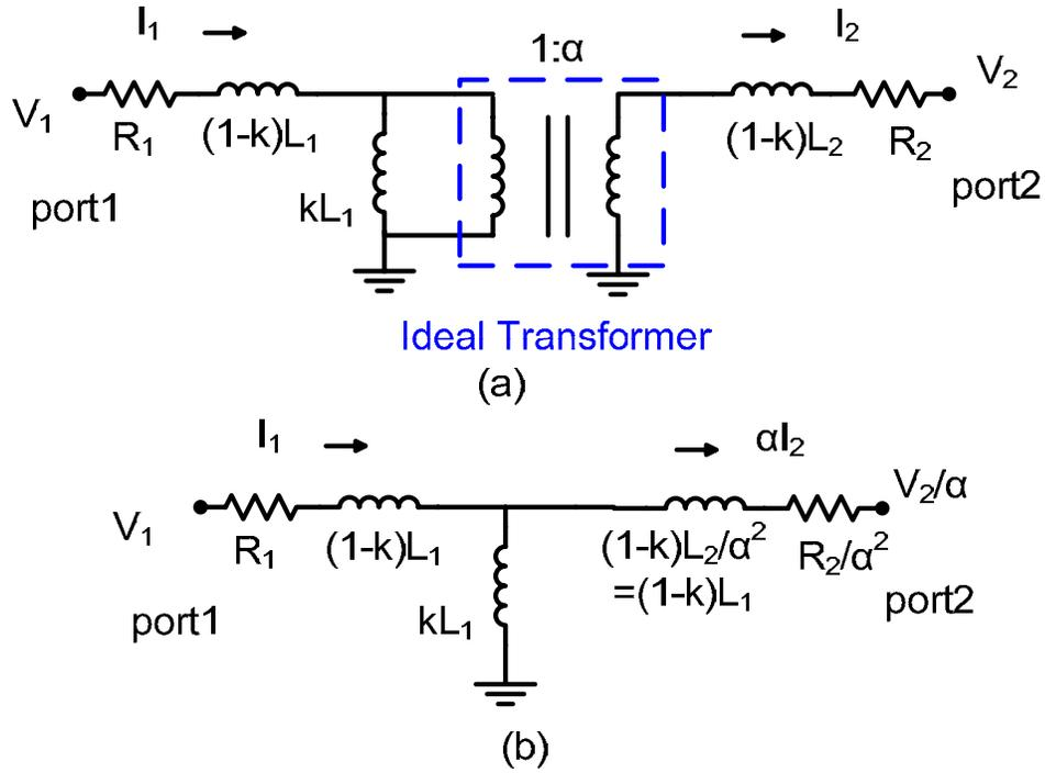
Figure 5.6: (a) Transformer model with leakage and magnetizing inductance; (b) Equivalent T-model
