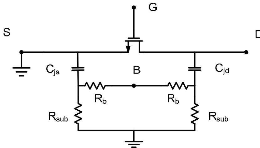
Figure 6.3: A device model of a common-source NMOS transistor with a simple substrate network.  $C_{js}$  and  $C_{jd}$  are junction capacitance of source and drain respectively.  $R_b$  is the effective body resistance.  $R_{sub}$  represents substrate resistance.
