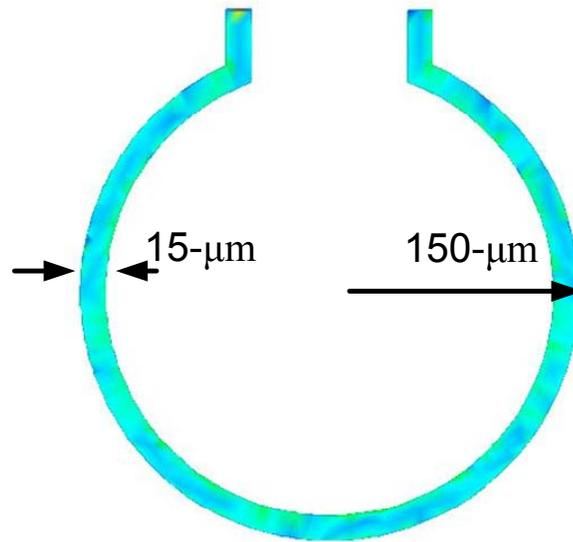
Figure 5.15: Current density of a circular single-turn inductor (top view)
