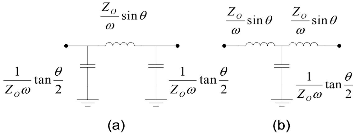
Figure 4.8: Lumped equivalent circuits of transmission lines, (a) “ $\pi$ ” configuration; (b) “T” configuration
