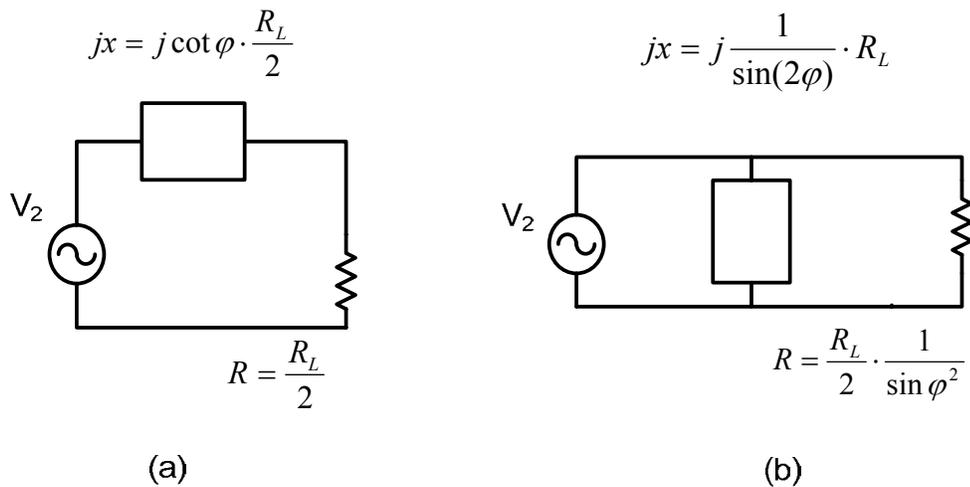
Figure 4.22: (a) RF load seen by the RF generator  $V_2$ ; (b) A parallel equivalent model
