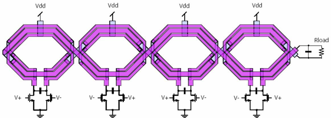
Figure 5.23: A power amplifier with “figure 8” transformer power combiner [5.8]
