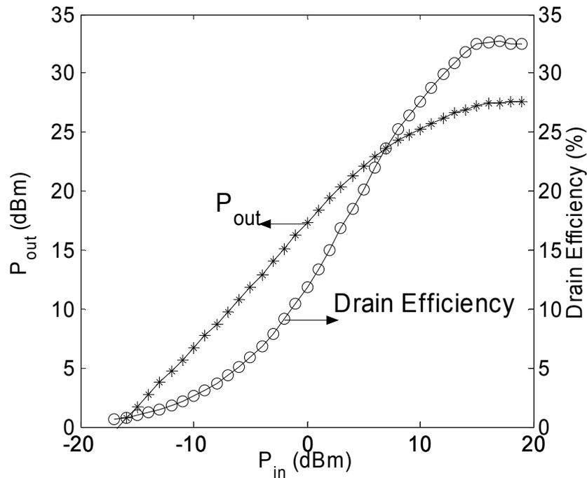
Figure 6.19: Measured output power and drain efficiency from single-tone test.
