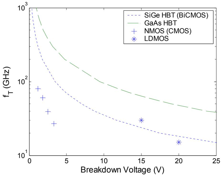
Figure 3.13: Comparison of breakdown voltages of different technologies. SiGe HBT and GaAs HBT are calculated from Johnson limit. NMOS breakdown voltages are taken from recommended supply voltage published on ITRS website. LDMOS breakdown voltages are taken from foundry online data provided by Jazz Semiconductors.
