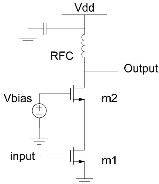
Figure 4.1: The cascode configuration with two NMOS transistors
