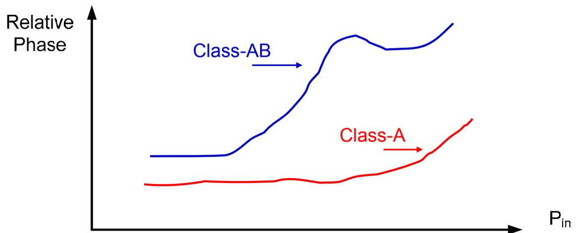
Figure 2.9 Conceptual AM-PM for different bias conditions
