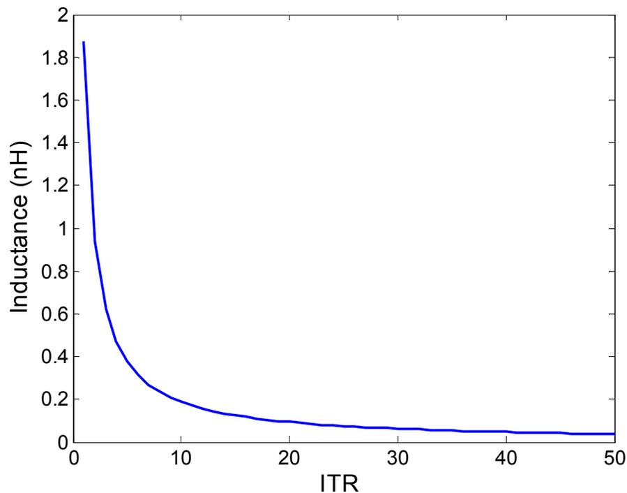
Figure 5.10: The required primary inductance for maximum efficiency vs. ITR (when  $\omega = 2$ -GHz,  $Q_1 = Q_2 = 10$ ,  $k = 0.7$ ,  $R_L = 50$ - $\Omega$ )
