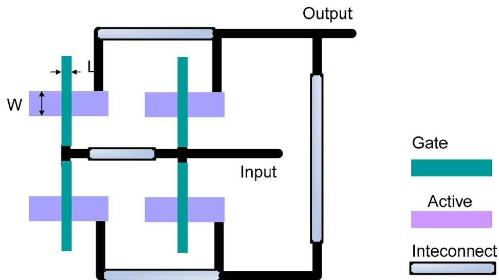
Figure 6.8: A conventional transistor layout. Note that the unequal delay among unit transistors leads to performance degradation.
