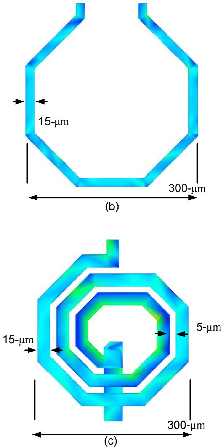
Figure 5.14: Current densities of three inductors implemented in the same technology with equal width: (a) Top view of the micro-strip line inductor; (b) Top view of the single-turn inductor; (c) Top view of the multi-turn inductor
