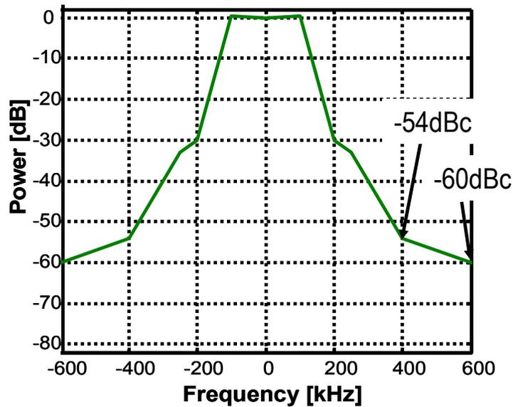
Figure 2.10: GSM-EDGE spectral mask
