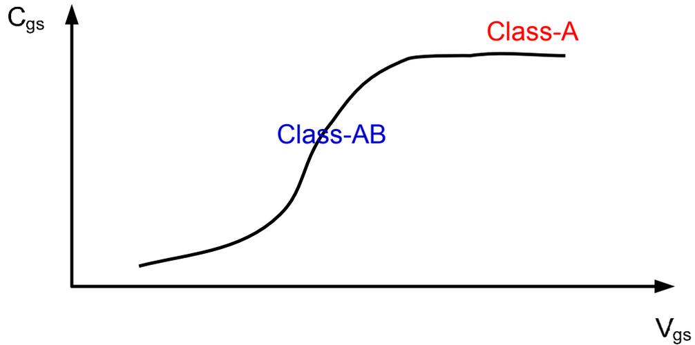
Figure 2.8:  $C_{gs}$  characteristic of typical NMOS devices vs.  $V_{gs}$
