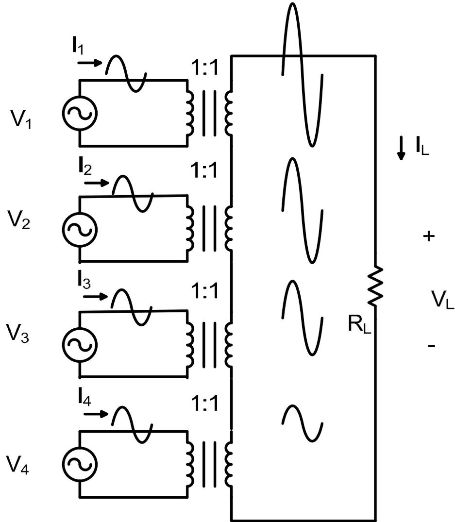
Figure 4.12: A four-way power combining transformer composed of 4 unity transformers
