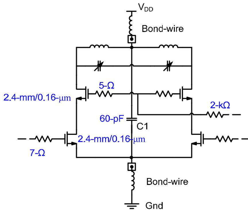
Figure 6.14: The simplified schematic of each unit amplifier.
