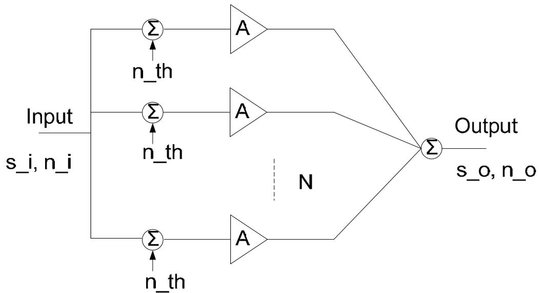
Figure 4.14: A simplified equivalent model for an N-way power combining PA with additive noise
