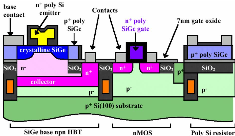
Figure 3.8: Diagram of SiGe HBT based BiCMOS by IBM
