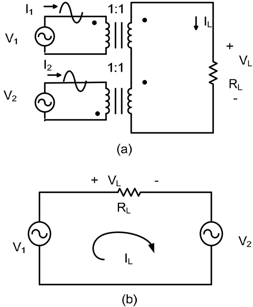
Figure 4.19: (a) An outphasing amplifier with the proposed power combiner; (b) An equivalent model of the outphasing amplifier
