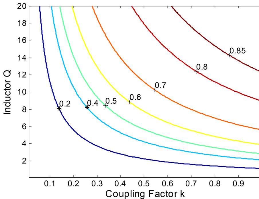
Figure 5.8: Power efficiency contour plot of a 1:n transformer, assuming  $Q_1 = Q_2$
