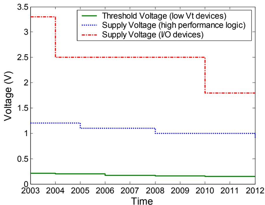
Figure 3.17: Scaling of supply voltages and threshold voltage for analog/RF circuits
