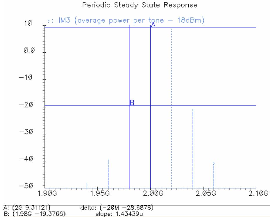
Figure 6.18: Two tone simulation results when all unit amplifiers are on. The simulation is performed when output power per tone is 18dBm (around 9dBv with 50 ohm reference). Note that the imbalance is mainly because input matching is not designed.
