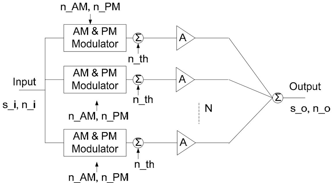
Figure 4.13: An equivalent model for an N-way power combining PA with additive noise<sup>30</sup>
