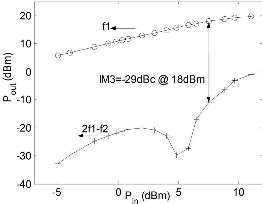
Figure 6.20: Measured output power and IM3 from a two-tone test (1-kHz tone spacing)
