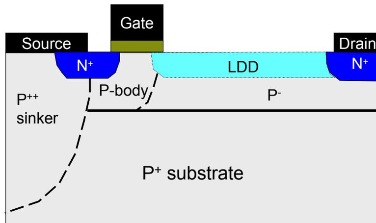
Figure 3.9: A LDMOS cross-section
