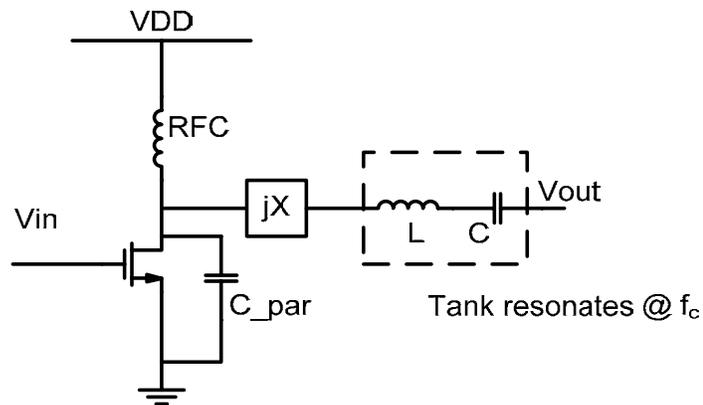
Figure 2.3: A simple class-E amplifier
