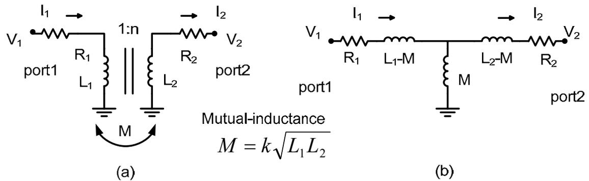
Figure 5.5: (a) Transformer model; (b) Transformer equivalent T-model
