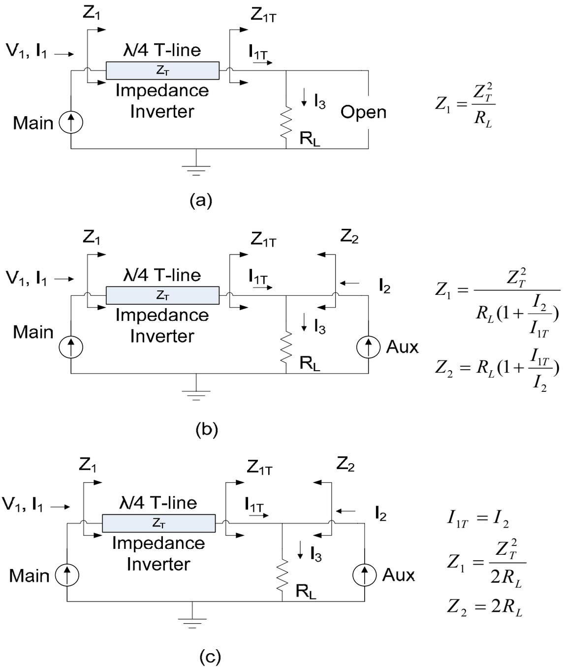
Figure 4.7: Operation of a Doherty amplifier, (a) low power mode; (b) medium-power mode; (c) peak-power mode
