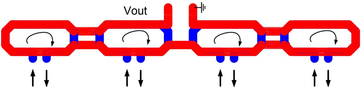
Figure 5.20: A power combining transformer with oval-like high-Q inductors
