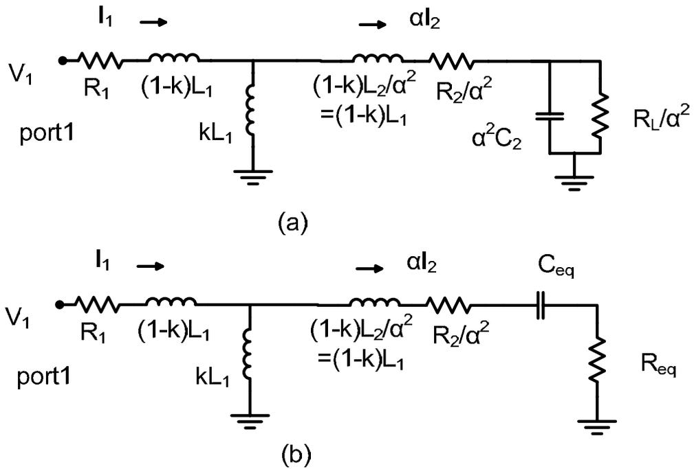
Figure 5.7: (a) Transformer equivalent T-model with a load resistor and tuning capacitor<sup>46</sup>; (b) Transformer T-model after parallel to series conversion at the load
