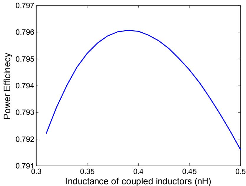
Figure 5.17: The variation of power efficiency vs. inductance of coupled inductors in the designed transformer
