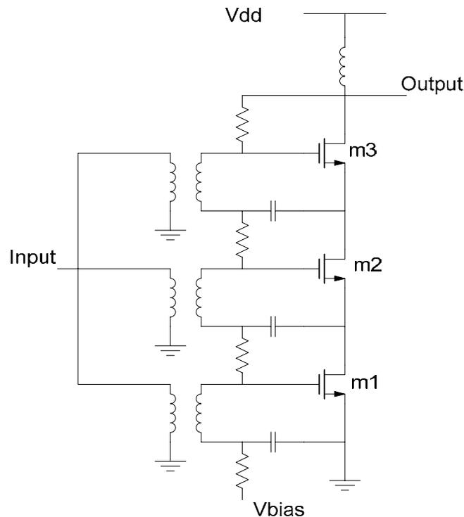
Figure 4.3: A three FET stacked power amplifier
