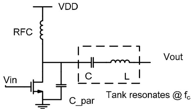
Figure 2.2: A voltage switching class-D amplifier
