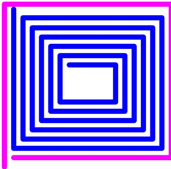
Figure 5.11: An on-chip transformer with high turn ratio formed by coupled inductors
