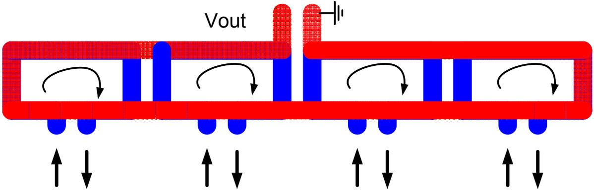
Figure 5.18: A simple power combining transformer. Some parts of primaries are not overlapped with the secondary which reduces coupling factor. Opposite currents flow in those parts of adjacent primaries. It reduces inductance and degrades Q.
