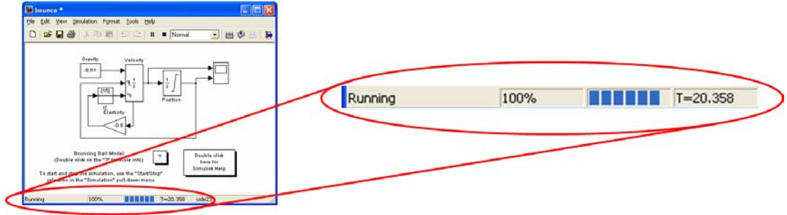
Figure 5.1: Zeno behavior that effectively makes a program (Matlab) halt.
