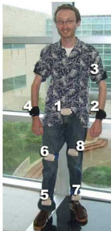
Fig. 1. A distributed wearable sensor network. The sensor on the right arm was malfunctioned during the experiment.
