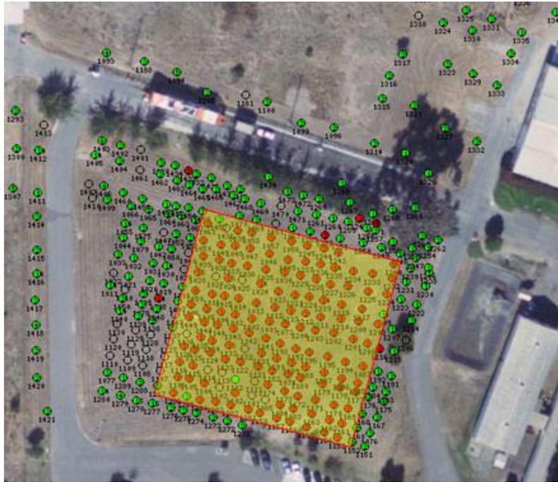
Figure 6.15: Sensor network deployment (not all deployed sensor nodes are shown). The disks and circles represent the positions of the sensor nodes. The network of 144 nodes used in the multi-target tracking and PEG experiments is highlighted.
