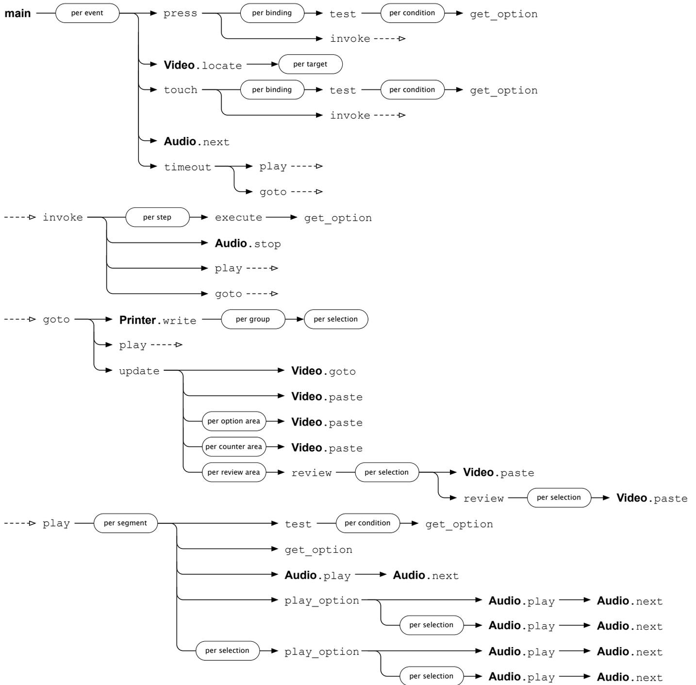
Figure 7.1: Call graph among Pvote routines, rooted from the event loop. Every use of iteration is indicated with a round bubble. Where a module name is not specified, the method belongs to **Navigator**.
