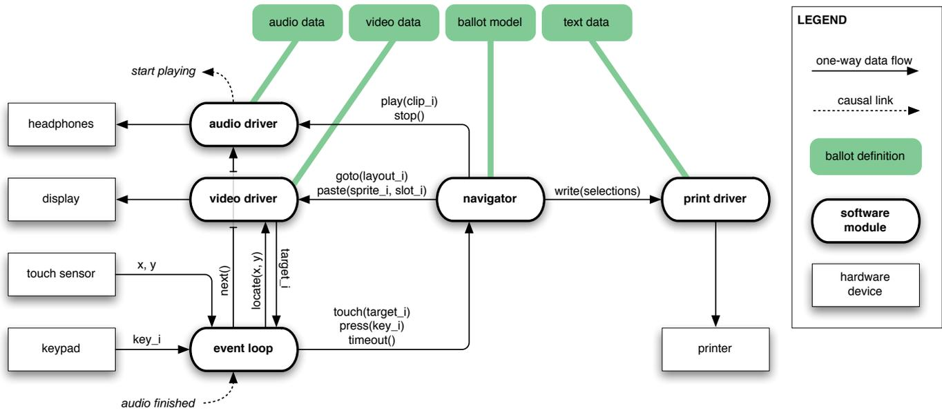
Figure 6.1: Block diagram of the virtual machine, which consists of the five software modules in bold. The arguments `clip_i`, `layout_i`, `sprite_i`, `target_i`, `key_i`, `x`, and `y` are integers; `selections` is a list of lists of integers.
