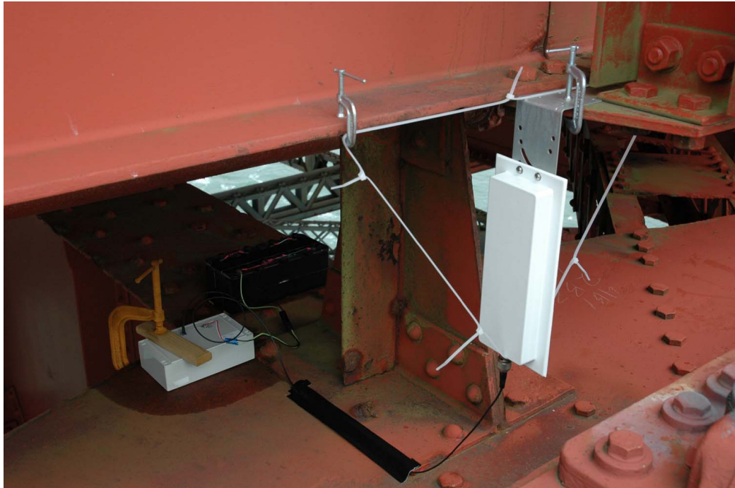
Figure 4.1. Board enclosure, antenna, and battery installed on the main span. The zip tie had to be put around the antenna to control wind vibration. Poor link quality was experienced with a vibrating antenna under strong wind. Corrosion of the C-clamp can be observed in the figure.
