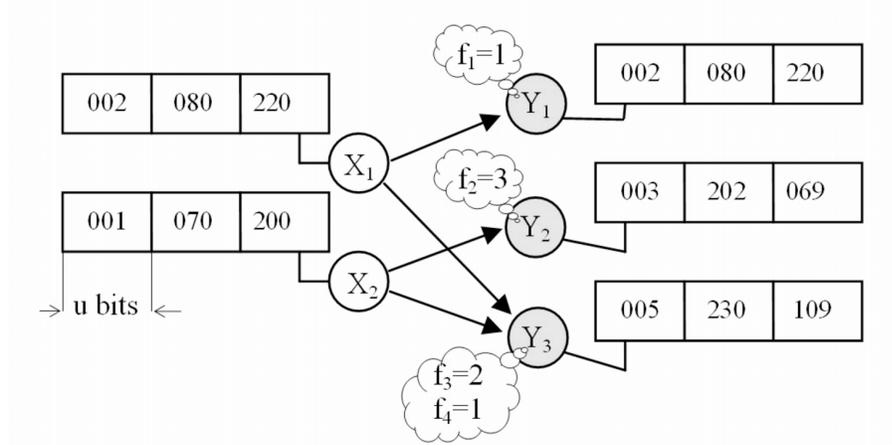
Figure 1.1: A simple example of a linear code over  $GF(2^8)$ . Here  $k = 2, n = 3, k/n = 2/3, q = 256$ . The primitive polynomial of the field is  $D^8 + D^4 + D^3 + D^2 + 1$ . Arithmetic is done by representing numbers as binary coefficients of polynomials and doing polynomial operations modulo the primitive polynomial. For example,  $70 \times 3 \rightarrow (D^6 + D^2 + D) \times (D + 1) = D^7 + D^6 + D^3 + D \rightarrow 202$ .
