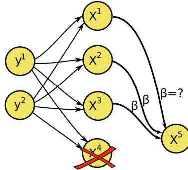
Figure 3.1: The repair problem: Assume that a  $(4,2)$  MDS erasure code is used to generate 4 fragments (stored in nodes  $x^1, \dots, x^4$ ) with the property that any 2 can be used to reconstruct the original data  $y^1, y^2$ . When node  $x^4$  fails, and a newcomer  $x^5$  needs to generate an erasure fragment from  $x^1, \dots, x^3$ , what is the minimum amount of information that needs to be communicated?
