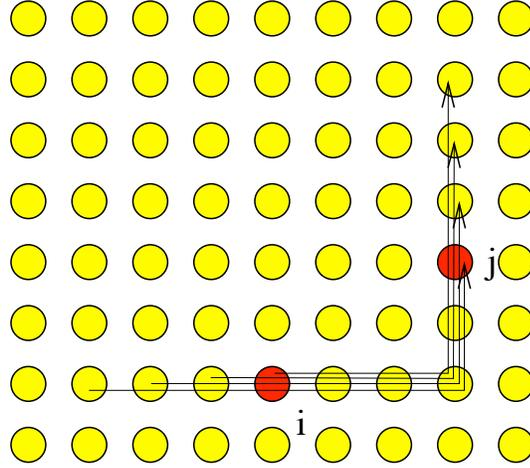
Figure 5.7: Counting the number of routes of length  $\ell = 9$  nodes, in the case where  $\ell_{ij} = 5$ . There are  $\ell - \ell_{ij} = 9 - 5 = 4$  possible routes with exactly  $\ell$  nodes going through node  $i$  then through node  $j$ . We admit only routes going horizontally first then vertically.
