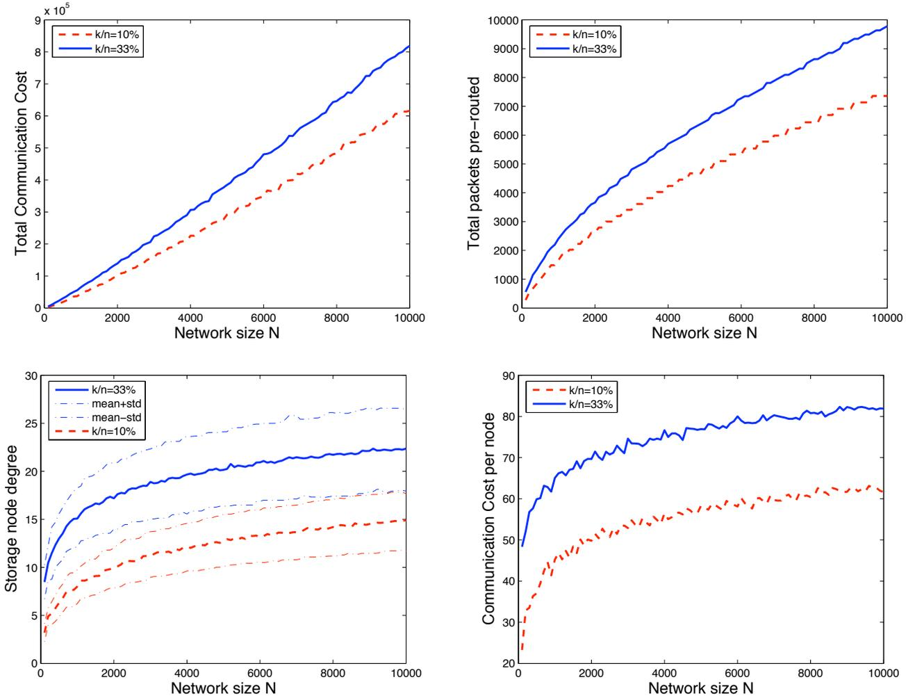
Figure 2.6: Experiments for perimetric storage scenario. For each subgraph, we plot  $k/n = 10\%$  (so  $k = 0.4\sqrt{N}$ ) and  $k/n = 33\%$  (so  $k = 4/3\sqrt{N}$ ). In both cases  $n = 4\sqrt{N}$
