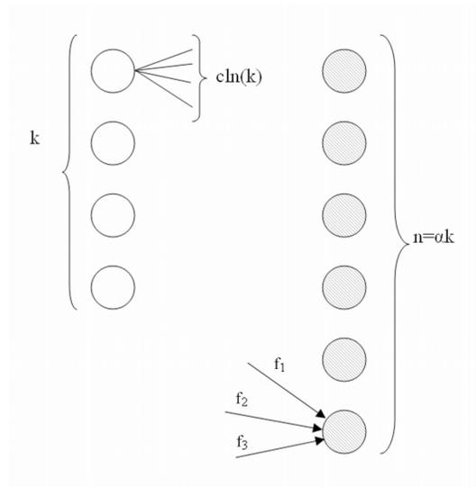
Figure 2.4: Decentralized erasure codes construction. There are  $d(k) = c \ln(k)$  edges starting from each data node and landing independently and uniformly on the storage nodes.
