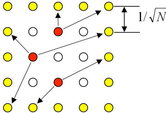
Figure 2.5: Perimetric storage: The  $n = 4\sqrt{N}$  nodes on the perimeter are used as storage, and  $k = O(\sqrt{N})$  nodes inside the grid are the data nodes.
