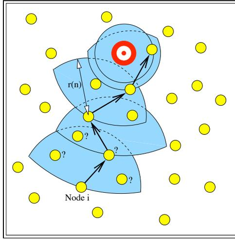
Figure 5.1: Random greedy routing. Node  $i$  has to choose the following node in the route among the nodes that are his neighbors (inside the ball of radius  $r(n)$  centered in node  $i$ ) *and* that are closer to the target than  $i$  (inside the ball of radius centered in the target, where  $d$  is the distance between node  $i$  and the target). Next node is thus randomly chosen in the intersection of the two balls.
