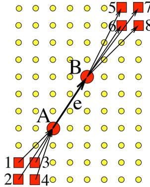
Figure 5.8: Number of paths including an edge  $e = (A, B)$  in the road map. Paths have two hops of equal length, where equality here is defined up to grid effects. Therefore, for a given edge  $e$ , there are at most 8 paths including  $e$ :  $(1, A, B)$ ,  $(2, A, B)$ ,  $(3, A, B)$ ,  $(4, A, B)$  and  $(A, B, 5)$ ,  $(A, B, 6)$ ,  $(A, B, 7)$ ,  $(A, B, 8)$ .
