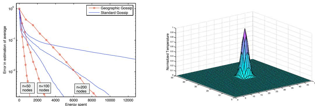
Figure 4.4: Estimation accuracy versus total spent energy for a field which is zero everywhere except in a sharp spike.
