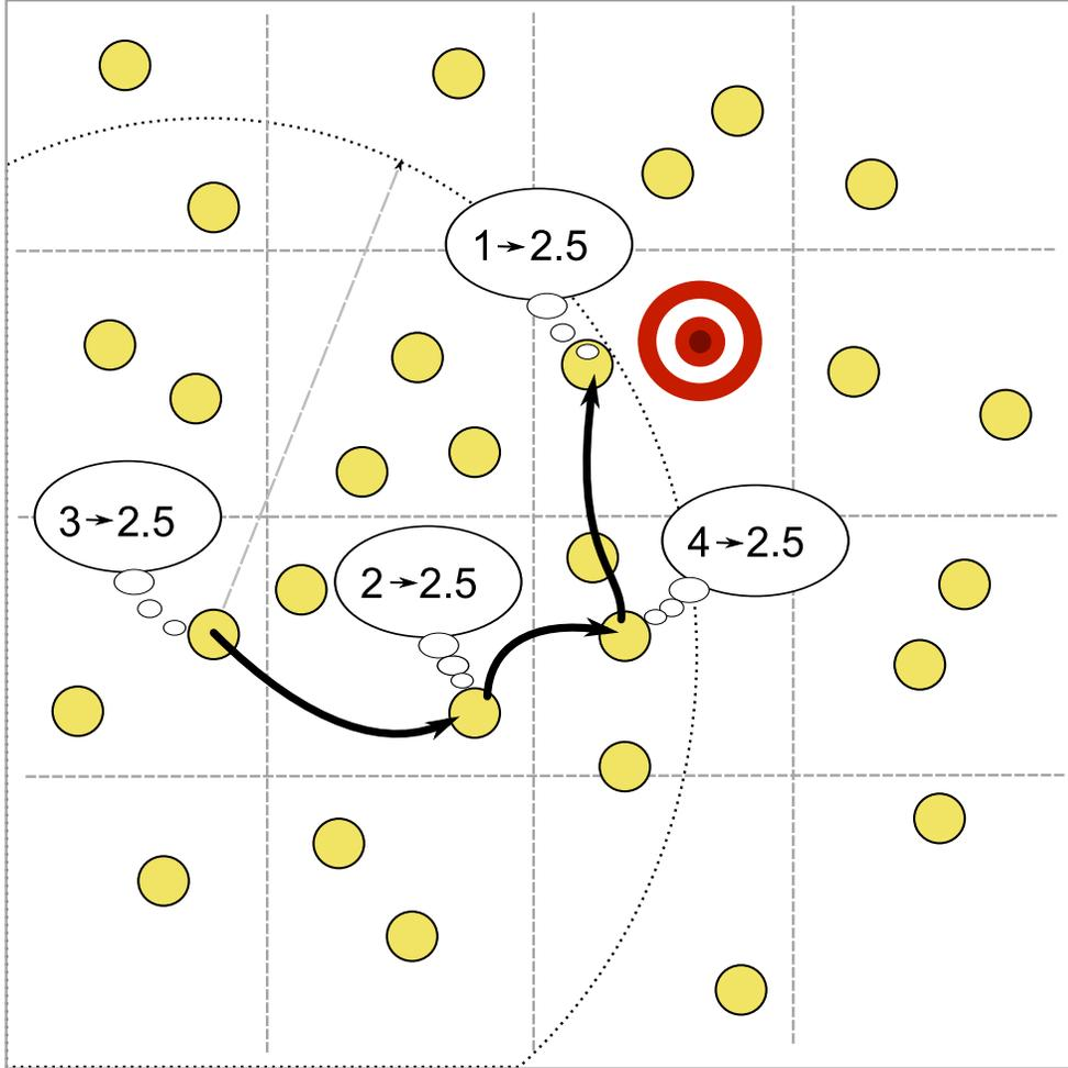
Figure 5.4: Example of box-path averaging: The node with initial value 3 selects a random position and places a target. Using  $(\leftrightarrow, \updownarrow)$ -box routing towards that target, all the nodes on the path replace their values with the average of the four nodes.
