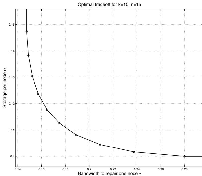
Figure 3.4: Optimal tradeoff curve between storage  $\alpha$  and repair bandwidth  $\gamma$ , for  $k = 5, n = 10$  (left) and  $k = 10, n = 15$  (right). For both plots  $\mathcal{M} = 1$  and  $d = n - 1$ . Note that traditional erasure coding corresponds to the points  $(\gamma = 1, \alpha = 0.2)$  and  $(\gamma = 1, \alpha = 0.1)$  for the top and bottom plots.
