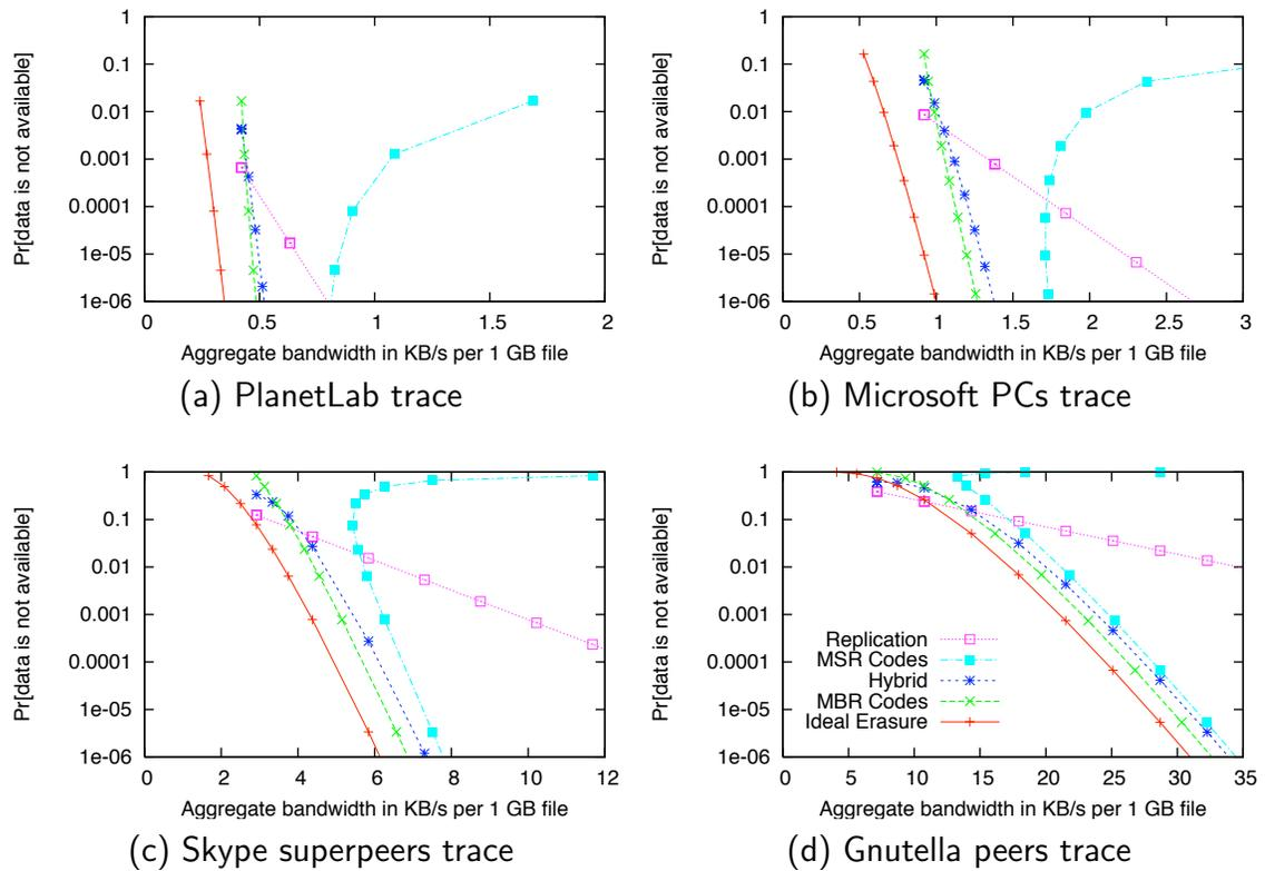
Figure 3.5: Availability-bandwidth tradeoff for  $k = 7$  with parameters derived from each of the traces. The key in (d) applies to all four plots.
