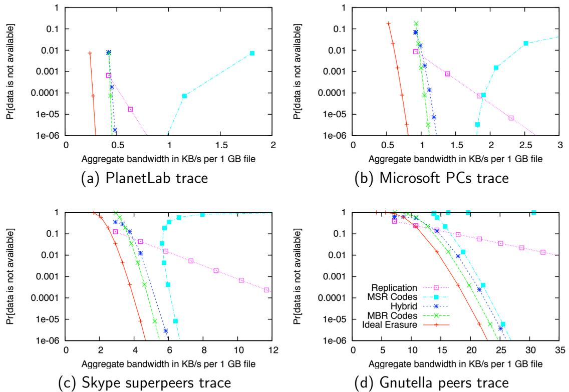
Figure 3.6: Availability-bandwidth tradeoff for  $k = 14$  with parameters derived from each of the traces.
