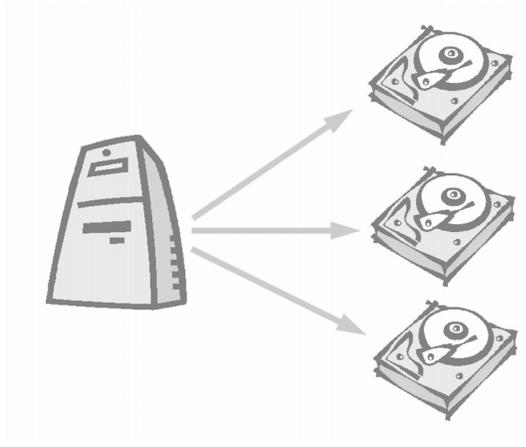
Figure 2.1: The classical distributed storage setup. Data which is initially centralized is encoded and stored in distributed storage nodes.
